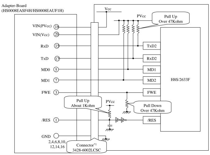
Setting the switches on the HS0008EASF4H on using H8S/2633F
