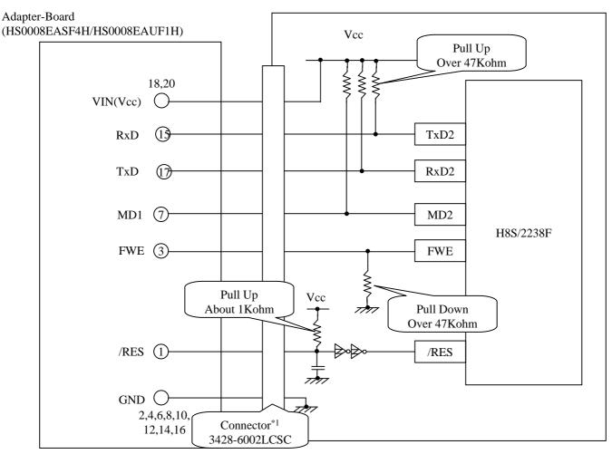
Setting the switches on the HS0008EASF4H on using H8/2238F
