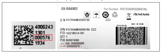
Figure 8. Identification of the Serial Number
