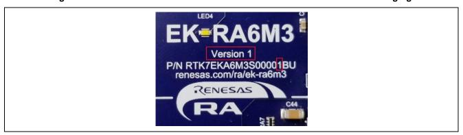
Figure 7. Identification of the Kit Version Number on the EK-RA6M3 Board
