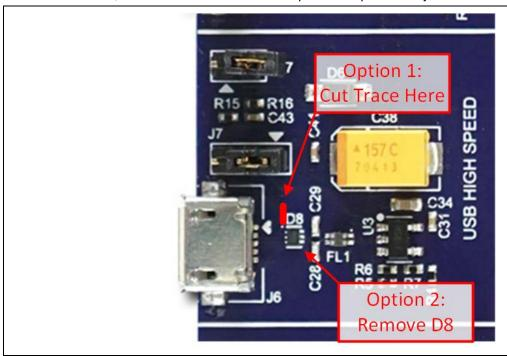
Figure 5. USB High Speed Rework Locations
