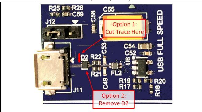
Figure 4. USB Full Speed Rework Locations
