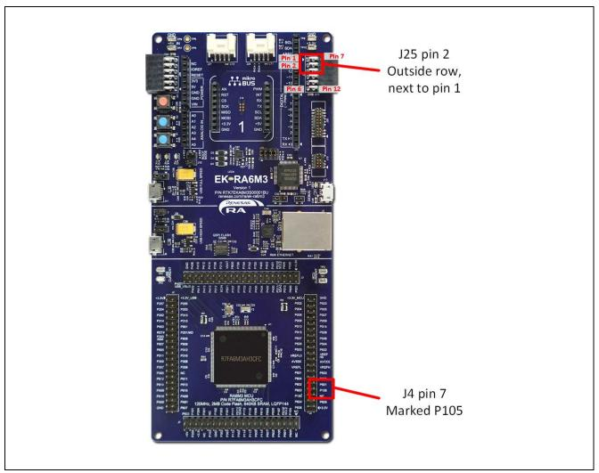
Figure 3. P105 Rework Pin Locations
