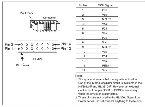
Figure 3.1 Pin Assignments of the Connector
