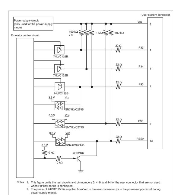
Figure 4.7 Interface Circuit in the E8a Emulator (Reference)
