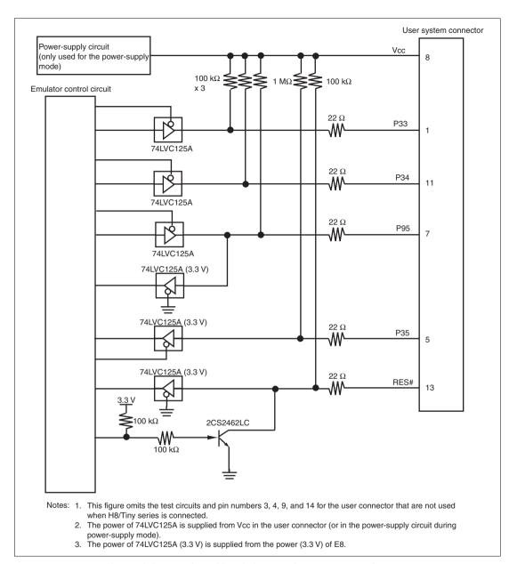
Figure 4.6 Interface Circuit in the E8 Emulator (Reference)
