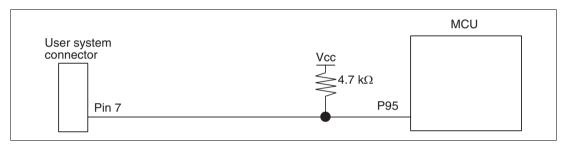
Figure 4.4 Connection of Emulator and Pin P95
