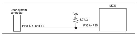
Figure 4.3 Connection of Emulator and Pins P33 to P35
