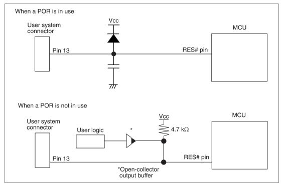
Figure 4.5 Examples of Reset Circuits
