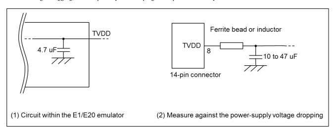
Figure 2-7 Circuit Configuration for Hot Plug-in
