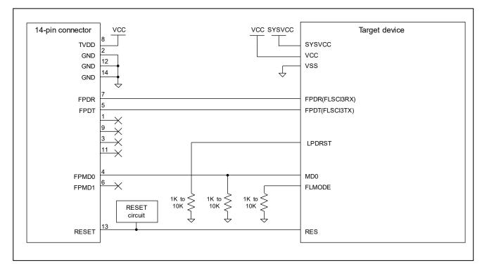
Figure 2-5 Example of Connection
