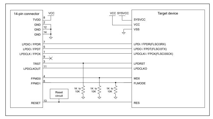
Figure 2-4 Example of Connection
