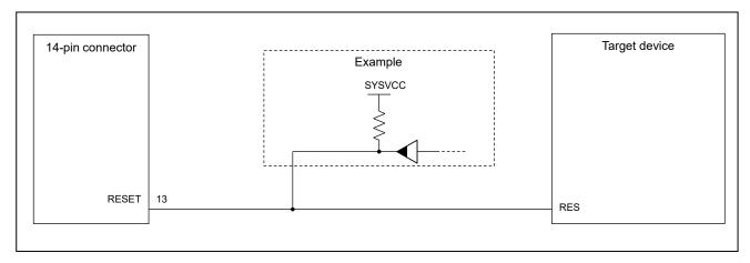
Figure 2-6 Example of Connecting a Reset Circuit
