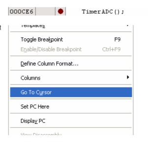
The code will run to the selected line and stop. A temporary breakpoint was automatically inserted in the code and then removed when the program stopped at the breakpoint.
