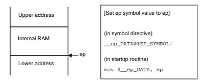
Figure 5-9. Example of ep Setting
