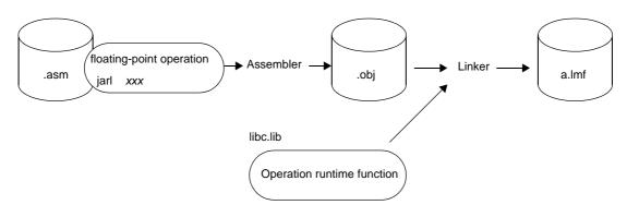
Figure 6-1. Image of Using Operation Runtime Function
