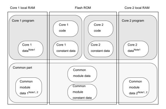
Figure 2-2. Sample Structure of a Multi-core Program
