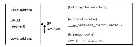
In the above example, the link directive is used to set so that the gp symbol value references the DATA1 segment. Since the gp symbol name is "\_\_gp\_DATA ", the address that is 32K-byte away from the start of the DATA1 segment which is determined when linking is set to the symbol "\_\_gp\_DATA" (see "Figure 5-6. Example of gp Setting (When Specifying Segment)").
