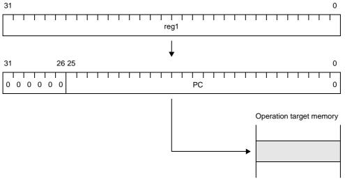
Figure 4-13. Register Addressing (JMP [reg1]) [V850E2]
