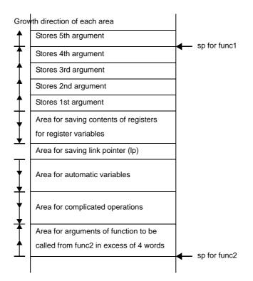
An example of a source calling a C function from a C function and an assembly source when that source is compiled is shown below.
