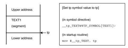
In the above example, the link directive is used to set so that the tp symbol value specifies the start of TEXT1 segment. Since the tp symbol name is "\_\_tp\_TEXT", the start address of TEXT1 segment which is determined when linking is set to the symbol "\_\_tp\_TEXT".
