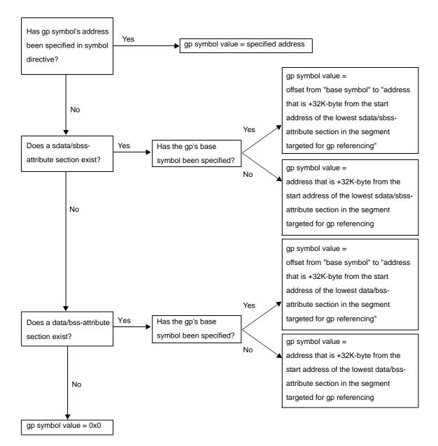
Figure 5-8. Rules for Determining Global Pointer Values
