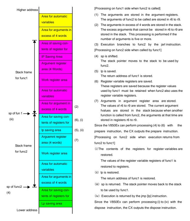
The items that are saved to the stack frame and the stack frame to be used are summarized below.
