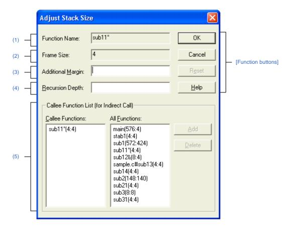
Figure A-51. Adjust Stack Size Dialog Box
