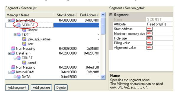
Figure 2-7. Segment Detail (When SCONST Is Selected)
