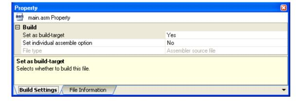
Figure A-13. Property Panel: [Build Settings] Tab (When Selecting Object Module File)
