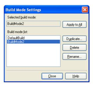
Select the build mode to be deleted from the build mode list and click the [Delete] button. The Message dialog box below will open.
