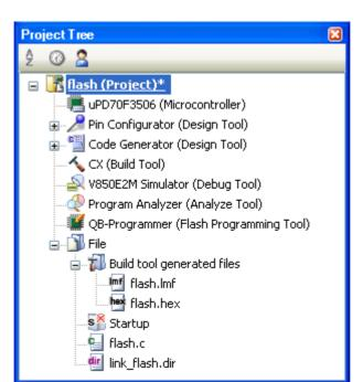
Figure 2-76. Generated Files for Flash Area
