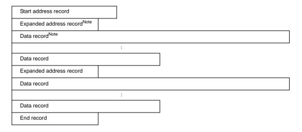
Note The expanded address record and data record are repeated.
