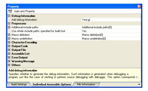
You can set assemble options for the assembler source file by setting the necessary properties in this tab.
