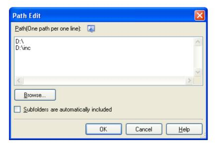
Enter the include path per line in [Path(One path per one line)].
