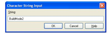
In the dialog box, enter the name of the build mode to be created and then click the [OK] button. The build mode with that name will be duplicated.
