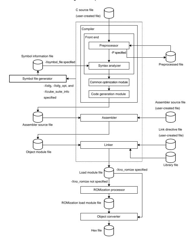
Figure B-1. Operation Flow of cx
