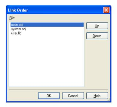
The names of the following files are listed in [File] in the order that the files are input to the linker.
