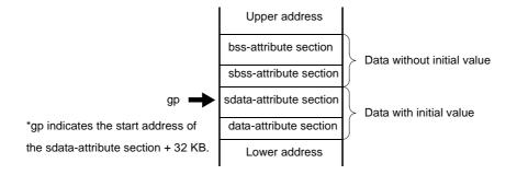
Therefore, the execution efficiency and object efficiency are enhanced if more data is allocated to the sdataattribute or sbss-attribute section, which can be accessed with a single instruction.
