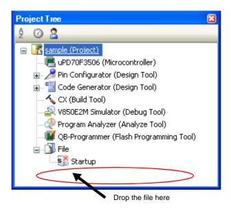
Caution To add other than the standard startup routine, drop the file onto the Startup node.
