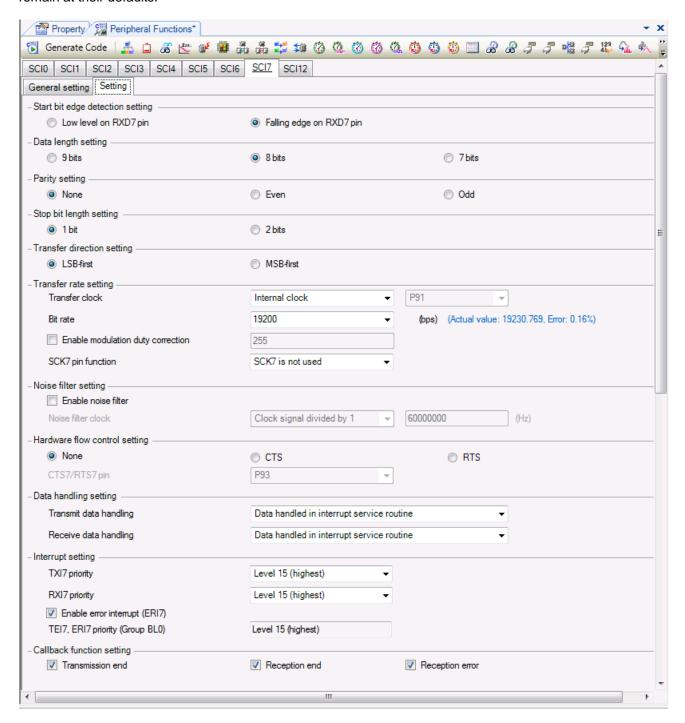
Figure 4-12 SCI7 Asynchronous Setting
