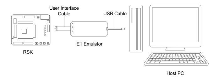
Figure 4-2: Debugger Connection Diagram
