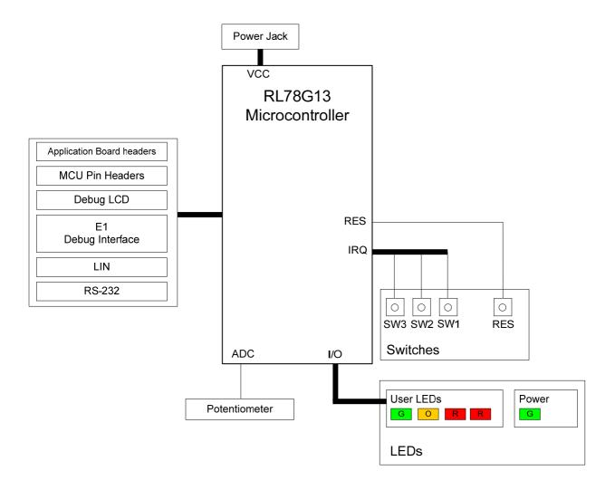
Figure 4-1: Internal RSK Block Diagram
