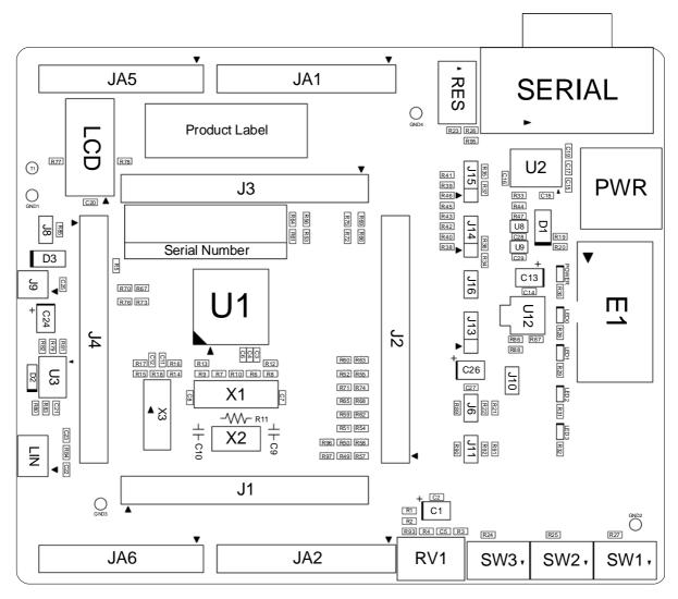
Figure 3-3: Top-Side Component Placement
