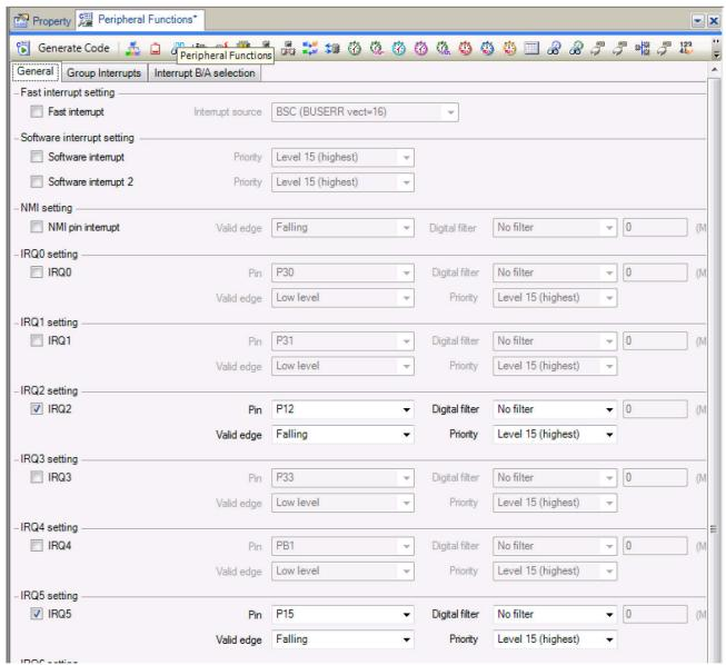
Figure 4-3 Interrupt Functions tab
