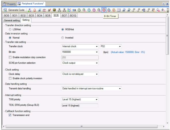
Figure 4-10 SCI6 SPI Master Setting
