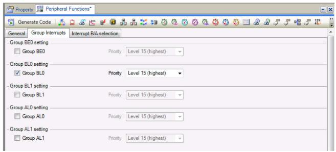
Figure 4-4 Group Interrupt Functions tab
