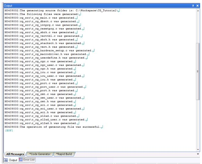
Figure 4-16 Code generator console
