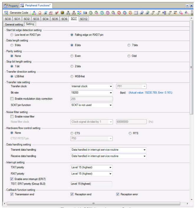
Figure 4-12 SCI7 Asynchronous Setting
