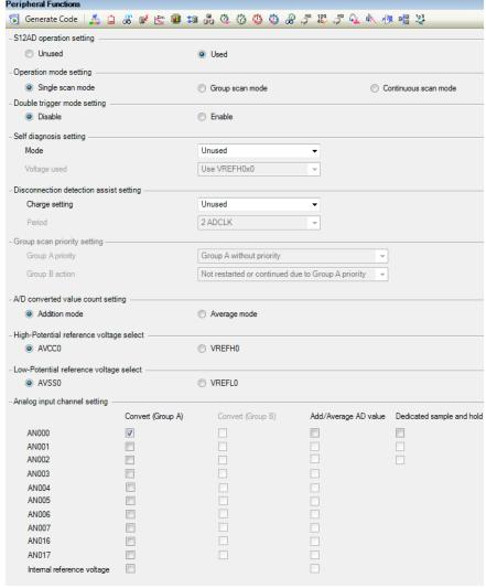
Figure 4-7 A/D Converter tab-1
