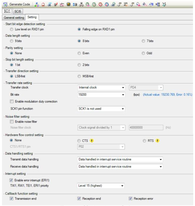
Figure 4-12 SCI1 Asynchronous Setting
