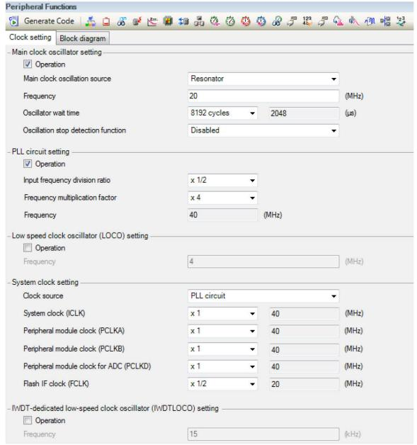
Figure 4-2 Clock setting tab
