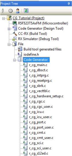
Figure 4-18 Code Generator Files in the Project Tree
