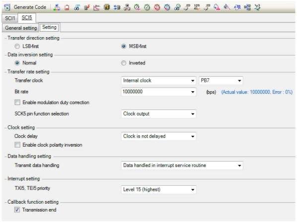
Figure 4-10 SCI5 SPI Master Setting
