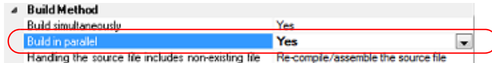
Figure 2.2 [Build in parallel] Property
