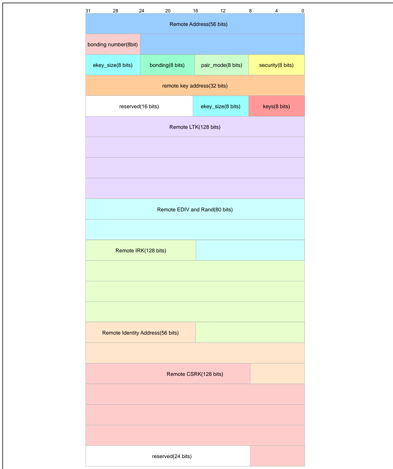
Figure 5.5. Remote device security data structure
