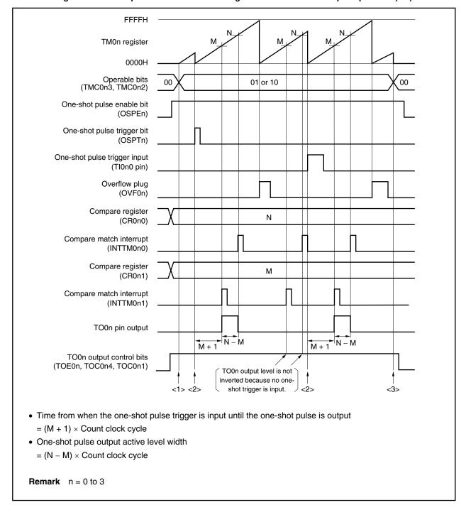
Figure 7-36. Example of Software Processing for One-Shot Pulse Output Operation (1/2)
