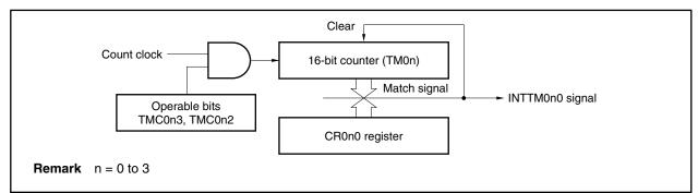
Figure 7-2. Block Diagram of Interval Timer Operation
