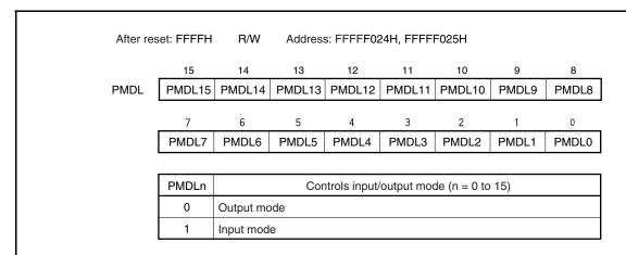
Remark The PMDL register can only be read or written in 16-bit units.
