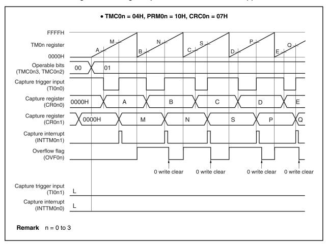
Figure 7-40. Timing Example of Pulse Width Measurement (2)
