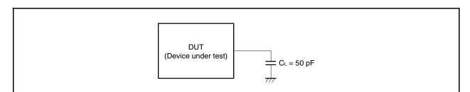
Caution If the load capacitance exceeds 50 pF due to the circuit configuration, reduce the load capacitance of the device to 50 pF or less by inserting a buffer or by some other means.
