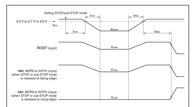
Caution Shifting to STOP mode and restoring from STOP mode must be performed at  $V_{DD} = 3.0 \text{ V}$  min. (fclk = 20 MHz) or  $V_{DD} = 2.7 \text{ V}$  min. (fclk = 10 MHz). Shifting to sub-STOP mode and restoring from sub-STOP mode must be performed at  $V_{DD} = 2.2 \text{ V}$  min. (fclk = 32.768 kHz).
