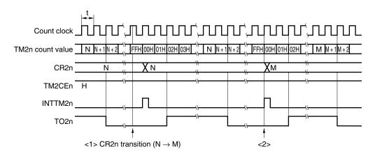
Caution In the case of read from the CR2n register between <1> and <2>, the value that is actually used differs (read value: M; actual value of CR2n register: N).
