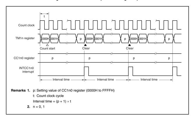
Figure 8-10. Interval Timer Operation Timing Example
