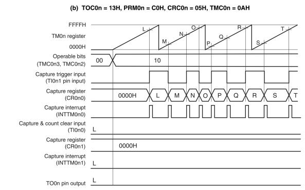
This is a timing example where an edge is not input to the Tl0n0 pin, in an application where the count value is captured to the CR0n0 register when the rising or falling edge of the Tl0n1 pin is detected.
