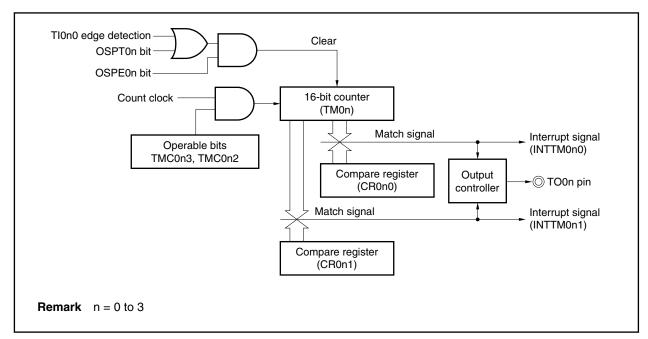
Figure 7-34. Block Diagram of One-Shot Pulse Output Operation
