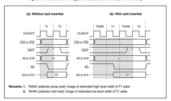
Figure 5-8. Address Wait Timing (Bus Read, Bus Size: 16 Bits, 16-Bit Access)
