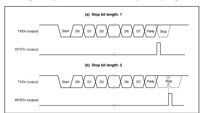
Figure 14-3. Asynchronous Serial Interface Transmission Completion Interrupt Timing
