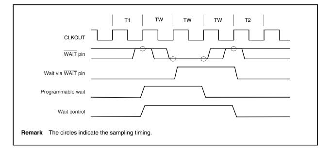
Figure 5-3. Example of Inserting Wait States
