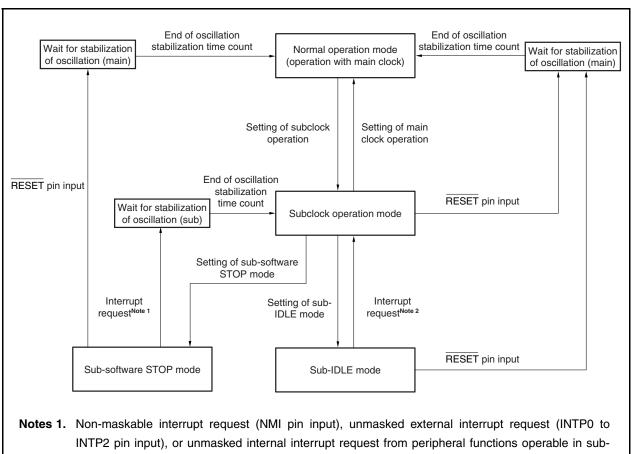
Figure 17-2. Status Transition (During Subclock Operation)
