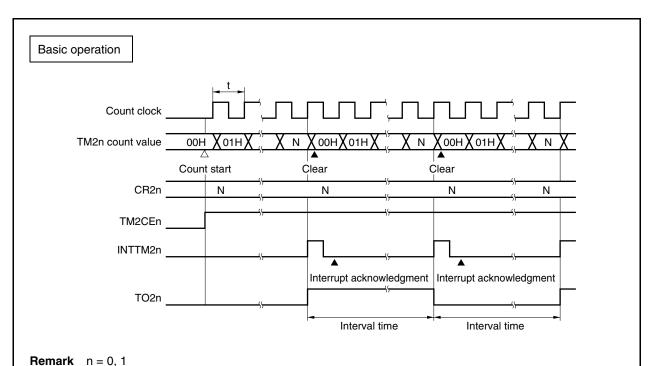
Figure 9-2. Timing of Interval Timer Operation (1/2)
