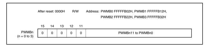
Caution To execute writing to the PWMBn register during PWMn operation, the access time is extended by a control action to synchronize the operation clock. How much the access time is to be extended differs depending on the specified PWMn operation clock. It is the shortest at 1  $\mu$ s (fxx = 20 MHz) when fxx is selected. The access time is lengthened as the operating clock frequency decreases, and the maximum access time is about 4  $\mu$ s (fxx = 20 MHz) when fxx/32 is selected.
