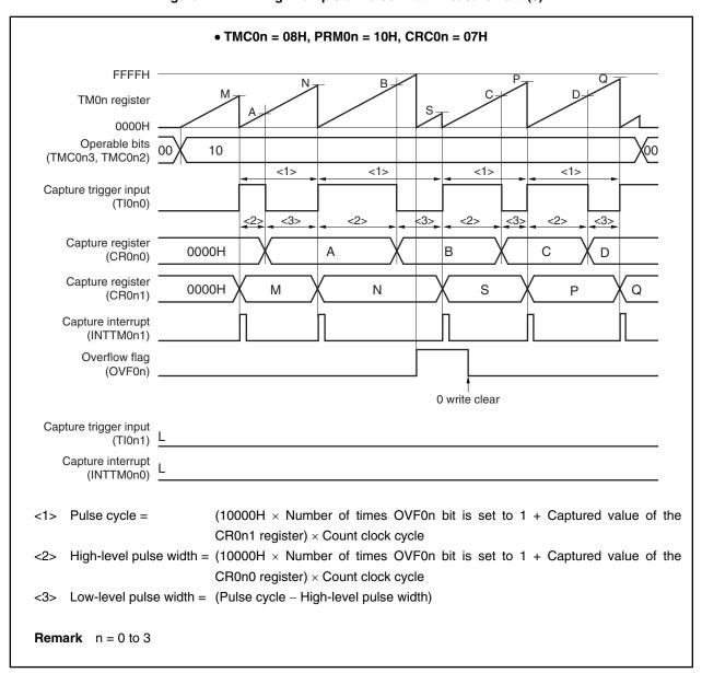
Figure 7-41. Timing Example of Pulse Width Measurement (3)
