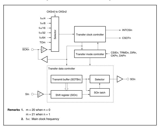
Figure 15-1. Clocked Serial Interface Block Diagram
