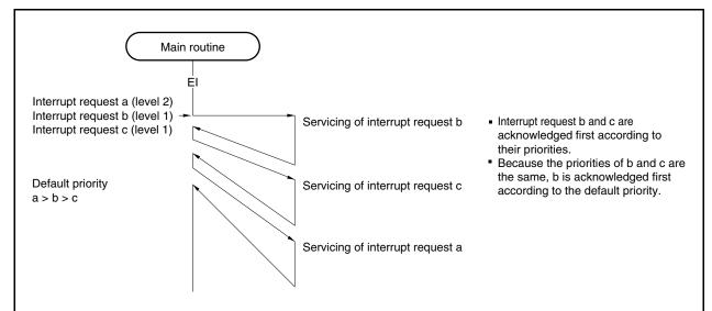
Caution To perform multiple interrupt servicing, the values of the EIPC and EIPSW registers must be saved before executing the EI instruction. When returning from multiple interrupt servicing, restore the values of EIPC and EIPSW after executing the DI instruction.
