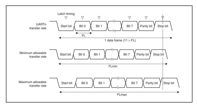
Figure 14-13. Allowable Baud Rate Range During Reception
