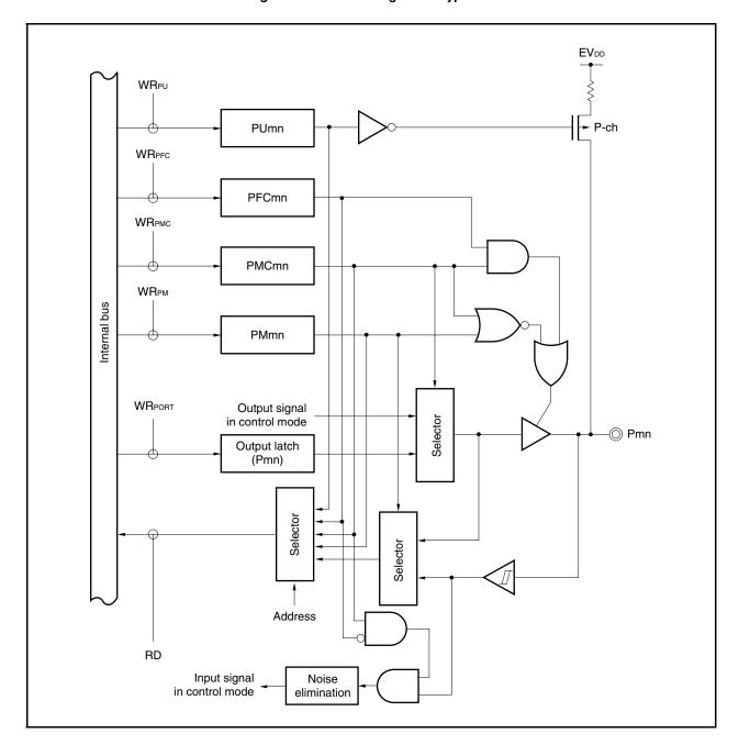
Figure 4-15. Block Diagram of Type D-2
