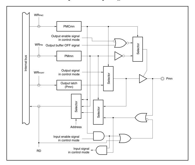
Figure 4-12. Block Diagram of Type C-1
