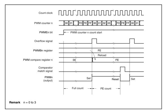
Figure 13-2. PWMn Operation Timing
