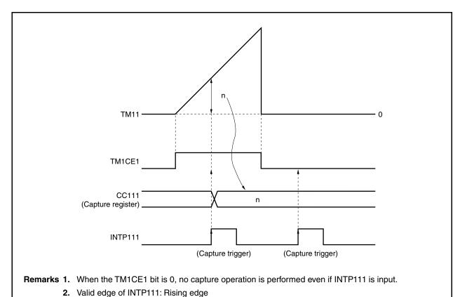
Figure 8-4. Capture Operation Example (TM11)
