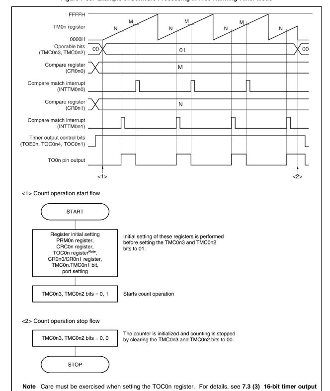
Figure 7-30. Example of Software Processing in Free-Running Timer Mode
