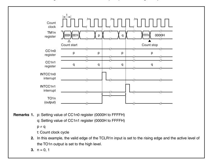
Figure 8-14. One-Shot Pulse Output Operation Timing Example
