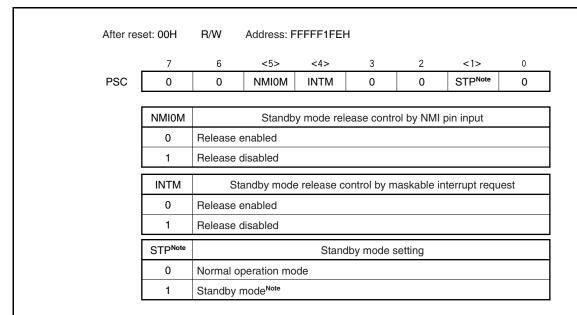
Note When setting software STOP mode, set the PSMR.PSM bit and then set the STP bit to 1.
