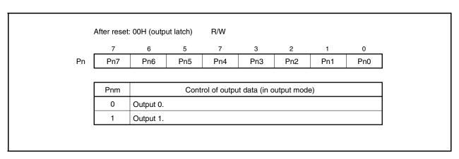
Writing to/reading from the Pn register is performed as follows regardless of the setting of the port n mode register (PMCn).
