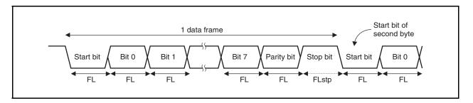
Representing the 1-bit data length by FL, the stop bit length by FLstp, and the base clock frequency by fcksr yields the following equation.
