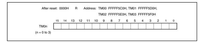
The count value of the TM0n register can be read by reading the TM0n register when the values of the TMC0n.TMC0n3 and TMC0n.TMC0n2 bits are other than 00. The value of the TM0n register is 0000H if it is read when the TMC0n3 and TMC0n2 bits are 00.
