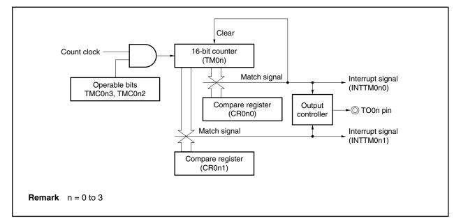
Figure 7-31. Block Diagram of PPG Output Operation
