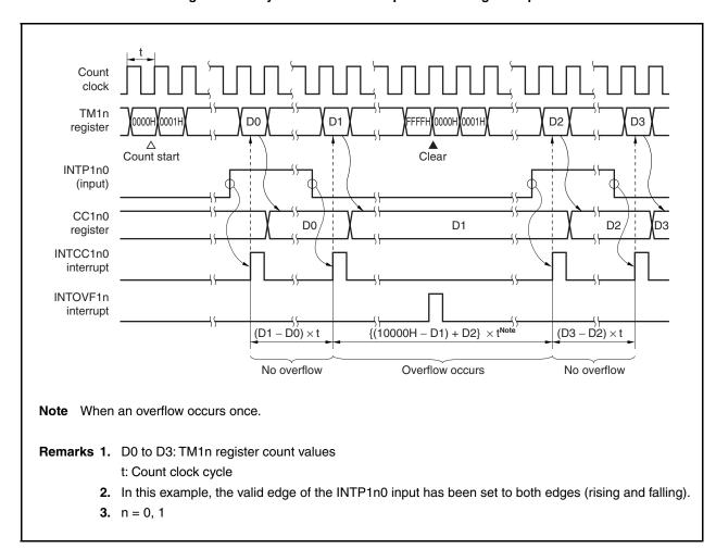
Figure 8-16. Cycle Measurement Operation Timing Example
