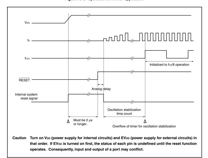
Figure 18-3. Operation on Power Application
