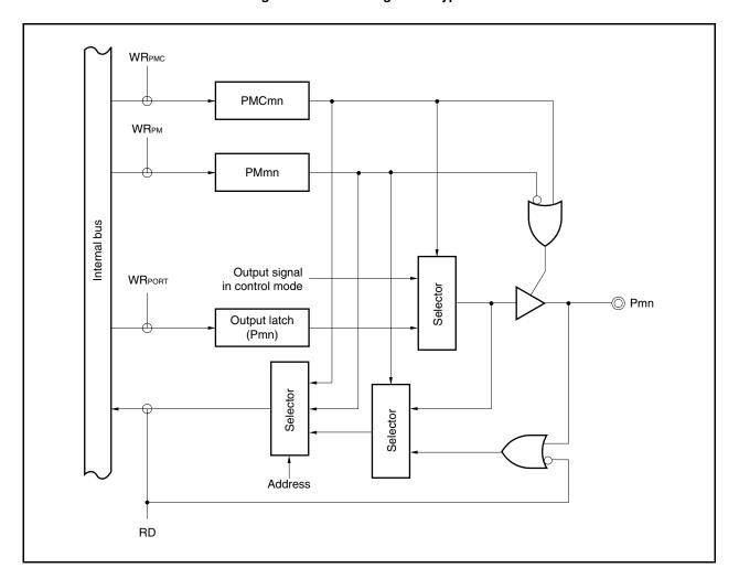
Figure 4-8. Block Diagram of Type B-1
