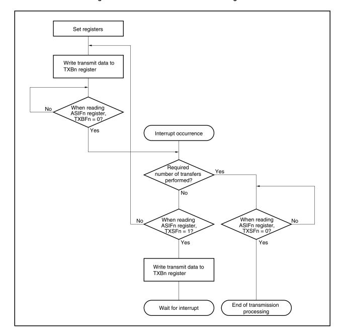
Figure 14-4. Continuous Transmission Processing Flow
