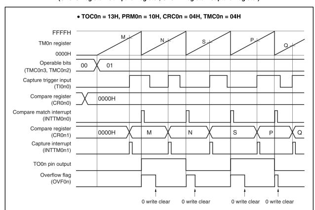
Figure 7-26. Timing Example of Free-Running Timer Mode (CR0n0 Register: Compare Register, CR0n1 Register: Capture Register)
