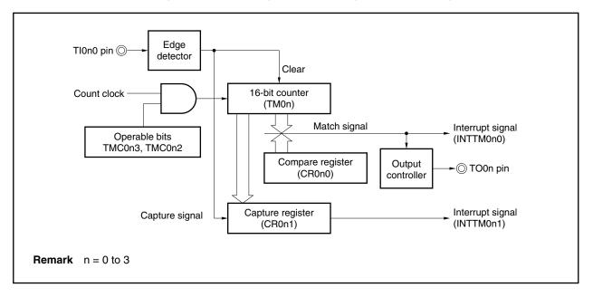
(a) TOC0n = 13H, PRM0n = 10H, CRC0n = 04H, TMC0n = 08H, CR0n0 = 0000H TM0n register 0000H Operable bits 10 00 (TMC0n3, TMC0n2) Capture & count clear input (TI0n0 pin input) Compare register 0000H (CR0n0) Compare match interrupt (INTTM0n0) Capture register 0000H S Ρ Q M Ν (CR0n1) Capture interrupt (INTTM0n1) TO0n pin output
