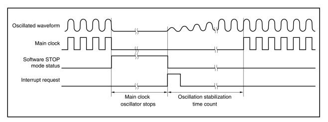
Figure 17-3. Oscillation Stabilization Time
