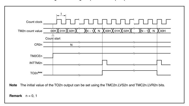
Figure 9-4. Timing of Square-Wave Output Operation
