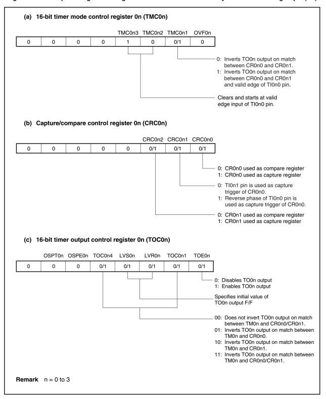
Figure 7-21. Example of Register Settings in Clear & Start Mode Entered by Tl0n0 Pin Valid Edge Input (2/2)
