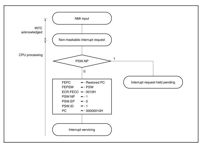
Figure 16-2. Servicing Configuration of Non-Maskable Interrupt
