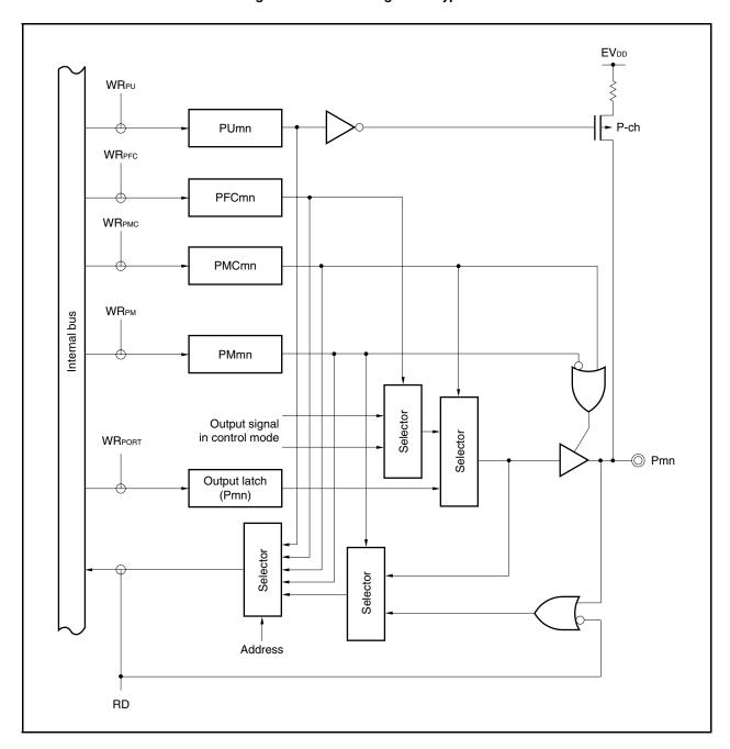
Figure 4-11. Block Diagram of Type B-4
