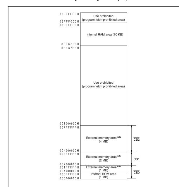
**Note** Each of these areas is a 512 KB space of 0100000H to 017FFFFH, 0200000H to 027FFFFH, or 0400000H to 047FFFFH (0180000H to 01FFFFFH, 0280000H to 03FFFFFH, and 0480000H to 07FFFFFH are an image).
