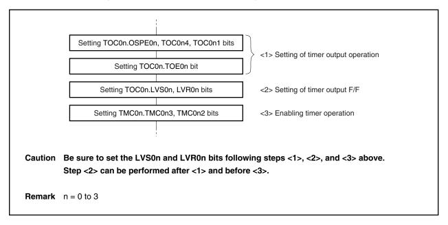
Figure 7-45. Timing Example of LVR0n and LVS0n Bits
