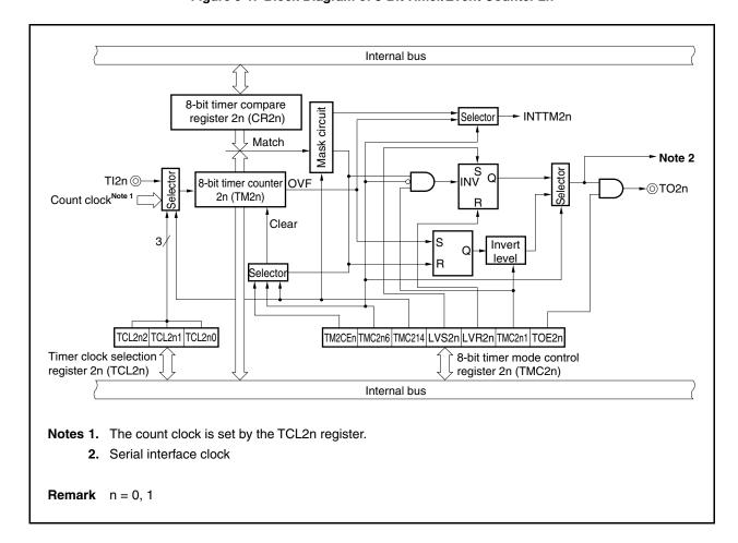
Figure 9-1. Block Diagram of 8-Bit Timer/Event Counter 2n
