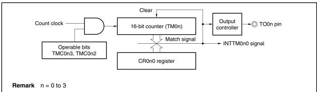
Figure 7-6. Block Diagram of Square Wave Output Operation
