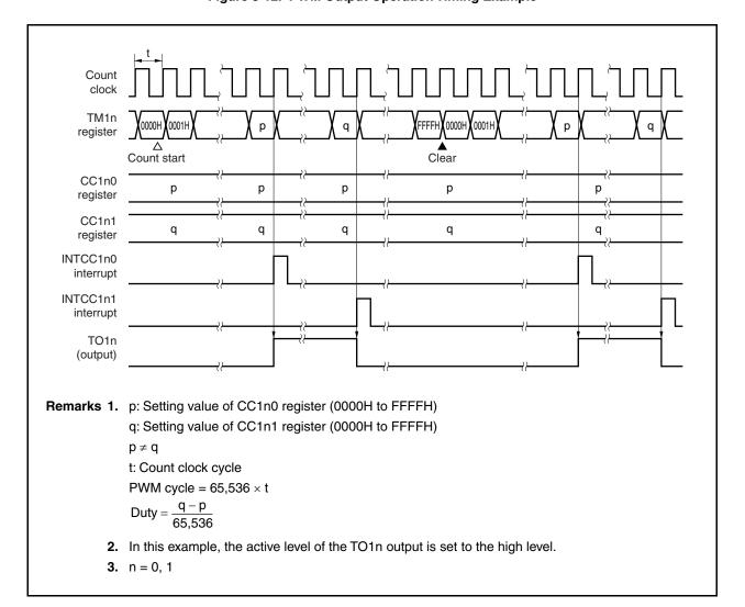
Figure 8-12. PWM Output Operation Timing Example
