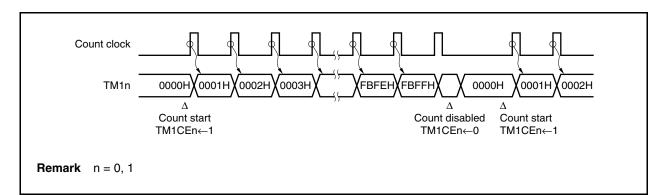
Figure 8-2. Basic Operation of 16-Bit Timer/Event Counter
