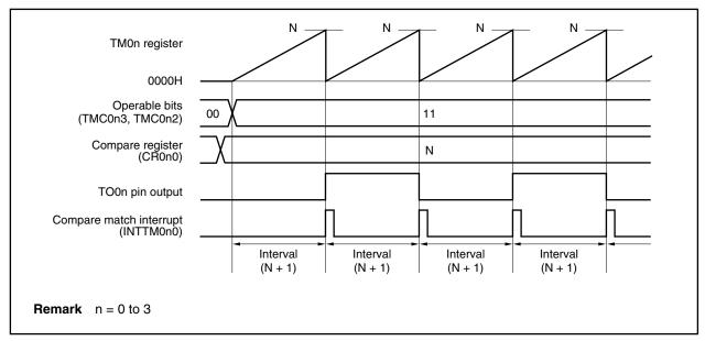
Figure 7-8. Example of Register Settings for Square Wave Output Operation
