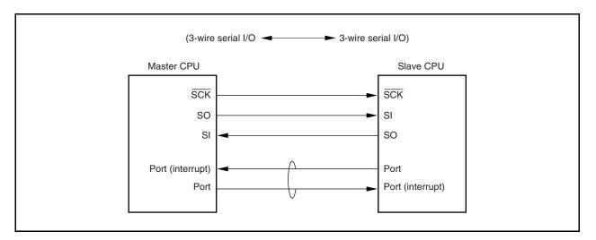
Figure 15-4. System Configuration Example of CSI
