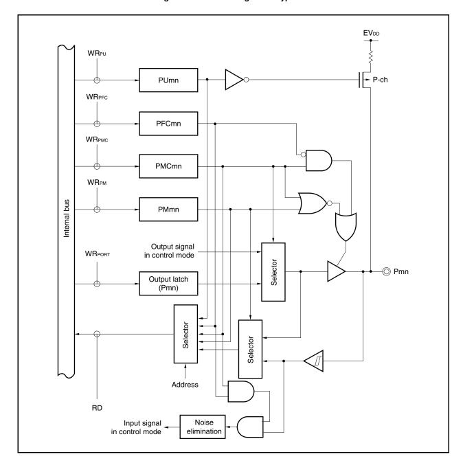
Figure 4-14. Block Diagram of Type D-1
