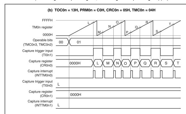
This is an application example where both the edges of the TI0n1 pin are detected and the count value is captured to the CR0n0 register in the free-running timer mode.
