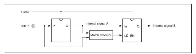
Figure 14-10. Noise Filter Circuit
