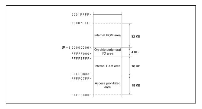
If R = r0 (zero register) is specified for the LD/ST disp16 [R] instruction, a range of addresses 00000000H  $\pm 32$  KB can be addressed by sign-extended disp16. All the resources of the internal hardware can be addressed by one pointer.
