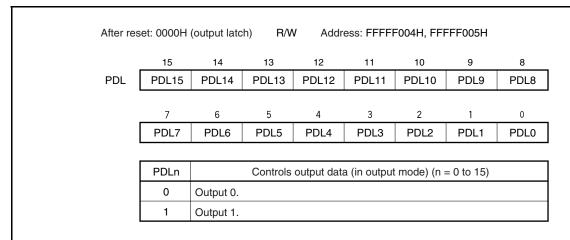
Remark The port DL register (PDL) can only be read or written in 16-bit units.
