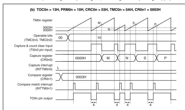
Figure 7-18. Timing Example of Clear & Start Mode Entered by Tl0n0 Pin Valid Edge Input (CR0n0 Register: Capture Register, CR0n1 Register: Compare Register) (2/2)
