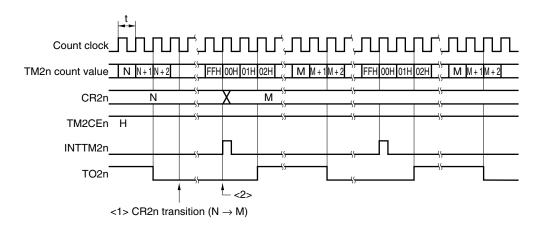
When the value of the CR2n register changes from N to M after the rising edge of the FFH clock
