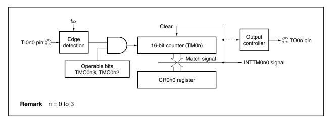
Figure 7-10. Block Diagram of External Event Counter Operation
