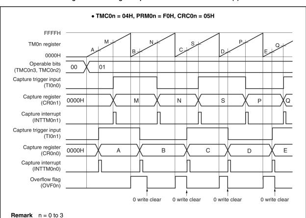
Figure 7-39. Timing Example of Pulse Width Measurement (1)
