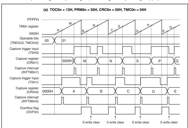
Figure 7-28. Timing Example of Free-Running Timer Mode (CR0n0 Register: Capture Register, CR0n1 Register: Capture Register) (1/2)
