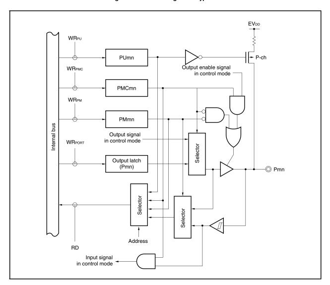
Figure 4-13. Block Diagram of Type C-2
