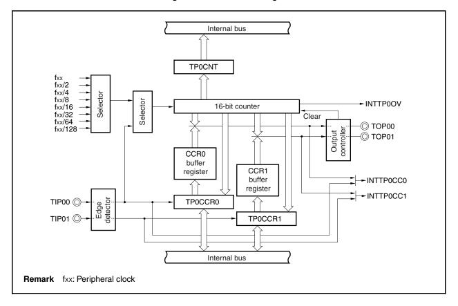
Figure 6-1. TMP0 Block Diagram
