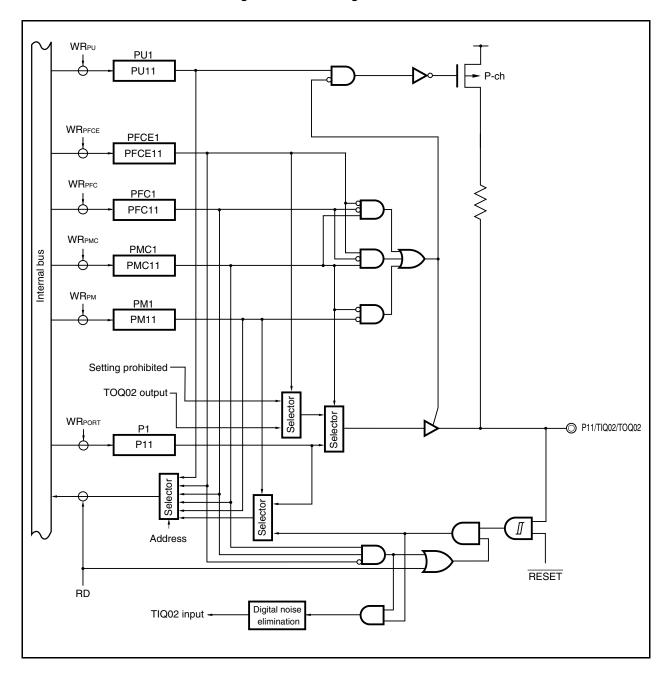
Figure 4-6. Block Diagram of P11 Pin
