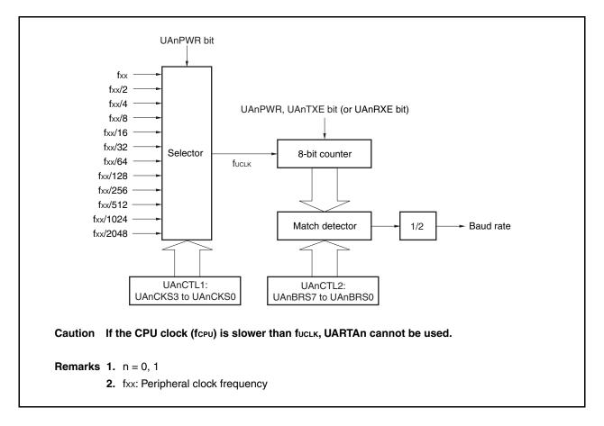
Figure 12-9. Configuration of Baud Rate Generator
