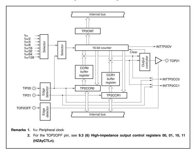
Figure 6-3. TMP2 Block Diagram
