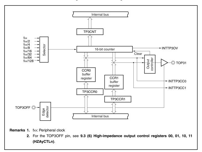
Figure 6-4. TMP3 Block Diagram
