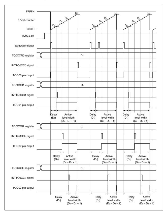
Figure 7-27. Basic Timing in One-Shot Pulse Output Mode
