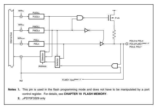
Figure 4-21. Block Diagram of PDL0 to PDL7 Pins
