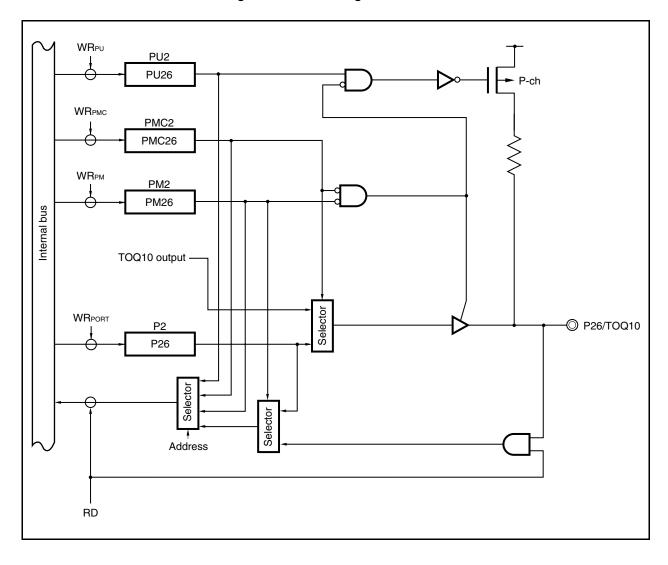
Figure 4-12. Block Diagram of P26 Pin
