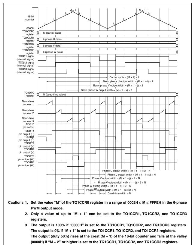
Figure 9-6. Timing Chart of 6-Phase PWM Output Mode
