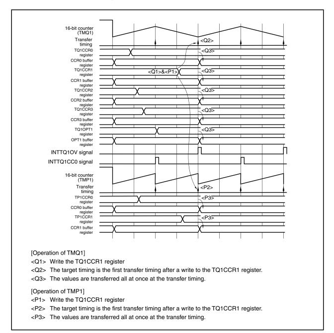
Figure 9-26. Basic Operation in Batch Mode
