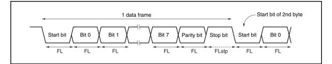
Assuming 1 bit data length: FL; stop bit length: FLstp; and base clock frequency: fuclk, we obtain the following equation.
