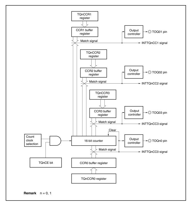
Figure 7-12. Configuration of TQnCCR1 to TQnCCR3 Registers
