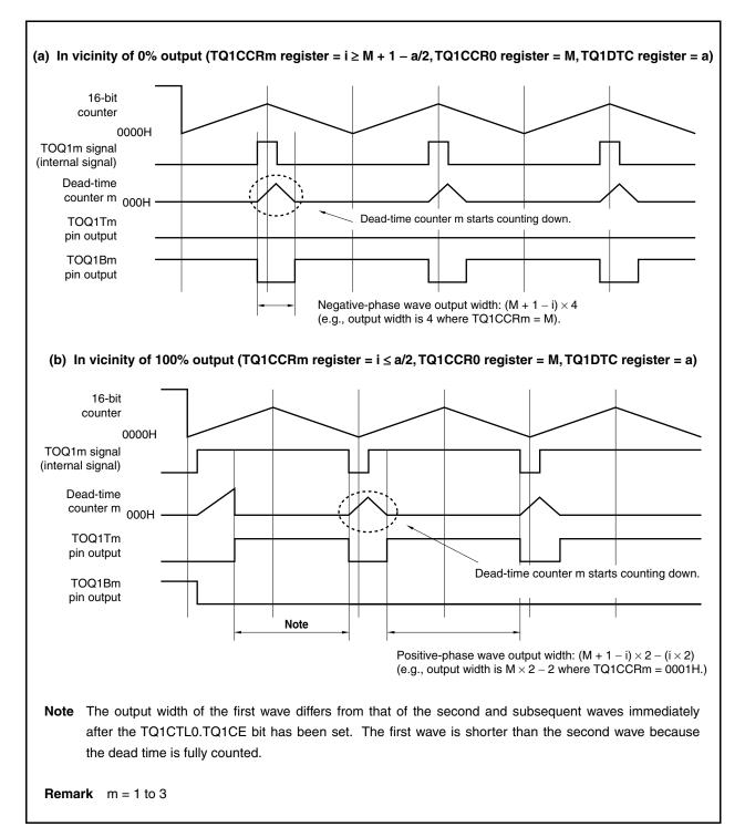
Figure 9-13. Operation of Dead-Time Counter m (1)
