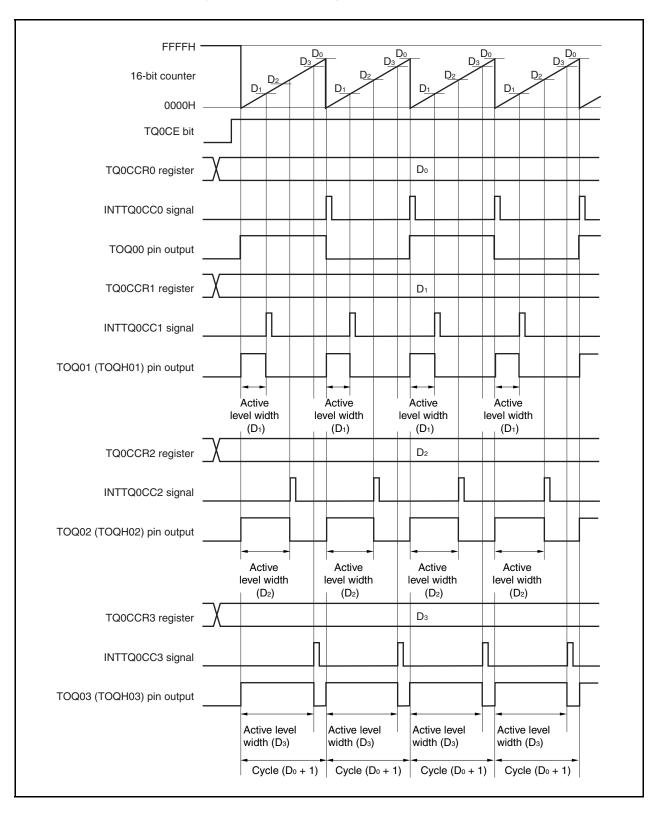
Figure 7-31. Basic Timing in PWM Output Mode
