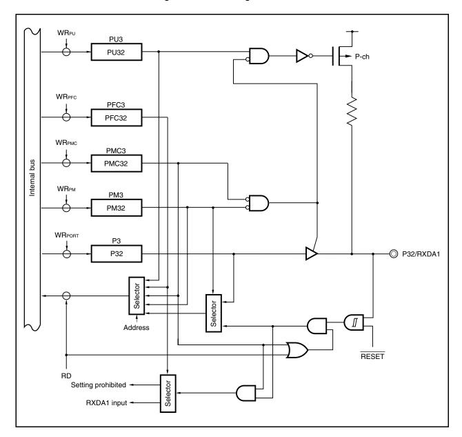
Figure 4-15. Block Diagram of P32 Pin
