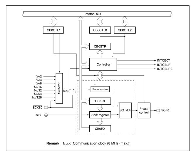
Figure 13-1. Block Diagram of CSIB0
