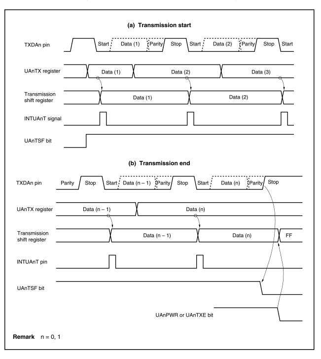
Figure 12-5. Continuous Transmission Operation Timing
