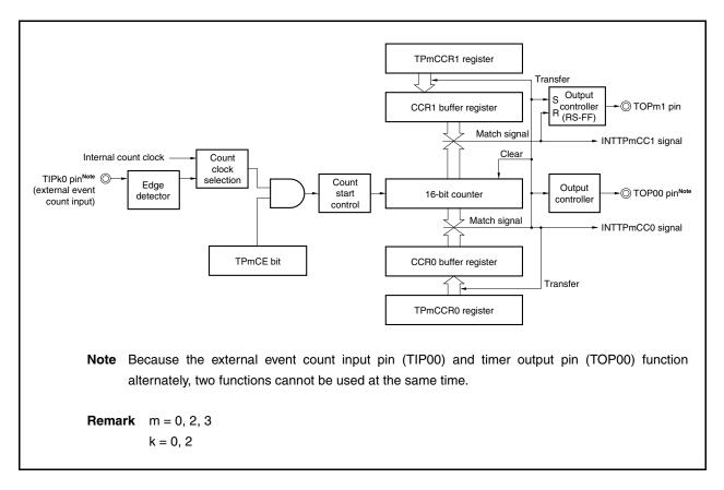
Figure 6-31. Configuration in PWM Output Mode
