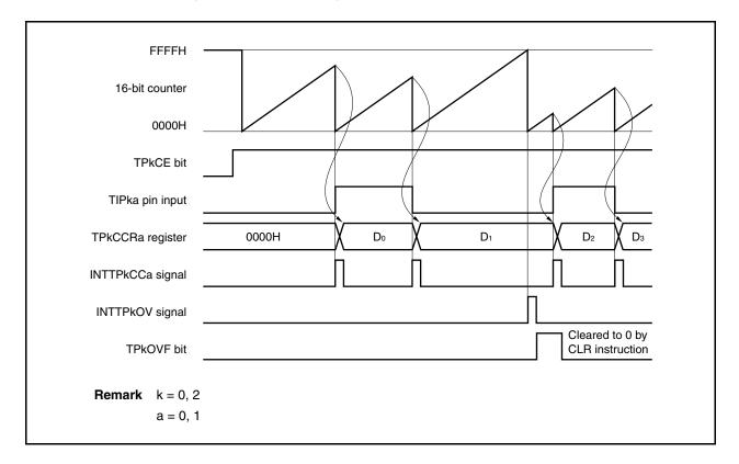
Figure 6-42. Basic Timing in Pulse Width Measurement Mode
