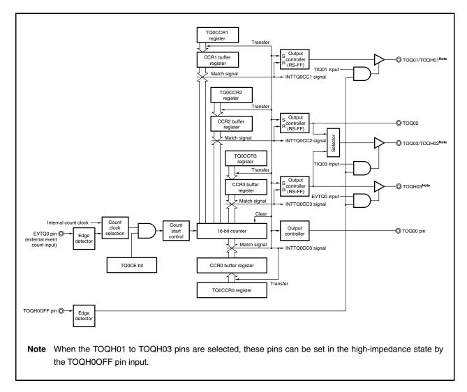
Figure 7-30. Configuration in PWM Output Mode
