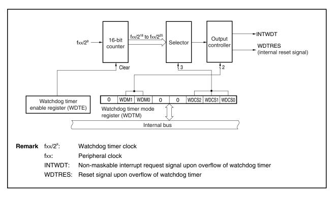
Figure 10-1. Block Diagram of Watchdog Timer
