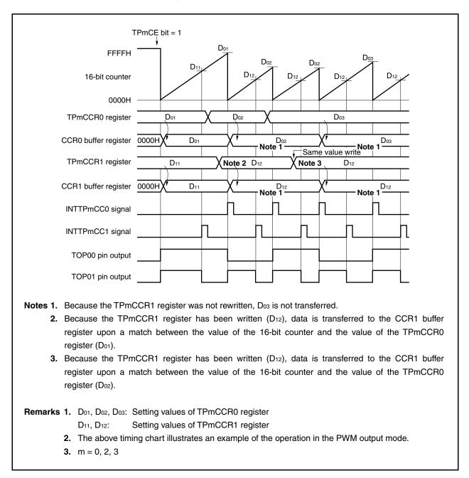
Figure 6-8. Timing of Batch Write
