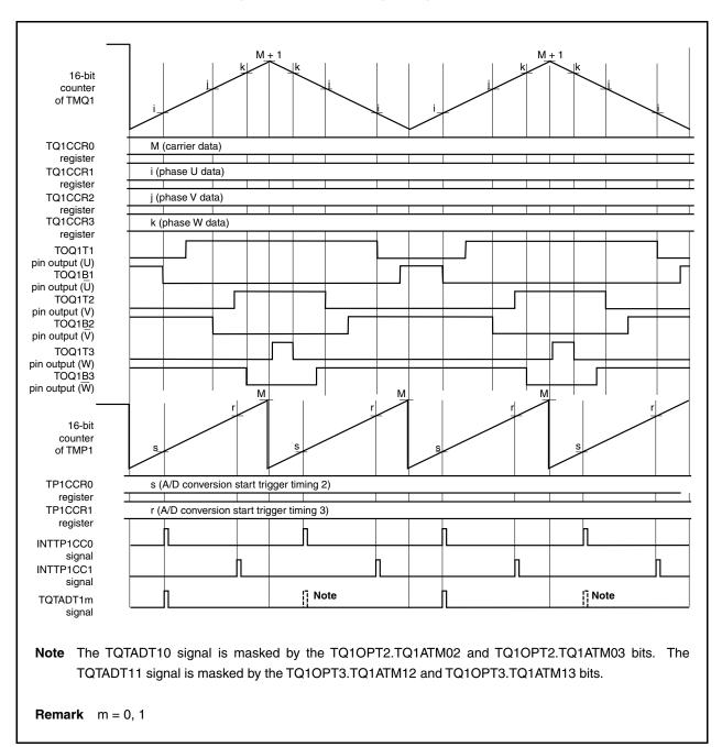
Figure 9-37. TMP1 During Tuning Operation
