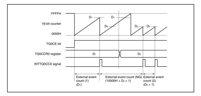
If the value of the TQ0CCR0 register is changed from  $D_1$  to  $D_2$  while the count value is greater than  $D_2$  but less than  $D_1$ , the count value is transferred to the CCR0 buffer register as soon as the TQ0CCR0 register has been rewritten. Consequently, the value that is compared with the 16-bit counter is  $D_2$ .
