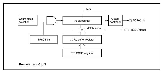
Figure 6-9. Configuration of Interval Timer
