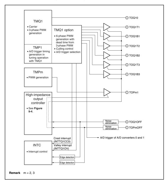
Figure 9-1. Block Diagram of Motor Control
