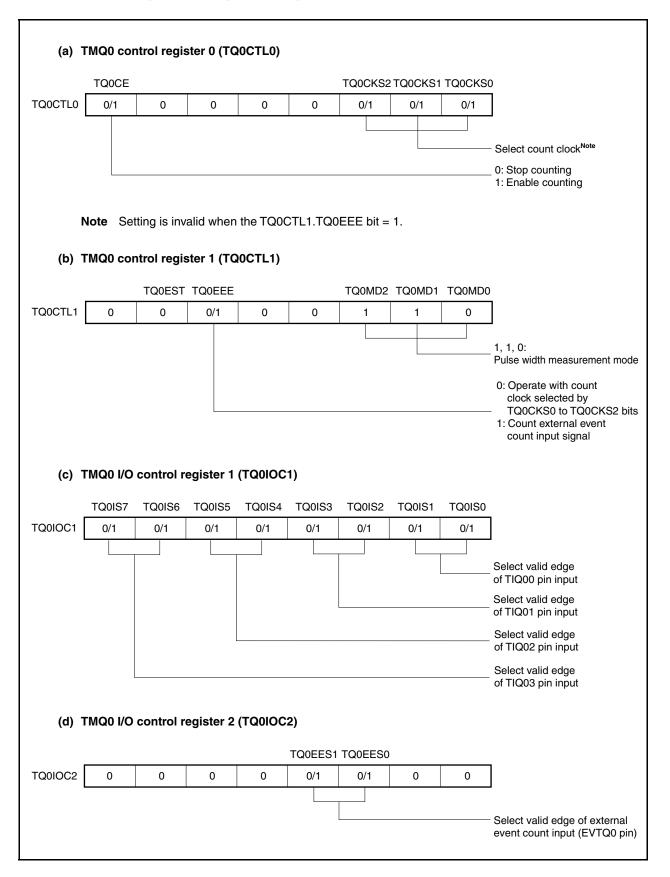
Figure 7-42. Register Setting in Pulse Width Measurement Mode (1/2)
