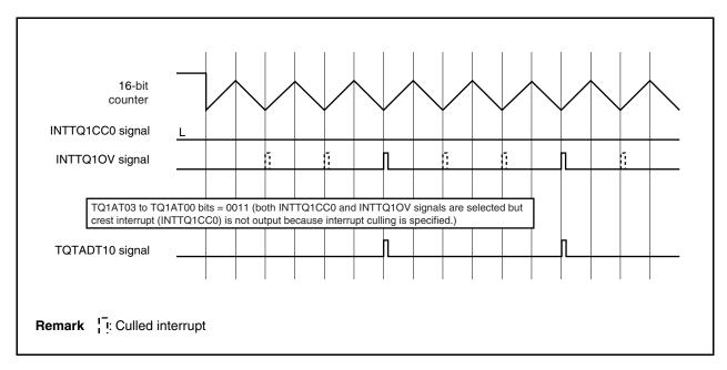
Figure 9-40. Example of A/D Conversion Start Trigger (TQTADT10) Signal Output (TQ1OPT1.TQ1ICE Bit = 0, TQ1OPT1.TQ1IOE Bit = 1, TQ1OPT1.TQ1ID4 to TQ1OPT1.TQ1ID0 Bits = 00010: With Interrupt Culling) (2)
