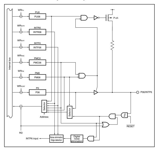
Figure 4-4. Block Diagram of P06 Pin
