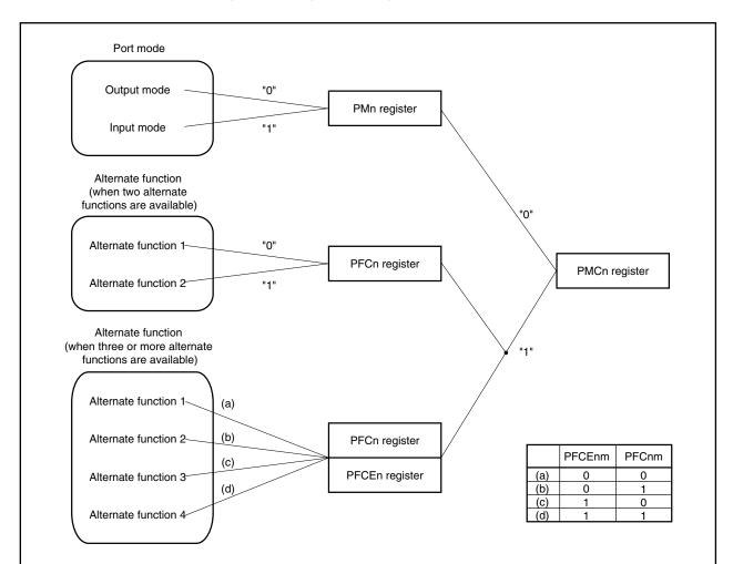
Figure 4-2. Register Settings and Pin Functions
