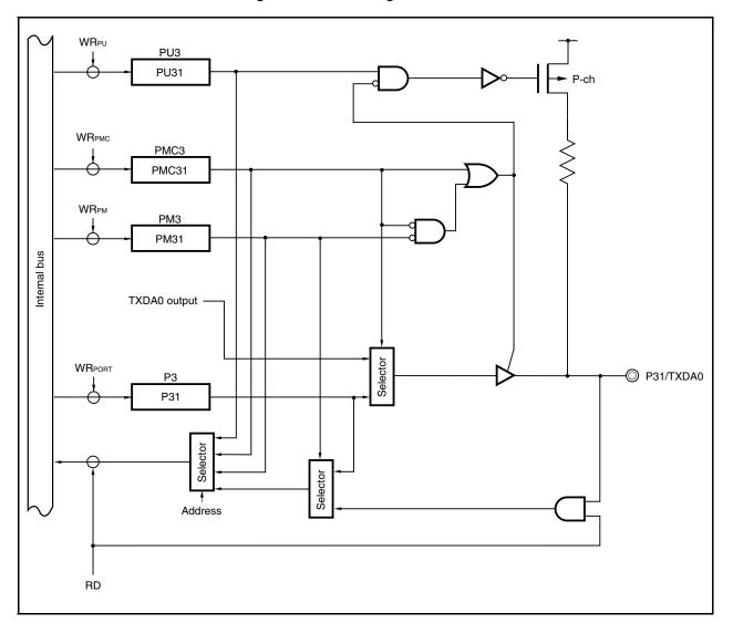
Figure 4-14. Block Diagram of P31 Pin
