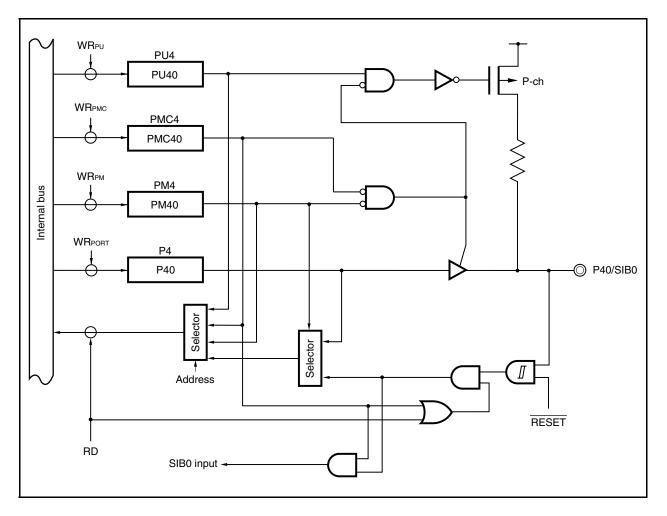
Figure 4-17. Block Diagram of P40 Pin
