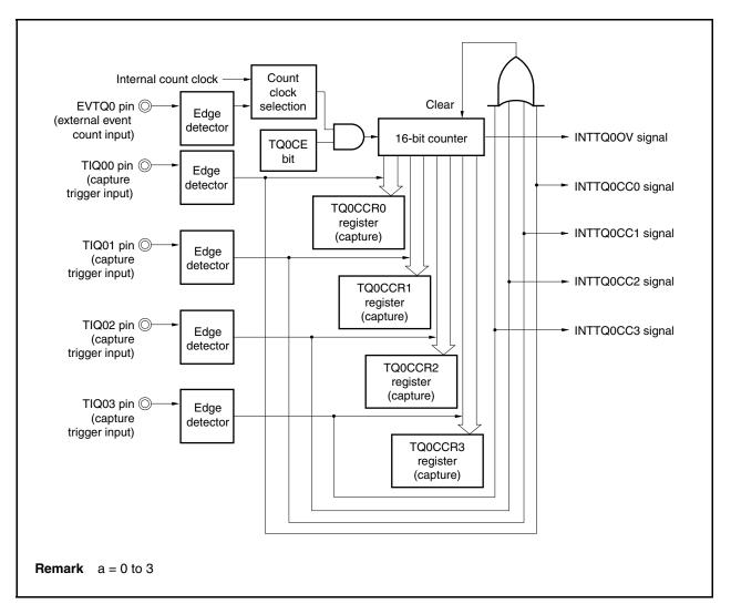
Figure 7-40. Configuration in Pulse Width Measurement Mode
