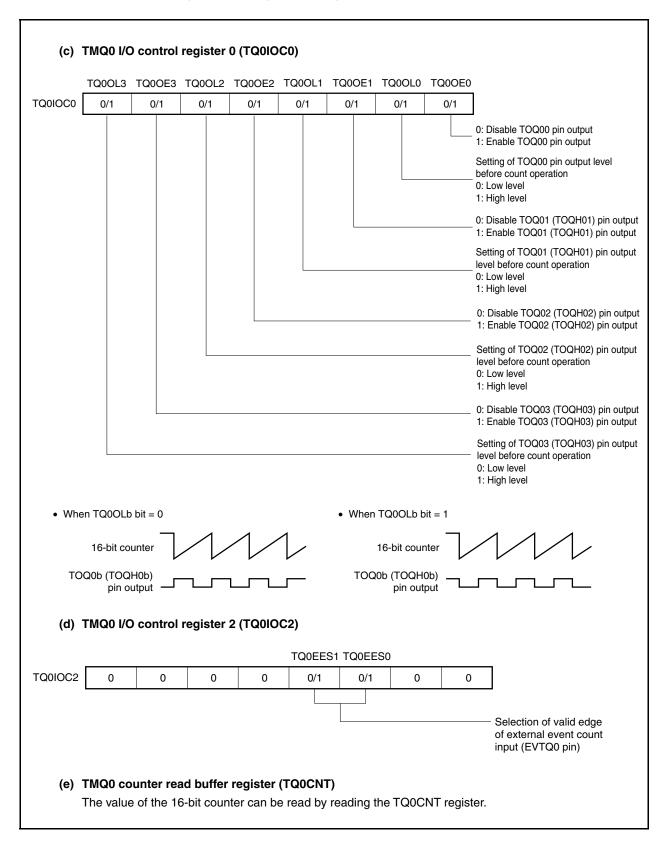
Figure 7-32. Register Setting in PWM Output Mode (2/3)
