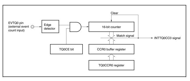
Figure 7-15. Configuration in External Event Count Mode
