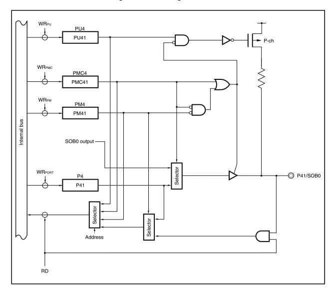
Figure 4-18. Block Diagram of P41 Pin
