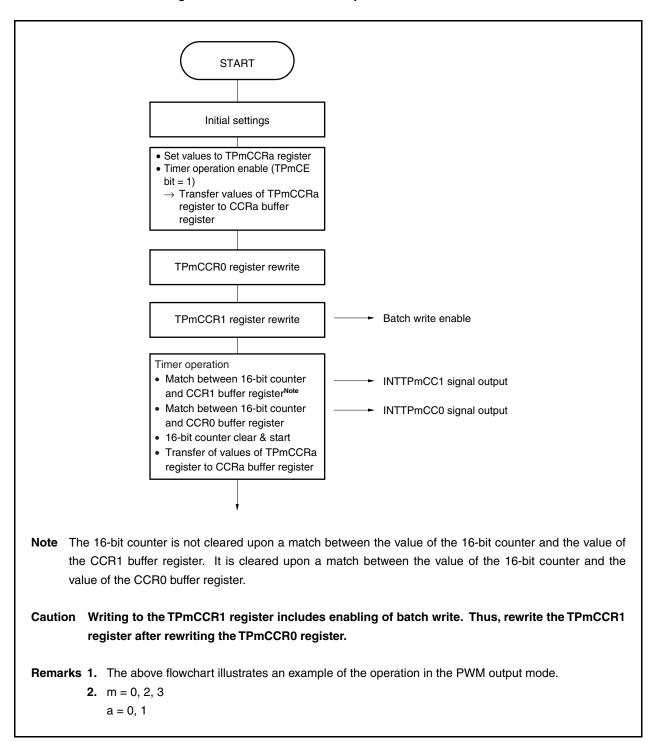
Figure 6-7. Flowchart of Basic Operation for Batch Write
