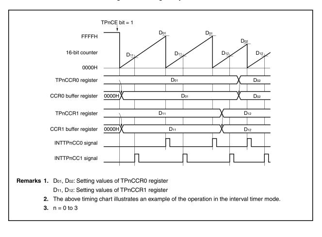
Figure 6-6. Timing of Anytime Write
