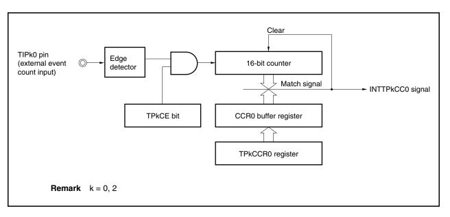
Figure 6-16. Configuration in External Event Count Mode
