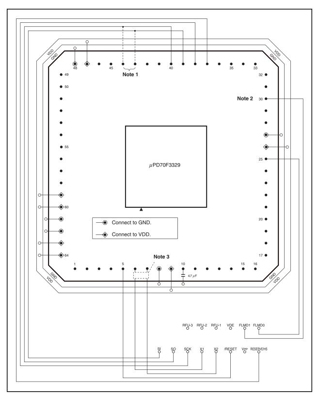
Figure 19-6. Wiring Example of V850ES/IK1 Flash Writing Adapter (FA-64GC-8BS) (1/2)
