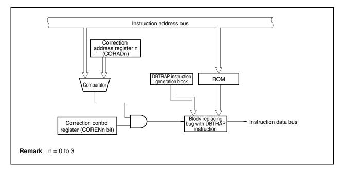
Figure 18-1. Block Diagram of ROM Correction
