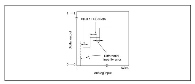
Figure 11-28. Differential Linearity Error
