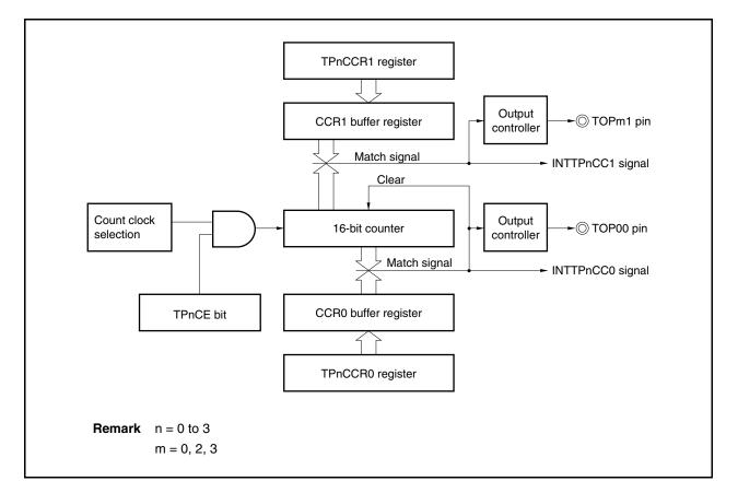
When the TPnCCR1 register is set to the same value as that of the TPnCCR0 register, the INTTPnCC1 signal is generated at the same timing as the INTTPnCC0 signal and the TOPm1 pin output is inverted. In other words, a PWM waveform with a duty factor of 50% can be output from the TOPm1 pin.
