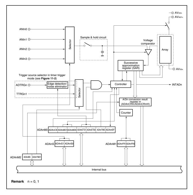
Cautions 1. If there is noise at the analog input pins (ANIn0 to ANIn3) or at the A/D converter reference voltage input pin (AVREFn), that noise may generate an illegal conversion result (n = 0, 1). Software processing will be needed to avoid a negative effect on the system from this illegal conversion result.
