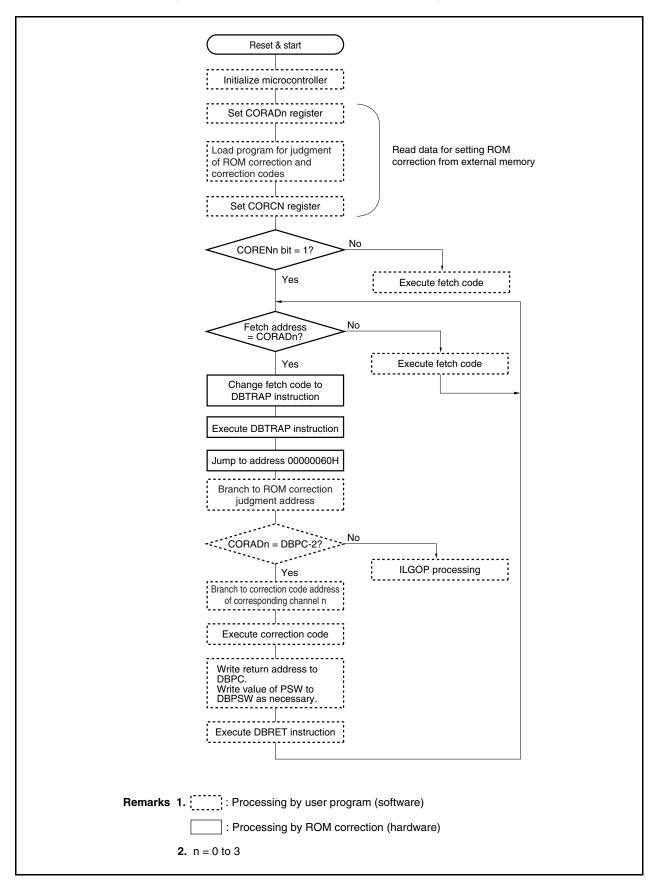
Figure 18-2. ROM Correction Operation and Program Flow
