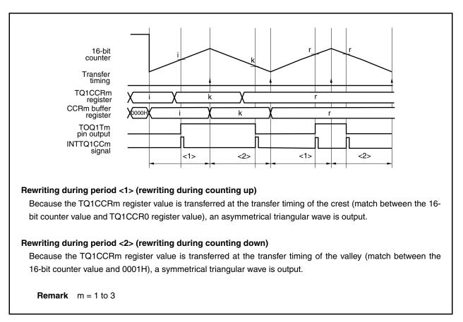
Figure 9-30. Example of Rewriting TQ1CCRm Register
