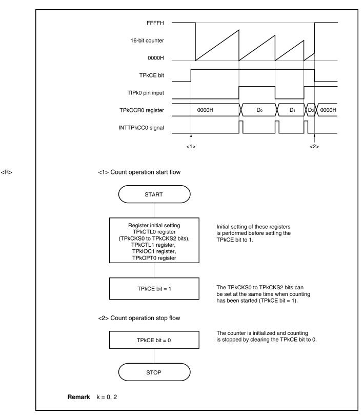
Figure 6-44. Software Processing Flow in Pulse Width Measurement Mode
