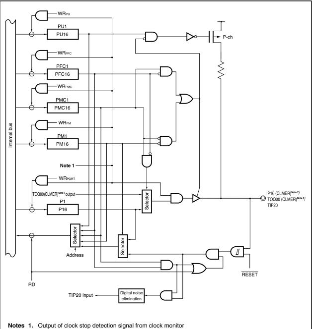
Figure 4-9. Block Diagram of P16 Pin
