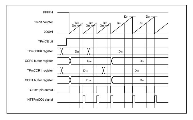
To transfer data from the TPmCCRa register to the CCRa buffer register, the TPmCCR1 register must be written.
