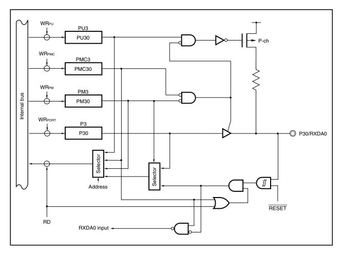
Figure 4-13. Block Diagram of P30 Pin
