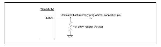
Figure 19-10. FLMD0 Pin Connection Example
