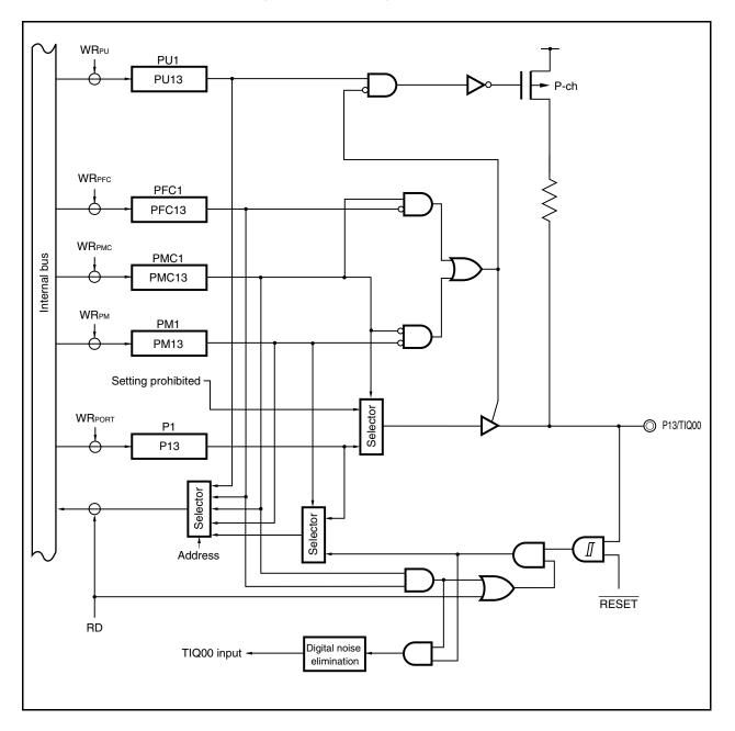
Figure 4-7. Block Diagram of P13 Pin
