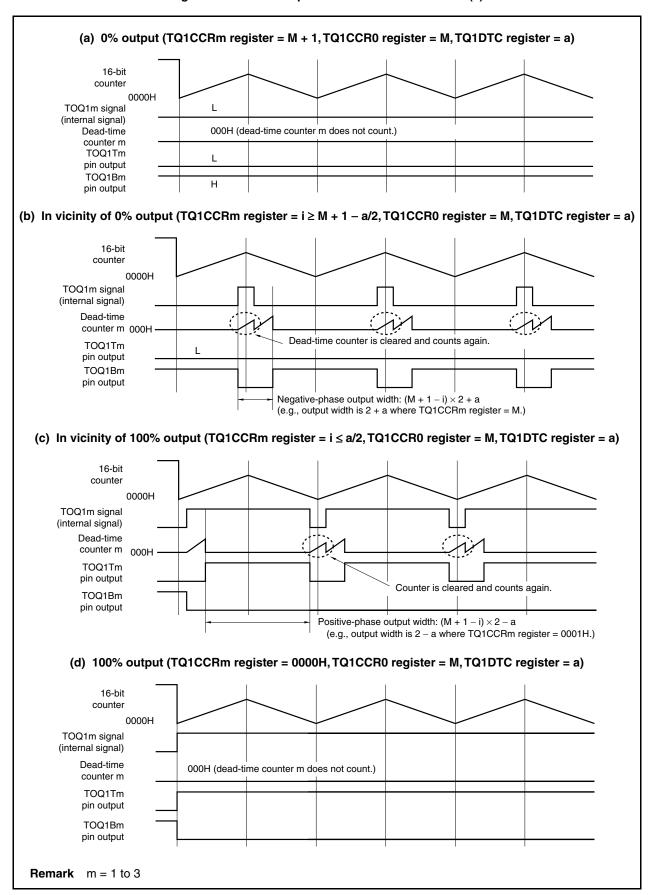
Figure 9-12. PWM Output Waveform with Dead Time (2)
