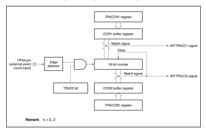
Figure 6-20. Configuration of TPkCCR1 Register
