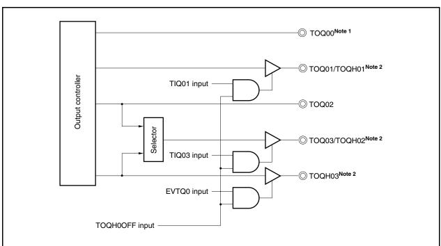
Figure 7-2. TMQ0 Output Pin Configuration
