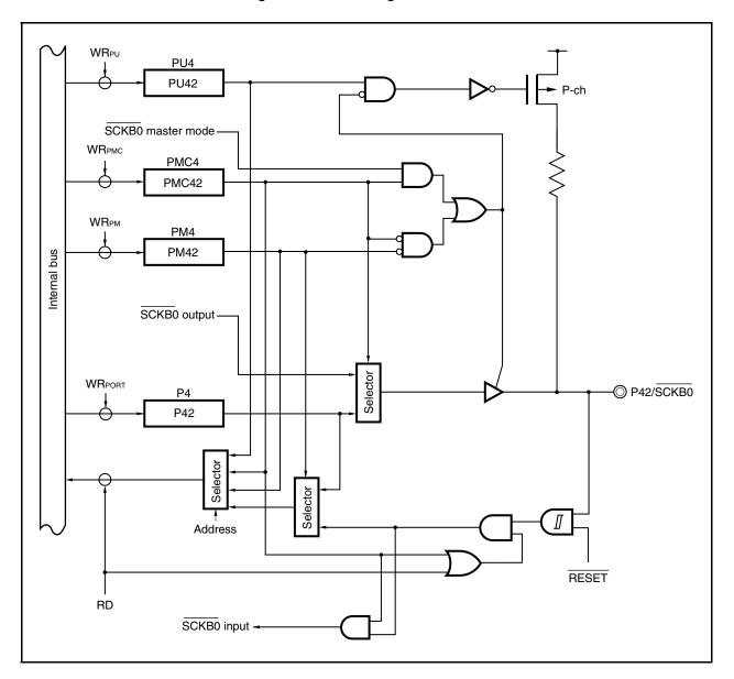
Figure 4-19. Block Diagram of P42 Pin
