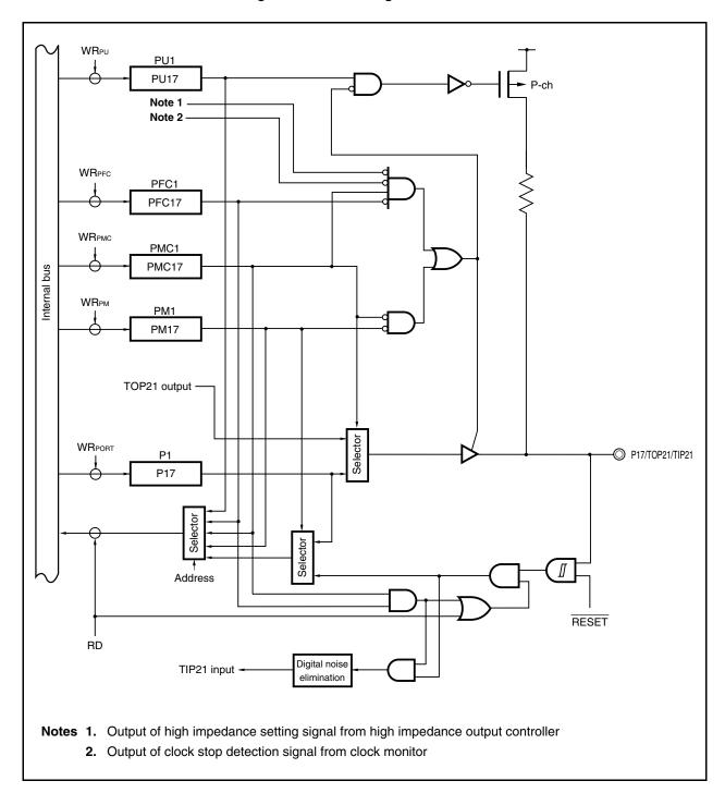
Figure 4-10. Block Diagram of P17 Pin
