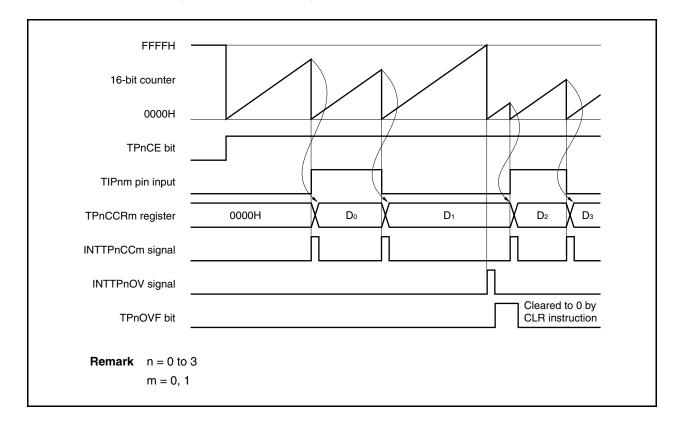
Figure 7-35. Basic Timing in Pulse Width Measurement Mode
