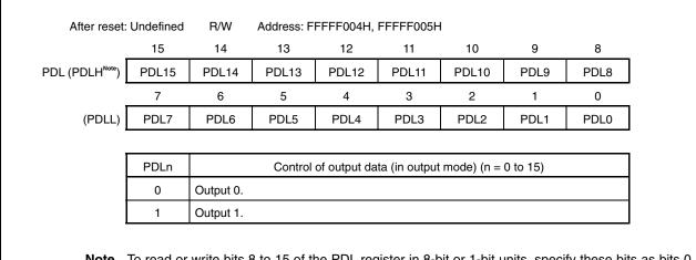
**Note** To read or write bits 8 to 15 of the PDL register in 8-bit or 1-bit units, specify these bits as bits 0 to 7 of the PDLH register.
