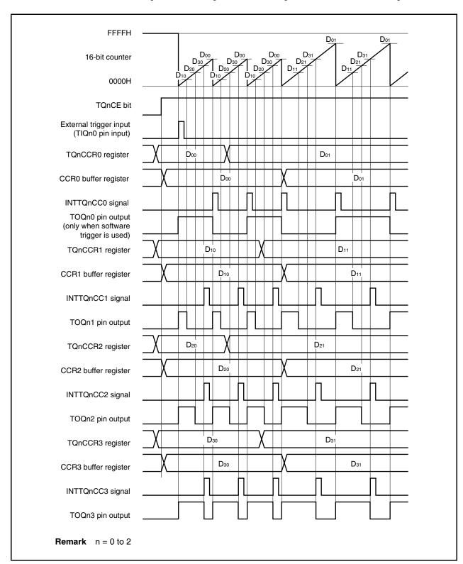
In order to transfer data from the TQnCCRm register to the CCRm buffer register, the TQnCCR1 register must be written.
