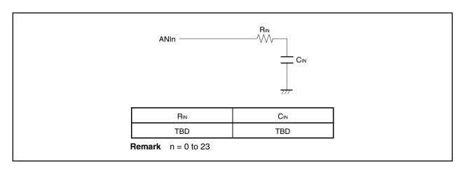
Figure 12-11. Internal Equivalent Circuit of ANIn Pin
