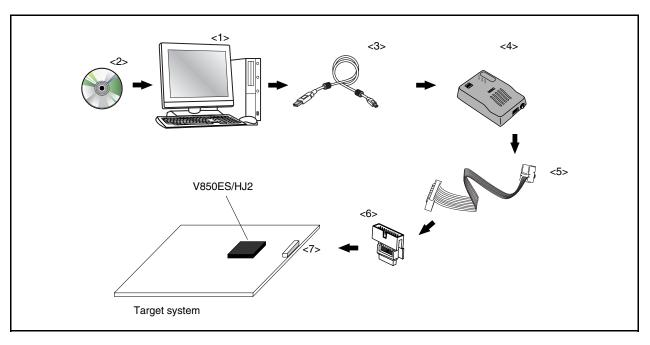
Figure A-3. On-Chip Emulation System Configuration
