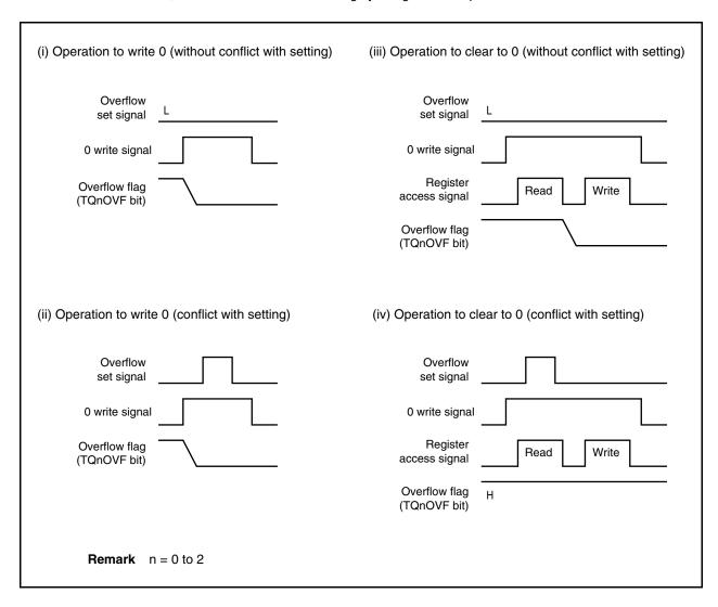
To clear the overflow flag to 0, read the overflow flag to check if it is set to 1, and clear it with the CLR instruction. If 0 is written to the overflow flag without checking if the flag is 1, the set information of overflow may be erased by writing 0 ((ii) in the above chart). Therefore, software may judge that no overflow has occurred even when an overflow actually has occurred.
