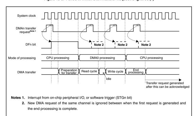
Figure 15-3. Period in Which DMA Transfer Request Is Ignored (1)
