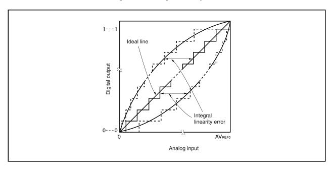
Figure 12-18. Integral Linearity Error
