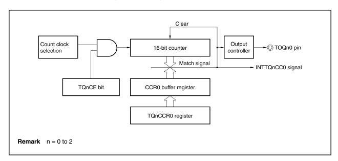
Figure 8-2. Configuration of Interval Timer
