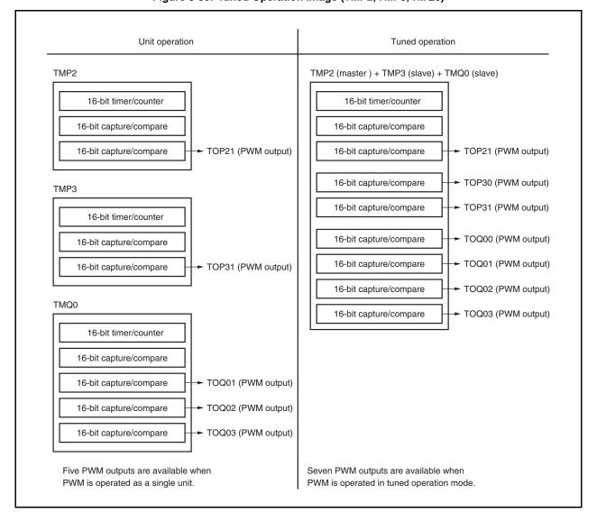
Figure 8-39. Tuned Operation Image (TMP2, TMP3, TMQ0)
