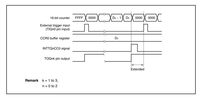
If the trigger is detected immediately before the INTTQnCC0 signal is generated, the INTTQnCC0 signal is not generated. The 16-bit counter is cleared to 0000H, the TOQnk pin is asserted, and the counter continues counting. Consequently, the inactive period of the PWM waveform is shortened.
