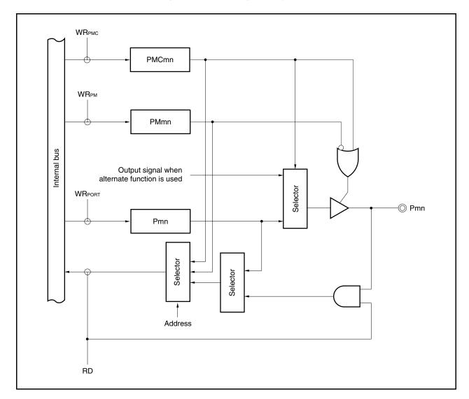
Figure 4-6. Block Diagram of Type D-2
