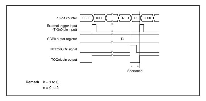
If the trigger is detected immediately before the INTTQnCCk signal is generated, the INTTQnCCk signal is not generated, and the 16-bit counter is cleared to 0000H and continues counting. The output signal of the TOQnk pin remains active. Consequently, the active period of the PWM waveform is extended.
