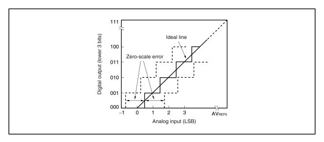
Figure 12-15. Zero-Scale Error
