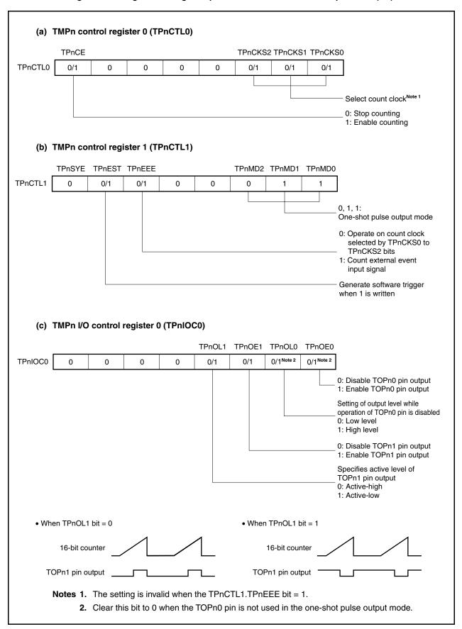
Figure 7-22. Register Setting for Operation in One-Shot Pulse Output Mode (2/2)
