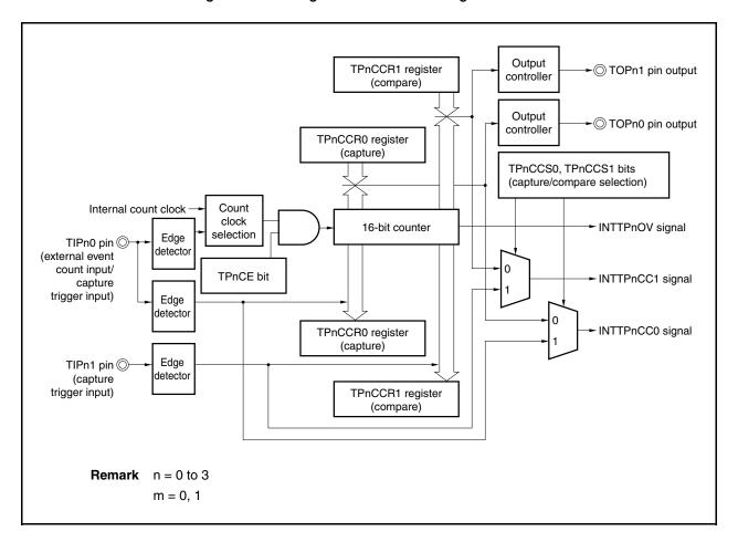
Figure 7-28. Configuration in Free-Running Timer Mode
