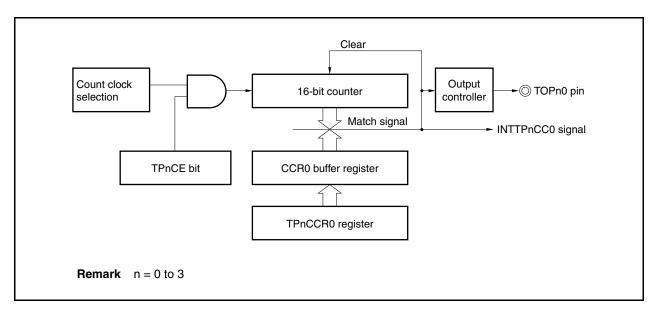
Figure 7-2. Configuration of Interval Timer
