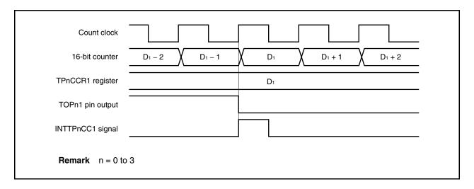
Usually, the INTTPnCC1 signal is generated in synchronization with the next counting up after the count value of the 16-bit counter matches the value of the TPnCCR1 register.
