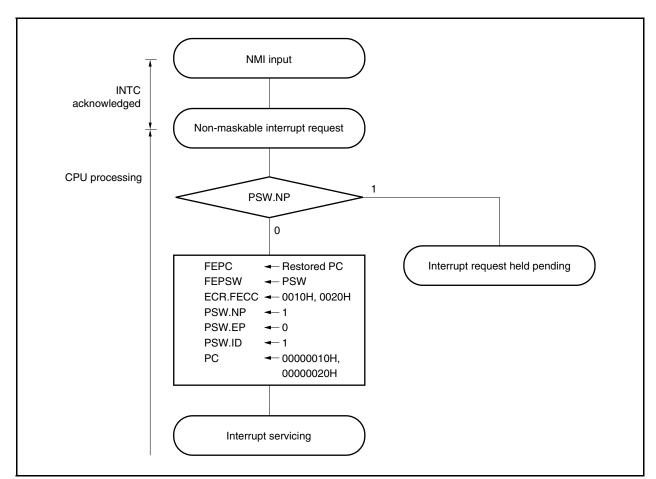
Figure 16-2. Servicing Configuration of Non-Maskable Interrupt
