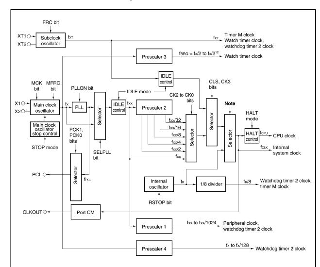
**Note** The internal oscillation clock is selected when watchdog timer 2 overflows during the oscillation stabilization time.
