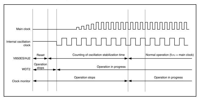
Figure 19-3. Operation After Reset Release
