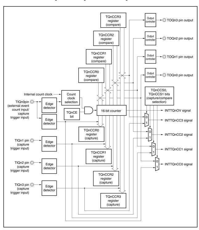
When the TQnCE bit is set to 1, 16-bit timer/event counter Q starts counting, and the output signals of the TQn0 to TQQn3 pins are inverted. When the count value of the 16-bit counter later matches the set value of the TQnCCRm register, a compare match interrupt request signal (INTTQnCCm) is generated, and the output signal of the TQnm pin is inverted.
