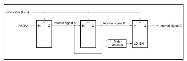
Figure 13-11. Noise Filter Circuit
