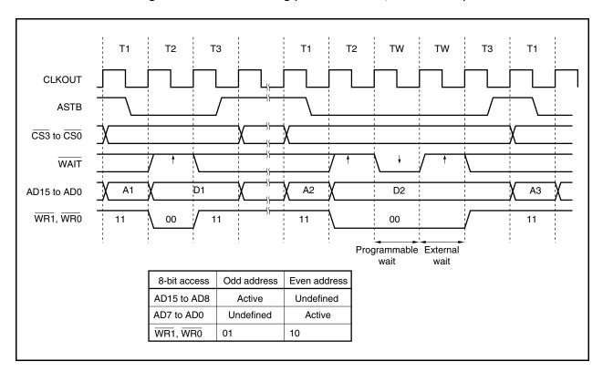
Figure 5-6. Bus Write Timing (Bus Size: 16 Bits, 16-Bit Access)
