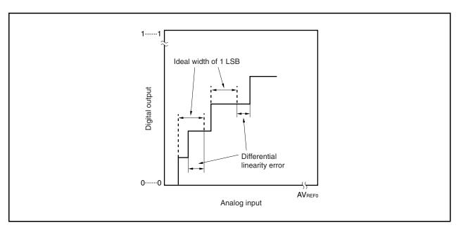
Figure 12-17. Differential Linearity Error
