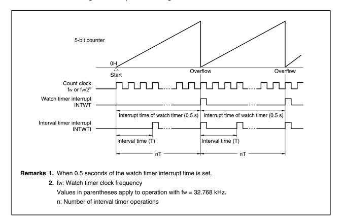
Figure 10-2. Operation Timing of Watch Timer/Interval Timer
