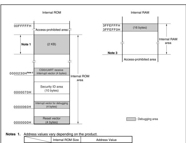
Figure 26-4. Memory Spaces Where Debug Monitor Programs Are Allocated
