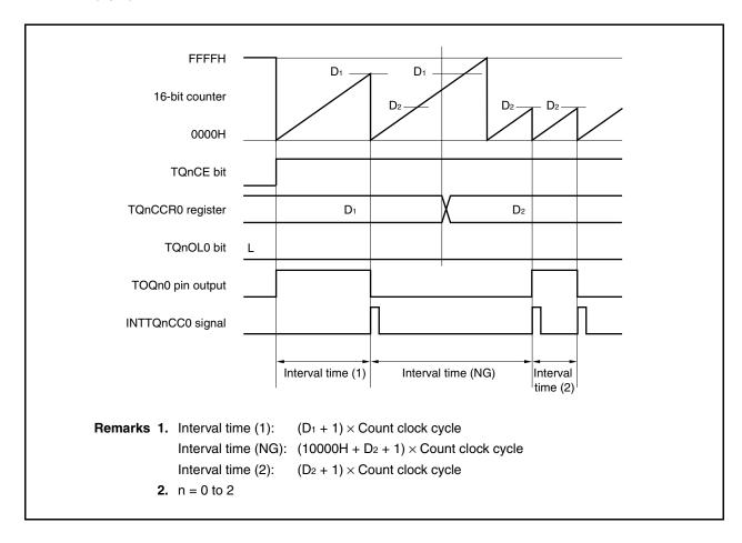
If the value of the TQnCCR0 register is changed from  $D_1$  to  $D_2$  while the count value is greater than  $D_2$  but less than  $D_1$ , the count value is transferred to the CCR0 buffer register as soon as the TQnCCR0 register has been rewritten. Consequently, the value of the 16-bit counter that is compared is  $D_2$ .
