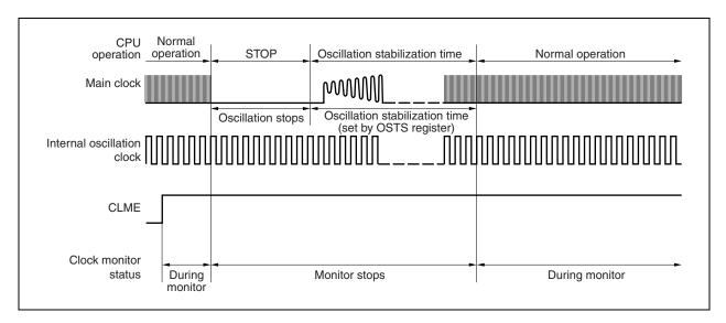
Figure 20-4. Operation in STOP Mode or After STOP Mode Is Released
