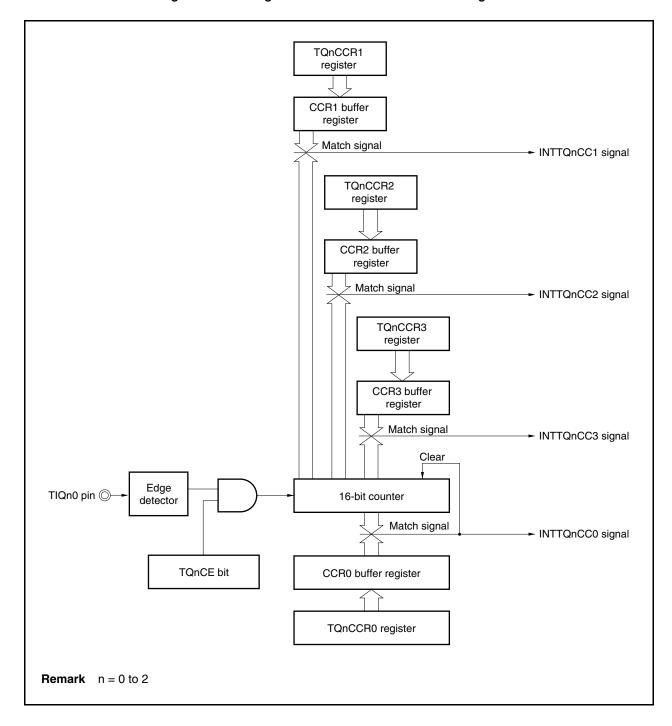
If the set value of the TQnCCRk register is smaller than the set value of the TQnCCR0 register, the INTTQnCCk signal is generated once per cycle.
