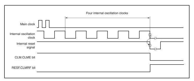
Figure 20-2. Reset Period Due to That Oscillation of Main Clock Is Stopped
