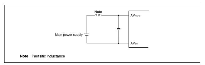
Figure 12-12. AVREFO Pin Processing Example
