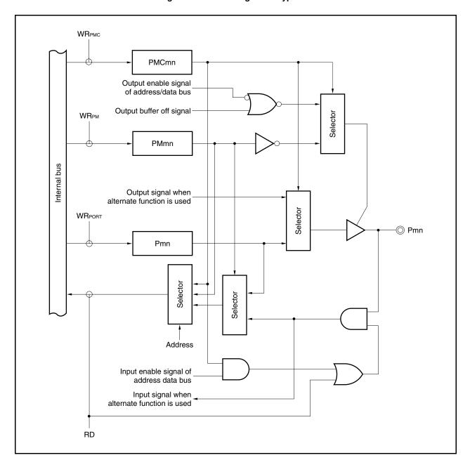
Figure 4-7. Block Diagram of Type D-3
