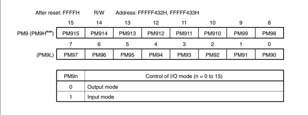
**Note** To read or write bits 8 to 15 of the PM9 register in 8-bit or 1-bit units, specify these bits as bits 0 to 7 of the PM9H register.
