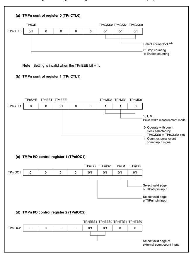
Figure 7-36. Register Setting in Pulse Width Measurement Mode (2/2)
