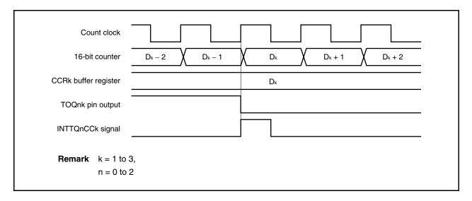
Usually, the INTTQnCCk signal is generated in synchronization with the next count up after the count value of the 16-bit counter matches the value of the CCRk buffer register.
