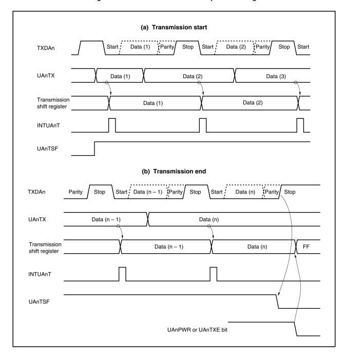
Figure 13-9. Continuous Transmission Operation Timing
