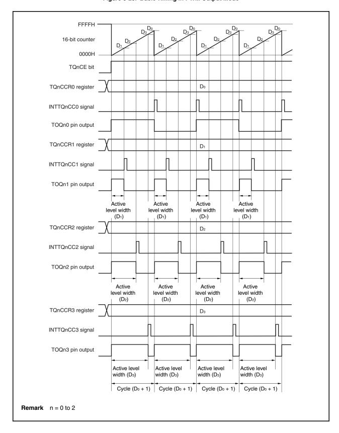
Figure 8-25. Basic Timing in PWM Output Mode
