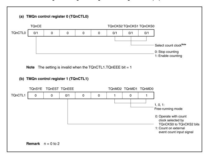
Figure 8-31. Register Setting in Free-Running Timer Mode (2/3)
