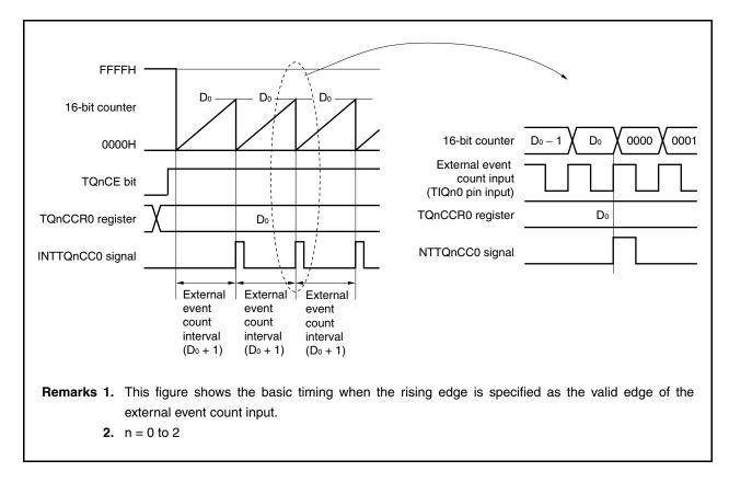
When the TQnCE bit is set to 1, the value of the 16-bit counter is cleared from FFFFH to 0000H. The counter counts each time the valid edge of external event count input is detected. Additionally, the set value of the TQnCCR0 register is transferred to the CCR0 buffer register.
