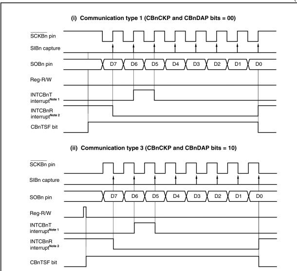
**Notes 1.** The INTCBnT interrupt is set when the data written to the CBnTX register is transferred to the data shift register in the continuous transmission or continuous transmission/reception mode. In the single transmission or single transmission/reception mode, the INTCBnT interrupt request signal is not generated, but the INTCBnR interrupt request signal is generated upon end of communication.
