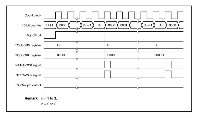
To output a 100% waveform, set a value of (set value of TQnCCR0 register + 1) to the TQnCCRk register. If the set value of the TQnCCR0 register is FFFFH, 100% output cannot be produced.
