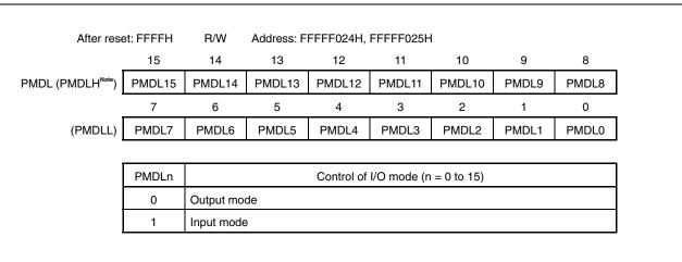
**Note** To read or write bits 8 to 15 of the PMDL register in 8-bit or 1-bit units, specify these bits as bits 0 to 7 of the PMDLH register.
