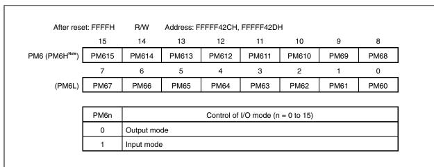
**Note** To read or write bits 8 to 15 of the PM6 register in 8-bit or 1-bit units, specify these bits as bits 0 to 7 of the PM6H register.
