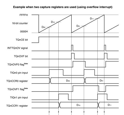
Note The TQnOVF0 and TQnOVF1 flags are set on the internal RAM by software.
