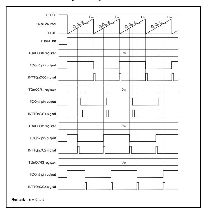
If the set value of the TQnCCRk register is greater than the set value of the TQnCCR0 register, the count value of the 16-bit counter does not match the value of the TQnCCRk register. Consequently, the INTTQnCCk signal is not generated, nor is the output of the TQQnk pin changed.
