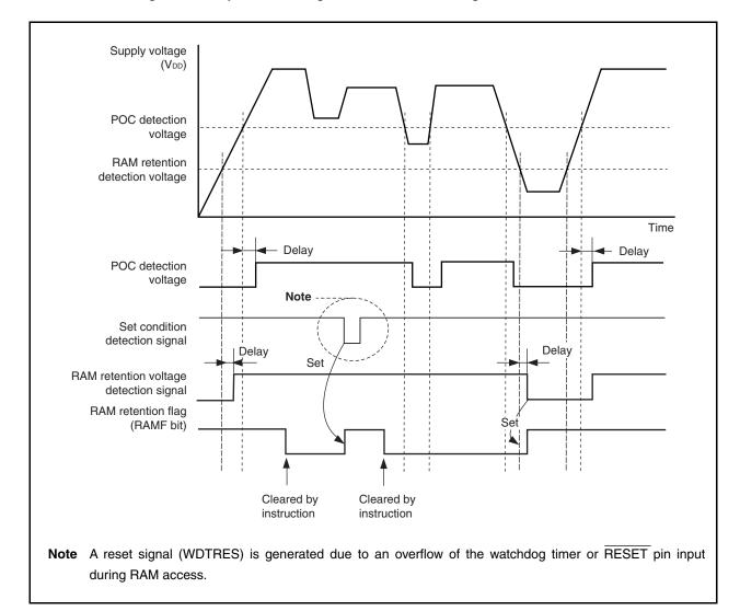
Figure 22-4. Operation Timing of RAM Retention Voltage Detection Function
