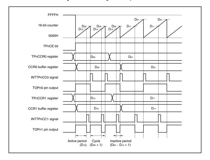
Figure 7-25. Basic Timing in PWM Output Mode
