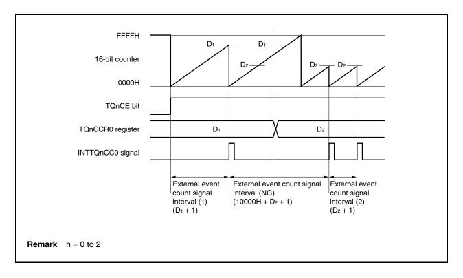
If the value of the TQnCCR0 register is changed from  $D_1$  to  $D_2$  while the count value is greater than  $D_2$  but less than  $D_1$ , the count value is transferred to the CCR0 buffer register as soon as the TQnCCR0 register has been rewritten. Consequently, the value that is compared with the 16-bit counter is  $D_2$ .
