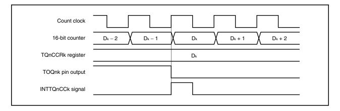
Usually, the INTTQnCCk signal is generated when the 16-bit counter counts up next time after its count value matches the value of the TQnCCRk register.
