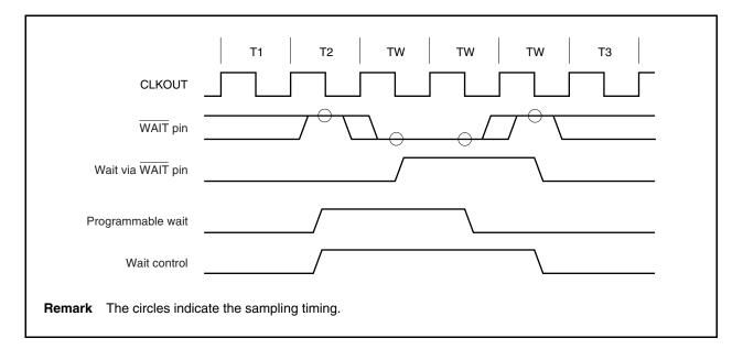
Figure 5-3. Inserting Wait Example
