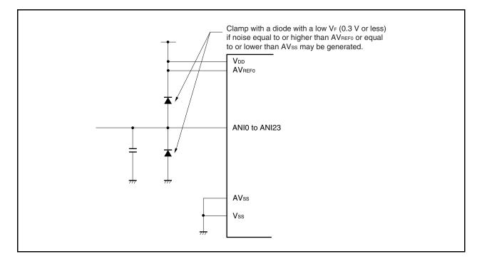
Figure 12-9. Processing of Analog Input Pin
