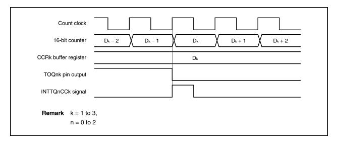
Usually, the INTTQnCCk signal is generated in synchronization with the next counting up after the count value of the 16-bit counter matches the value of the TQnCCRk register.
