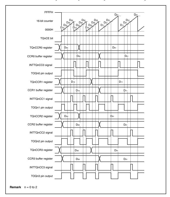
To transfer data from the TQnCCRm register to the CCRm buffer register, the TQnCCR1 register must be written.
