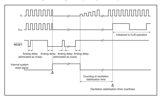
Figure 19-1. Timing of Reset Operation by RESET Pin Input
