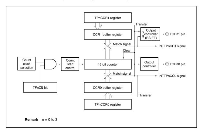
Figure 7-24. Configuration in PWM Output Mode
