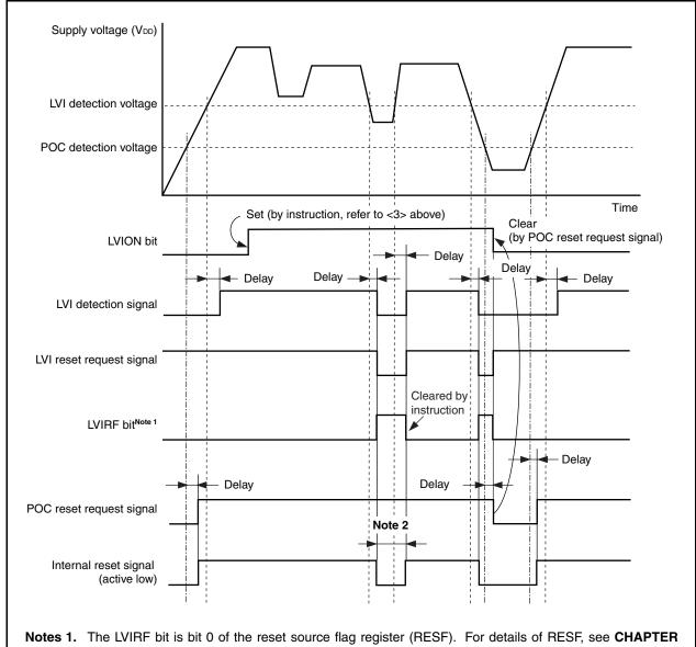
Figure 22-2. Operation Timing of Low-Voltage Detector (LVIMD Bit = 1)
