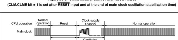
Figure 20-3. Clock Monitor Status After RESET Input
