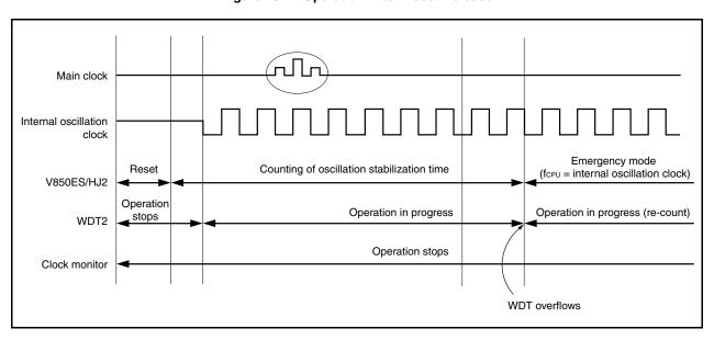
Figure 19-4. Operation After Reset Release
