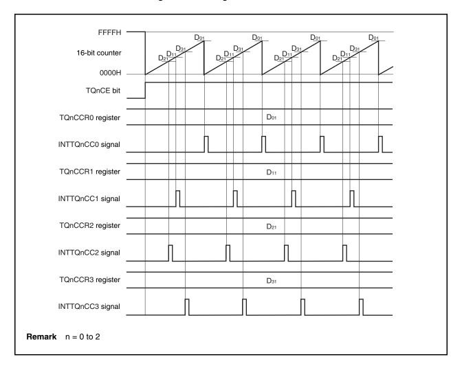
If the set value of the TQnCCRk register is greater than the set value of the TQnCCR0 register, the INTTQnCCk signal is not generated because the count value of the 16-bit counter and the value of the TQnCCRk register do not match.
