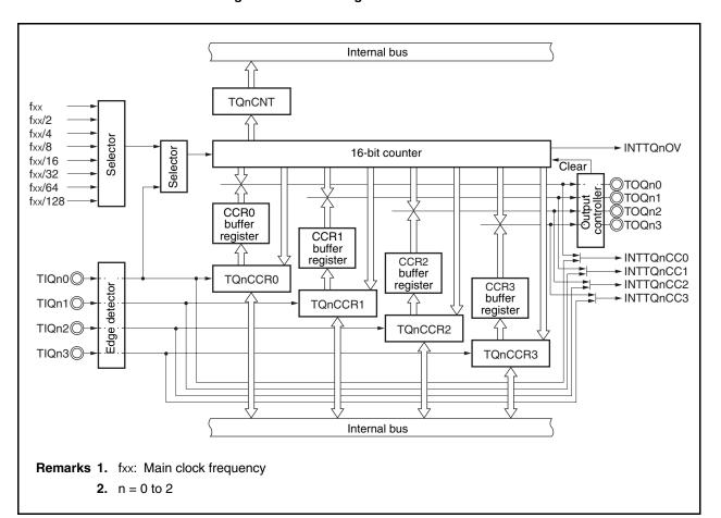
Figure 8-1. Block Diagram of TMQ0 to TMQ2
