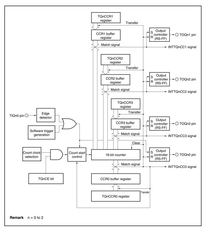
Figure 8-20. Configuration in One-Shot Pulse Output Mode
