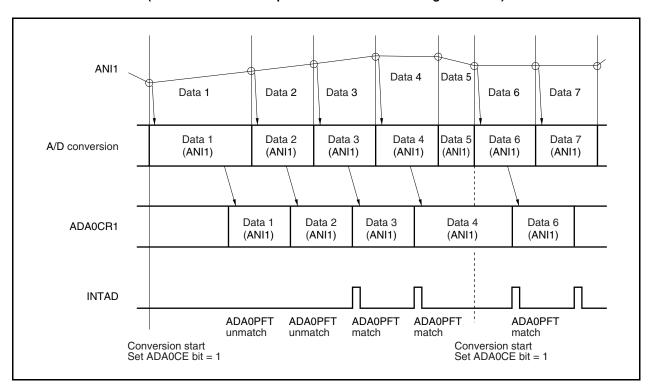
Figure 12-6. Timing Example of Continuous Select Mode Operation (When Power-Fail Comparison Is Made: ADA0S Register = 01H)
