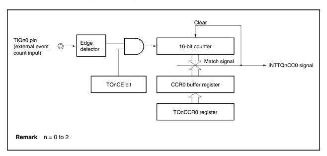
Figure 8-9. Configuration in External Event Count Mode
