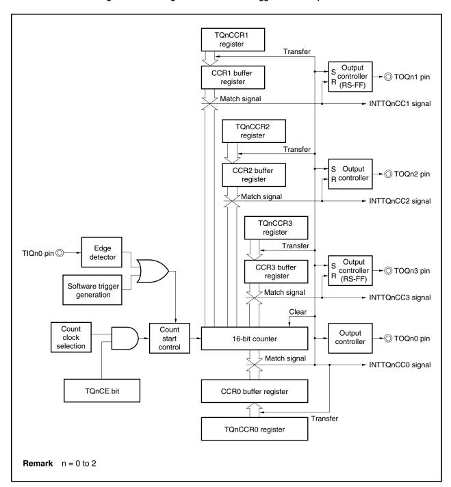
Figure 8-16. Configuration in External Trigger Pulse Output Mode
