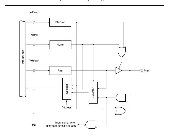
Figure 4-5. Block Diagram of Type D-1
