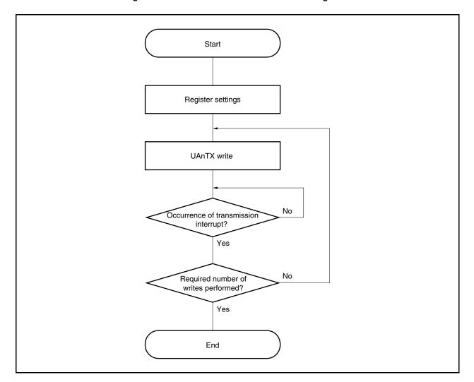
Figure 13-8. Continuous Transmission Processing Flow
