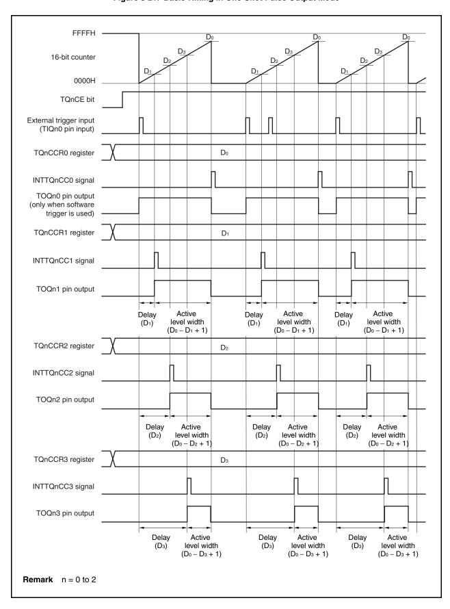
Figure 8-21. Basic Timing in One-Shot Pulse Output Mode
