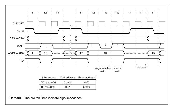
Figure 5-5. Bus Read Timing (Bus Size: 8 Bits)
