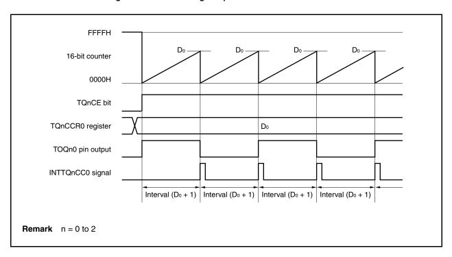
When the TQnCE bit is set to 1, the value of the 16-bit counter is cleared from FFFFH to 0000H in synchronization with the count clock, and the counter starts counting. At this time, the output of the TQnO pin is inverted. Additionally, the set value of the TQnCCR0 register is transferred to the CCR0 buffer register.
