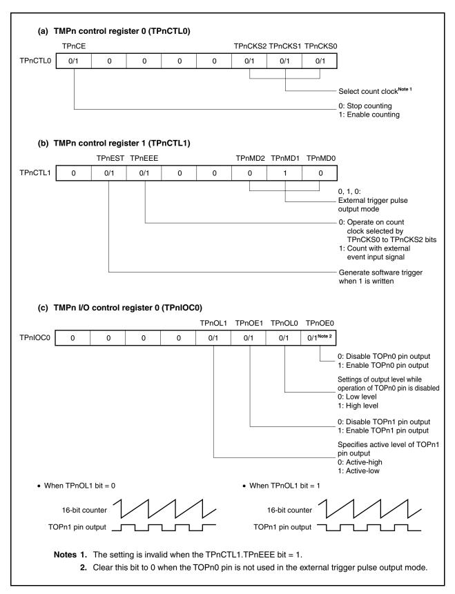
Figure 7-18. Setting of Registers in External Trigger Pulse Output Mode (2/2)
