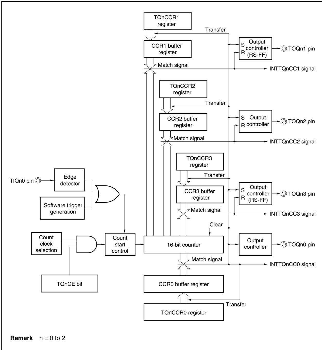
Figure 8-17. Basic Timing in External Trigger Pulse Output Mode
