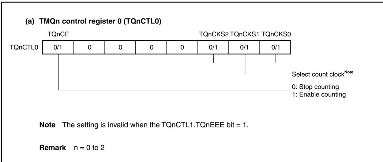
Figure 8-18. Setting of Registers in External Trigger Pulse Output Mode (2/3)
