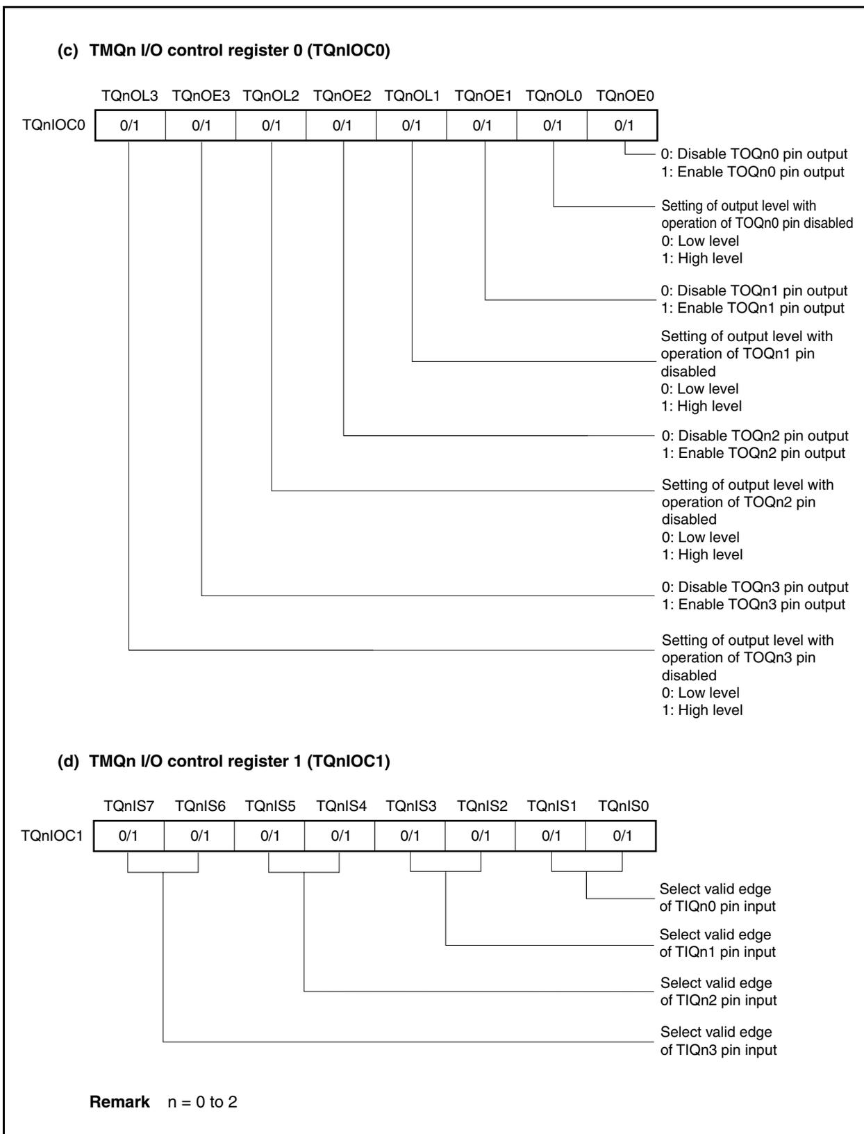
Figure 8-31. Register Setting in Free-Running Timer Mode (3/3)
