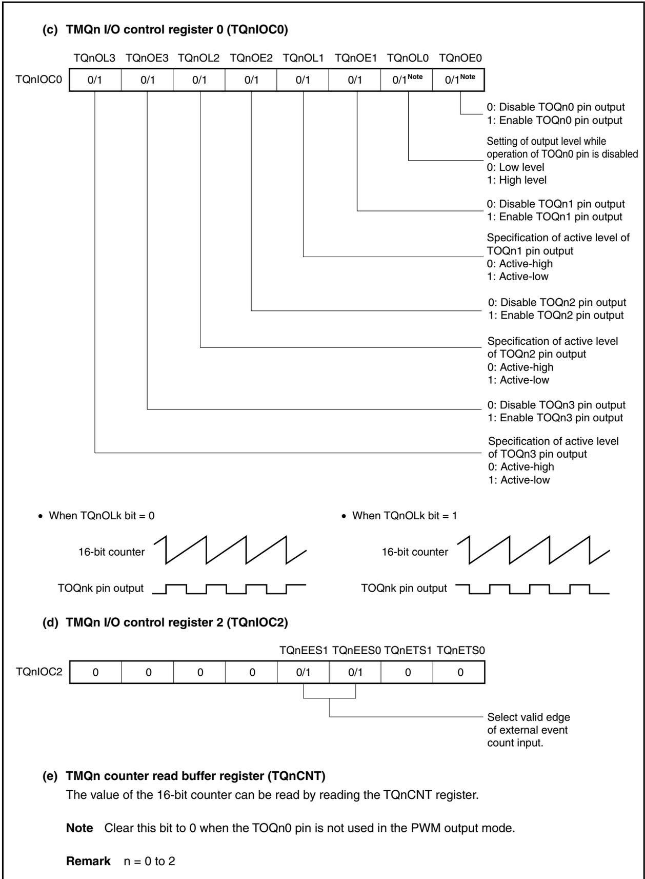
Figure 8-26. Register Setting in PWM Output Mode (3/3)
