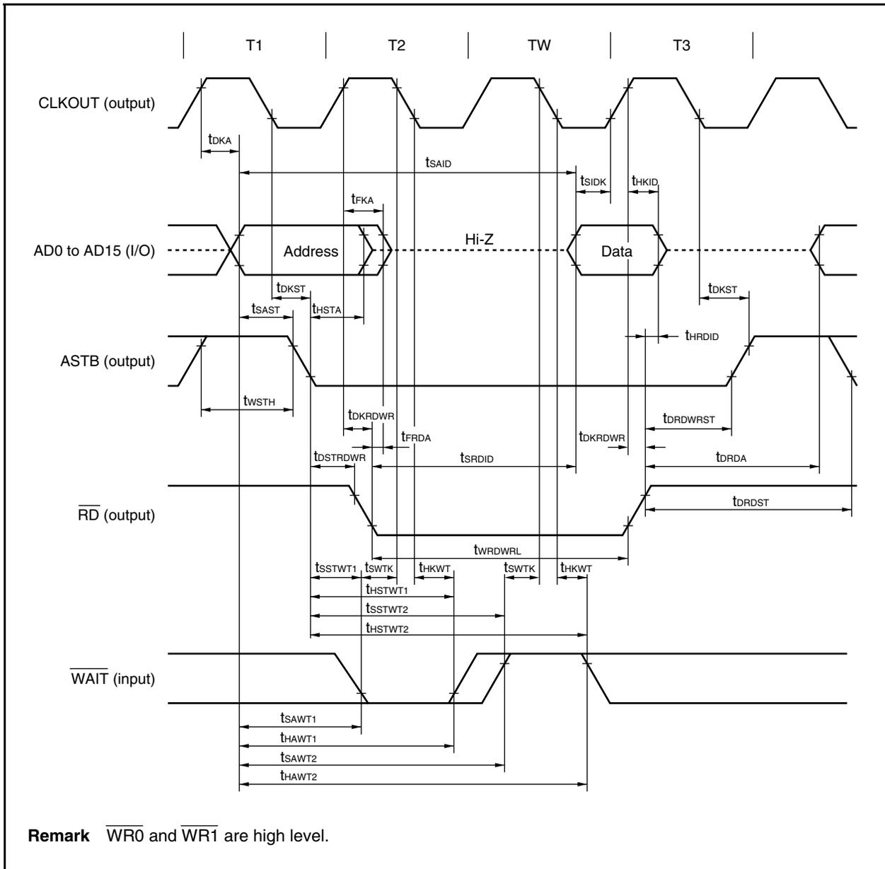
Write Cycle (CLKOUT Synchronous/Asynchronous, 1 Wait)
