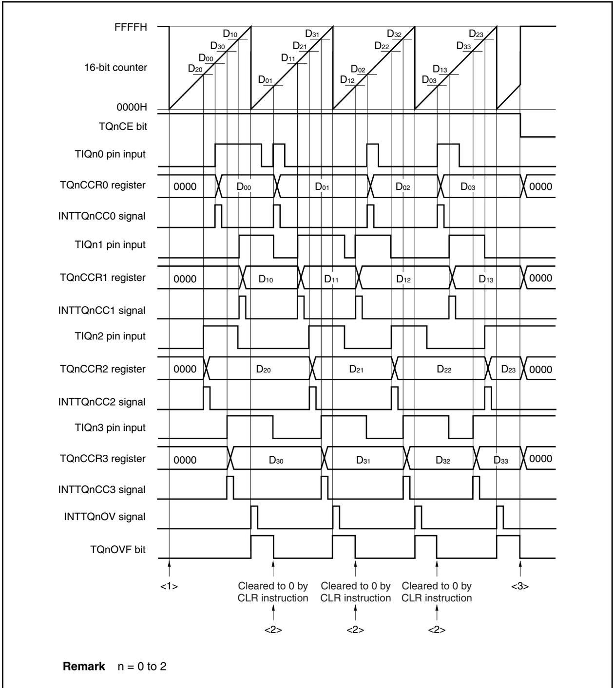
Figure 8-33. Software Processing Flow in Free-Running Timer Mode (Capture Function) (2/2)
