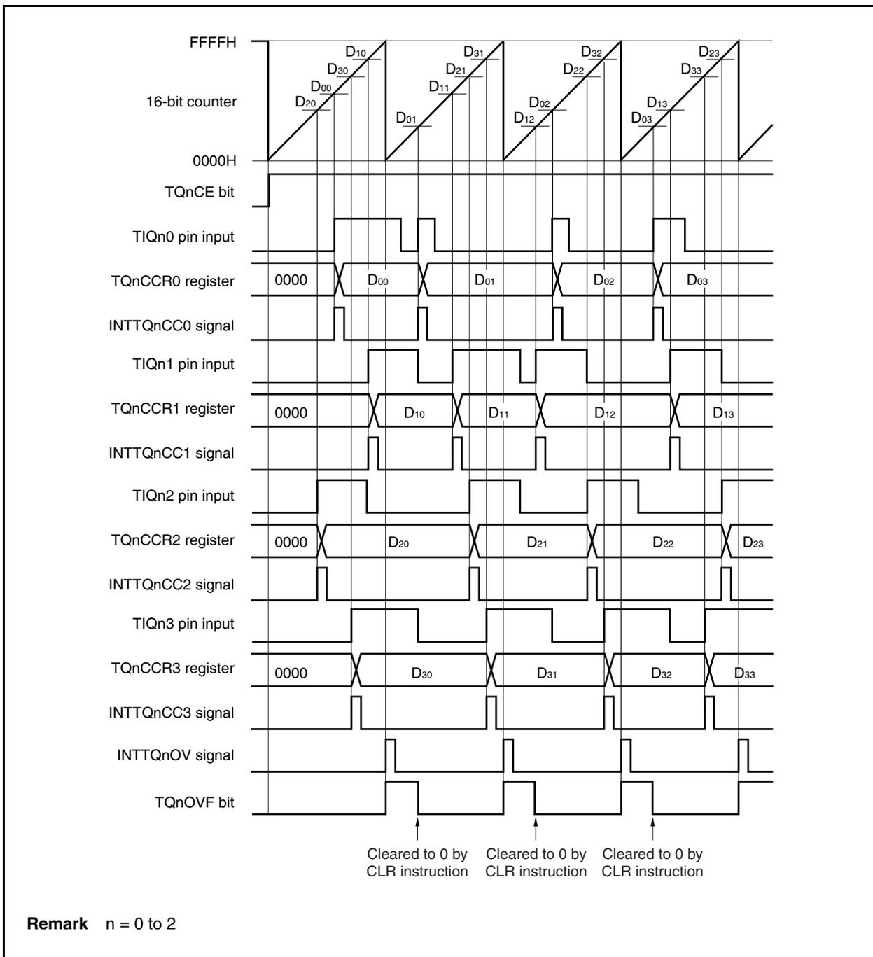
Figure 8-31. Register Setting in Free-Running Timer Mode (1/3)
