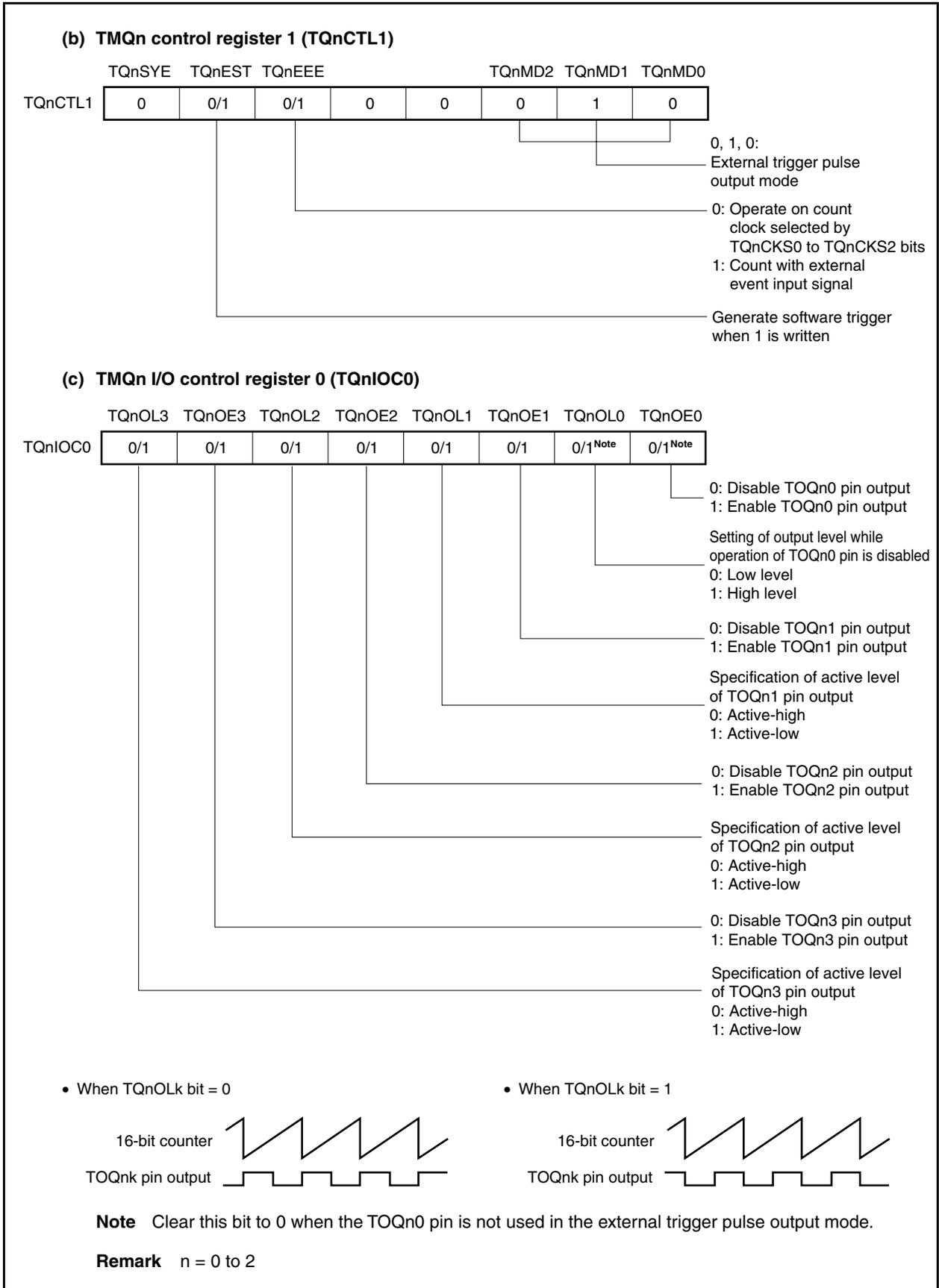
Figure 8-18. Setting of Registers in External Trigger Pulse Output Mode (3/3)
