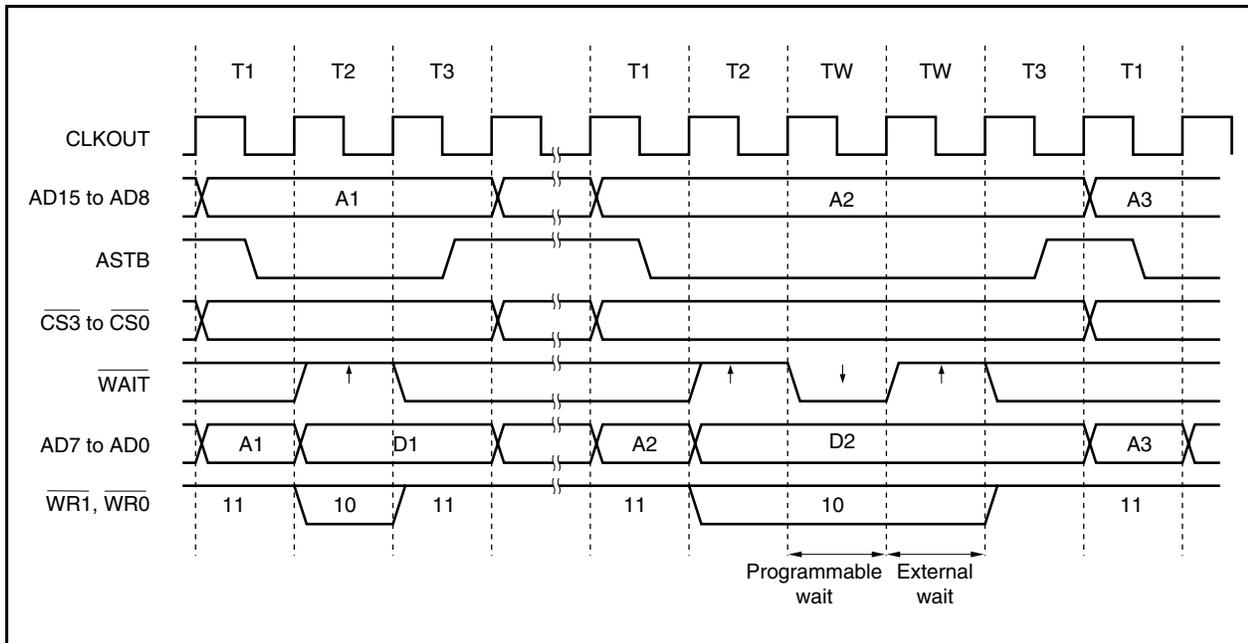
Figure 5-8. Bus Hold Timing (Bus Size: 16 Bits, 16-Bit Access)
