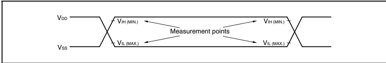
**(2) AC test output measurement points**
