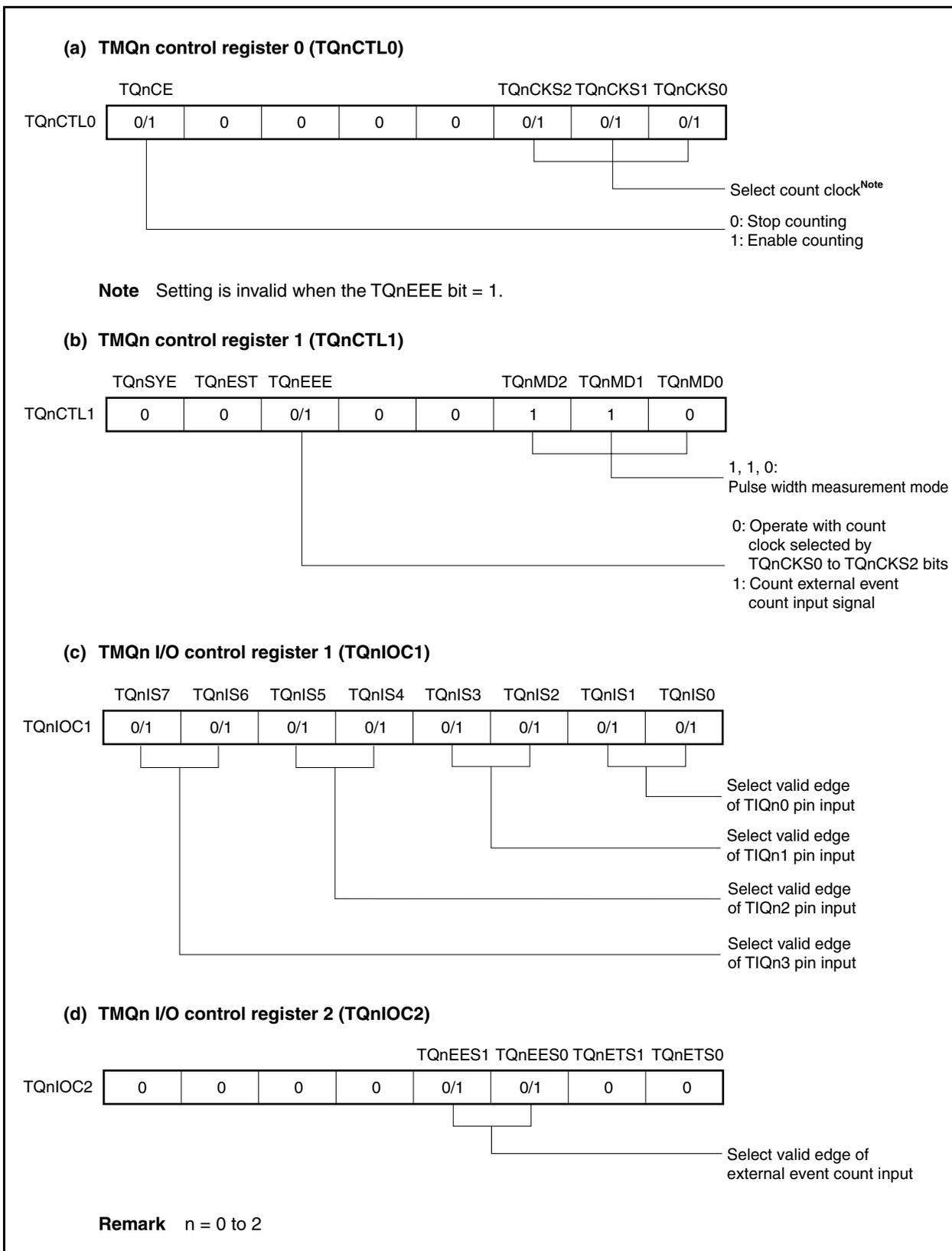
Figure 8-36. Register Setting in Pulse Width Measurement Mode (2/2)
