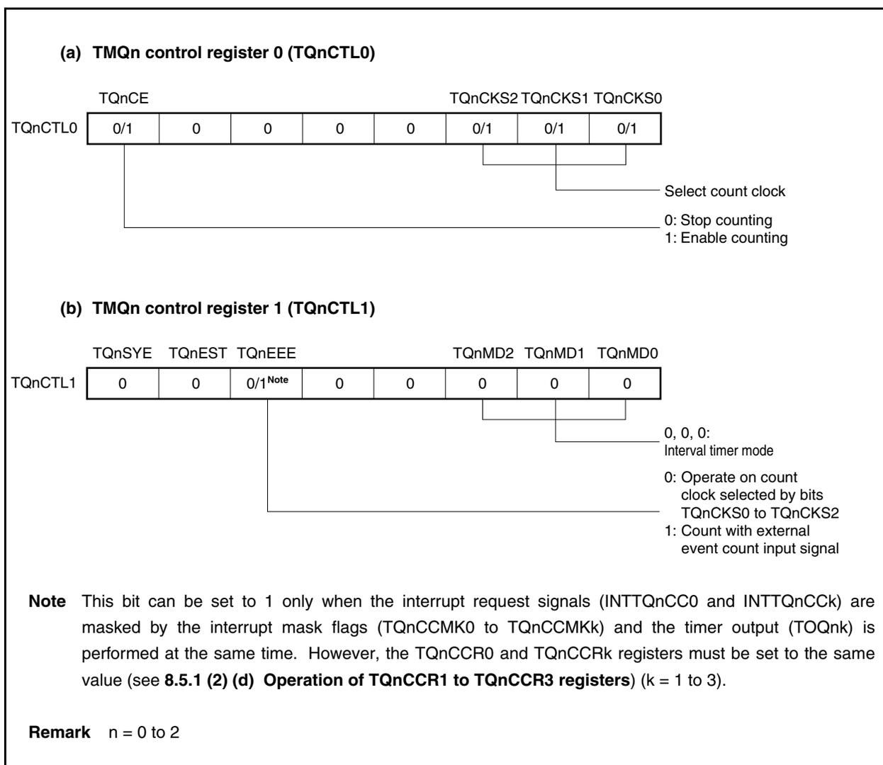
Figure 8-4. Register Setting for Interval Timer Mode Operation (2/2)
