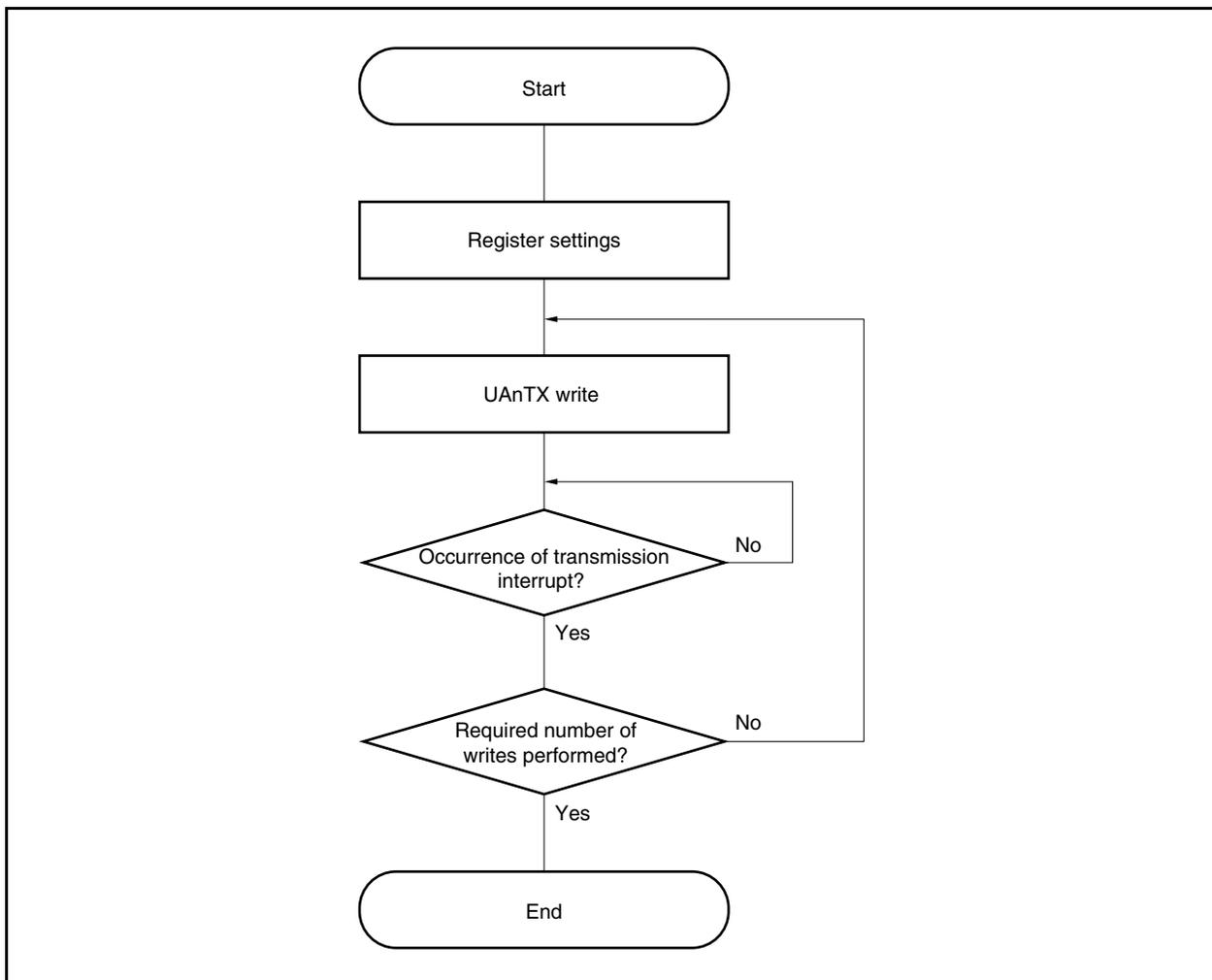
Figure 13-9. Continuous Transmission Operation Timing
