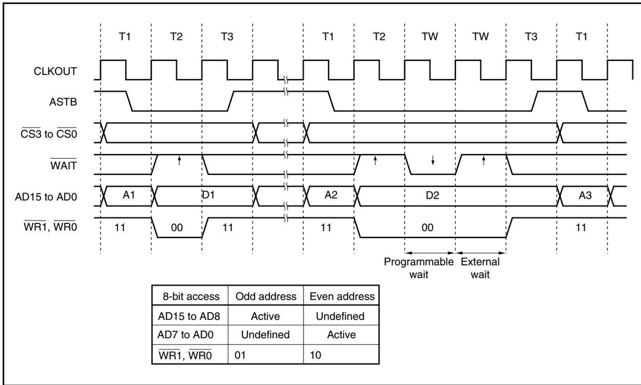
Figure 5-7. Bus Write Timing (Bus Size: 8 Bits)
