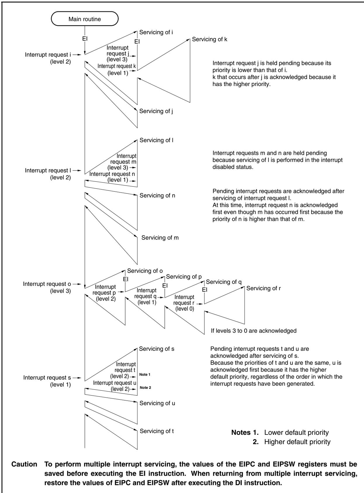
Figure 16-8. Example of Servicing Interrupt Request Signals Simultaneously Generated
