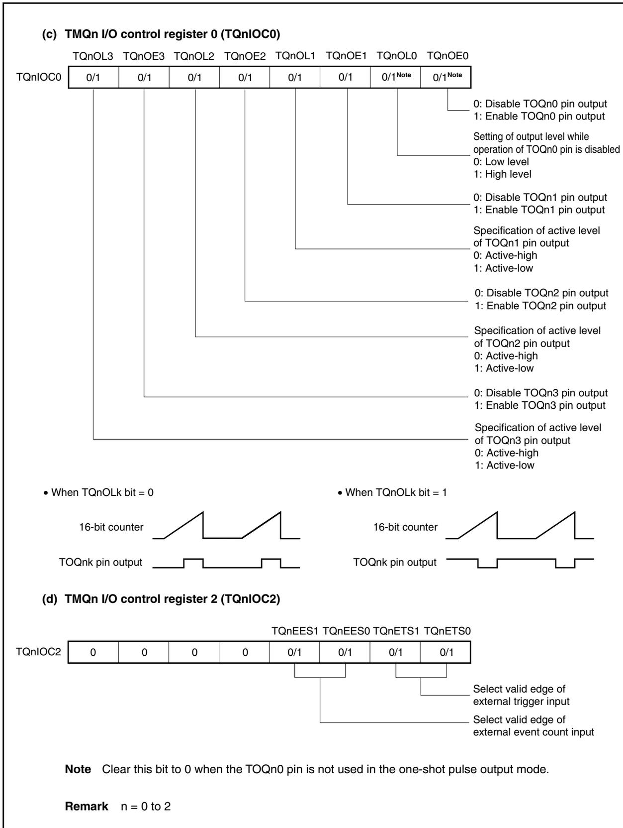
Figure 8-22. Register Setting for Operation in One-Shot Pulse Output Mode (3/3)
