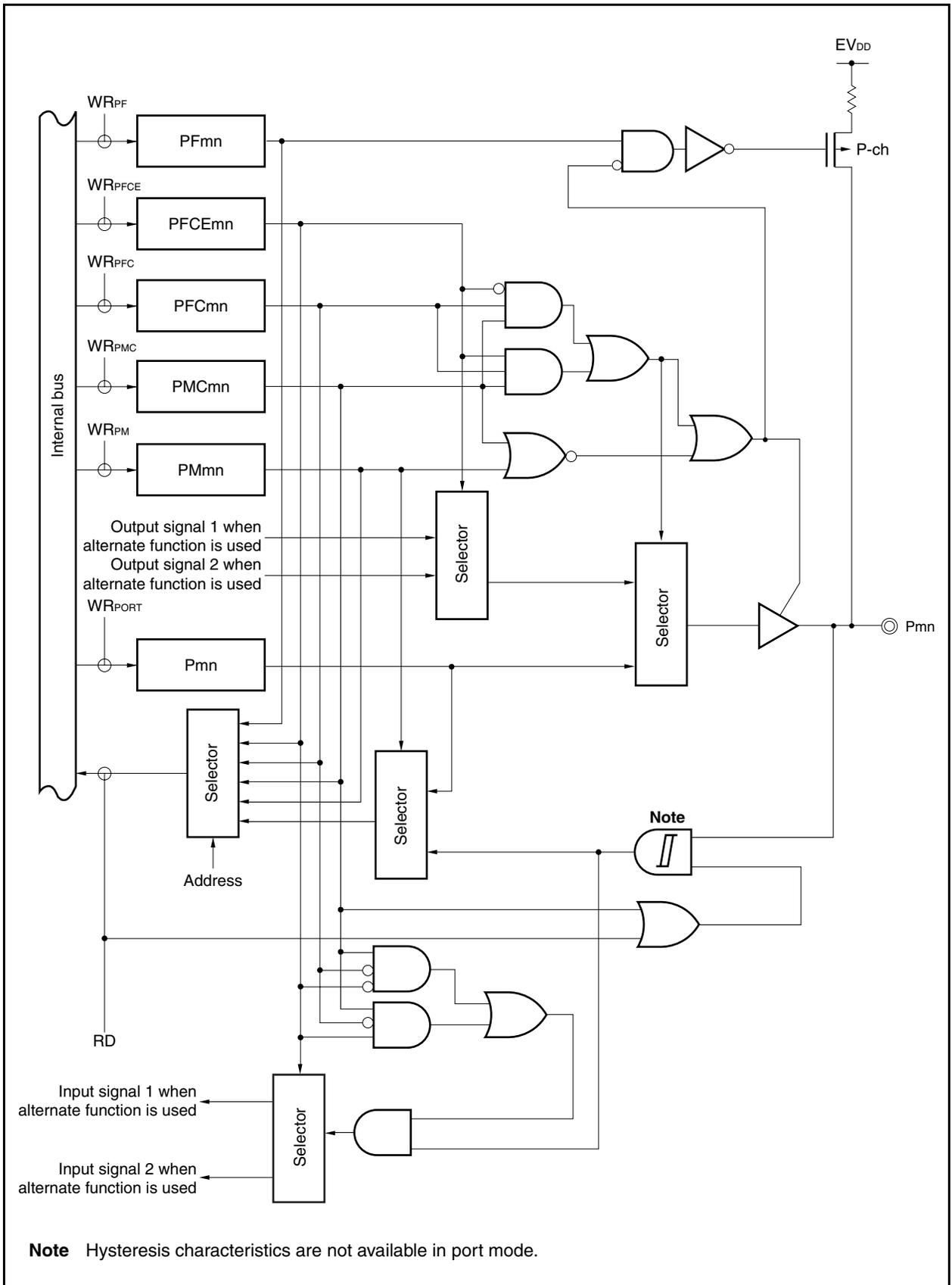
Figure 4-29. Block Diagram of Type W-1
