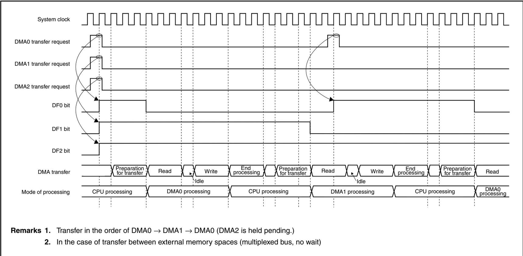
Figure 15-3. Period in Which DMA Transfer Request Is Ignored (1)
