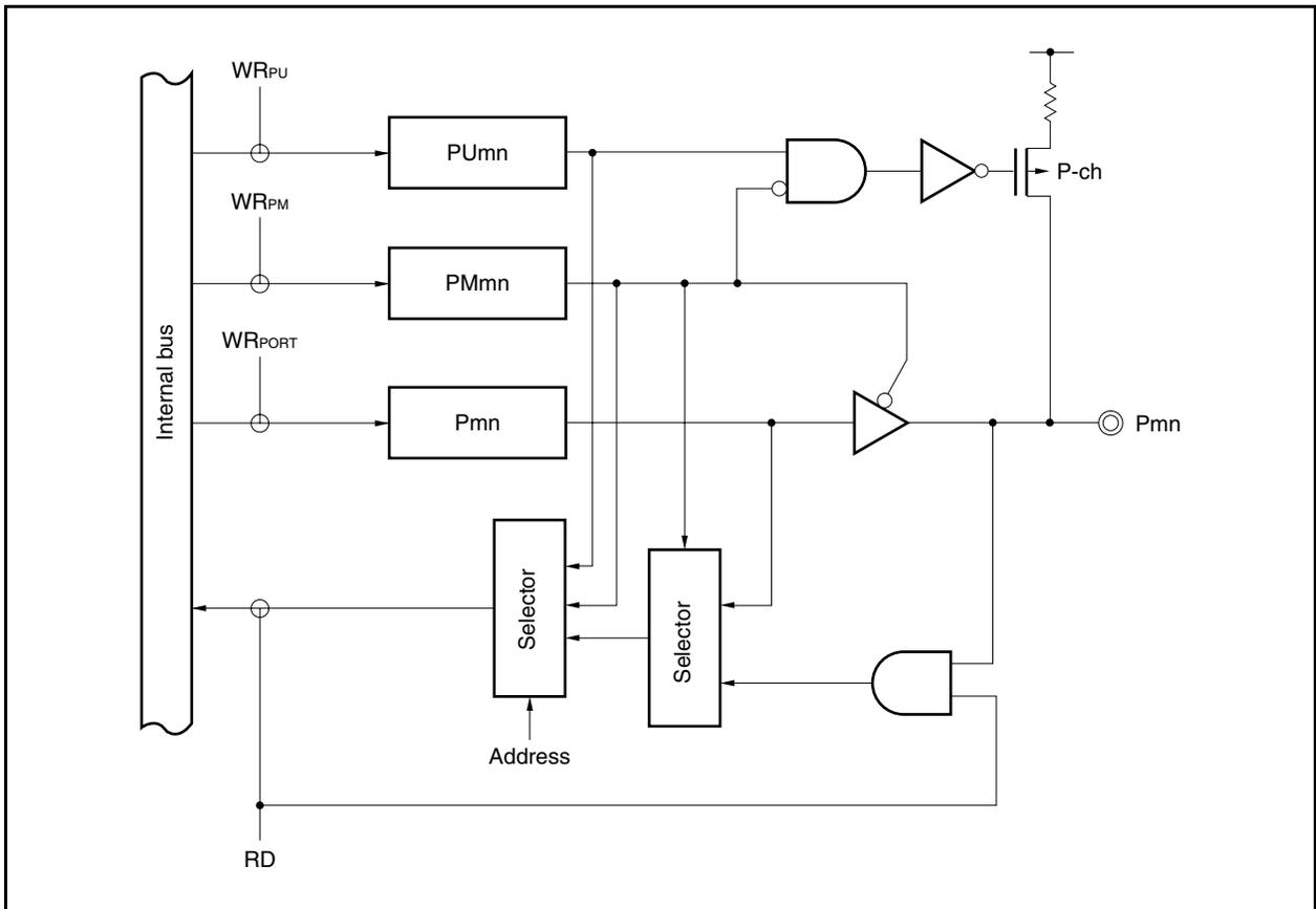
Figure 4-5. Block Diagram of Type D-1
