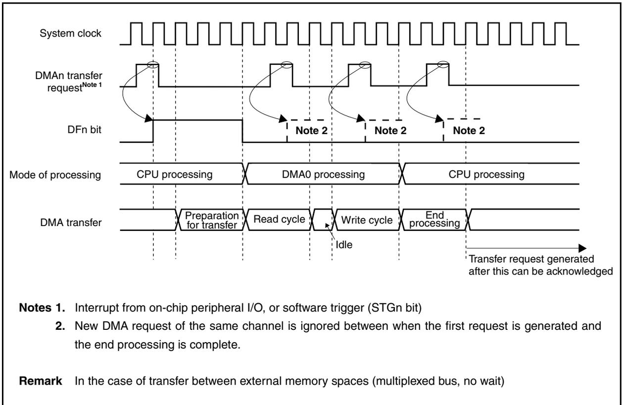
Figure 15-4. Period in Which DMA Transfer Request Is Ignored (2)
