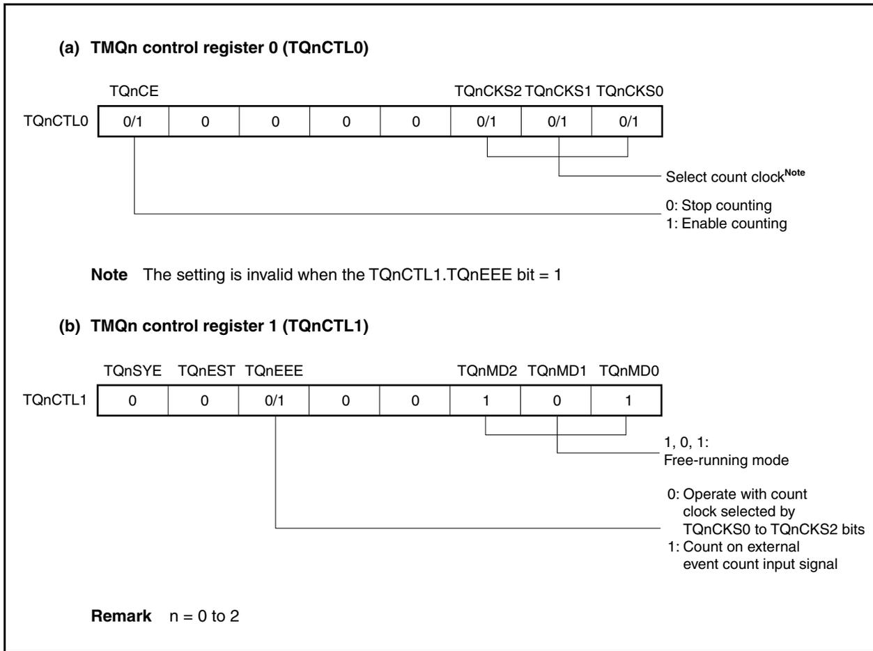
Figure 8-31. Register Setting in Free-Running Timer Mode (2/3)
