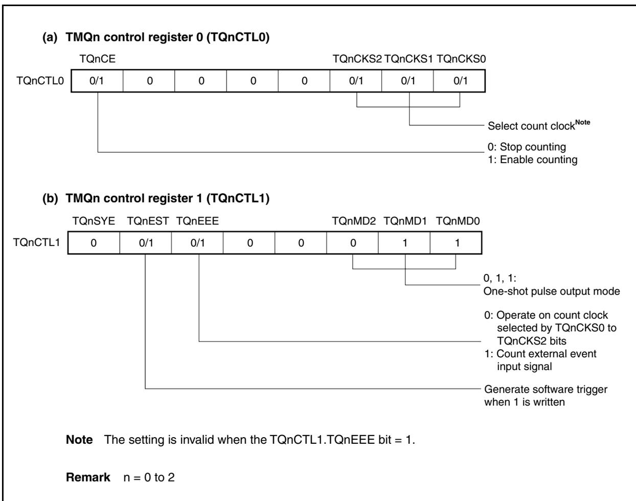
Figure 8-22. Register Setting for Operation in One-Shot Pulse Output Mode (2/3)
