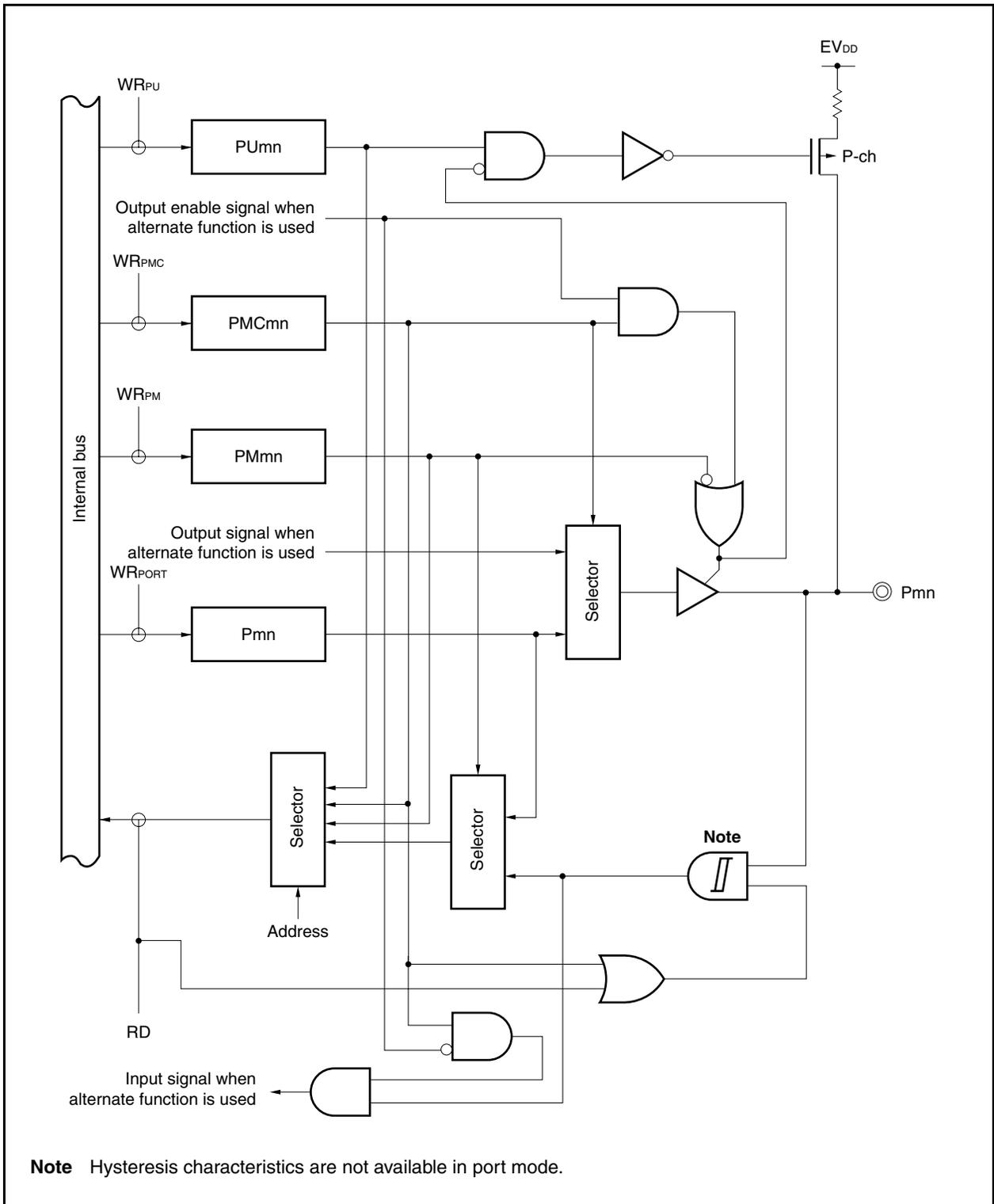
Figure 4-12. Block Diagram of Type G-2
