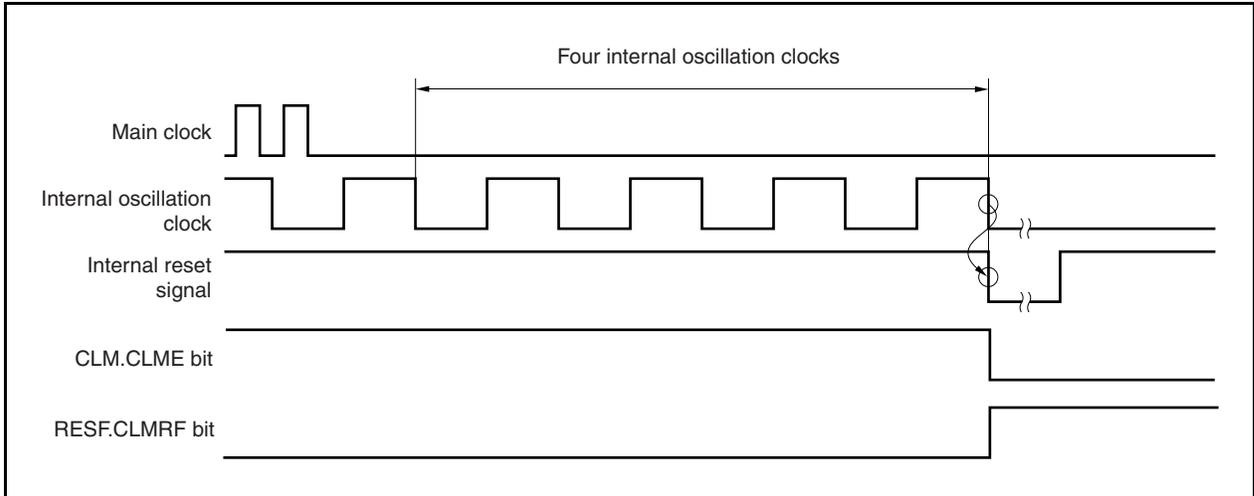
**(2) Clock monitor status after  $\overline{\text{RESET}}$  input**
