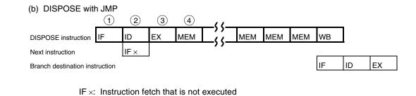
[Description] The pipeline consists of n (Number of register lists) + 4 stages, IF, ID, EX, n + 1 times MEM,
