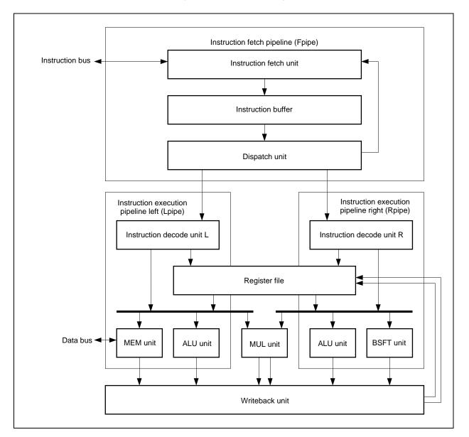
Figure C-2. Pipeline Configuration
