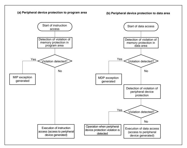
Figure 7-1. Standing of Memory Protection and Peripheral Device Protection
