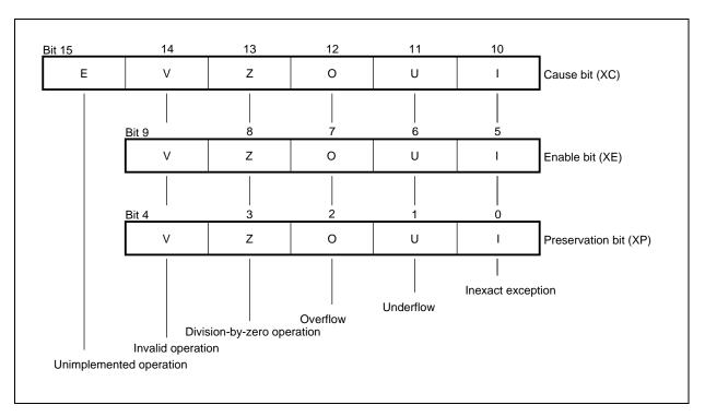
Figure 5-1. Cause, Enable, and Preservation Bits of FPSR Register
