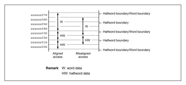
Figure 3-1. Example of Data Placement for Misaligned Access
