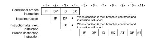
[Description] This figure shows an operation where a Bcond instruction is executed by the instruction execution pipeline right (Rpipe).
