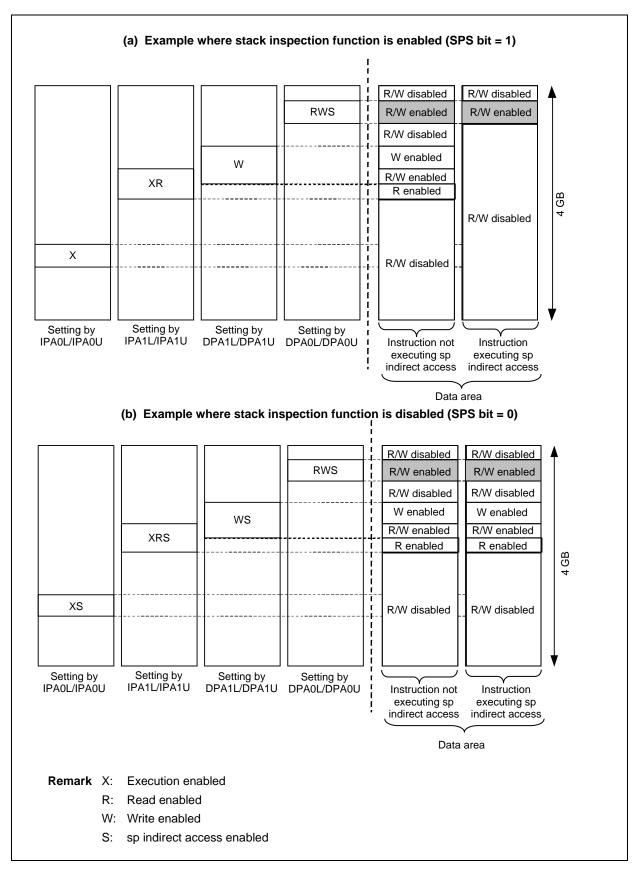
Figure 6-1. Example of Stack Inspection Function
