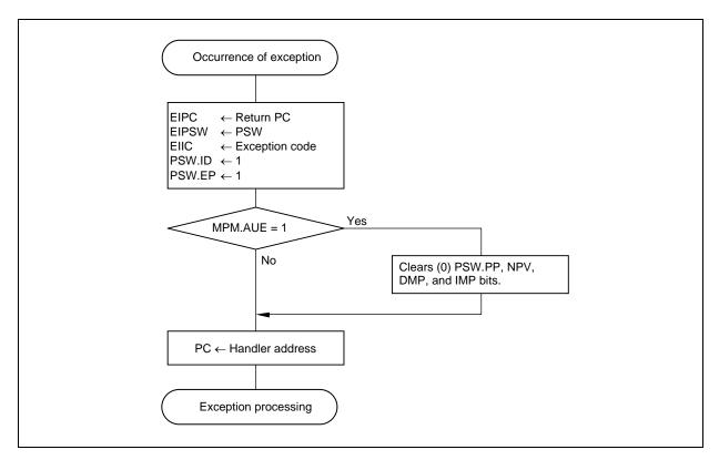
Figure 6-4. Processing Format of El Level Exception Without Acknowledgment Conditions
