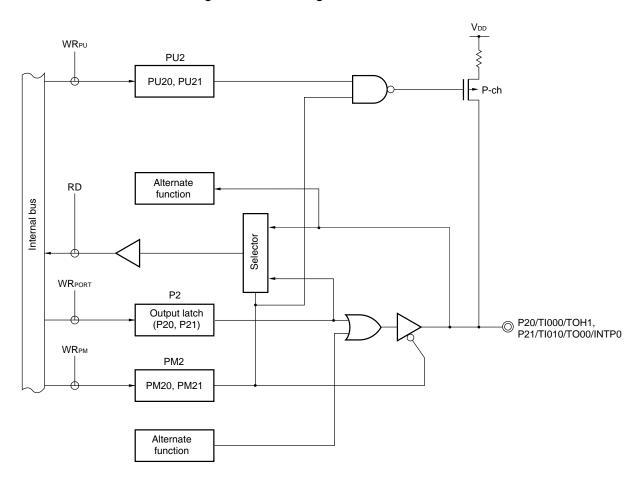
Figure 4-2. Block Diagram of P20 and P21
