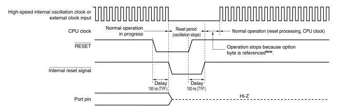
**Note** The operation stop time is 277  $\mu$ s (MIN.), 544  $\mu$ s (TYP.), and 1.075 ms (MAX.).
