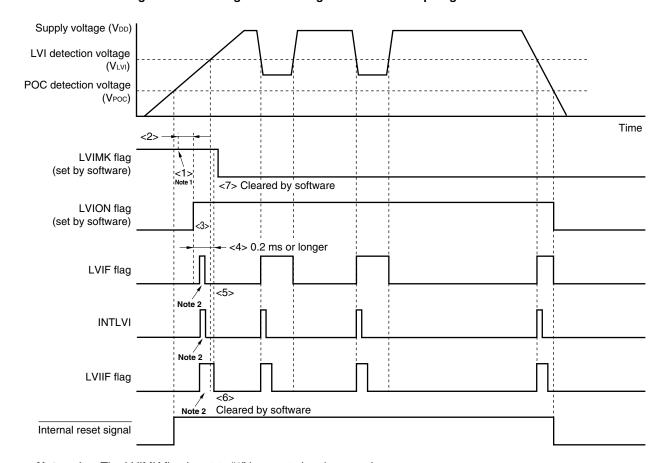
Figure 13-5. Timing of Low-Voltage Detector Interrupt Signal Generation
