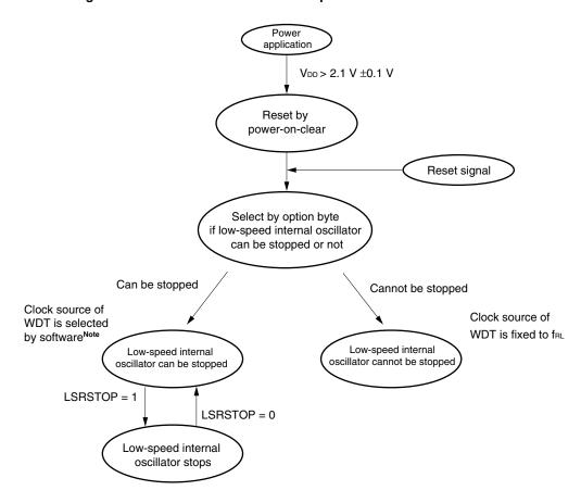
Figure 5-14. Status Transition of Low-Speed Internal Oscillator
