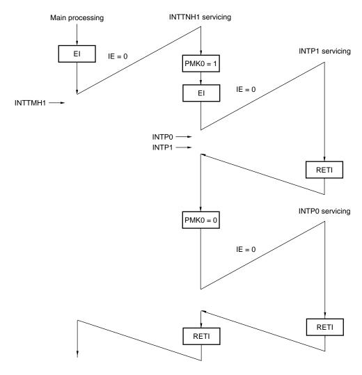
In the interrupt INTTMH1 servicing, servicing is performed such that the INTP1 interrupt is given priority, since the INTP0 interrupt was first masked.
