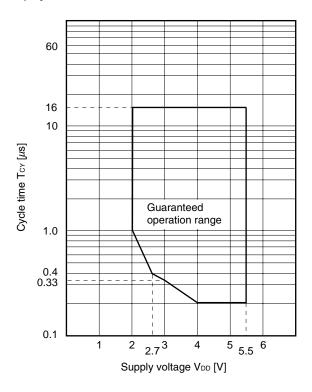
Tcy vs. VDD (High-speed internal oscillator Clock)
