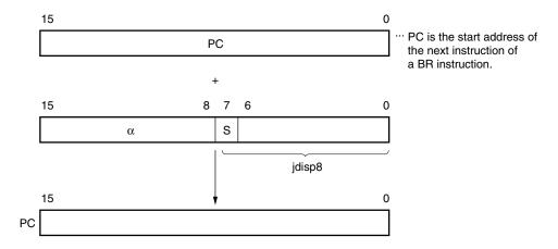
When S = 0,  $\alpha$  indicates that all bits are "0". When S = 1,  $\alpha$  indicates that all bits are "1".
