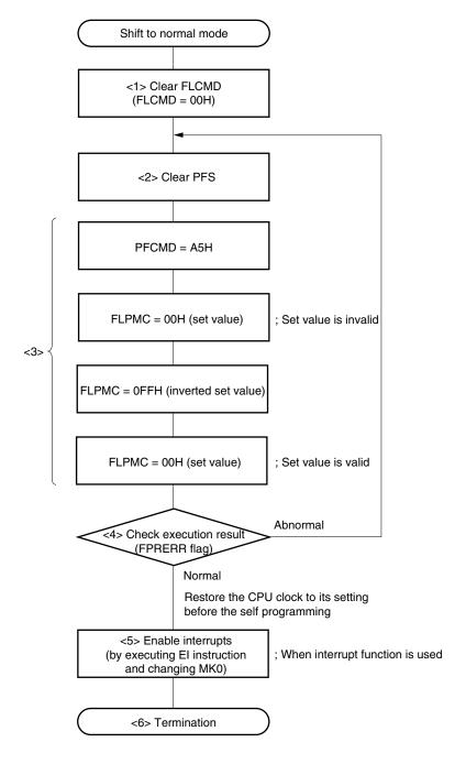
Figure 15-21. Example of Shifting to Normal Mode
