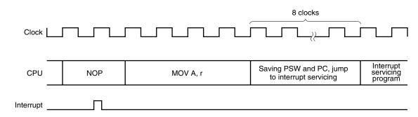
If an interrupt request flag (xxIF) is set at the last clock of the instruction, the interrupt acknowledgment processing starts after the next instruction is executed.
