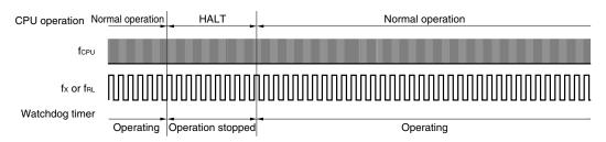
Figure 8-8. Operation in HALT Mode
