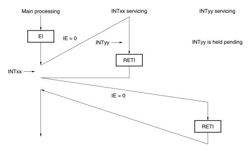
Because interrupts are not enabled in interrupt INTxx servicing (the EI instruction is not issued), interrupt request INTyy is not acknowledged, and multiple interrupts are not generated. The INTyy request is held pending and acknowledged after the INTxx servicing is performed.
