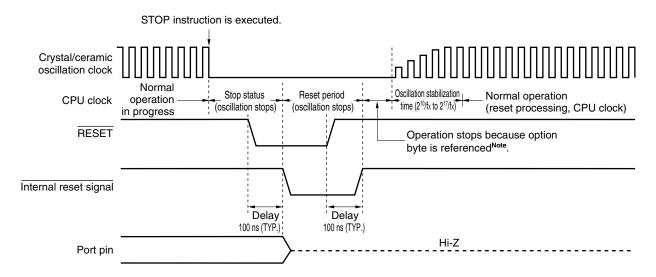
**Note** The operation stop time is 276  $\mu$ s (MIN.), 544  $\mu$ s (TYP.), and 1.074 ms (MAX.).
