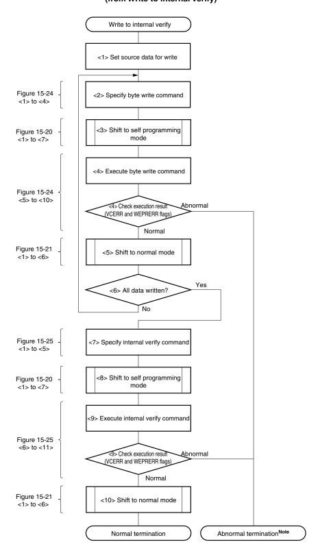
Figure 15-30. Example of Operation When Interrupt-Disabled Time Should Be Minimized (from Write to Internal Verify)
