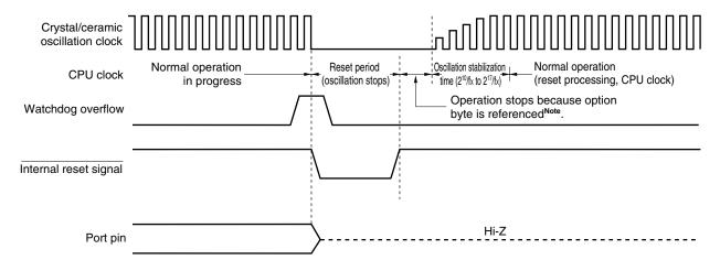
**Note** The operation stop time is 276  $\mu$ s (MIN.), 544  $\mu$ s (TYP.), and 1.074 ms (MAX.).
