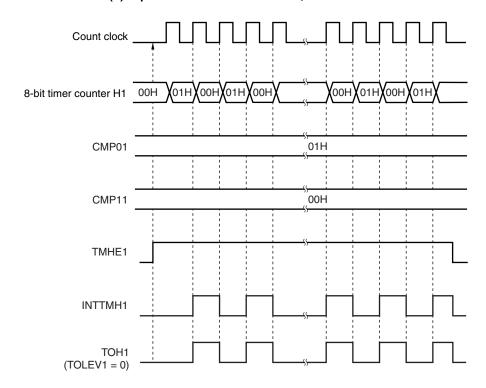
Figure 7-8. Operation Timing in PWM Output Mode (4/4)
