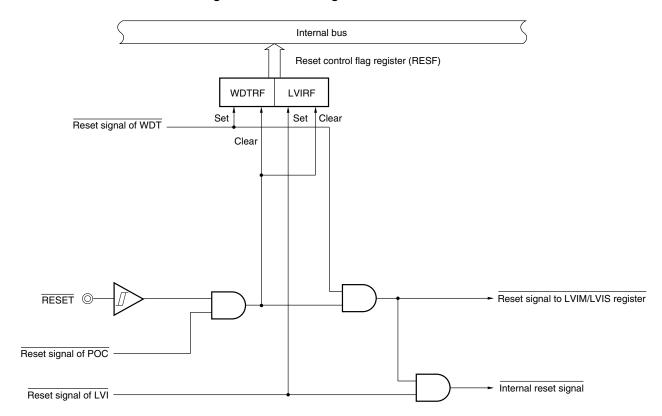
Figure 11-1. Block Diagram of Reset Function
