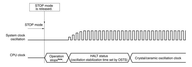
**Note** The operation stop time is 17  $\mu$ s (MIN.), 34  $\mu$ s (TYP.), and 67  $\mu$ s (MAX.).
