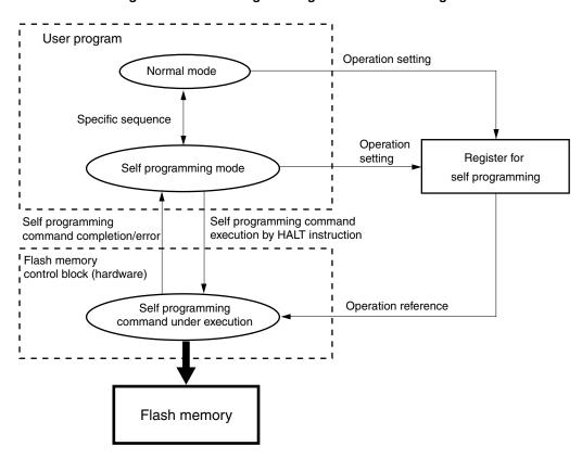
Figure 15-11. Self Programming State Transition Diagram
