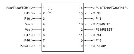
INTP0, INTP1: External interrupt input TI000, TI010: Timer input TO00, TOH1: Timer output P20 to P23: Port 2 P32, P34: Port 3 V<sub>DD</sub>: Power supply P40 to P47: Port 4 Vss: Ground
