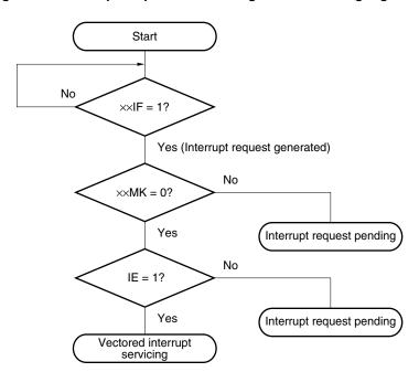
Figure 9-6. Interrupt Request Acknowledgment Processing Algorithm
