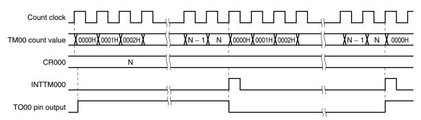
Figure 6-28. Square-Wave Output Operation Timing
