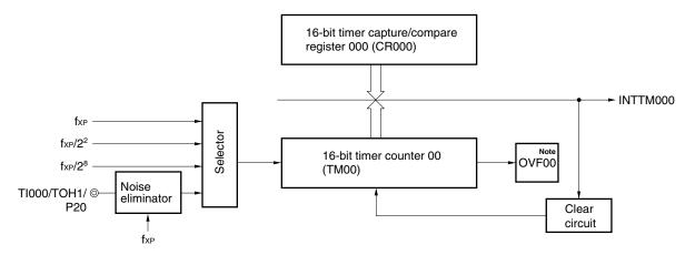
Note OVF00 is set to 1 only when 16-bit timer capture/compare register 000 is set to FFFFH.
