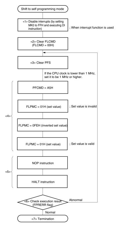
Figure 15-20. Example of Shifting to Self Programming Mode
