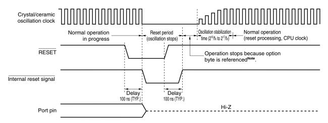
**Note** The operation stop time is 276  $\mu$ s (MIN.), 544  $\mu$ s (TYP.), and 1.074 ms (MAX.).
