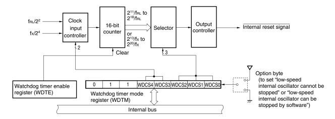
Remarks 1. fr.L: Low-speed internal oscillation clock oscillation frequency
