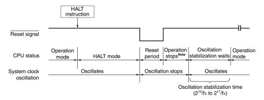
**Note** Operation is stopped (276  $\mu$ s (MIN.), 544  $\mu$ s (TYP.), 1.074 ms (MAX.)) because the option byte is referenced.
