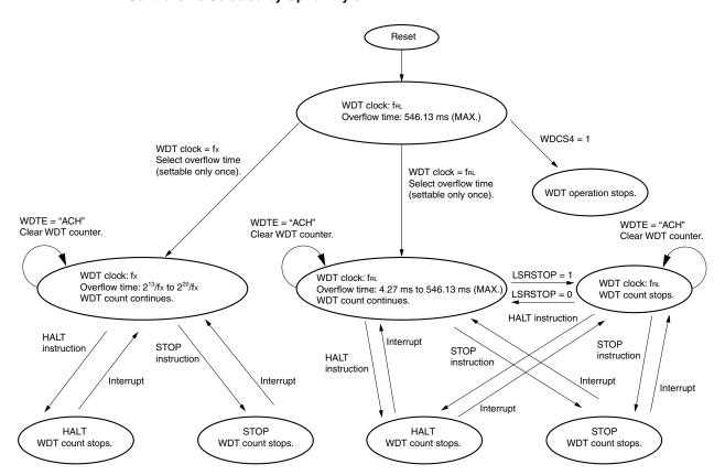
Figure 8-5. Status Transition Diagram When "Low-Speed Internal Oscillator Can Be Stopped by Software" Is Selected by Option Byte
