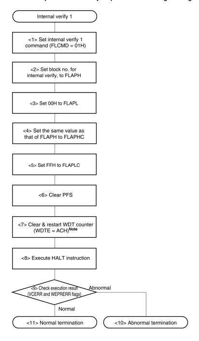
Figure 15-25. Example of Internal Verify 1 Operation in Self Programming Mode
