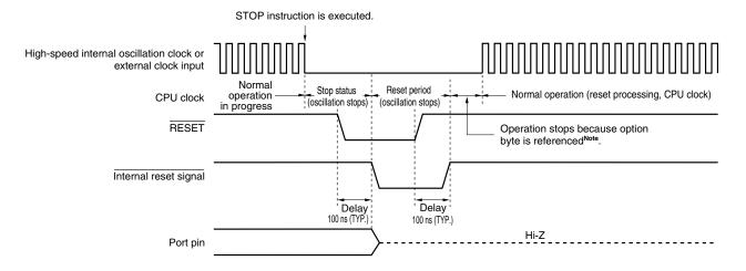
**Note** The operation stop time is 277  $\mu$ s (MIN.), 544  $\mu$ s (TYP.), and 1.075 ms (MAX.).
