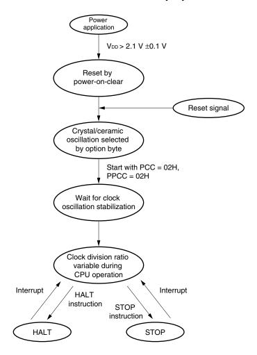
Figure 5-11. Status Transition of Default Start by Crystal/Ceramic Oscillation
