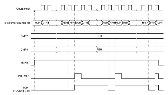
Figure 7-8. Operation Timing in PWM Output Mode (3/4)
