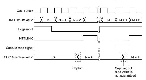
Figure 6-38. Capture Register Data Retention Timing
