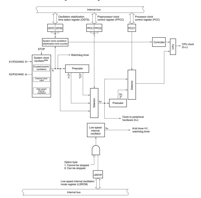
Figure 5-1. Block Diagram of Clock Generators
