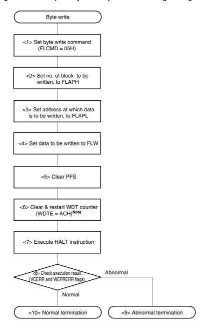
Figure 15-24. Example of Byte Write Operation in Self Programming Mode
