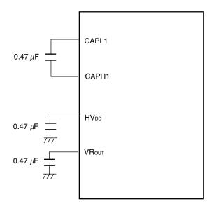
Figure 12-2. Connecting Capacitors
