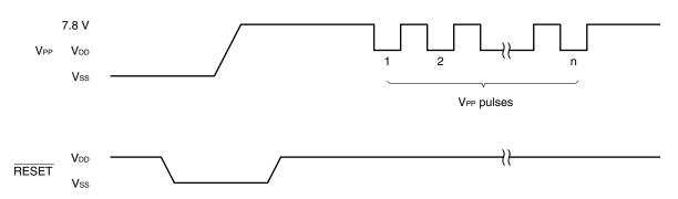
Figure 16-2. Communication Mode Selection Format
