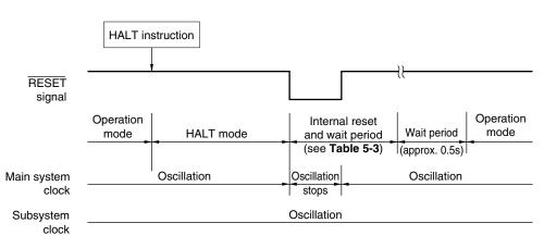
Figure 14-2. Releasing HALT Mode by RESET Input
