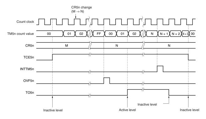
Figure 7-13. Timing of PWM Output Operation (When Active Level = H)
