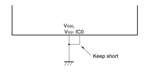
• Connect the IC0 pin directly to the Vsso or Vss1 pin.
