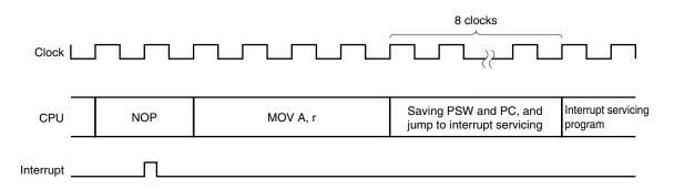
If the interrupt request flag (xxIF) is generated in the final clock of the instruction, interrupt request acknowledgment processing will begin after execution of the next instruction is complete.
