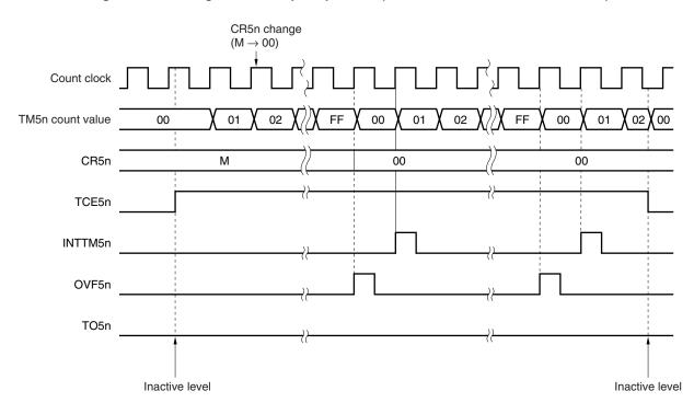
Figure 7-14. Timing of PWM Output Operation (When CR5n = 00H, Active Level = H)
