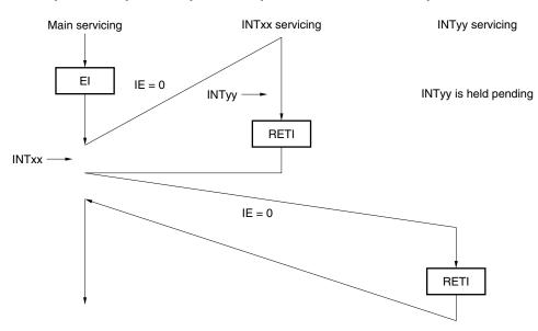
Example 2. Multiple interrupts are not performed because interrupts are disabled
