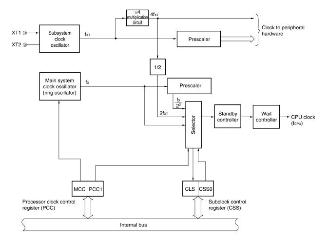
Figure 5-1. Block Diagram of Clock Generator
