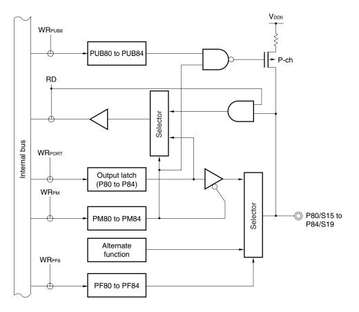
Figure 4-10. Block Diagram of P80 to P84
