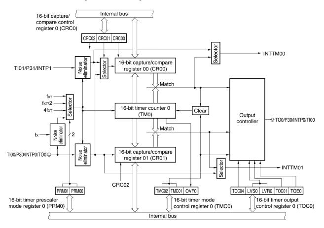
Figure 6-1. Block Diagram of 16-Bit Timer/Event Counter 0
