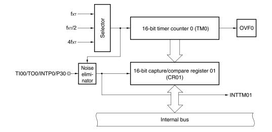
Figure 6-14. Configuration Diagram for Pulse-Width Measurement by Free-Running Counter
