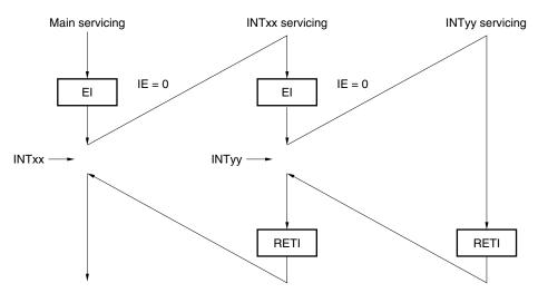
The interrupt request INTyy is acknowledged during the servicing of interrupt INTxx and multiple interrupts are performed. Before each interrupt request is acknowledged, the EI instruction is issued and the interrupt request is enabled.
