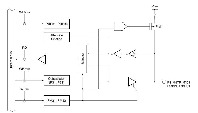
Figure 4-8. Block Diagram of P31 and P33
