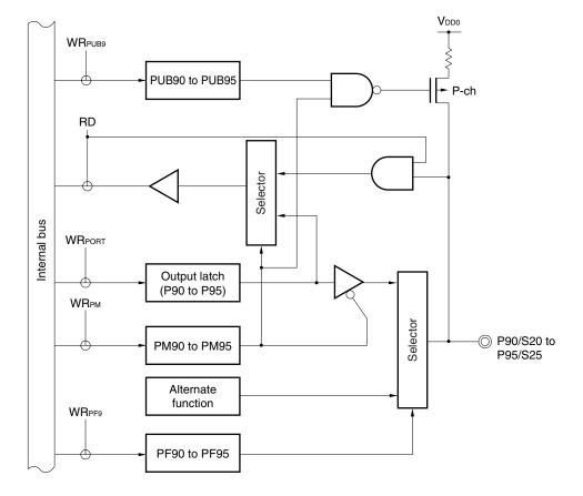
Figure 4-11. Block Diagram of P90 to P95
