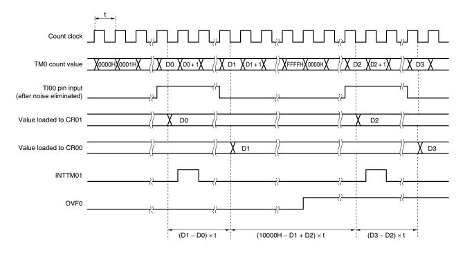
Figure 6-20. Timing of Pulse-Width Measurement Operation with Free-Running Counter and Two Capture Registers (When Rising Edge Is Specified as Valid Edge)
