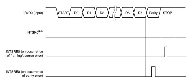
Note INTSR0 is not generated if a receive error is generated when ISRM bit is cleared to 0.
