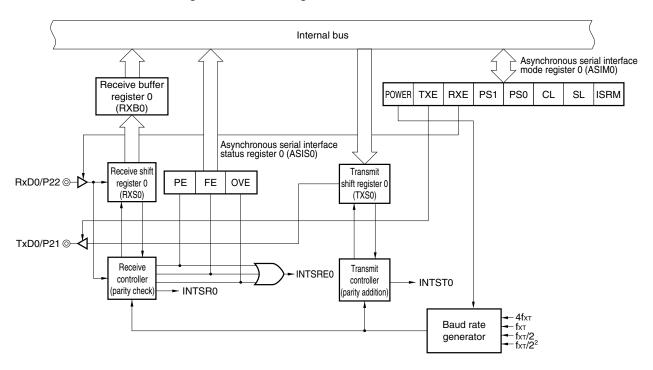
Figure 9-1. Block Diagram of Serial Interface UART0
