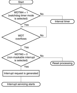
Figure 13-6. Flow from Generation of Non-Maskable Interrupt Request to Acknowledgment
