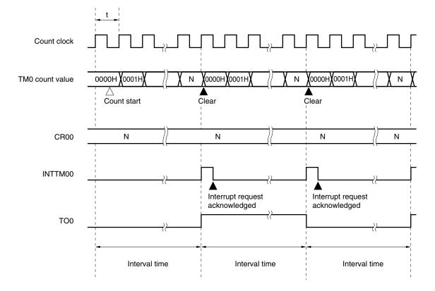
Figure 6-9. Interval Timer Operation Timing
