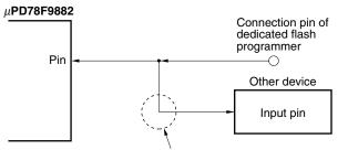
If the signal output by the dedicated flash programmer affects another device in the flash memory programming mode, isolate the signals of the other device.
