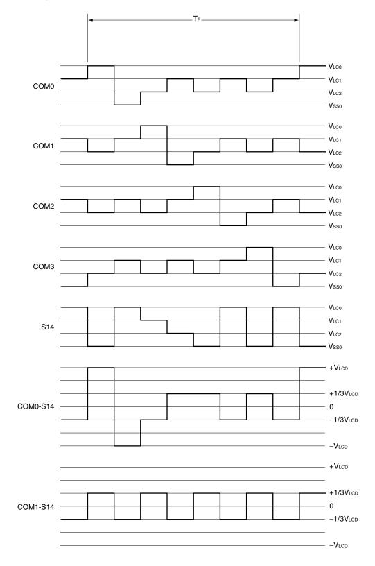
Figure 10-15. Four-Time Slot LCD Drive Waveform Examples (1/3 Bias Mode)
