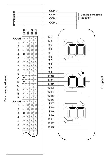
Figure 10-11. Example of Connecting Static LCD Panel
