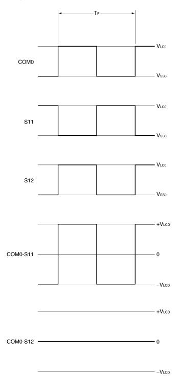
Figure 10-12. Static LCD Drive Waveform Examples
