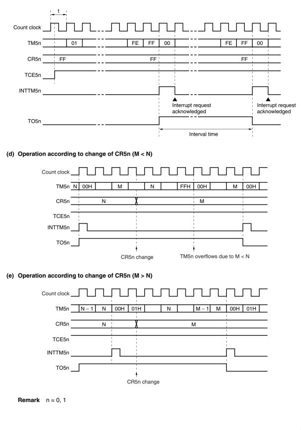
Figure 7-8. Timing of Interval Timer Operation (2/2)
