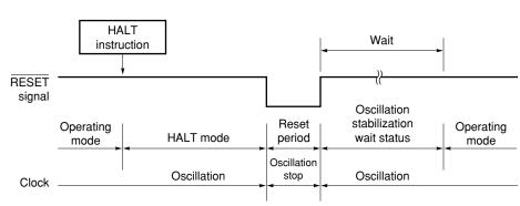
Figure 13-3. Releasing HALT Mode by RESET Input
