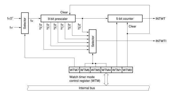
Figure 8-1. Watch Timer Block Diagram
