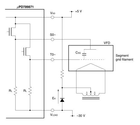
Figure 11-9. Leakage Emission Caused by Csg
