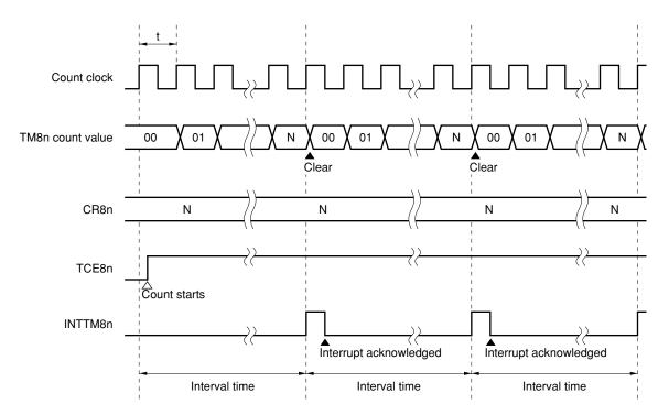
Figure 7-5. Interval Timer Operation Timing
