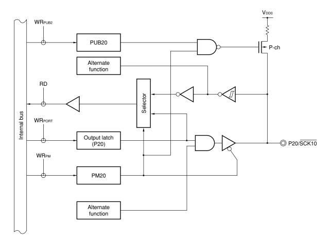
Figure 4-4. Block Diagram of P20
