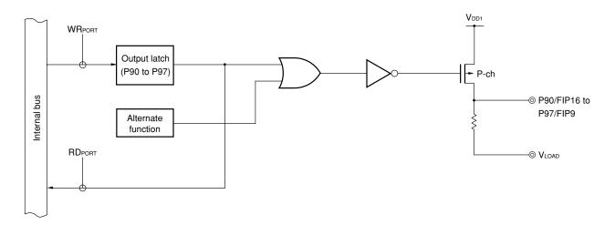
Figure 4-10. Block Diagram of P90 to P97 (µPD78F9872)
