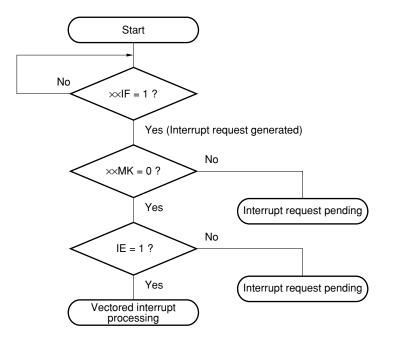
Figure 12-9. Interrupt Acknowledgement Program Algorithm
