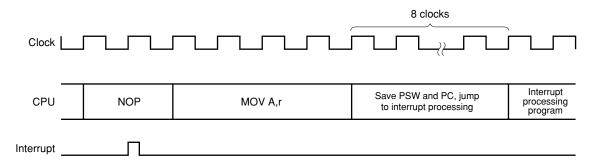
If an interrupt request flag ( $\times$  IF) is set at the last clock of the instruction, the interrupt acknowledgement processing starts after the next instruction is executed.
