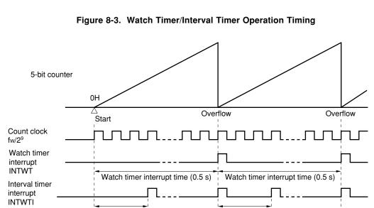
Caution When operation of the watch timer and 5-bit counter has been enabled by setting the watch timer mode control register (WTM) (setting WTM0 (bit 0 of WTM) to 1), the time until the first interrupt request after this setting will not be exactly the same as the time set by WTM3 (bit 3 of WTM). This is because the 5-bit counter starts counting one cycle after the output of the 9-bit prescaler. The INTWT signal will be generated at the set time from its second generation.
