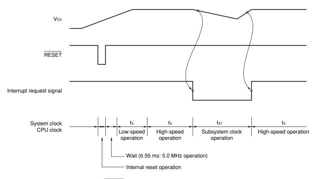
Figure 5-8. Switching Between System Clock and CPU Clock
