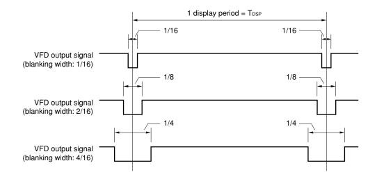
Figure 11-5. Blanking Width of VFD Output Signal
