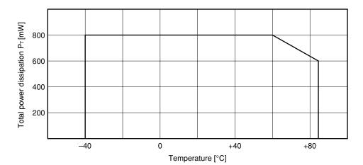
Figure 11-11. Total Power Dissipation  $P_T$  (T<sub>A</sub> = -40 to +85°C)
