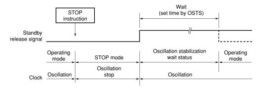
**Remark** The broken lines indicate the case where the interrupt request that has released the standby mode is acknowledged.
