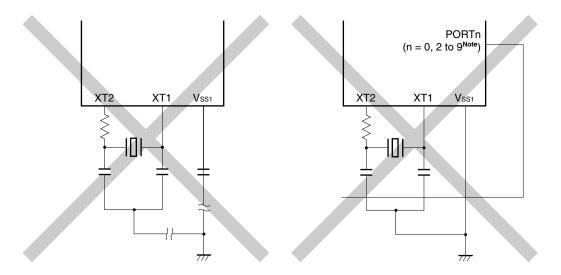
Figure 5-7. Examples of Incorrect Resonator Connection (2/2)
