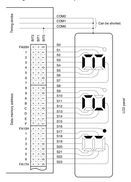
Figure 16-11. Connection Example of Static LCD Panel
