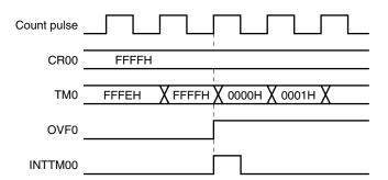
Figure 7-31. Operation Timing of OVF0 Flag
