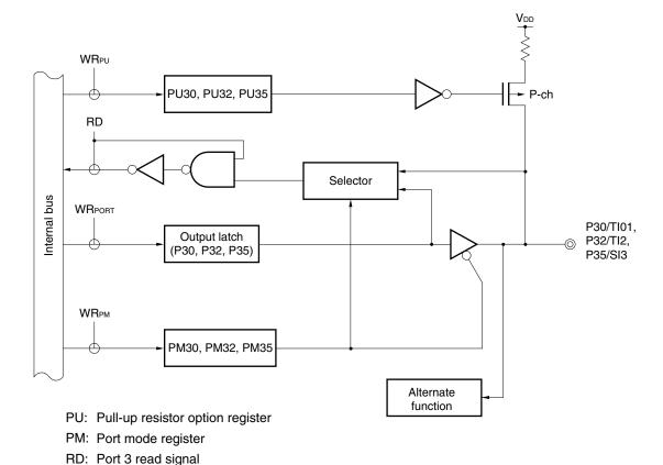
Figure 4-5. Block Diagram of P30, P32, and P35
