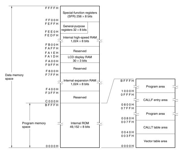
Figure 3-1. Memory Map (for  $\mu$ PD780957(A))
