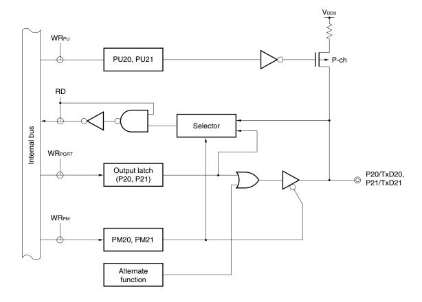
Figure 4-3. Block Diagram of P20 and P21
