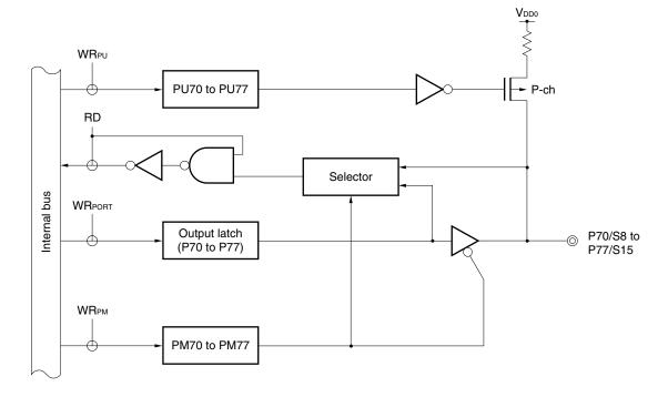
Figure 4-13. Block Diagram of P70 to P77
