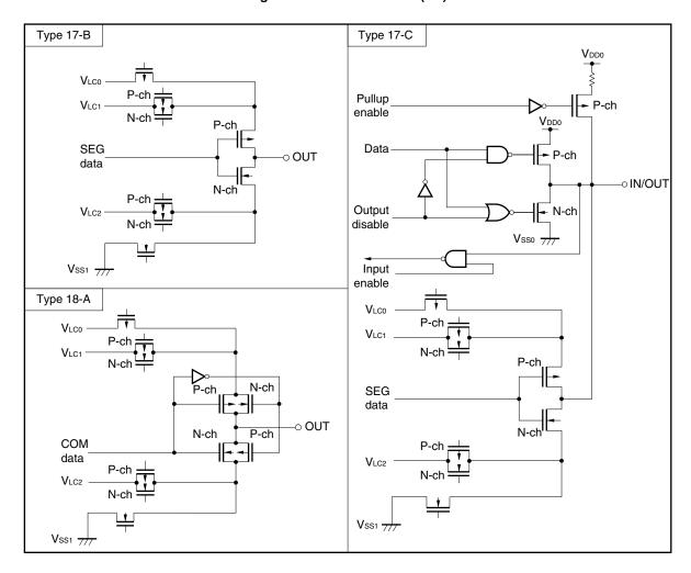
Figure 2-4. Pin I/O Circuits (2/2)
