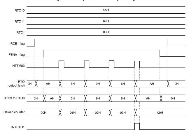
Figure 6-4. Example of Real-Time Output Timing
