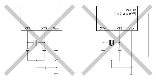
Figure 5-9. Examples of Incorrect Resonator Connection (2/2)
