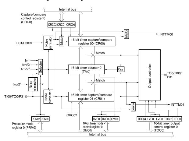
Figure 7-1. Block Diagram of 16-Bit Timer/Event Counter 0
