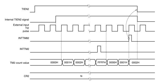
Figure 8-7. Timing of External Event Counter Operation
