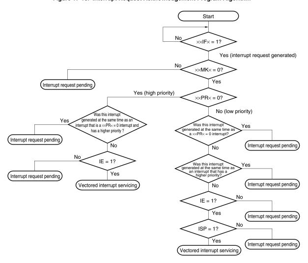
Figure 17-10. Interrupt Request Acknowledgement Program Algorithm
