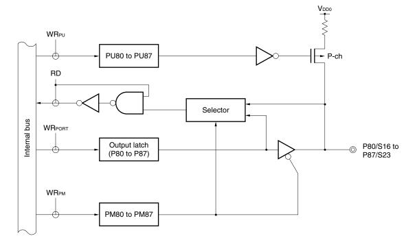
Figure 4-14. Block Diagram of P80 to P87
