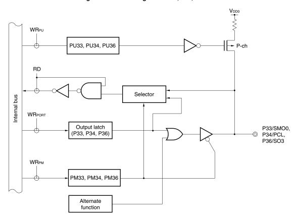
Figure 4-7. Block Diagram of P33, P34, and P36
