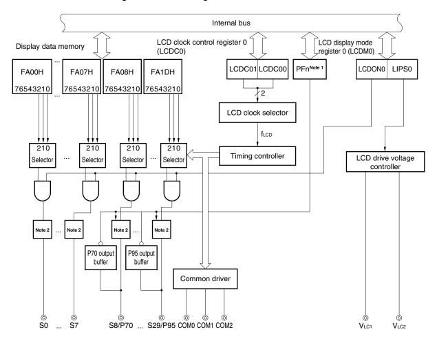
Figure 16-1. Block Diagram of LCD Controller/Driver
