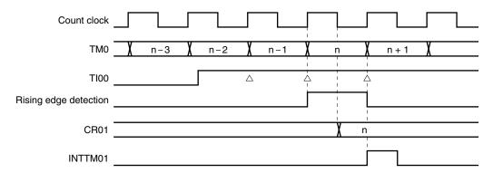
Figure 7-18. Timing of Two-Pulse-Width Measurement Operation with Free-Running Counter (with Both Edges Specified)
