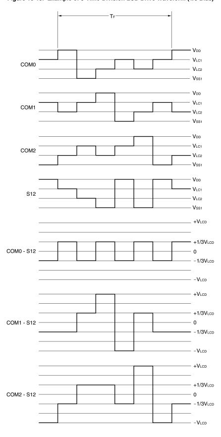
Figure 16-15. Example of 3-Time-Division LCD Drive Waveform (1/3 Bias)
