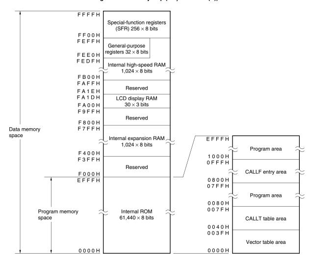
Figure 3-2. Memory Map (for  $\mu$ PD780958(A))
