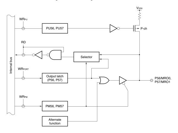
Figure 4-10. Block Diagram of P56 and P57
