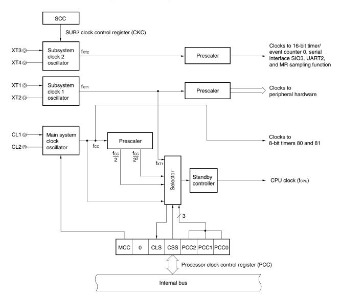
Figure 5-1. Block Diagram of Clock Generator
