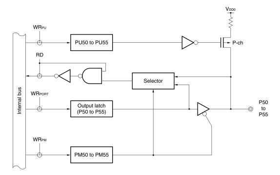
Figure 4-9. Block Diagram of P50 to P55
