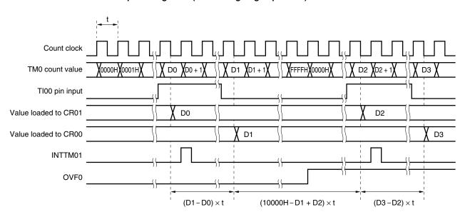
Figure 7-20. Timing of Pulse-Width Measurement Operation with Free-Running Counter and Two Capture Registers (with Rising Edge Specified)
