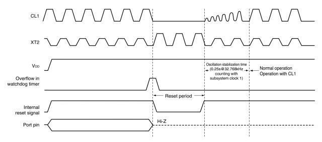
Figure 19-4. Reset Timing After Power Application
