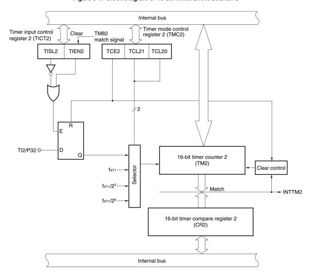
Figure 8-1. Block Diagram of 16-Bit Timer/Event Counter 2
