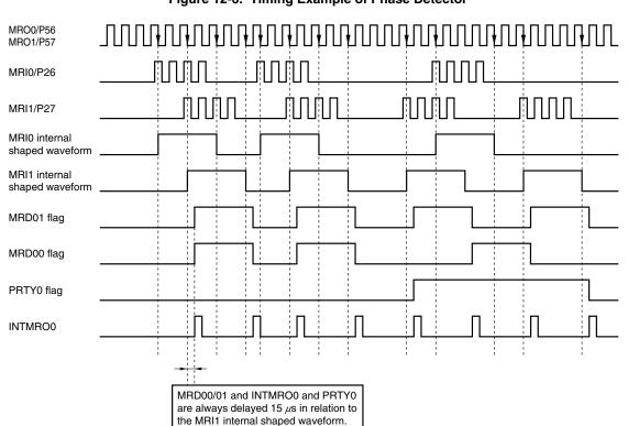
Figure 12-6. Timing Example of Phase Detector
