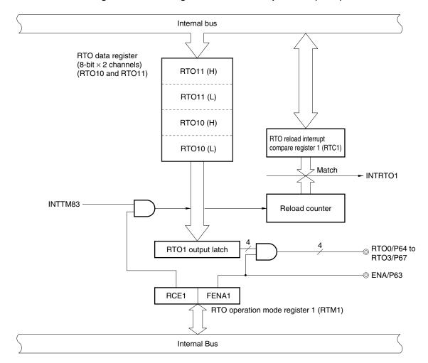
Figure 6-1. Block Diagram of Real-Time Output Port 1 (RTO1)
