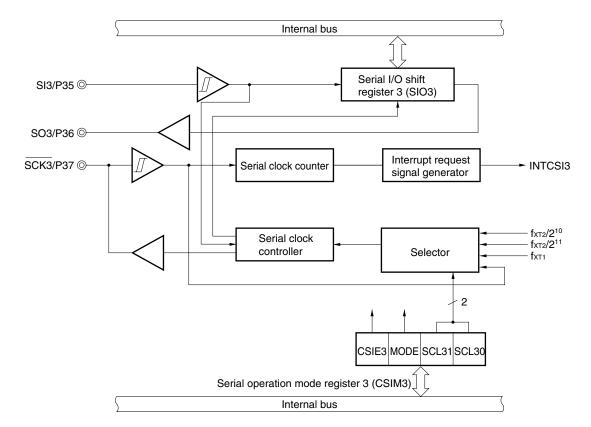
Figure 15-1. Block Diagram of Serial Interface SIO3
