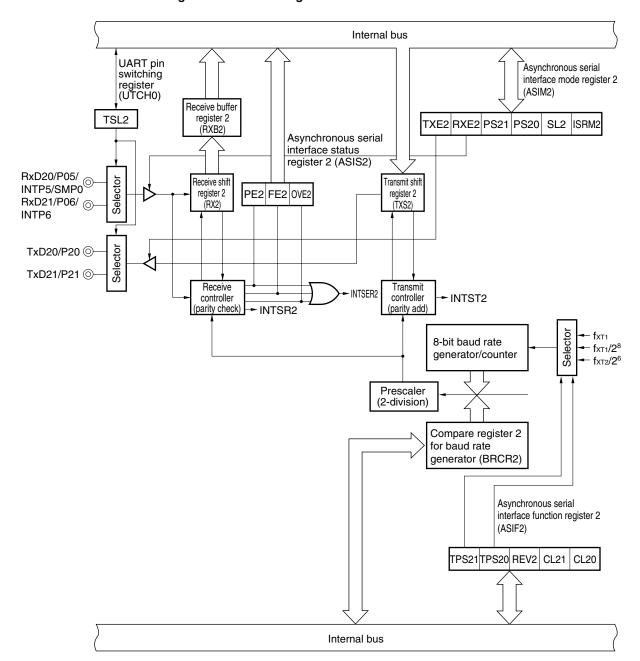
Figure 14-1. Block Diagram of Serial Interface UART2
