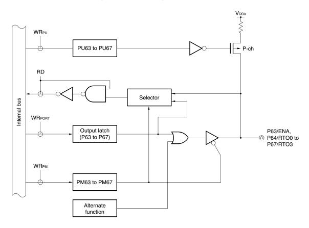
Figure 4-12. Block Diagram of P63 to P67
