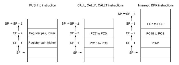
Figure 3-9. Data Restored from Stack Memory
