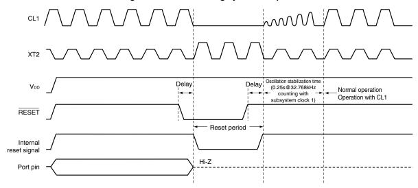
Figure 19-3. Reset Timing by Watchdog Timer Overflow
