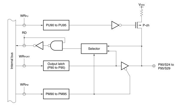
Figure 4-15. Block Diagram of P90 to P95
