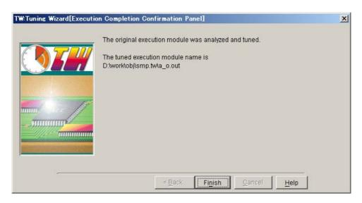
To complete wizard processing (performance analysis or tuning), check a message to report that the TW850 has completed wizard processing (performance analysis or tuning) is displayed in the message display area, and click the <Finish> button.
