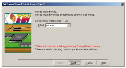
To continue the wizard processing (performance analysis or tuning), check a message to report that the TW850 has started the wizard processing (performance analysis or tuning) is displayed in the message display area, and click the  $\langle \underline{N} \text{ext} \rangle$  button.
