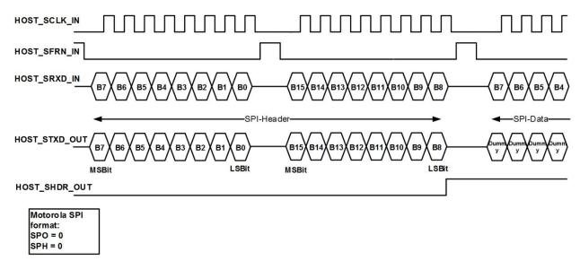
Figure 3-10: SPI Slave Timing
