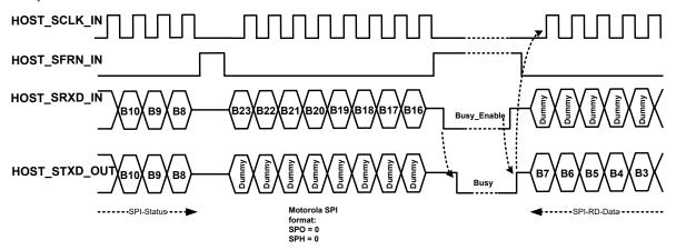
Figure 3-12: SPI Read-Timing (Busy\_POL=0)
