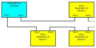
Figure 8-1: Network topologies with the TPS-1
