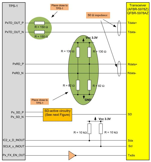
Figure B-8: 100BASE-FX Interface Example
