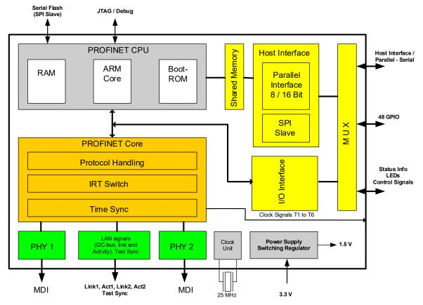
Figure 1-2: TPS-1 Block Diagram
