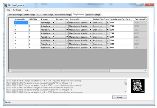
Figure A-5: Configuration of Diagnosis Channel if needed
