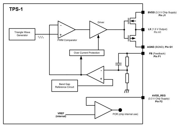
Figure 8-2: Internal voltage regulator
