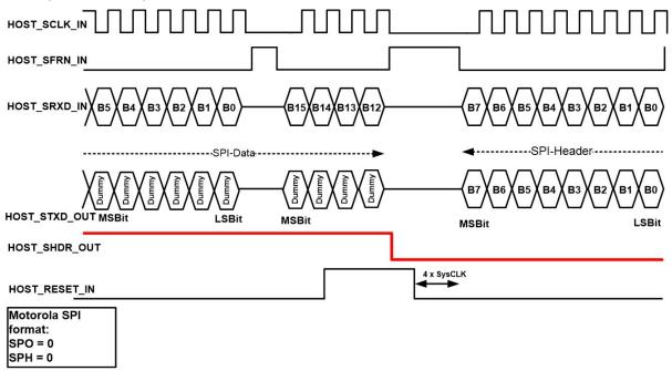
Figure 3-16: SPI Slave Reset Timing
