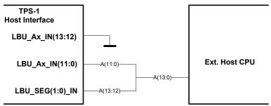
Figure 3-3: TPS-1 with address page 4 Kbyte
