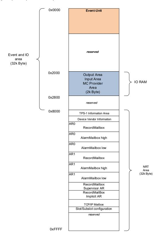
Figure 4-1: TPS-1 Shared Memory Structure (Dual Ported RAM)
