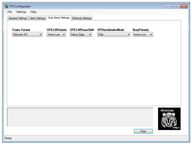
Figure A-3: Serial host interface configuration
