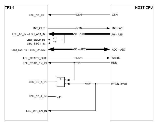
Figure 3-6: Connection example for an 8-bit data bus
