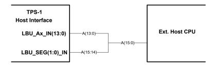
Figure 3-2: TPS-1 with address page 16 Kbyte
