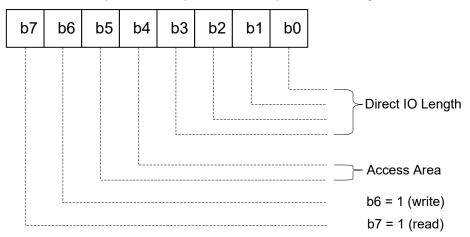
Figure 3-9: Command byte for SPI slaves (host interface)
