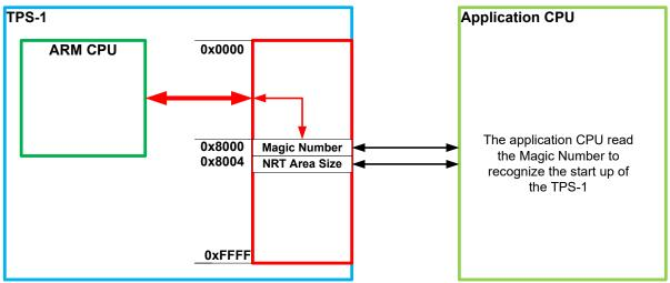
Figure 3-1: TPS-1 with address page 16 Kbyte
