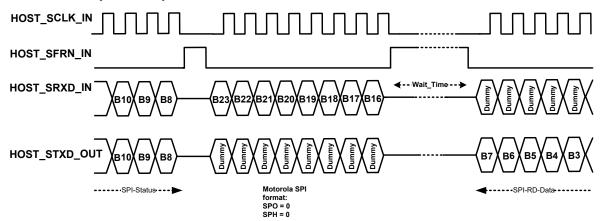
Figure 3-14: SPI Read-Timing Wait Mode
