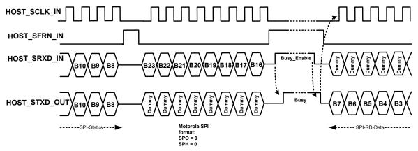
Figure 3-13: SPI Read-Timing (Busy\_POL=1)
