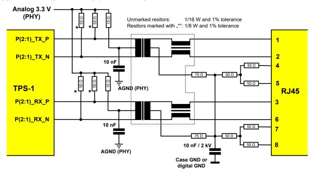
Figure B-6: 100BASE-TX Interface circuit Example
