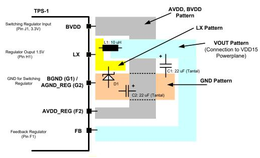
Figure B-3: Switching Regulator layout example
