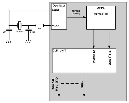
Figure 9-1: Wiring of the TPS-1 clock
