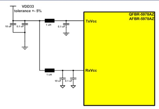
Figure B-10: Power Supply for AVAGO Transceiver
