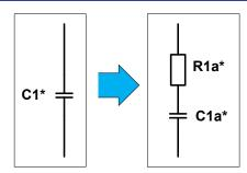
Figure B-2: Change Tantalum to Ceramic Capacitor
