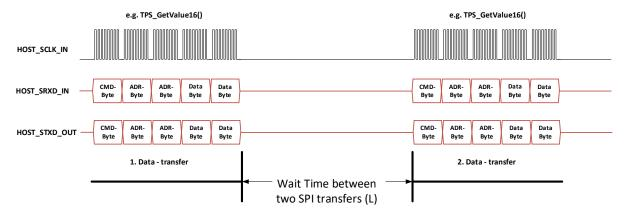
Figure 3-15: Two SPI transfers with wait time
