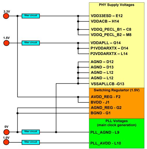
Figure B-5: Voltage Supply Concept
