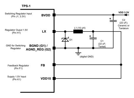
Figure B-1: Wiring of the switching regulator
