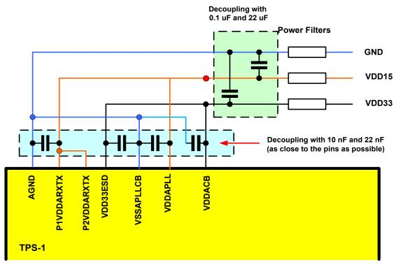
Figure B-4: Decoupling capacitors for supply voltage
