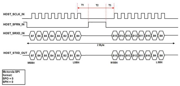
Figure 3-11: SPI Transfer with HOST\_SFRN\_IN Signal
