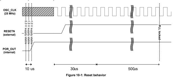
The start-up time of the oscillator depends on the external components (quartz, RLC). As a general rule of thumb, it is roughly in the range of 5 to 20 ms and at higher temperatures in the range of 80 ms.
