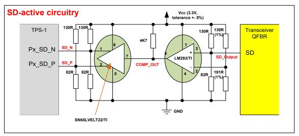
Figure B-9: Circuitry for the SD Signal
