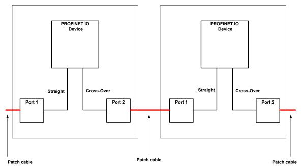
Figure C-1: Line Structure with crossover on board
