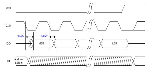
Figure 5-2: Serial Flash output timing requirement
