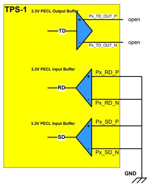
Figure B-11: Unused pins at 100Base-FX interface
