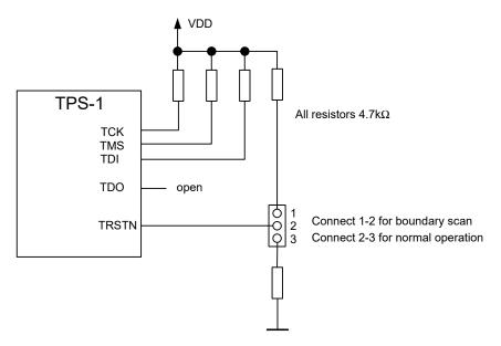
Figure 11-2: JTAG useable for boundary scan
