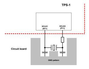
Figure 9-2: Ground pattern for crystal unit
