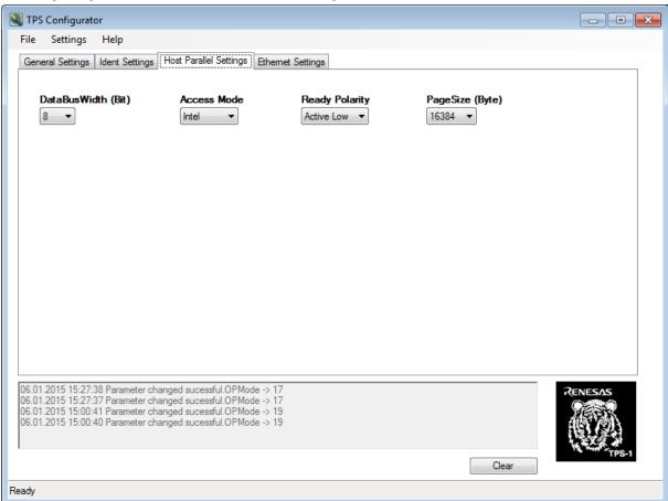
Figure A-2: Parallel host interface configuration
