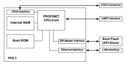
Figure 5-1: TPS-1 structure for the boot process
