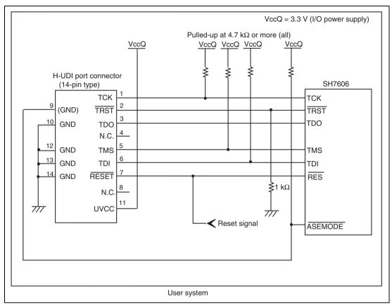
Figure 1.2 Recommended Circuit for Connection between the H-UDI Port Connector and MPU when the Emulator is in Use
