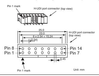
Figure 1.1 Pin Assignments of the H-UDI Port Connector (14 Pins)
