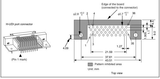
Figure 1.2 Pin Assignments of the H-UDI Port Connector (36 Pins)
