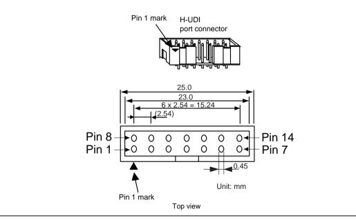
Figure 1.3 Pin Assignments of the H-UDI Port Connector (14 Pins)
