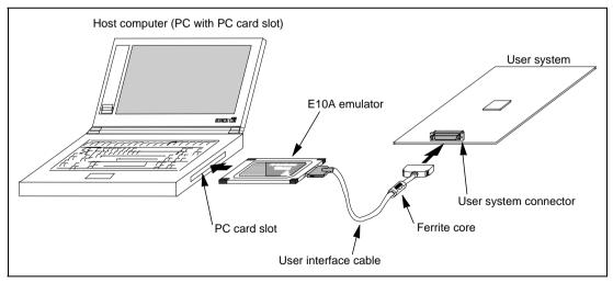
Figure 1.1 Connecting Ferrite Core
