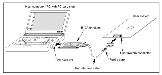
Figure 1.1 Connecting Ferrite Core
