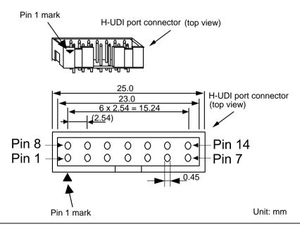
Figure 1.3 Pin Arrangement of the H-UDI Port Connector (14 Pins)
