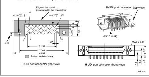
Figure 1.2 Pin Arrangement of the H-UDI Port Connector (36 Pins)
