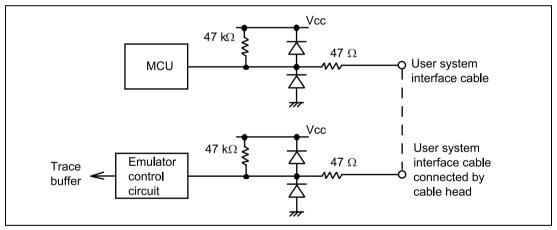
Figure 3.10 IRQ0-IRQ7 User System Interface Circuit
