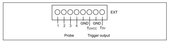
Figure 3.12 External Probe Connector
