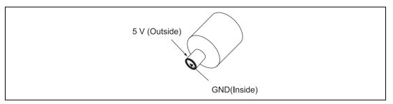
Figure 3.5 Polarity of Power Supply Plug
