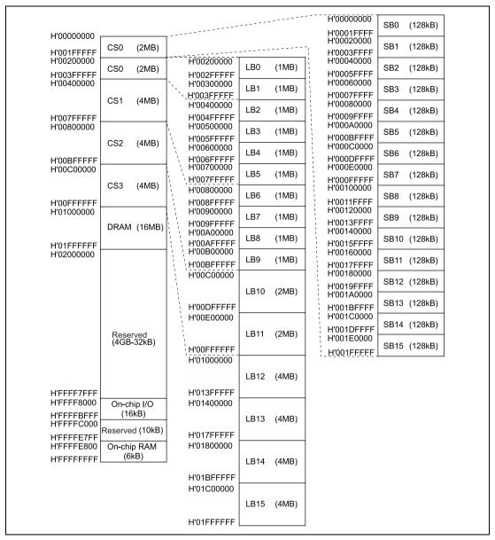
Figure 4.5 Memory Block in Extended Mode without ROM
