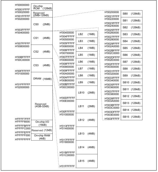
Figure 4.6 Memory Block in Extended Mode with ROM
