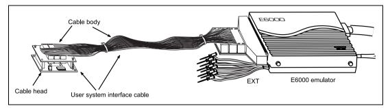
Figure 3.4 Plugging User System Interface Cable Body to E6000 Emulator
