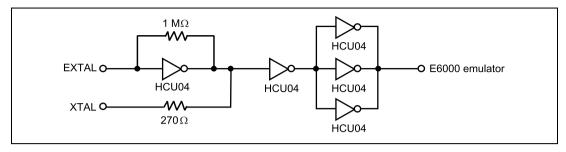
Figure 3.11 Oscillator Circuit
