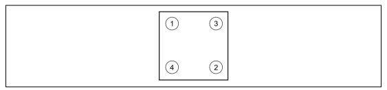
Figure 3.3 Sequence of Screw Tightening
