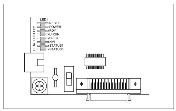
Figure 4.4 LED Location and Indication on the Board
