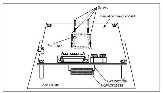
Figure 5.6 Disconnecting Emulation Memory Board
