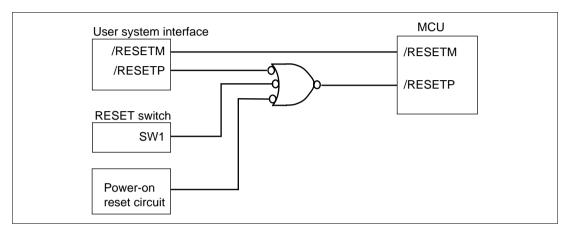
Figure 4.3 Reset Circuit Logic Diagram
