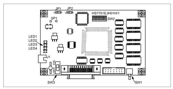
Figure 4.1 Switches, Socket, and LEDs
