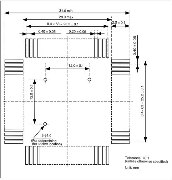
Figure 5.7 Recommended Dimensions for Mount Pad
