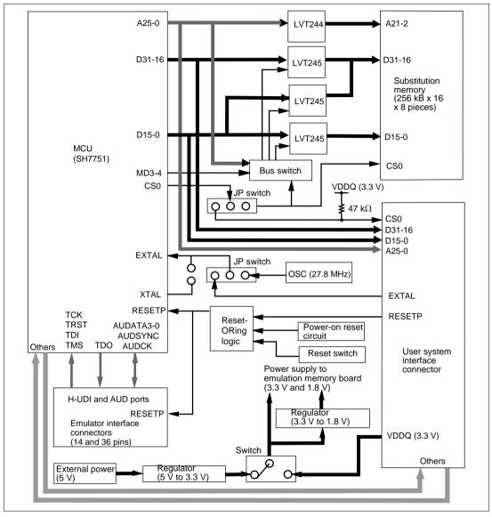
Figure 8.1 Emulation Memory Board Block Diagram
