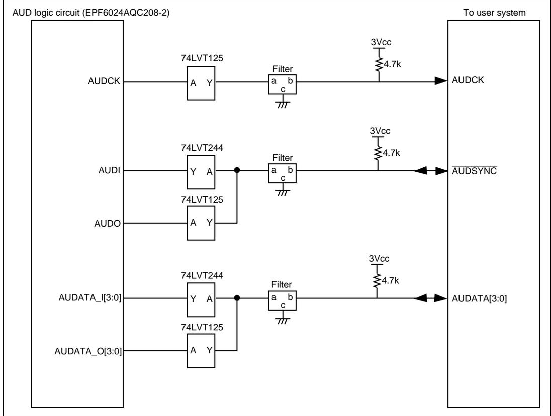
**Figure 6.9** User System Interface Circuit of the AUD Pin (HS7729KCI02H)
