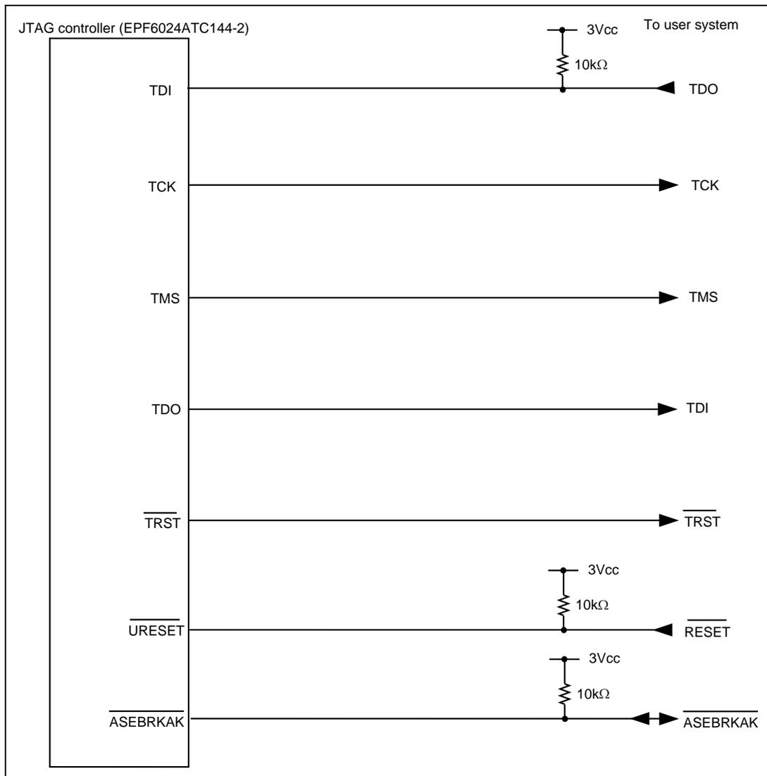
**Figure 6.5 User System Interface Circuit of the Hitachi-UDI Pin (HS7729KCM02H)
