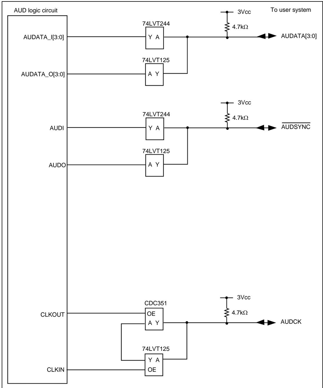
**Figure 6.11 User System Interface Circuit of the AUD Pin (HS7729KCI02H)
