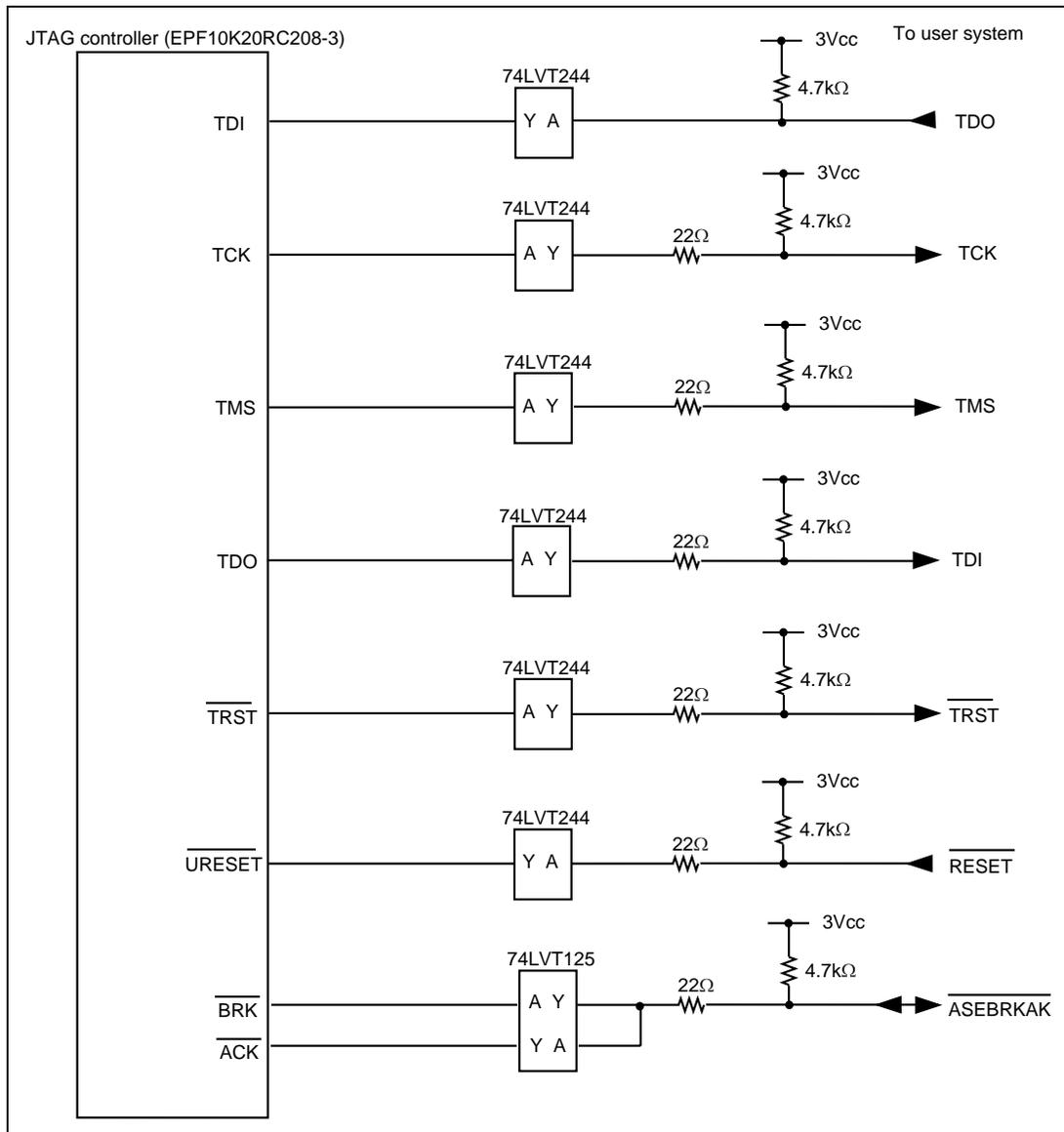
**Figure 6.7 User System Interface Circuit (HS7729KCI01H)**
