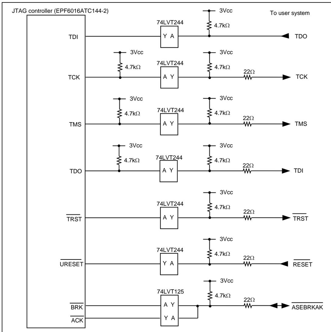
**Figure 6.4 User System Interface Circuit (HS7729KCM01H)**
