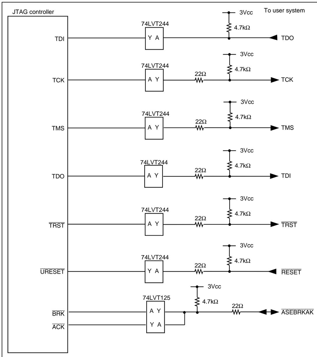
**Figure 6.10 User System Interface Circuit of the Hitachi-UDI Pin (HS7729KCI02H)
