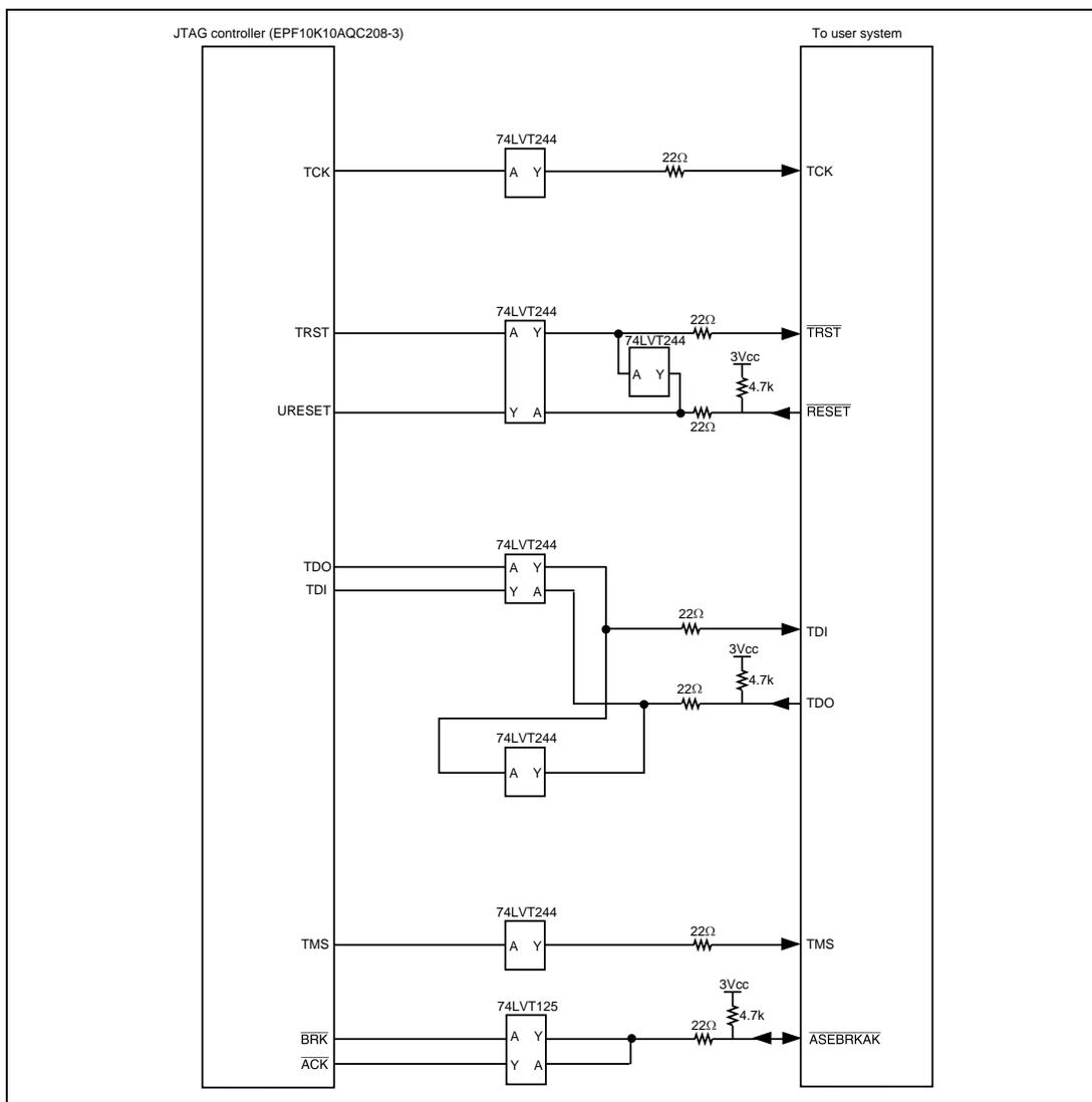
**Figure 6.8 User System Interface Circuit of the Hitachi-UDI Pin (HS7729KCI02H)
