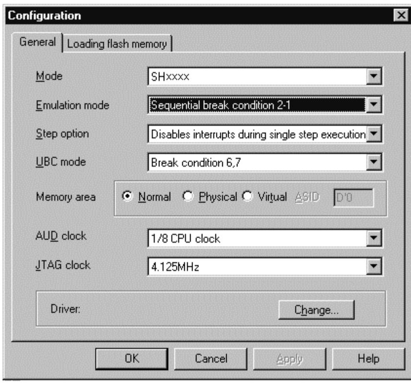
**Figure 3.50 [Configuration] Dialog Box (Sequential Break Setting)**
