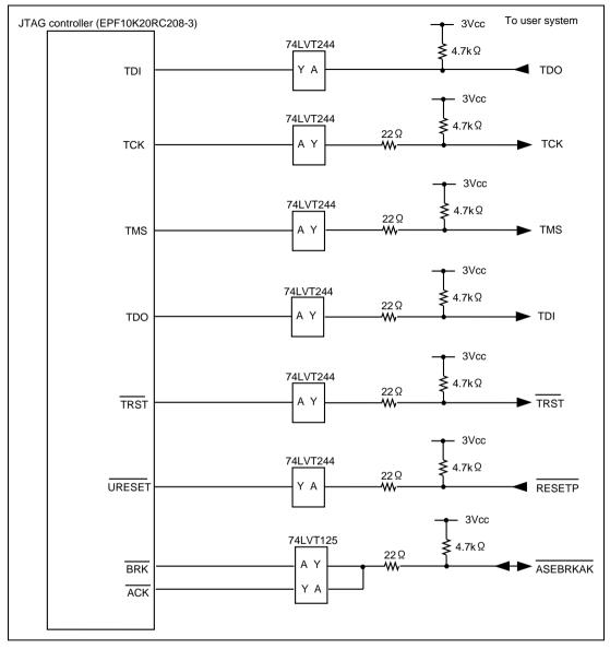
Figure 6.7 User System Interface Circuit (HS7727KCI01H) (Model Name: HS0005KCI03H)
