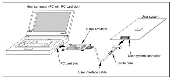
Figure 6.1 Connecting Ferrite Core
