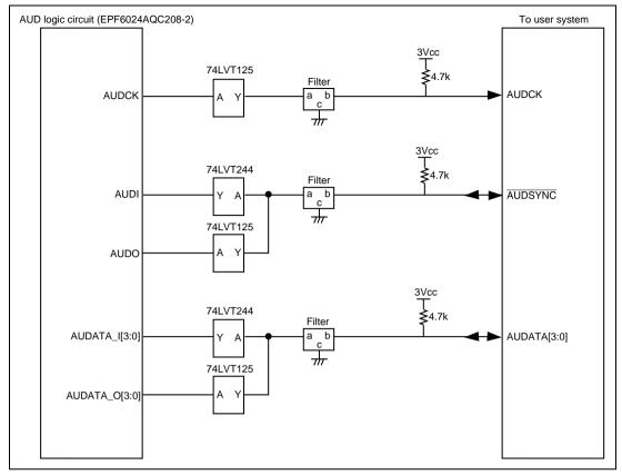
Figure 6.9 User System Interface Circuit of the AUD Pin (HS7727KCI02H) (Model Name: HS0005KCI04H)
