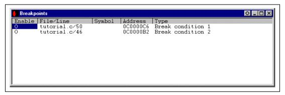
Figure 3.51 [Breakpoints] Window (After Sequential Break Condition Setting)
