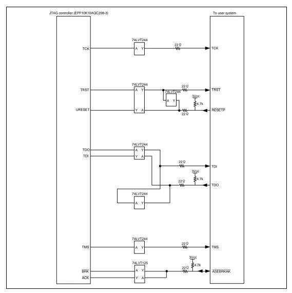
Figure 6.8 User System Interface Circuit of the Hitachi-UDI Pin (HS7727KCI02H) (Model Name: HS0005KCI04H)
