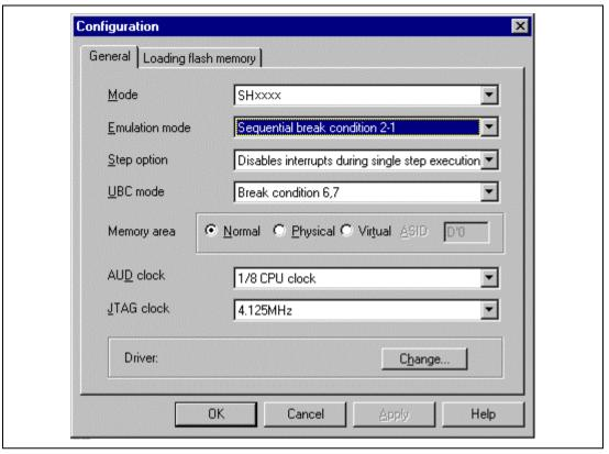
Figure 3.50 [Configuration] Dialog Box (Sequential Break Setting)
