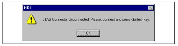
Figure 2.11 [JTAG Connector Disconnected] Dialog Box
