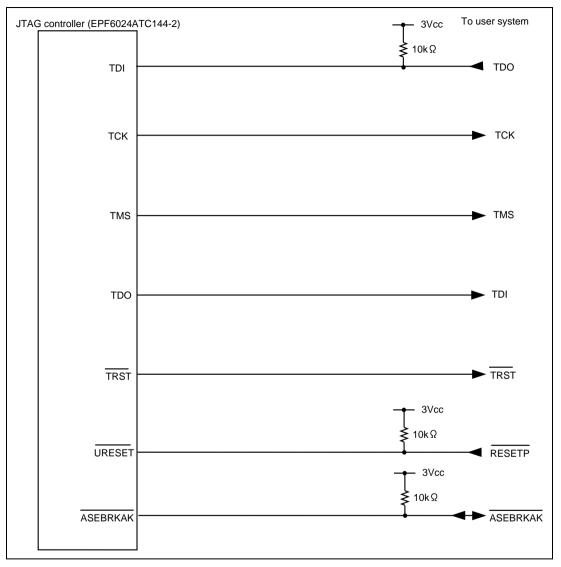
Figure 6.5 User System Interface Circuit of the Hitachi-UDI Pin (HS7727KCM02H) (Model Name: HS0005KCM02H)
