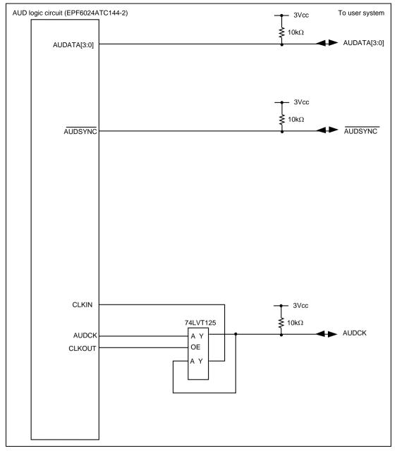
Figure 6.6 User System Interface Circuit of the AUD Pin (HS7727KCM02H) (Model Name: HS0005KCM02H)
