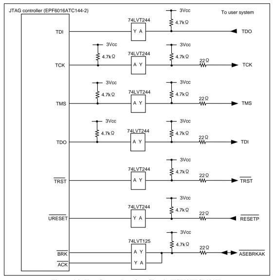
Figure 6.4 User System Interface Circuit (HS7727KCM01H) (Model Name: HS0005KCM03H)
