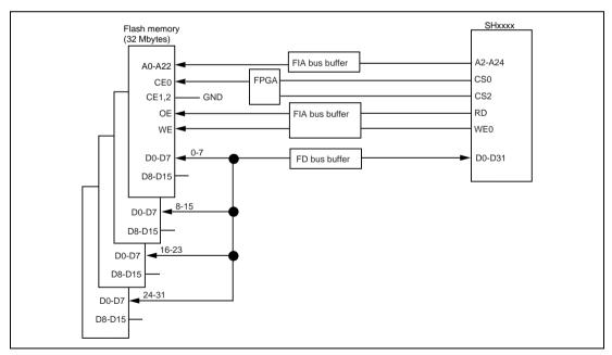
Figure 3.69 Flash Memory Wiring
