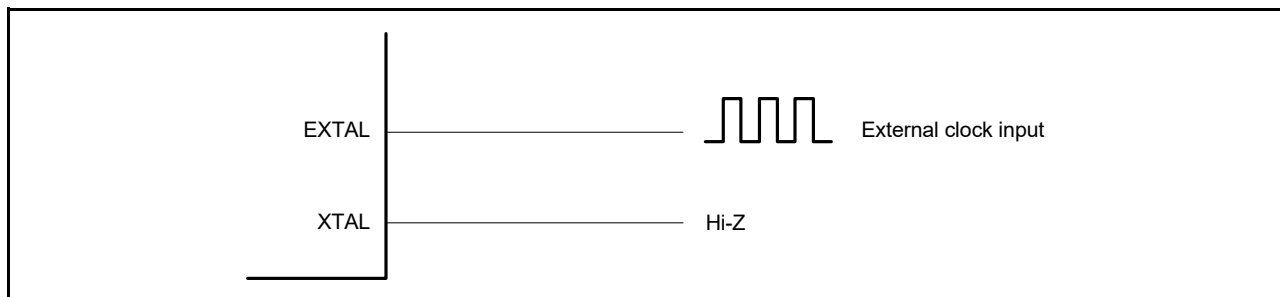
Figure 8.3 Equivalent circuit for external clock
