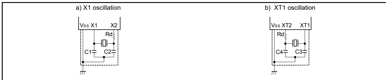
Figure 6 - 23 Examples of External Circuits
