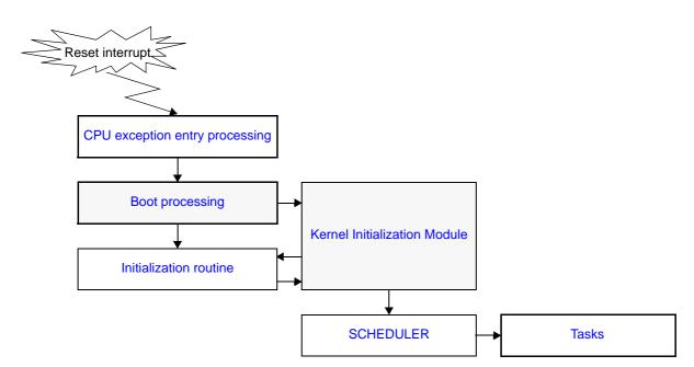
Figure 15-1 Processing Flow (System Initialization)
