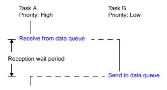
Note Data units of 4 bytes are transmitted or received at a time.
