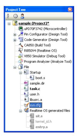
Note 2 When replacing the system configuration file, first remove the added system configuration file from the project, then add another one again.
