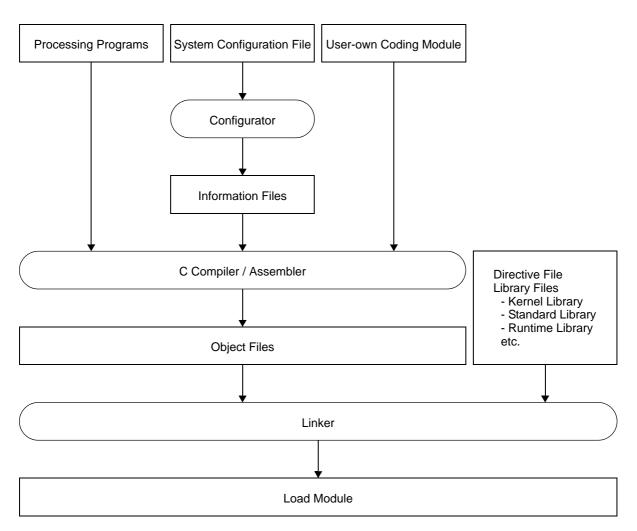
Figure 2-1 Example of System Construction
