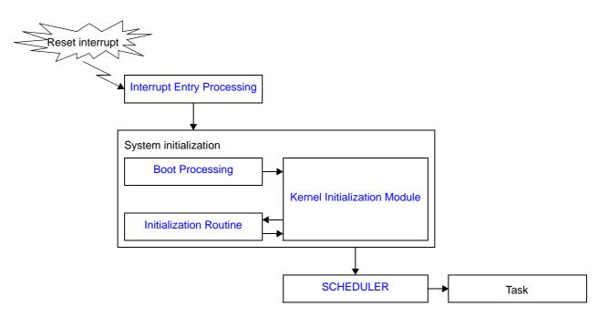
Figure 10-1 Processing Flow (System Initialization)
