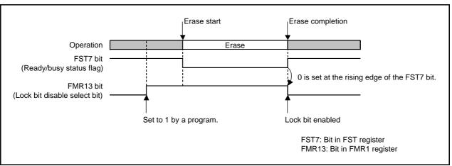
Figure 24.6 FMR13 Bit Operation Timing
