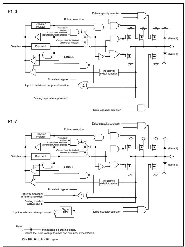
Figure 7.4 Configuration of I/O Ports (4)
