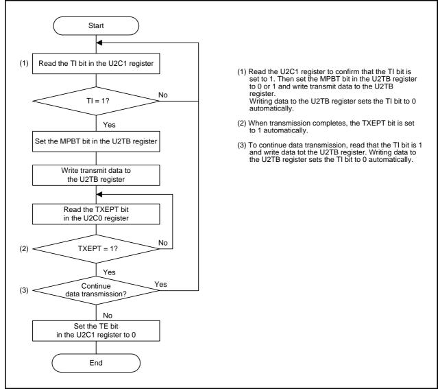
Figure 21.19 Sample Flowchart of Multiprocessor Data Transmission
