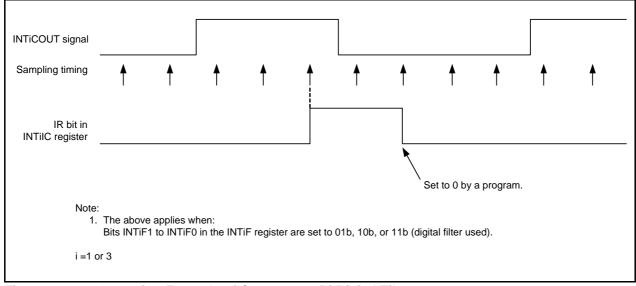
Figure 23.4 Operating Example of Comparator Bi Digital Filter
