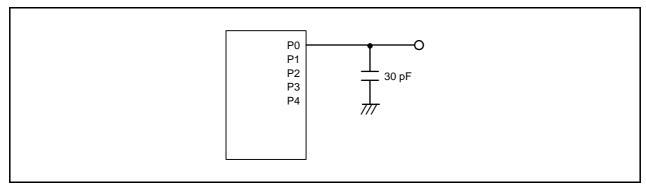
Figure 26.1 Ports P0 to P4 Timing Measurement Circuit
