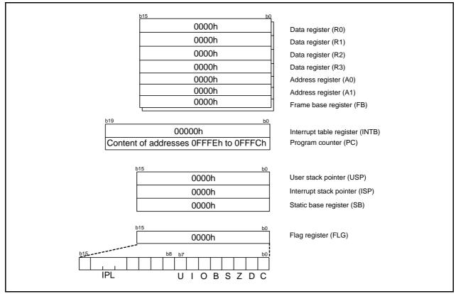
Figure 5.2 CPU Register Status after Reset
