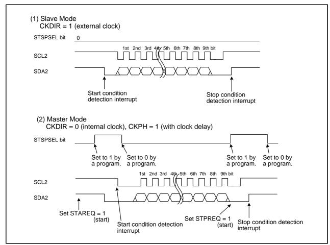
Figure 21.16 STSPSEL Bit Functions
