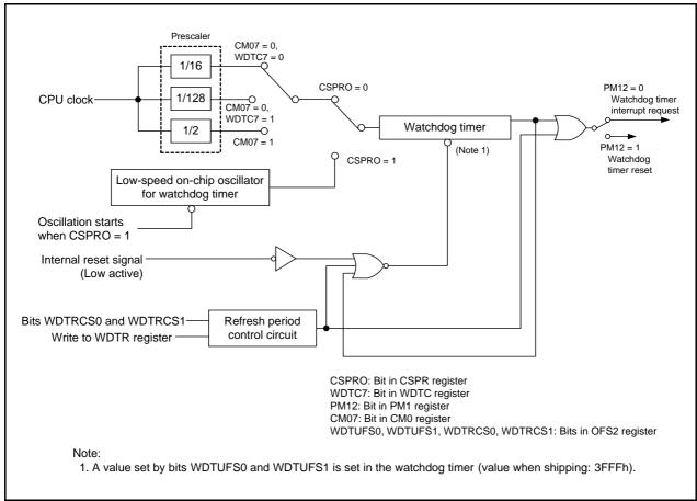
Figure 14.1 Watchdog Timer Block Diagram
