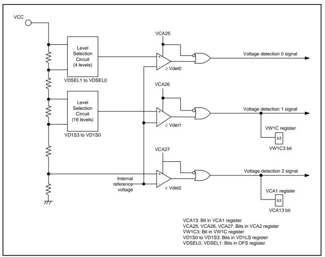
Figure 6.1 Voltage Detection Circuit Block Diagram
