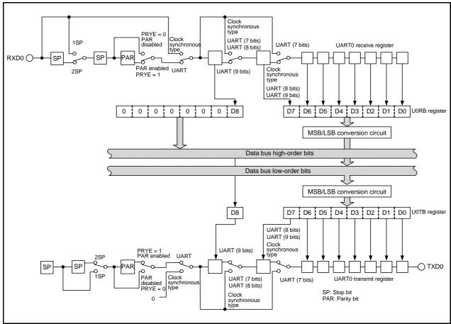
Figure 20.2 Block Diagram of UART0 Transmit/Receive Unit
