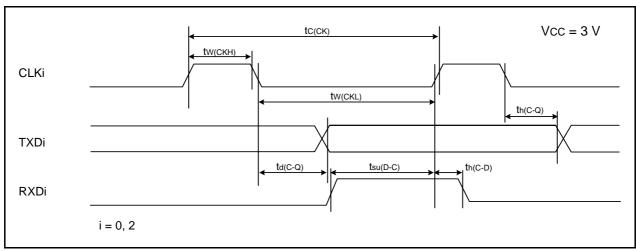
Figure 26.10 Serial Interface Timing Diagram when Vcc = 3 V
