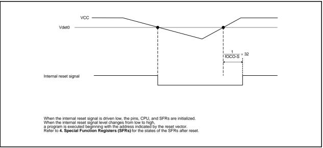
Figure 6.5 Operating Example of Voltage Monitor 0 Reset
