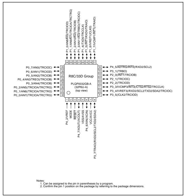
Figure 1.3 Pin Assignment (Top View)
