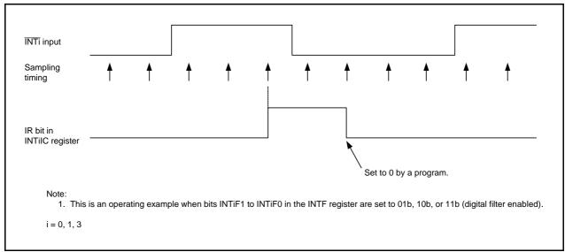
Figure 11.10 Operating Example of INTi Input Filter
