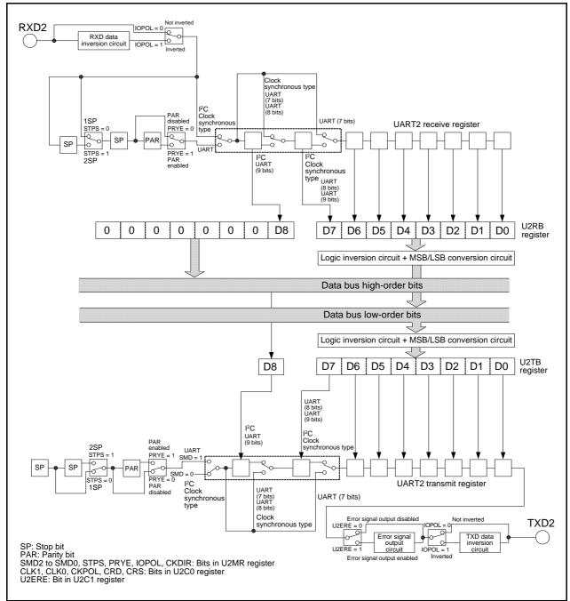
Figure 21.2 Block Diagram of UART2 Transmit/Receive Unit
