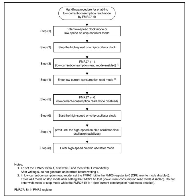
Figure 25.3 Handling Procedure Example of Low-Current-Consumption Read Mode
