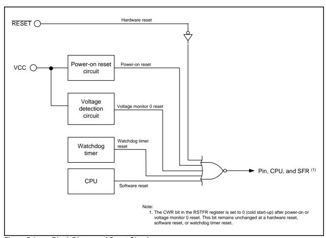
Figure 5.1 Block Diagram of Reset Circuit
