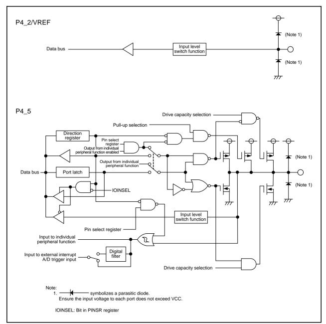
Figure 7.9 Configuration of I/O Ports (9)
