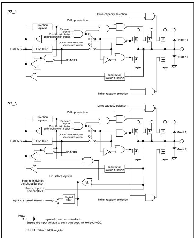
Figure 7.6 Configuration of I/O Ports (6)
