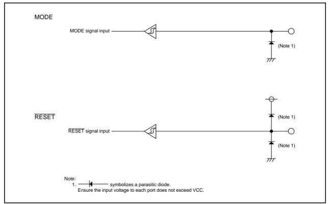
Figure 7.11 Configuration of I/O Pins
