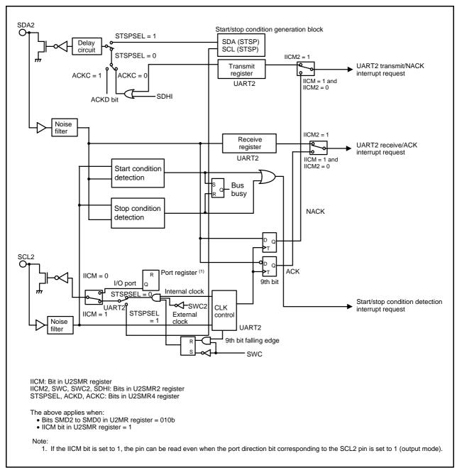
Figure 21.13 I<sup>2</sup>C Mode Block Diagram
