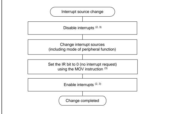
IR bit: The interrupt control register bit for the interrupt whose source is to be changed
