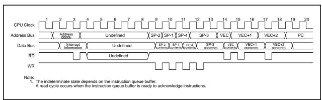
Figure 11.3 Time Required for Executing Interrupt Sequence
