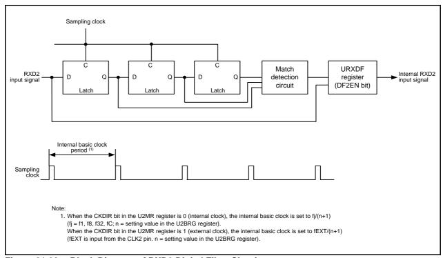
Figure 21.22 Block Diagram of RXD2 Digital Filter Circuit
