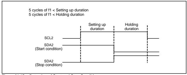
Figure 21.15 Detection of Start and Stop Conditions
