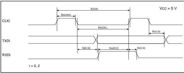
Figure 26.6 Serial Interface Timing Diagram when Vcc = 5 V
