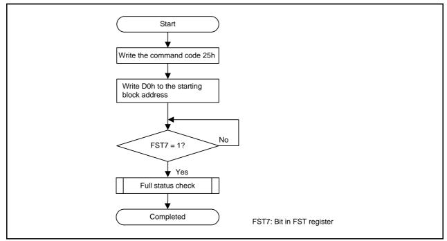
Figure 24.14 Block Blank Check Flowchart
