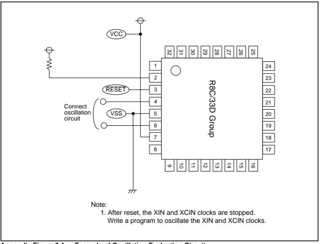
Appendix Figure 3.1 Example of Oscillation Evaluation Circuit
