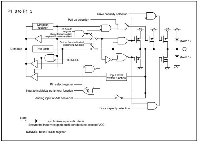
Figure 7.2 Configuration of I/O Ports (2)
