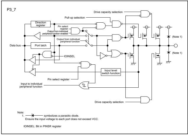
Figure 7.8 Configuration of I/O Ports (8)
