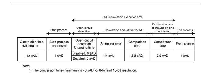
Figure 22.3 A/D Conversion Cycles ( $\phi$ AD = fAD)
