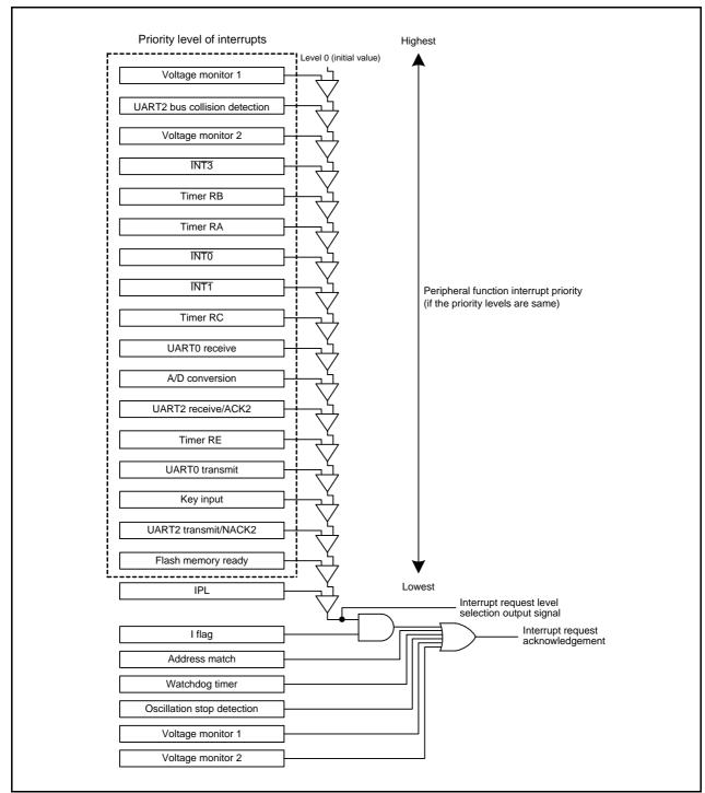
Figure 11.8 Interrupt Priority Level Selection Circuit
