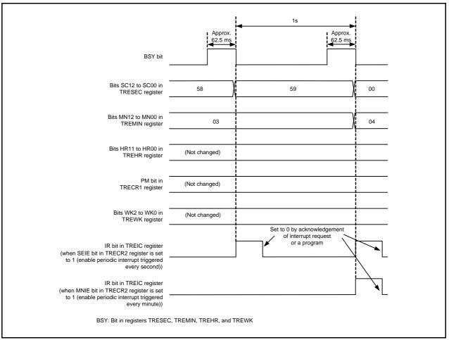
Figure 19.3 Operating Example in Real-Time Clock Mode
