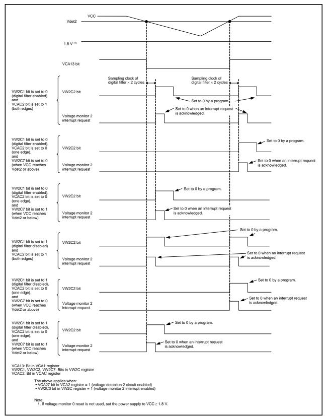
Figure 6.7 Operating Example of Voltage Monitor 2 Interrupt
