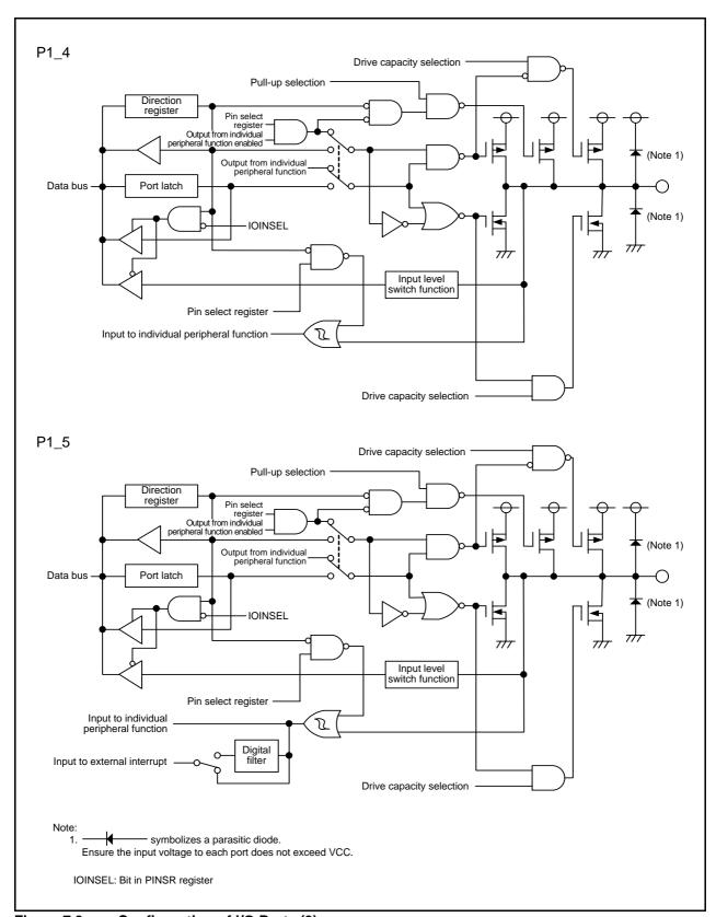
Figure 7.3 Configuration of I/O Ports (3)
