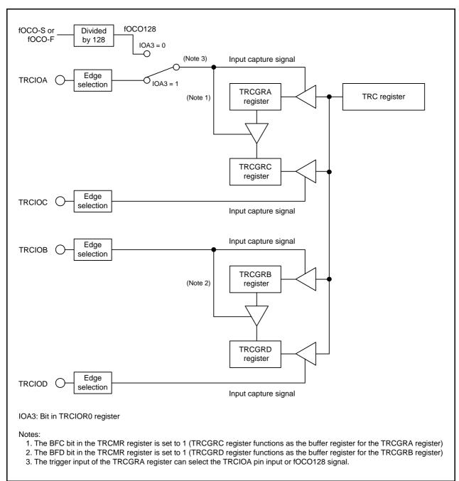
Figure 18.7 **Block Diagram of Input Capture Function**
