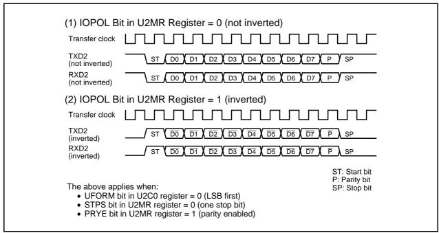
Figure 21.11 TXD and RXD I/O Inversion
