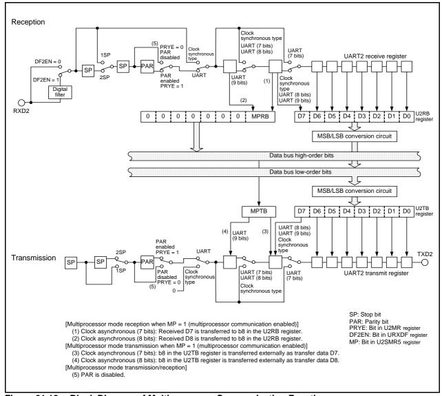
Figure 21.18 Block Diagram of Multiprocessor Communication Function
