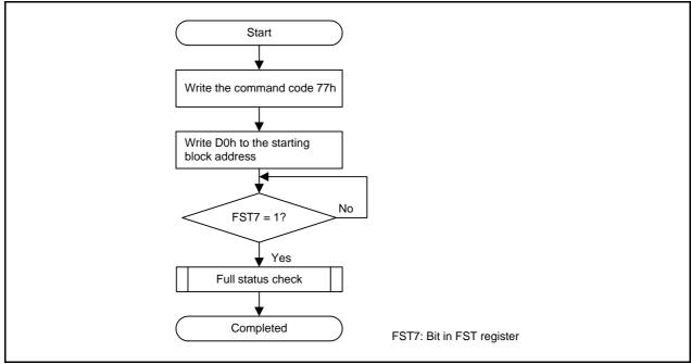
Figure 24.12 Lock Bit Program Flowchart
