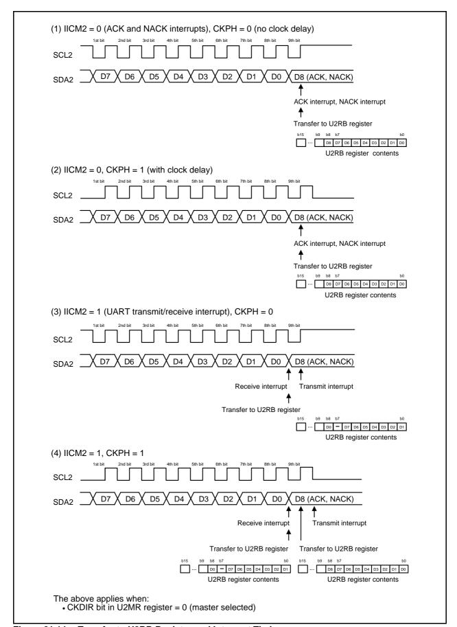
Figure 21.14 Transfer to U2RB Register and Interrupt Timing
