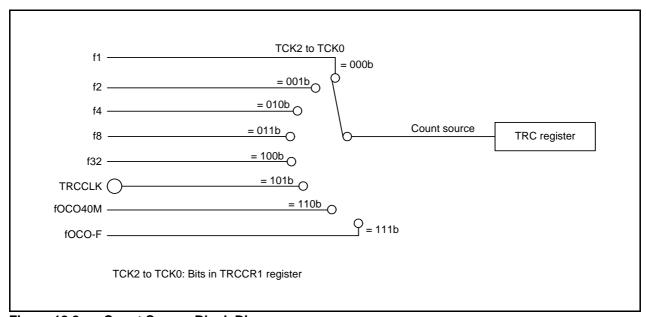
Figure 18.2 Count Source Block Diagram
