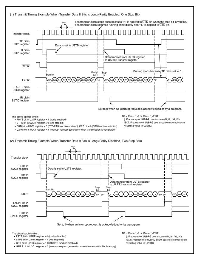
Figure 21.7 Transmit Timing in UART Mode
