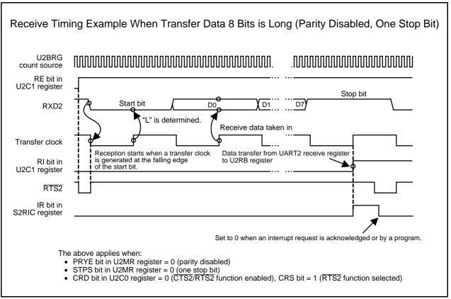
Figure 21.8 Receive Timing in UART Mode
