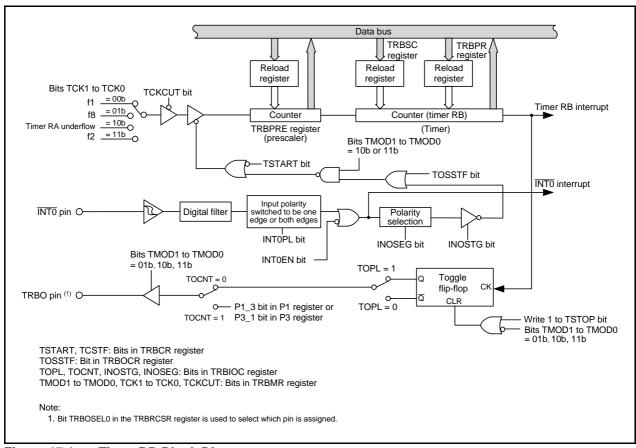
Figure 17.1 Timer RB Block Diagram
