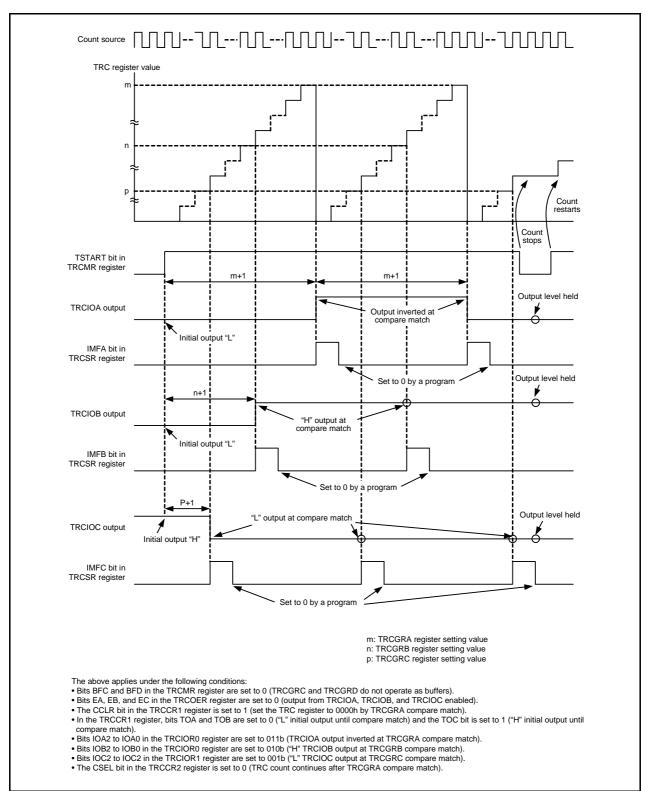
Figure 18.10 Operating Example of Output Compare Function
