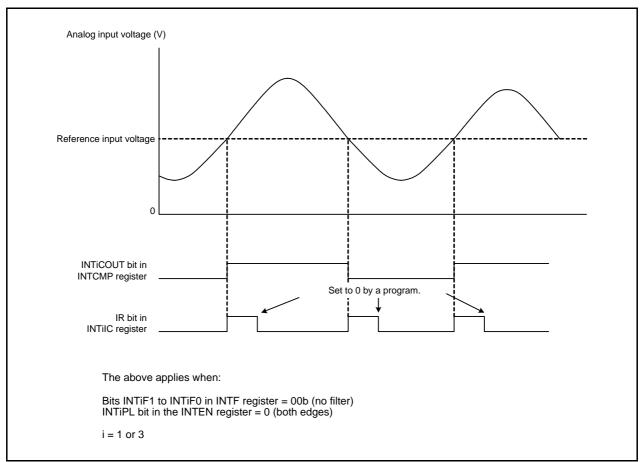
Figure 23.2 Operating Example of Comparator Bi (i = 1 or 3)
