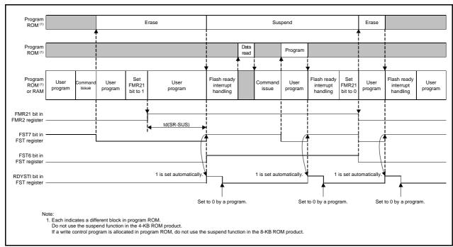
Figure 24.3 Suspend Operation Timing
