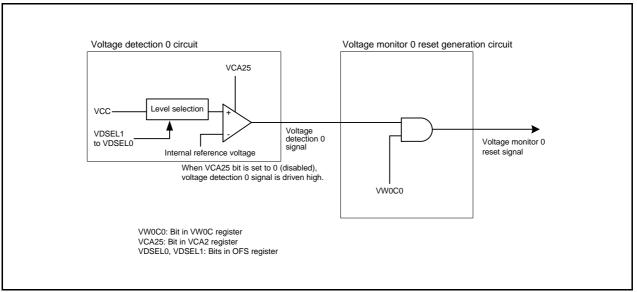
Figure 6.2 Block Diagram of Voltage Monitor 0 Reset Generation Circuit
