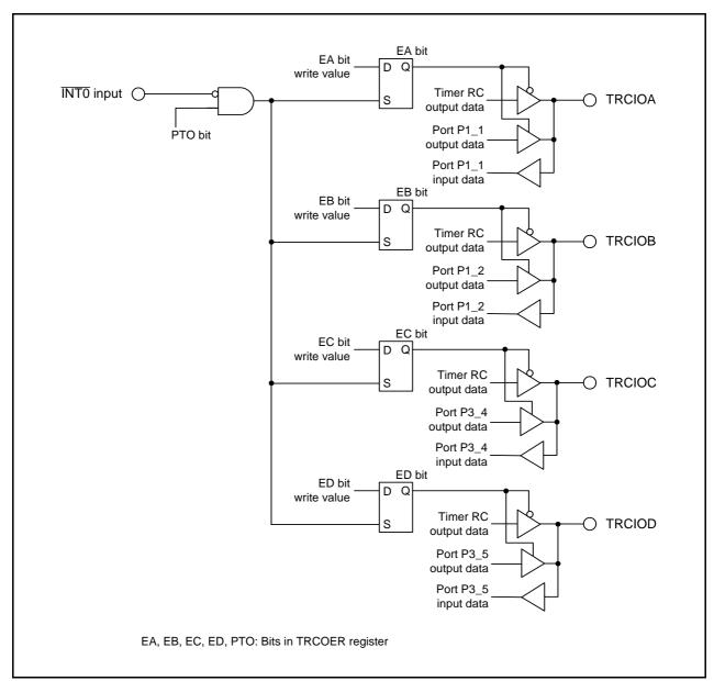
Figure 18.6 Forced Cutoff of Pulse Output
