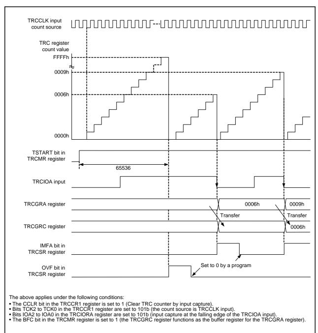
Figure 18.8 Operating Example of Input Capture Function
