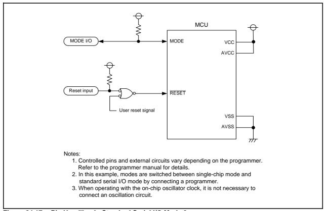
Figure 24.17 Pin Handling in Standard Serial I/O Mode 3
