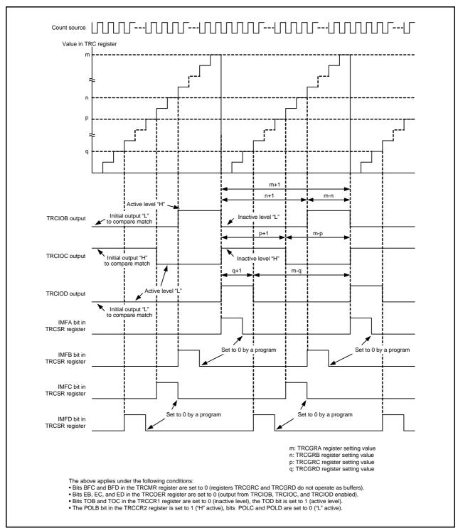
Figure 18.14 Operating Example of PWM Mode
