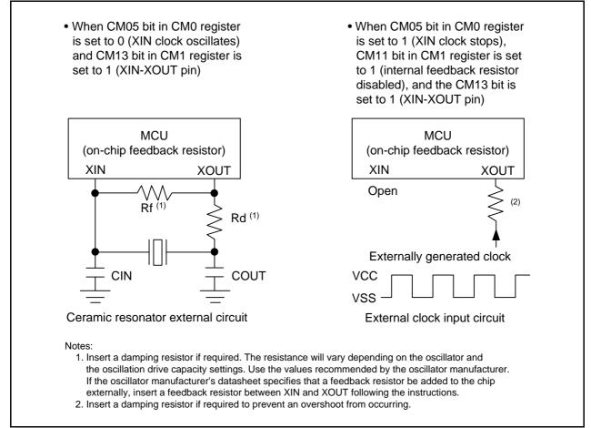
Figure 9.4 Examples of XIN Clock Connection Circuit
