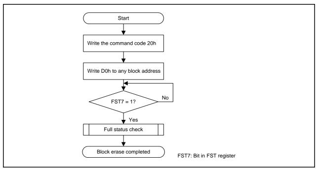
Figure 24.9 Block Erase Flowchart (Flash Ready Status Interrupt Disabled)
