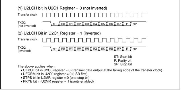
Figure 21.10 Serial Data Logic Switching
