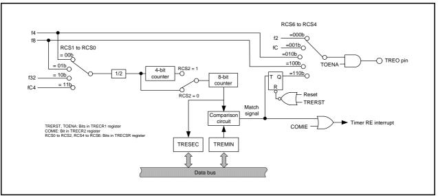
Figure 19.4 Block Diagram of Output Compare Mode
