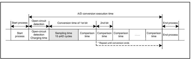
Figure 22.2 Timing Diagram of A/D Conversion
