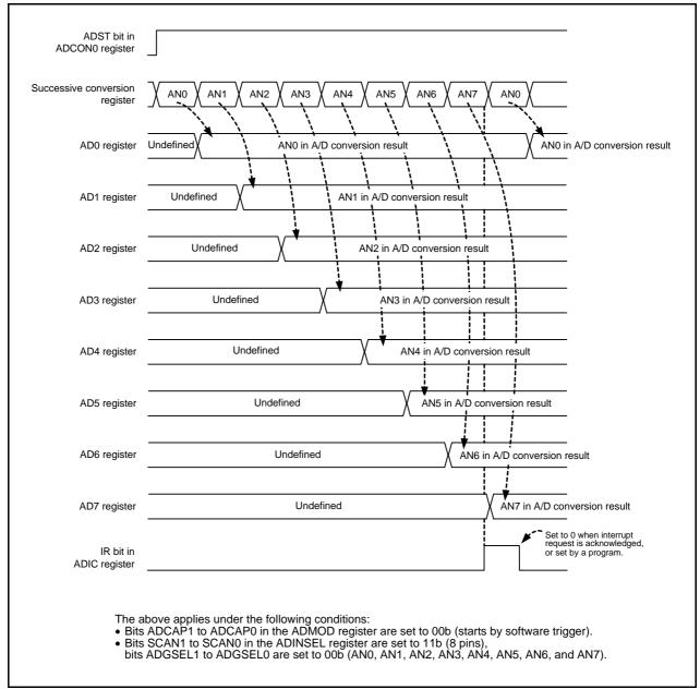
Figure 22.9 Operating Example of Repeat Sweep Mode
