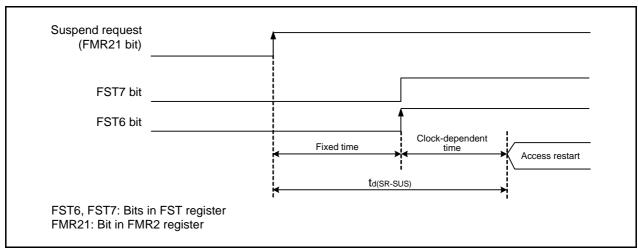
Figure 26.2 Time delay until Suspend
