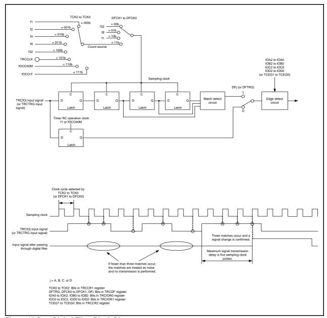
Figure 18.5 Digital Filter Block Diagram
