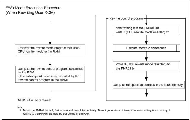
Figure 24.4 How to Set and Exit EW0 Mode
