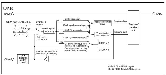
Figure 20.1 UARTO Block Diagram
