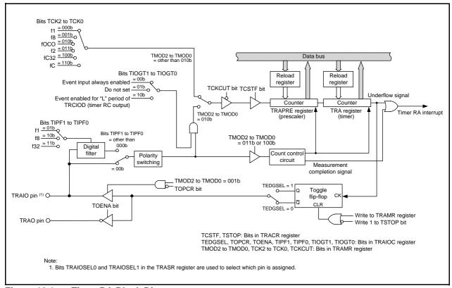
Figure 16.1 Timer RA Block Diagram
