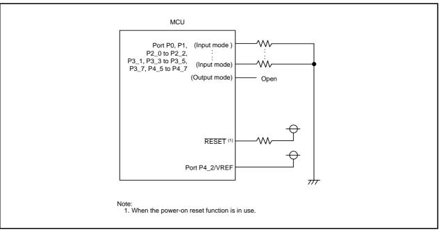
Figure 7.12 Unassigned Pin Handling
