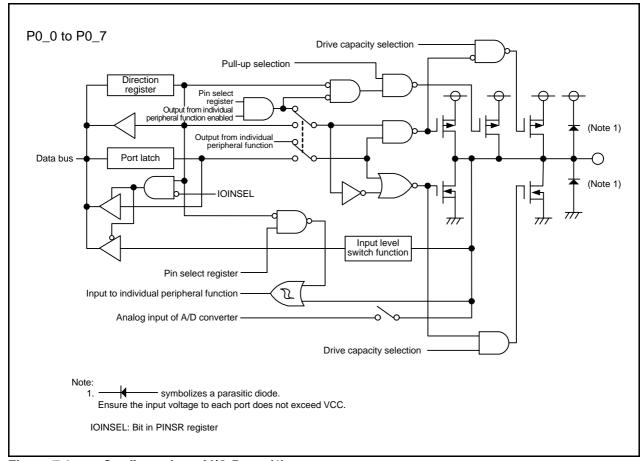
Figure 7.1 Configuration of I/O Ports (1)
