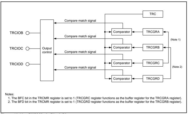
Figure 18.13 PWM Mode Block Diagram
