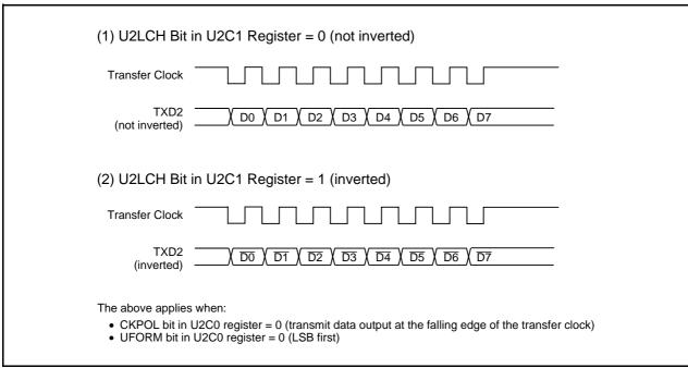
Figure 21.6 Serial Data Logic Switching
