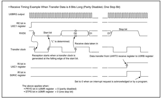
Figure 20.7 Receive Timing in UART Mode
