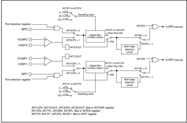
Figure 23.1 Comparator B Block Diagram
