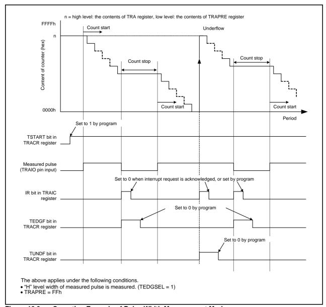
Figure 16.3 Operating Example of Pulse Width Measurement Mode
