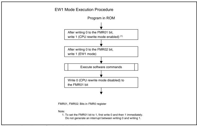
Figure 24.5 How to Set and Exit EW1 Mode
