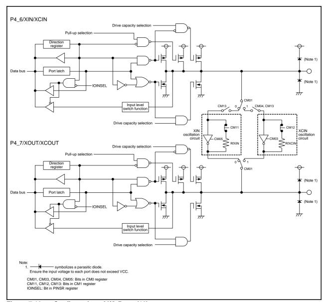
Figure 7.10 Configuration of I/O Ports (10)
