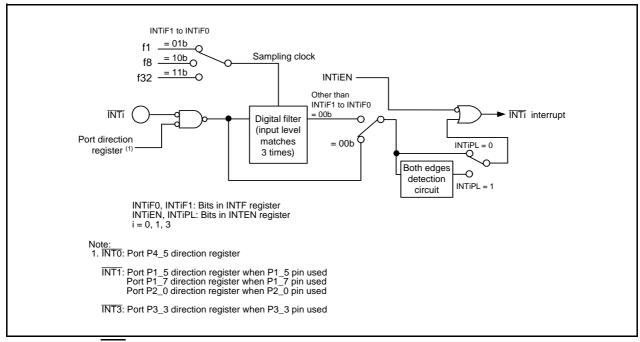
Figure 11.9 INTi Input Filter Configuration
