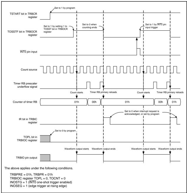
Figure 17.4 Operating Example of Programmable One-Shot Generation Mode
