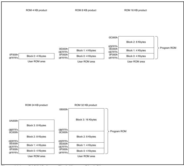
Figure 24.1 R8C/33D Group Flash Memory Block Diagram
