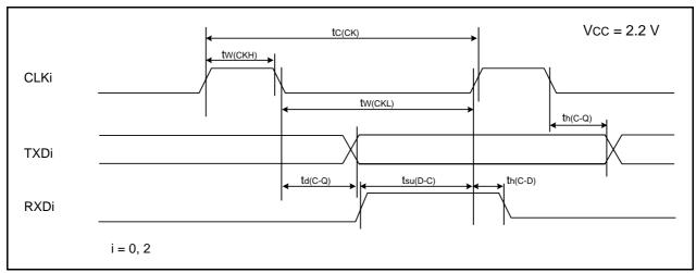
Figure 26.14 Serial Interface Timing Diagram when Vcc = 2.2 V
