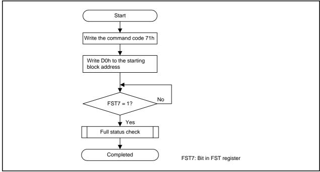
Figure 24.13 Read Lock Bit Status Flowchart
