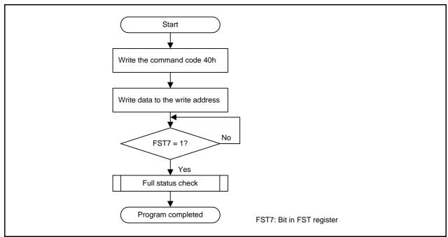
Figure 24.7 Program Flowchart (Flash Ready Status Interrupt Disabled)
