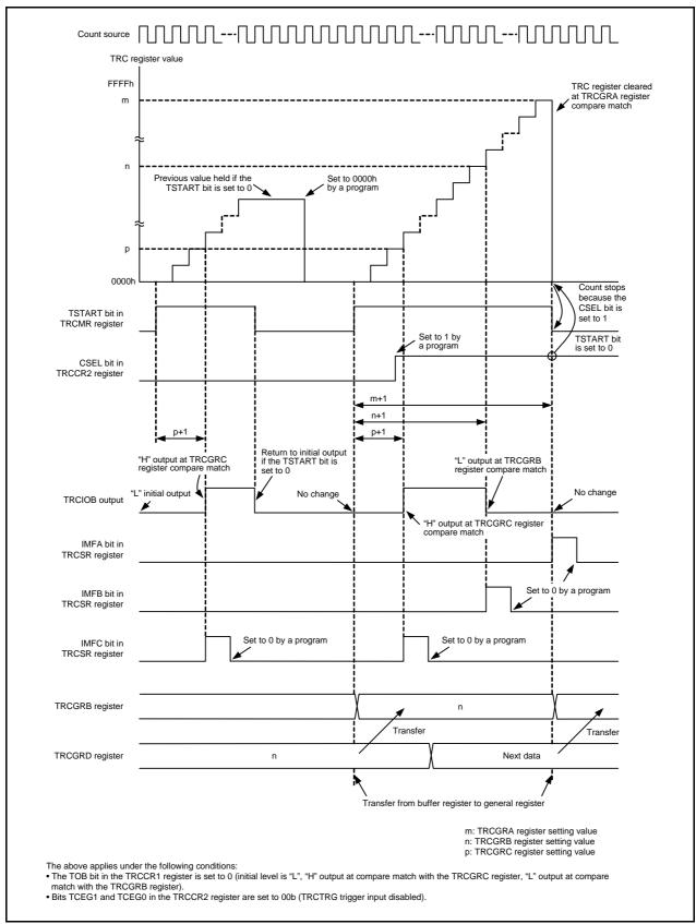
Figure 18.17 Operating Example of PWM2 Mode (TRCTRG Trigger Input Disabled)
