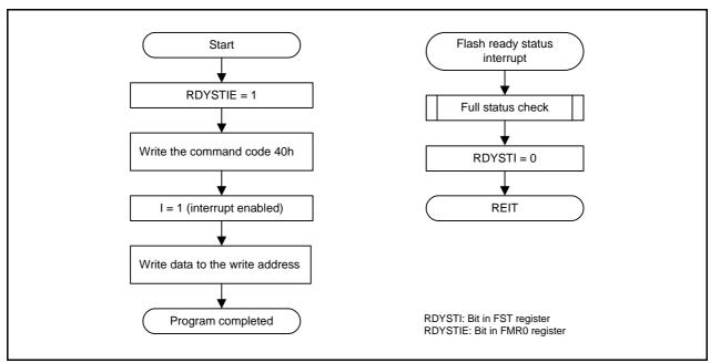
Figure 24.8 Program Flowchart (Flash Ready Status Interrupt Enabled)
