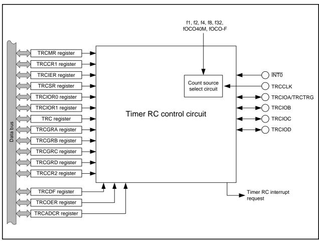
Figure 18.1 Timer RC Block Diagram
