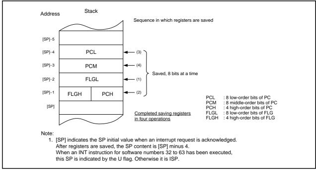
Figure 11.6 Register Saving Operation
