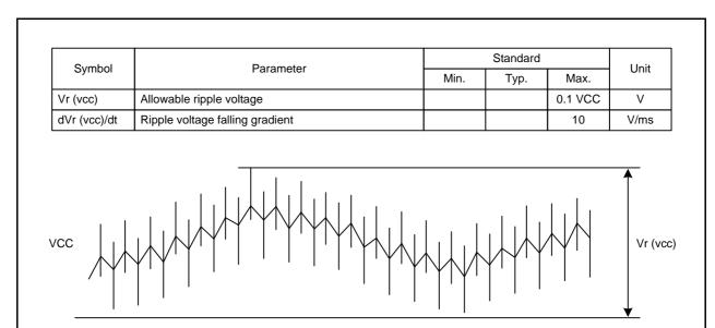
Figure 27.3 Definition of ripple voltage
