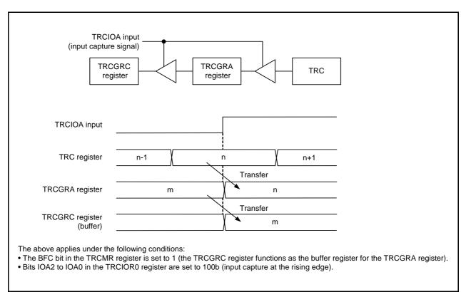
Figure 18.3 Buffer Operation for Input Capture Function
