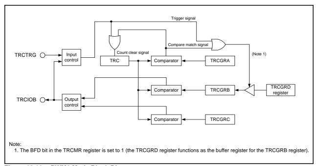
Figure 18.16 PWM2 Mode Block Diagram
