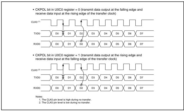
Figure 20.4 Transfer Clock Polarity
