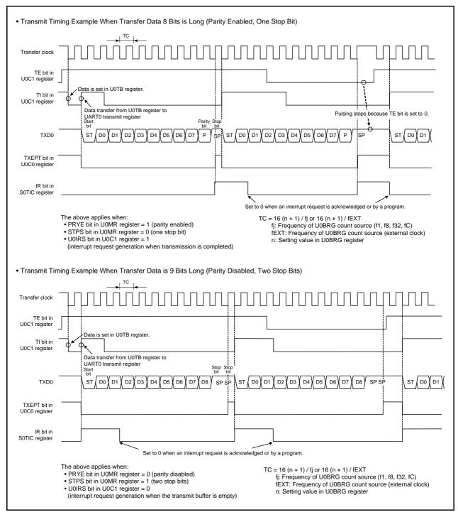
Figure 20.6 Transmit Timing in UART Mode
