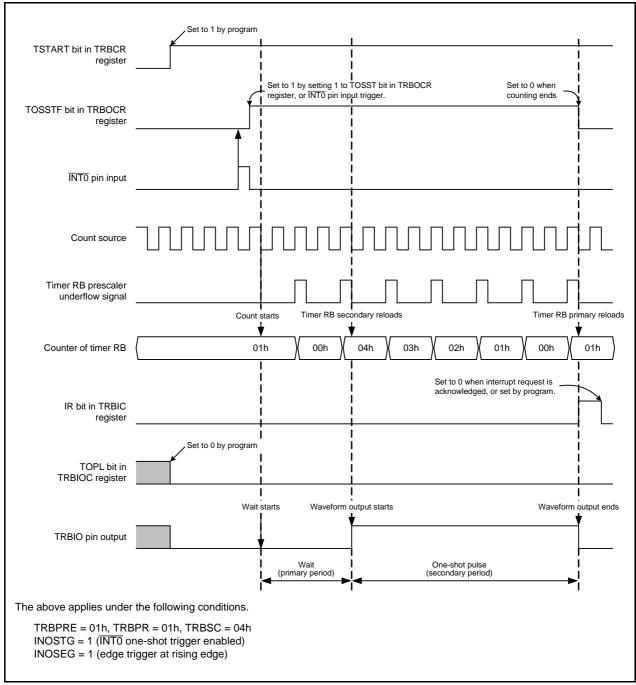
Figure 17.5 Operating Example of Programmable Wait One-Shot Generation Mode
