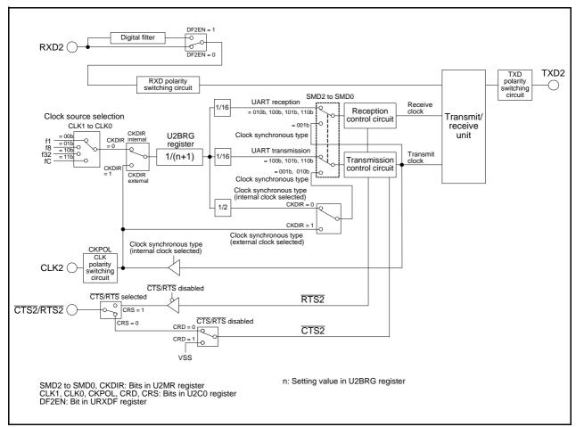
Figure 21.1 UART2 Block Diagram
