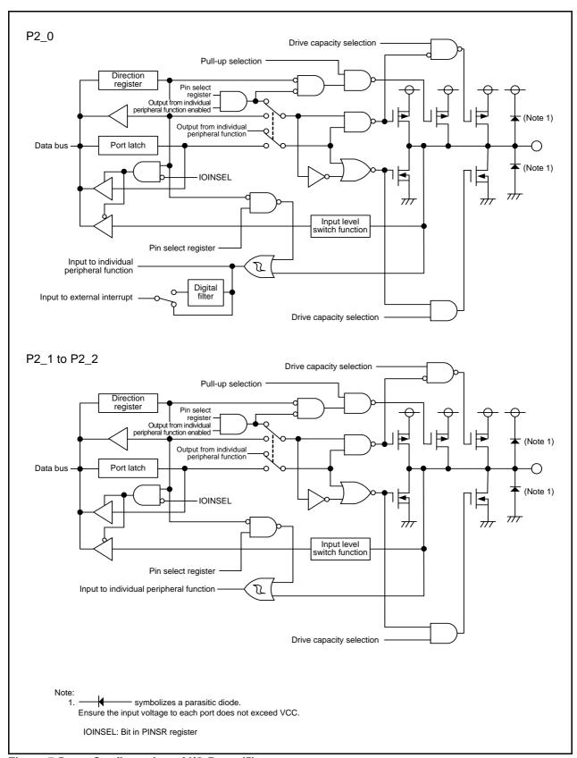
Figure 7.5 Configuration of I/O Ports (5)
