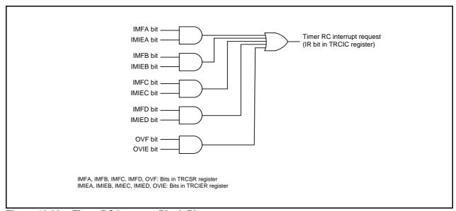
Figure 18.20 Timer RC Interrupt Block Diagram
