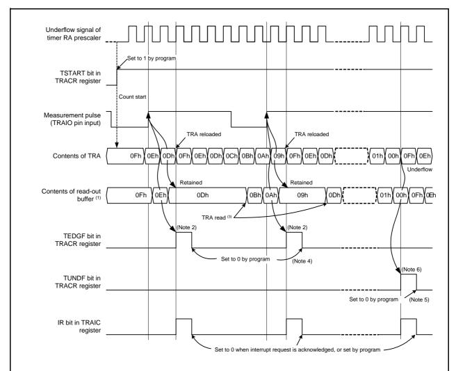
Conditions: The period from one rising edge to the next rising edge of the measured pulse is measured (TEDGSEL = 0) with the default value of the TRA register as 0Fh.
