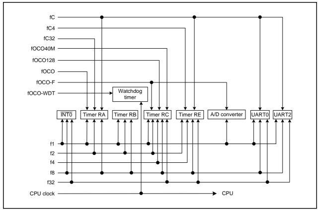
Figure 9.2 Peripheral Function Clock
