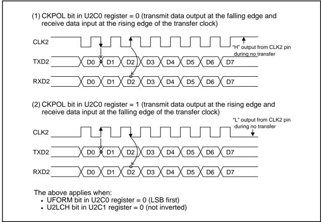
Figure 21.4 Transfer Clock Polarity
