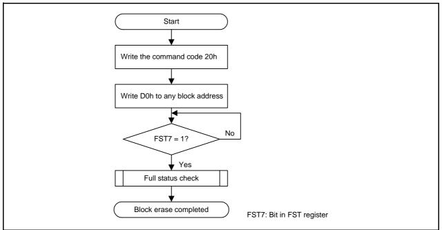
Figure 27.10 Block Erase Flowchart (Flash Ready Status Interrupt Disabled)
