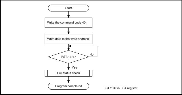
Figure 27.8 Program Flowchart (Flash Ready Status Interrupt Disabled)
