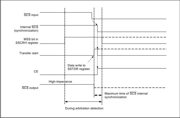
Figure 23.13 Arbitration Check Timing
