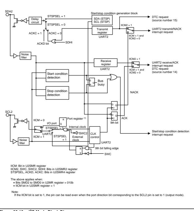
Figure 22.13 I<sup>2</sup>C Mode Block Diagram
