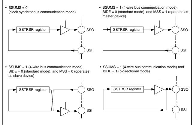
Figure 23.3 Association between Data I/O Pins and SSTRSR Register
