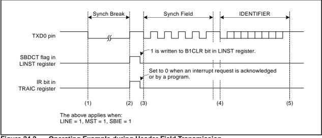
Figure 24.2 Operating Example during Header Field Transmission
