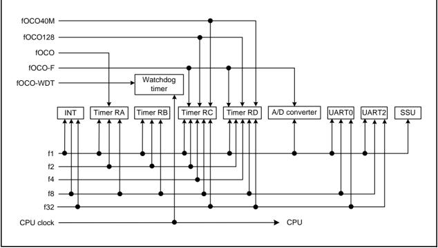
Figure 9.2 Peripheral Function Clock
