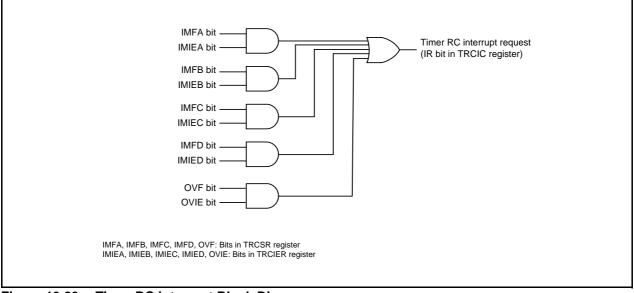
Figure 19.20 Timer RC Interrupt Block Diagram
