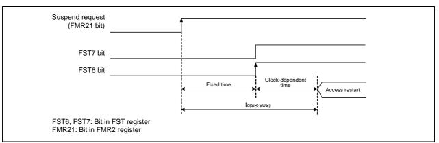
Figure 29.2 Time delay until Suspend
