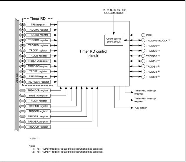
Figure 20.1 Timer RD Block Diagram
