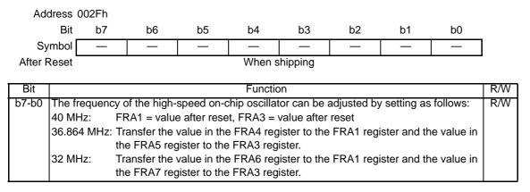
Set the PRC0 bit in the PRCR register to 1 (write enabled) before rewriting the FRA3 register. Also, rewrite the FRA3 register when the FRA00 bit in the FRA0 register is set 0 (high-speed on-chip oscillator off).
