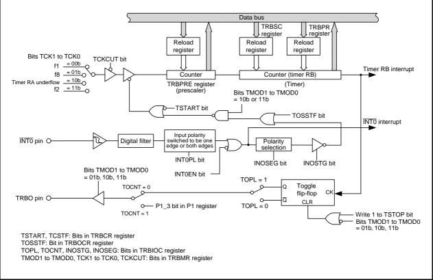
Figure 18.1 Timer RB Block Diagram
