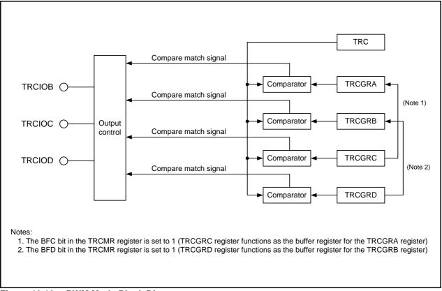
Figure 19.13 PWM Mode Block Diagram
