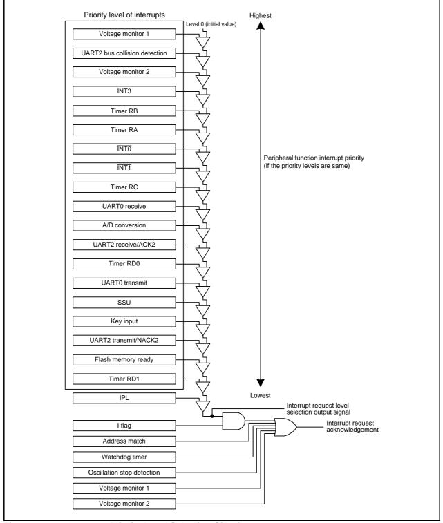
Figure 11.8 Interrupt Priority Level Selection Circuit
