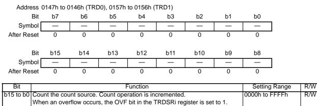
Access the TRDi register in 16-bit units. Do not access it in 8-bit units.
