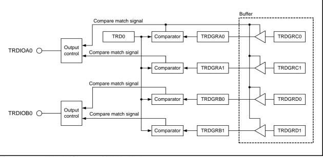
Figure 20.22 Block Diagram of PWM3 Mode
