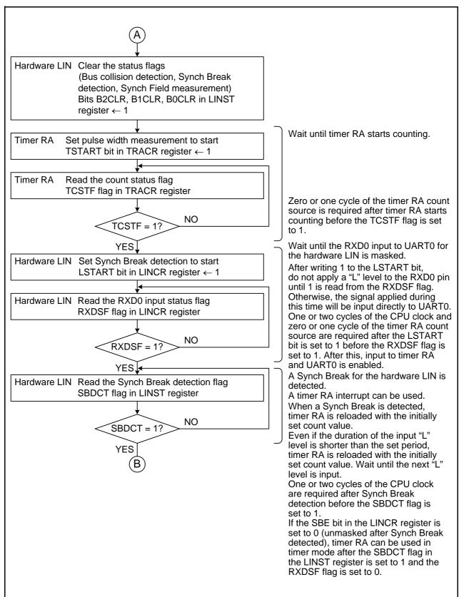
Figure 24.7 Header Field Reception Flowchart Example (2)
