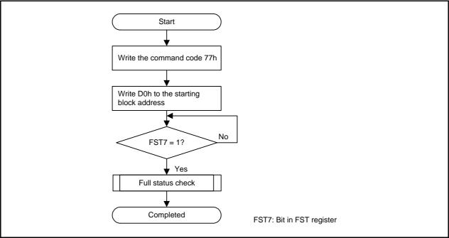
Figure 27.13 Lock Bit Program Flowchart
