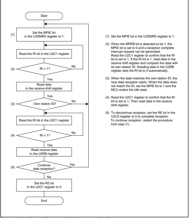
Figure 22.21 Sample Flowchart of Multiprocessor Data Reception
