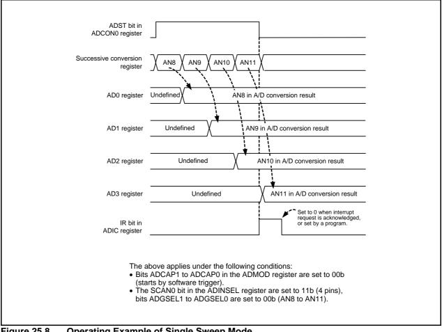
Figure 25.8 **Operating Example of Single Sweep Mode**
