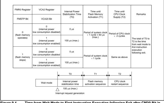
Figure 9.4 Time from Wait Mode to First Instruction Execution following Exit after CM30 Bit in CM3 Register is Set to 1 (MCU Enters Wait Mode)
