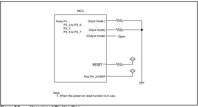
Figure 7.9 Unassigned Pin Handling
