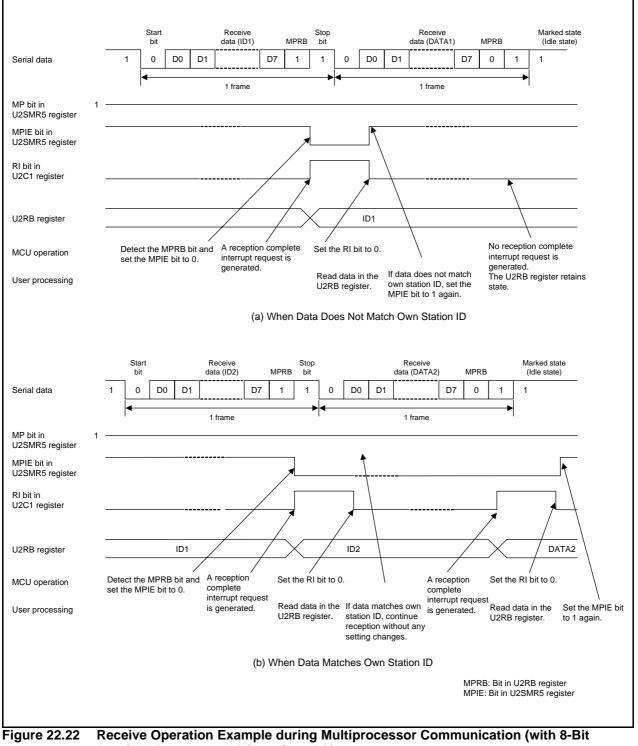
Data/Multiprocessor Bit/One-Stop Bit)
