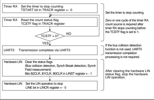
Figure 24.10 Example of Hardware LIN Communication Completion Flowchart
