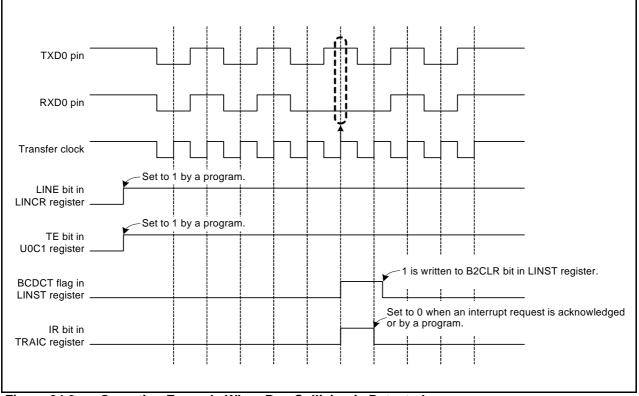
Figure 24.9 Operating Example When Bus Collision is Detected
