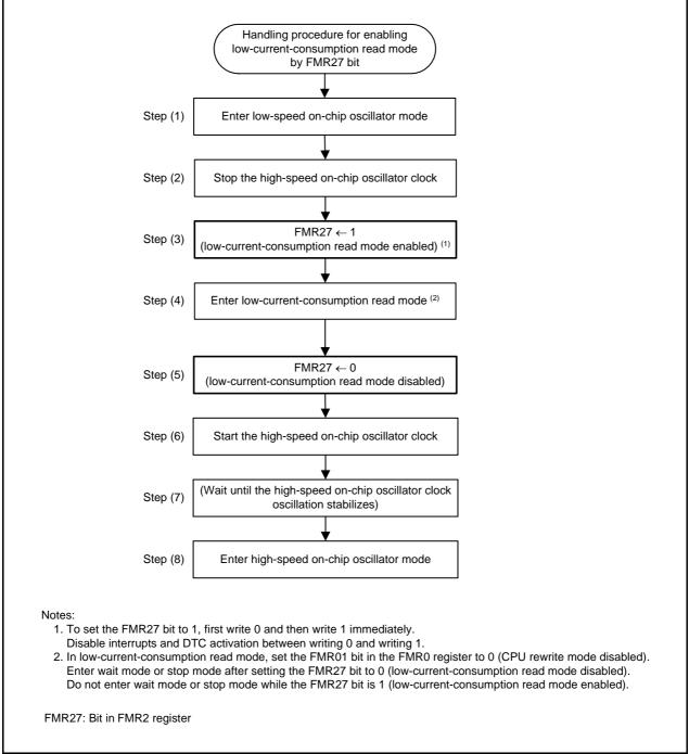
Figure 28.4 Handling Procedure Example of Low-Current-Consumption Read Mode
