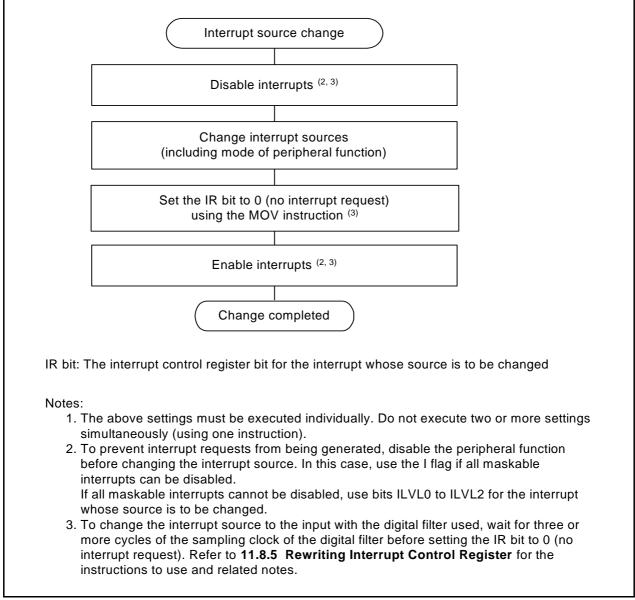
Figure 11.13 Procedure Example for Changing Interrupt Sources
