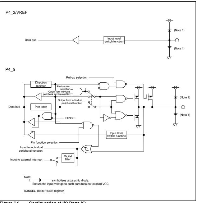
Figure 7.6 Configuration of I/O Ports (6)
