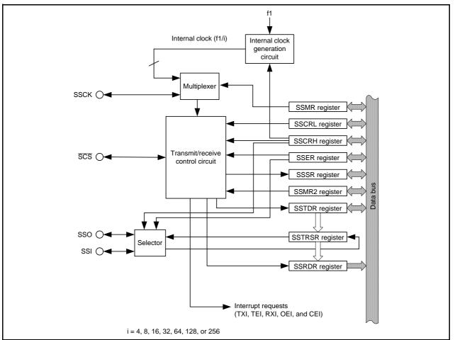
Figure 23.1 Block Diagram of Synchronous Serial Communication Unit
