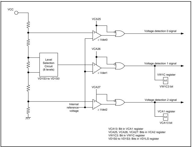
Figure 6.1 Voltage Detection Circuit Block Diagram
