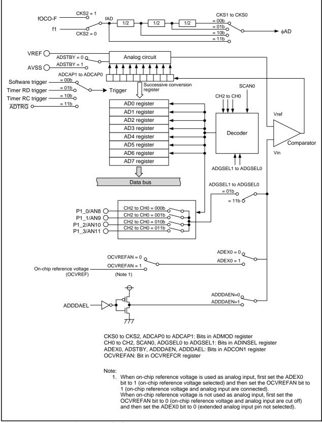
Figure 25.1 Block Diagram of A/D Converter
