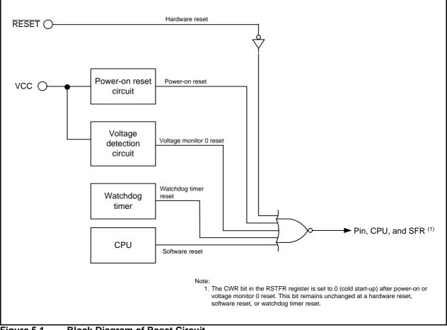
Figure 5.1 Block Diagram of Reset Circuit
