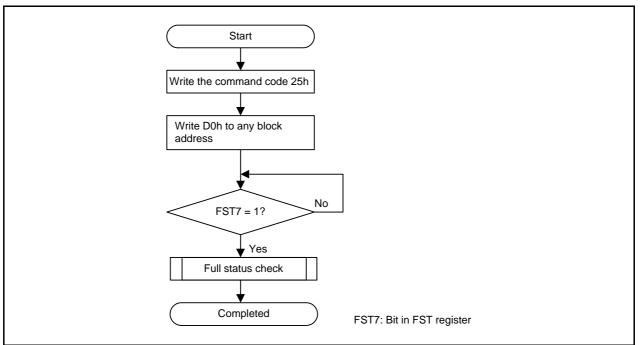
Figure 27.15 Block Blank Check Flowchart
