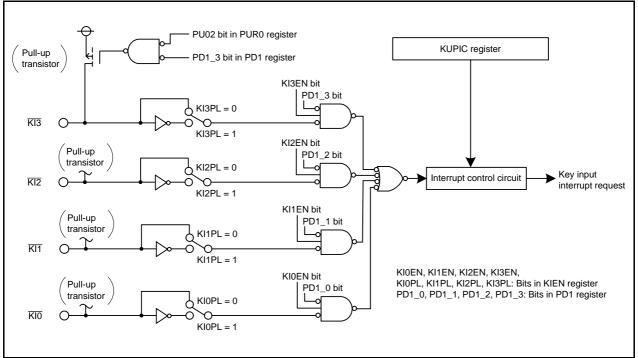
Figure 11.11 Block Diagram of Key Input Interrupt
