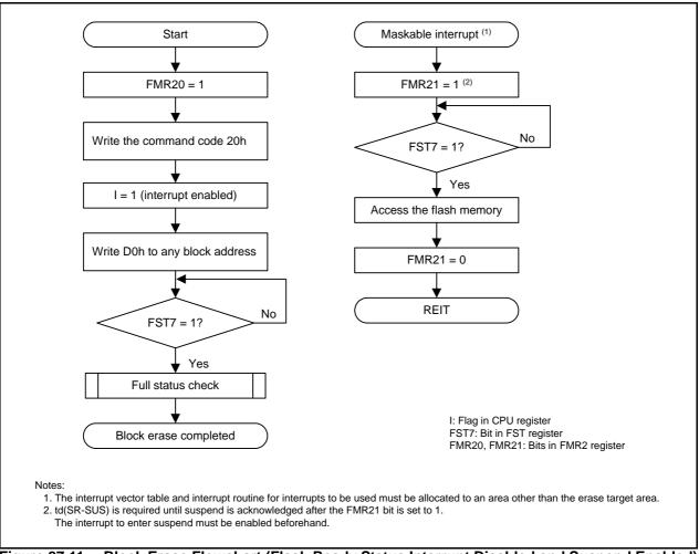
Figure 27.11 Block Erase Flowchart (Flash Ready Status Interrupt Disabled and Suspend Enabled)
