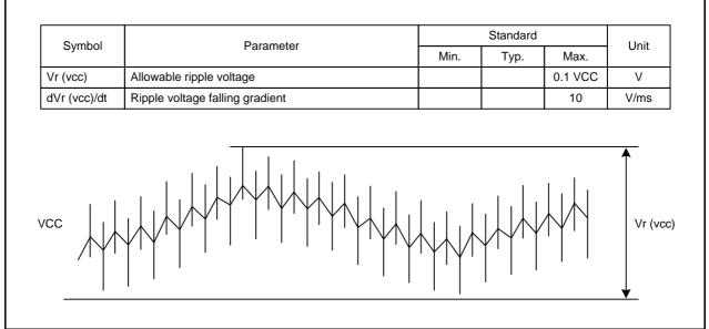
Figure 30.6 Definition of ripple voltage
