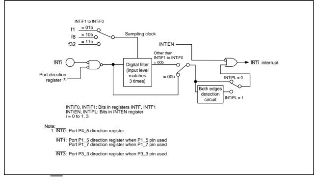
Figure 11.9 INTi Input Filter Configuration
