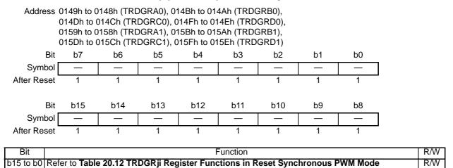
Access registers TRDGRAi to TRDGRDi in 16-bit units. Do not access them in 8-bit units.
