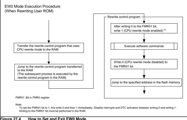
Figure 27.4 How to Set and Exit EW0 Mode
