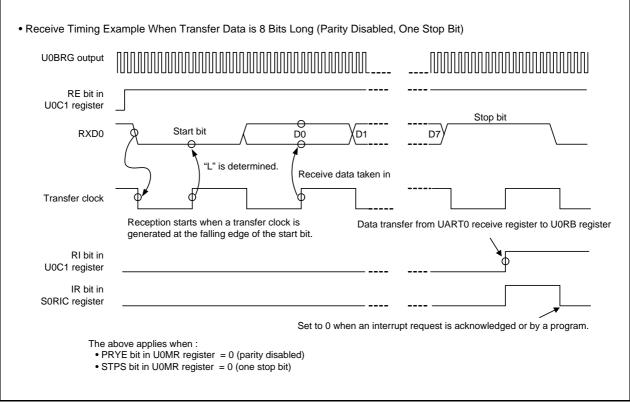
Figure 21.7 Receive Timing in UART Mode
