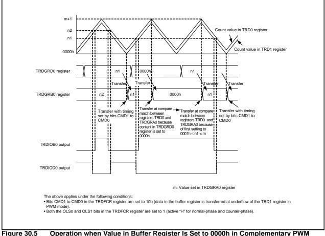
Figure 30.5 Operation when Value in Buffer Register Is Set to 0000h in Complementary PWM Mode
