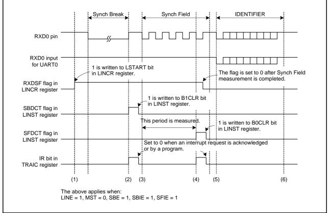
Figure 24.5 Operating Example during Header Field Reception
