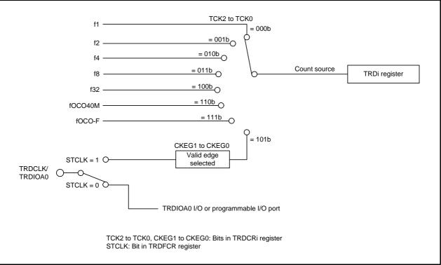
Figure 20.2 Block Diagram of Count Source
