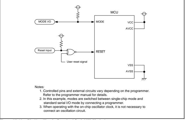
Figure 27.18 Pin Handling in Standard Serial I/O Mode 3
