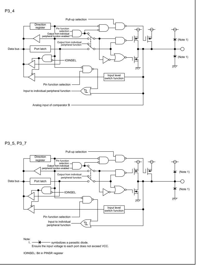
Figure 7.5 Configuration of I/O Ports (5)
