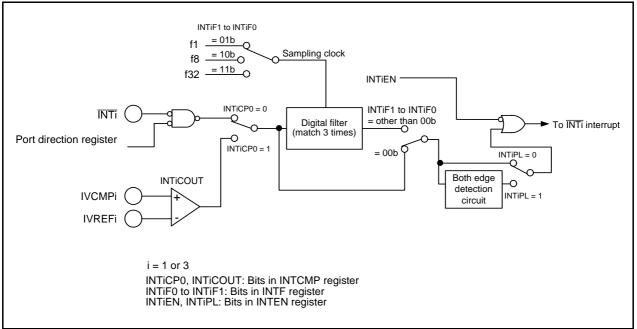
Figure 26.3 Configuration of Comparator Bi Digital Filter
