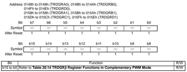
Access registers TRDGRAi to TRDGRDi in 16-bit units. Do not access them in 8-bit units. The TRDGRC0 register is not used in complementary PWM mode.
