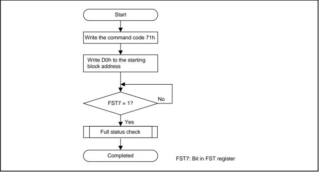
Figure 27.14 Read Lock Bit Status Flowchart
