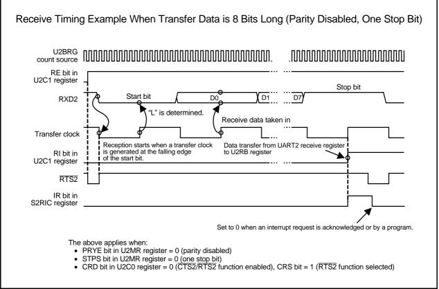
Figure 22.8 Receive Timing in UART Mode
