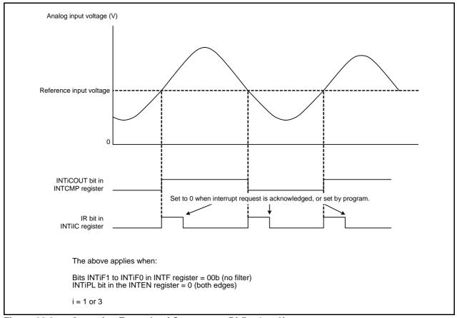
Figure 26.2 Operating Example of Comparator Bi (i = 1 or 3)
