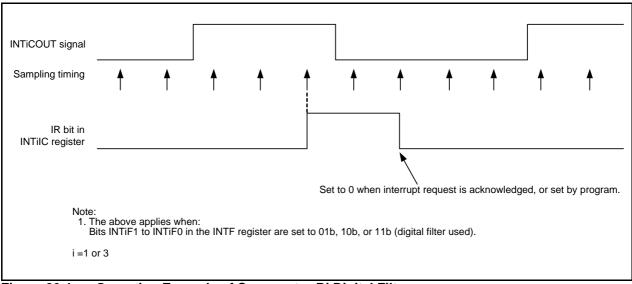
Figure 26.4 Operating Example of Comparator Bi Digital Filter
