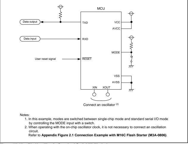
Figure 27.17 Pin Handling in Standard Serial I/O Mode 2
