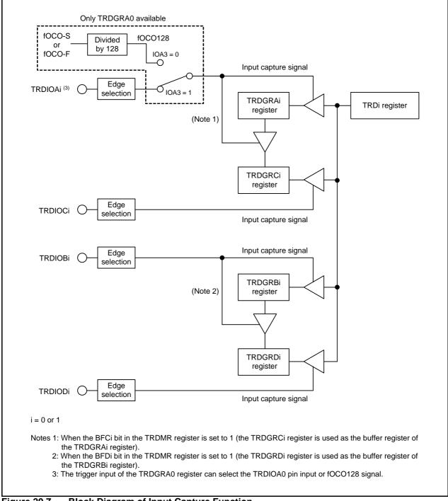
Figure 20.7 Block Diagram of Input Capture Function
