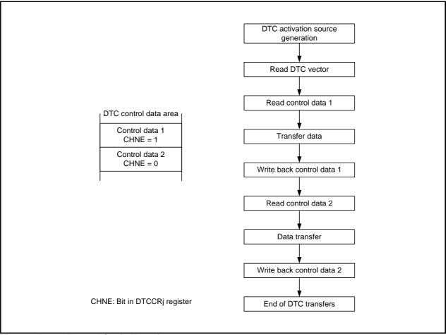
Figure 15.10 Flow of Chain Transfers
