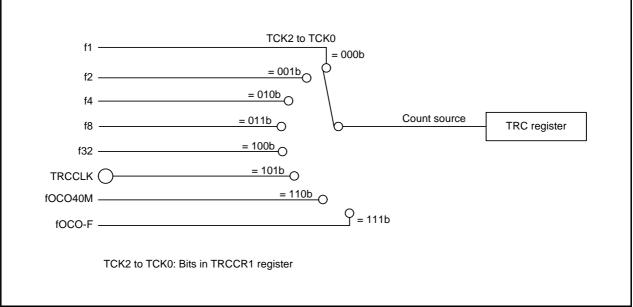
Figure 19.2 Count Source Block Diagram
