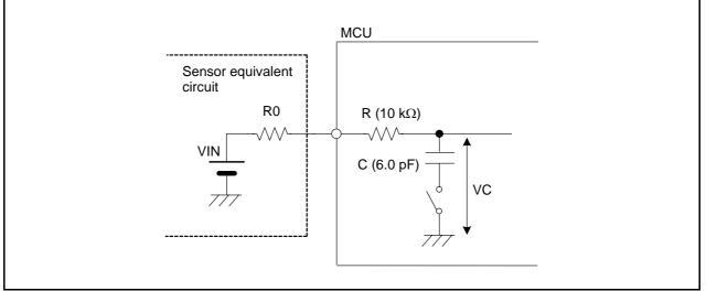
Figure 25.10 Analog Input Pin and External Sensor Equivalent Circuit
