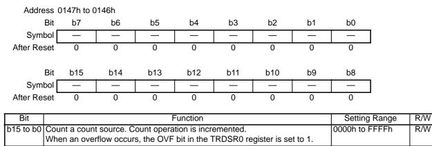
Access the TRD0 register in 16-bit units. Do not access it in 8-bit units. The TRD1 register is not used in PWM3 mode.
