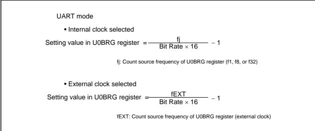
Figure 21.8 Formula for Calculating Setting Value in U0BRG Register
