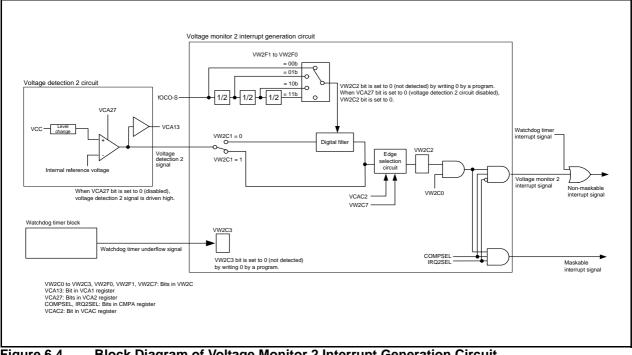
Block Diagram of Voltage Monitor 2 Interrupt Generation Circuit Figure 6.4
