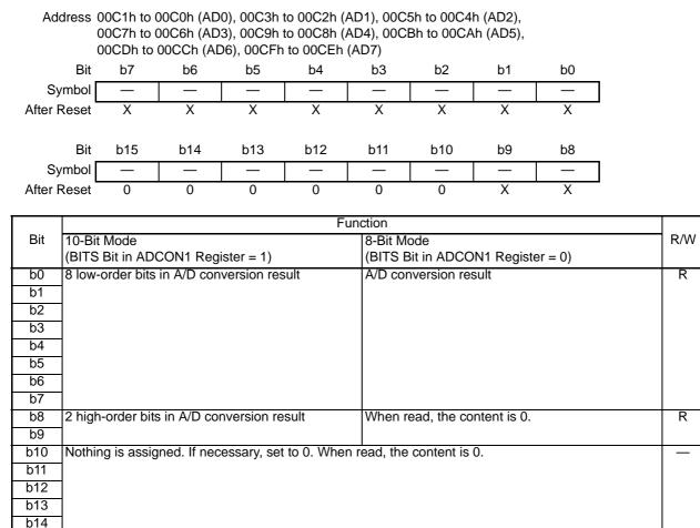
If the contents of the ADCON1, ADMOD, ADINSEL, or OCVREFCR register are written during A/D conversion, the conversion result is undefined.
