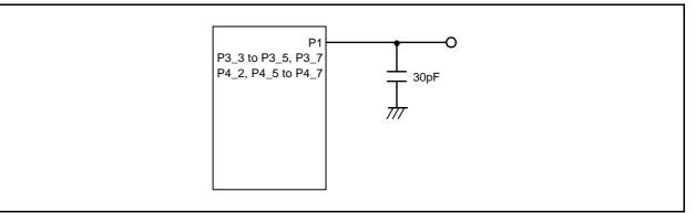
Figure 29.1 Ports P1, P3\_3 to P3\_5, P3\_7, P4\_2, and P4\_5 to P4\_7 Timing Measurement Circuit
