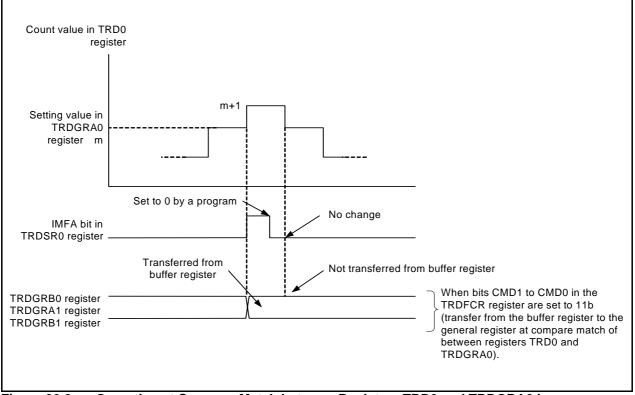
Figure 30.2 Operation at Compare Match between Registers TRD0 and TRDGRA0 in Complementary PWM Mode
