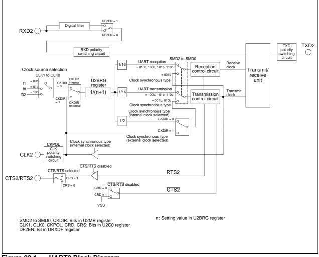
Figure 22.1 UART2 Block Diagram
