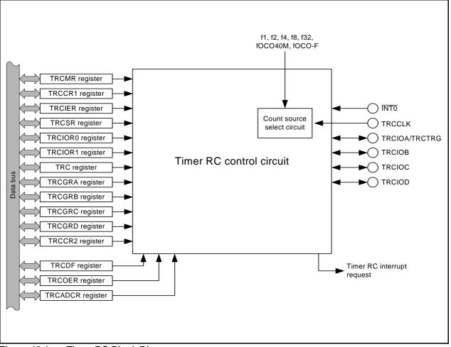
Figure 19.1 Timer RC Block Diagram
