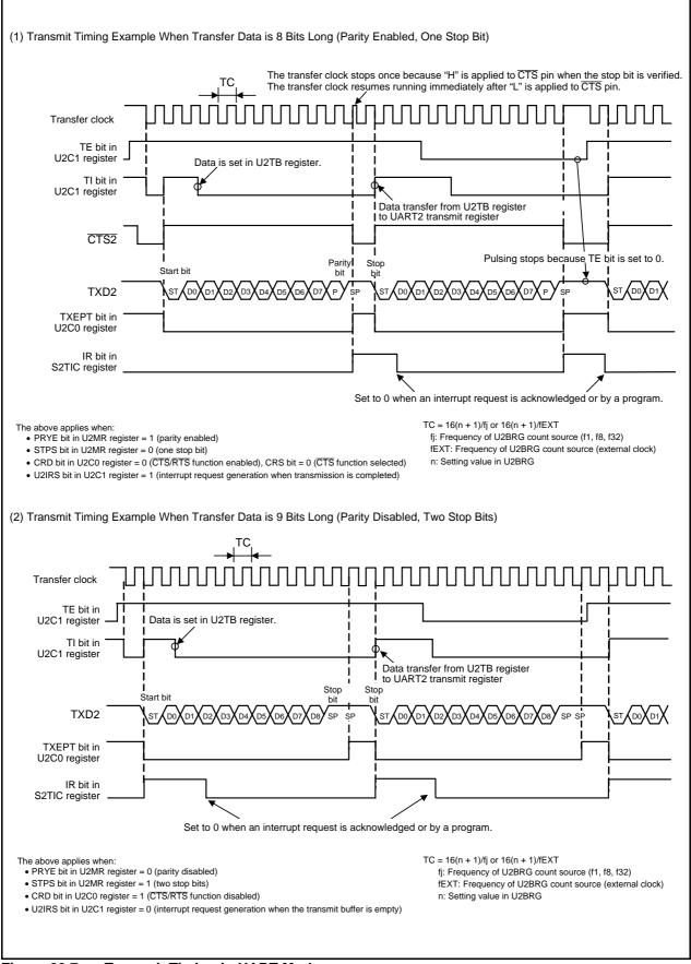
Figure 22.7 Transmit Timing in UART Mode
