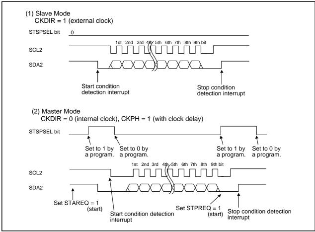
Figure 22.16 STSPSEL Bit Functions
