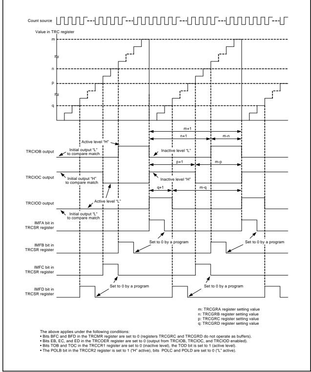
Figure 19.14 Operating Example of PWM Mode
