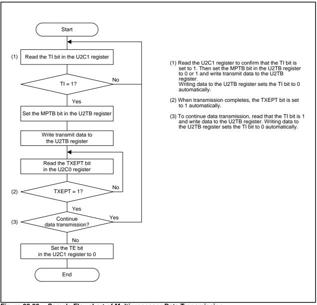
Figure 22.20 Sample Flowchart of Multiprocessor Data Transmission
