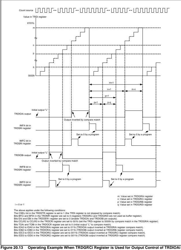
Pin and TRDGRDi Register is Used for Output Control of TRDIOBI Pin
