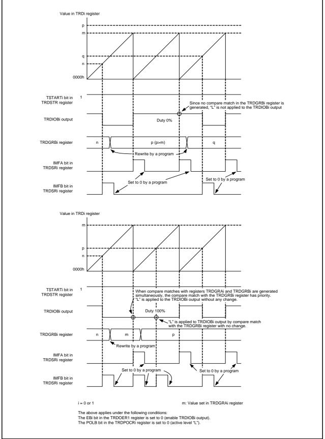
Figure 20.16 Operating Example of PWM Mode (Duty 0%, Duty 100%)
