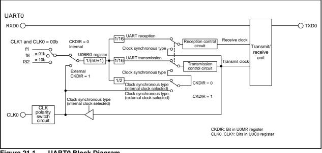
Figure 21.1 UART0 Block Diagram
