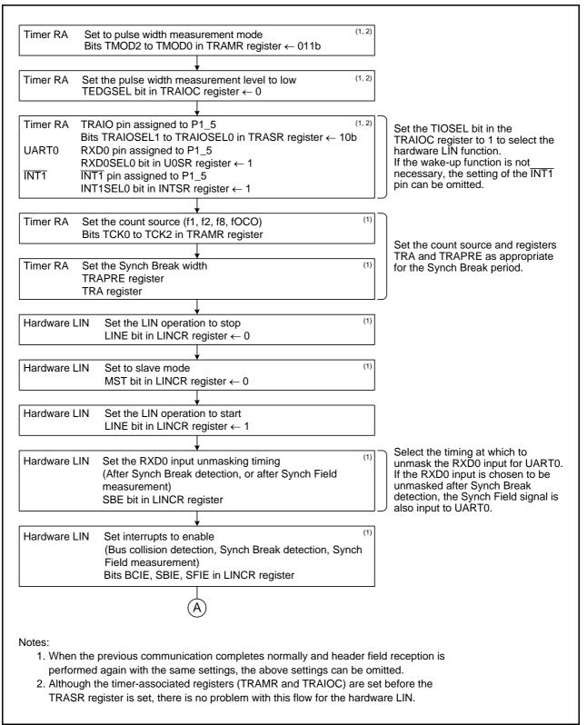
Figure 24.6 Header Field Reception Flowchart Example (1)
