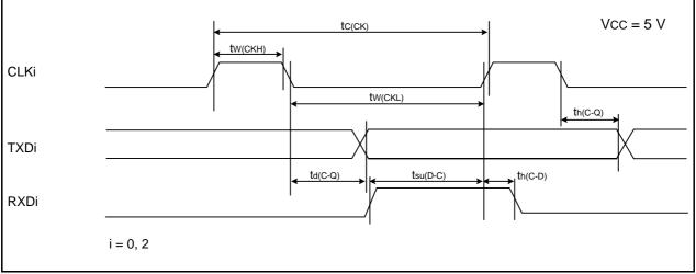
Figure 29.9 Serial Interface Timing Diagram when Vcc = 5 V
