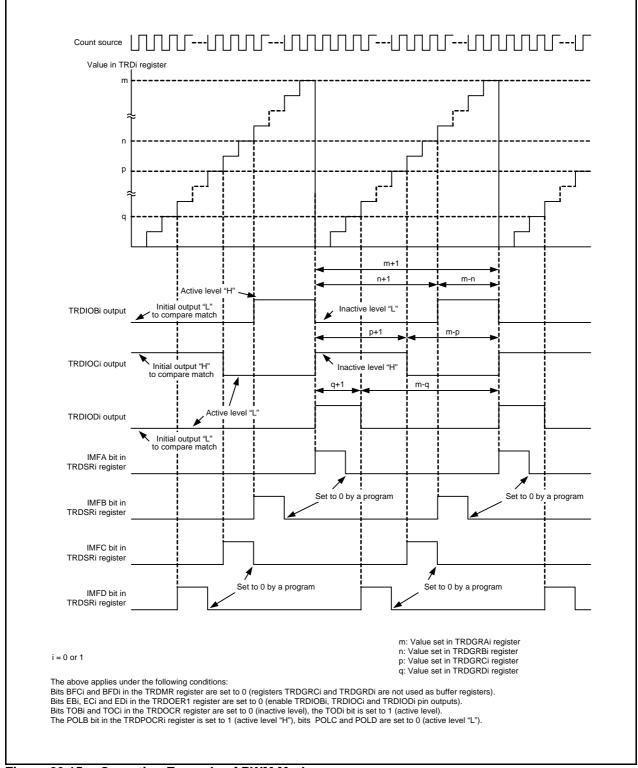
Figure 20.15 Operating Example of PWM Mode
