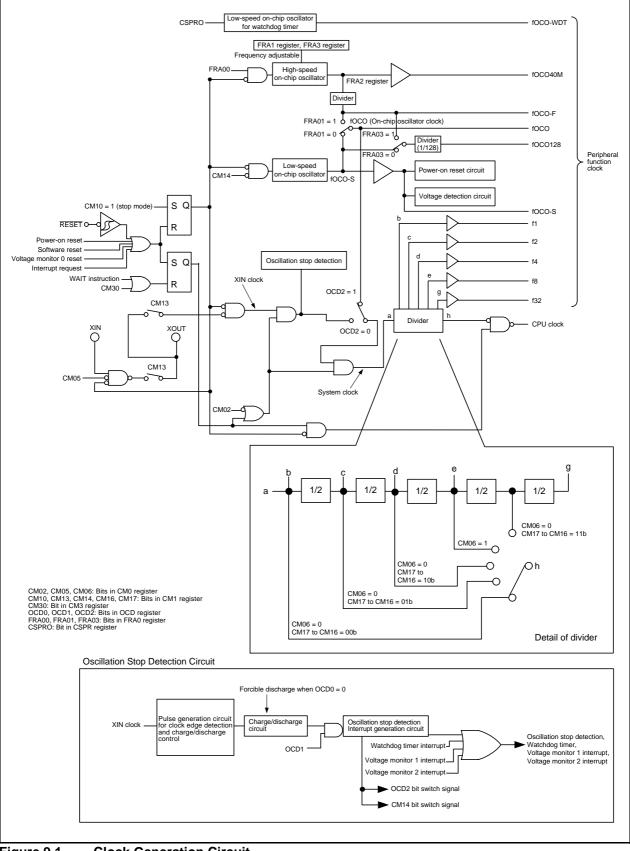
Figure 9.1 Clock Generation Circuit
