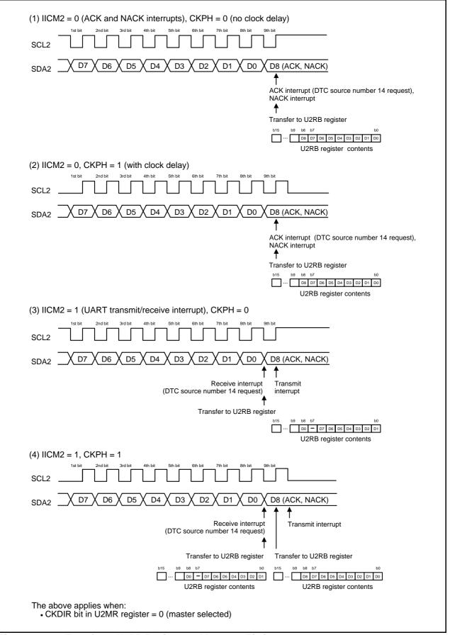
Figure 22.14 Transfer to U2RB Register and Interrupt Timing
