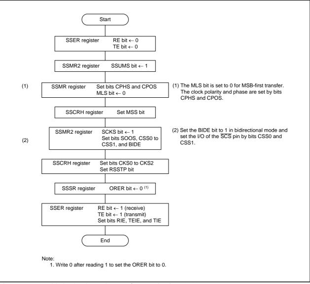
Figure 23.10 Initialization in 4-Wire Bus Communication Mode
