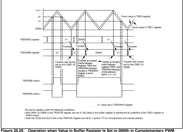
Figure 20.28 Operation when Value in Buffer Register Is Set to 0000h in Complementary PWM Mode
