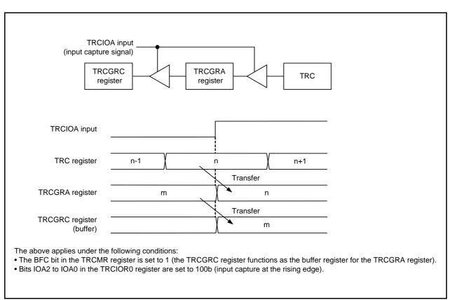
Figure 19.3 Buffer Operation for Input Capture Function
