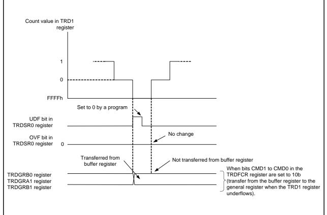
Figure 30.3 Operation when TRD1 Register Underflows in Complementary PWM Mode
