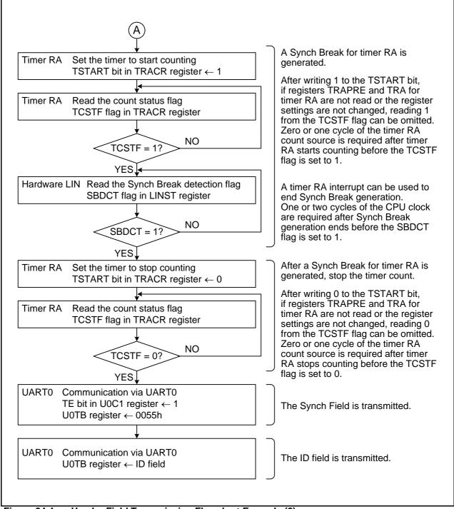
Figure 24.4 Header Field Transmission Flowchart Example (2)
