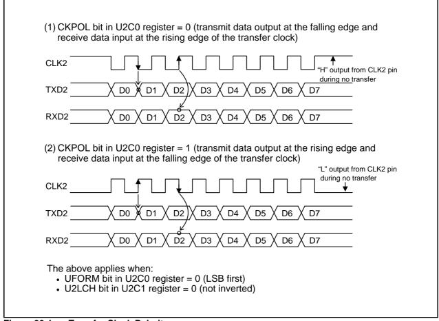
Figure 22.4 Transfer Clock Polarity
