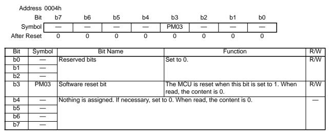
Set the PRC1 bit in the PRCR register to 1 (write enabled) before rewriting the PM0 register.
