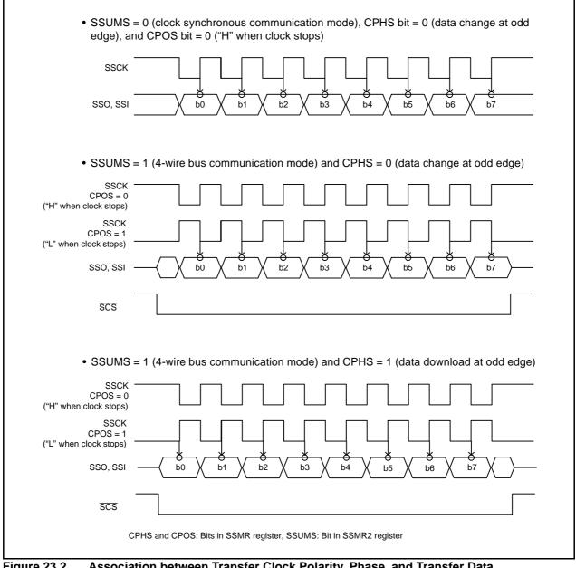
Association between Transfer Clock Polarity, Phase, and Transfer Data Figure 23.2
