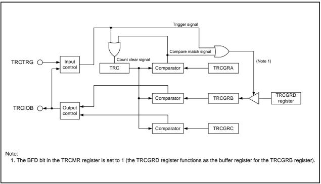
Figure 19.16 PWM2 Mode Block Diagram
