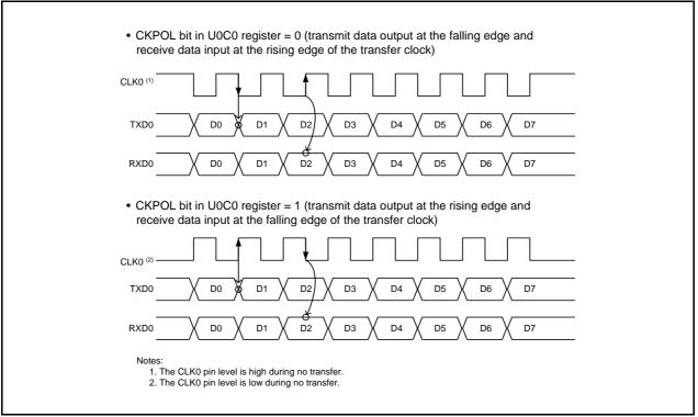
Figure 21.4 Transfer Clock Polarity
