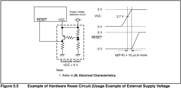
Figure 5.5 Example of Hardware Reset Circuit (Usage Example of External Supply Voltage Detection Circuit) and Operation
