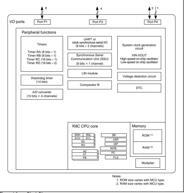
Figure 1.3 Block Diagram
