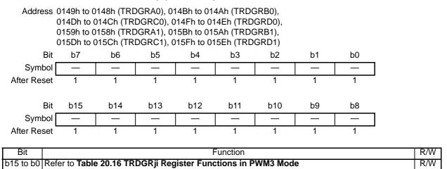
Access registers TRDGRAi to TRDGRDi in 16-bit units. Do not access them in 8-bit units.
