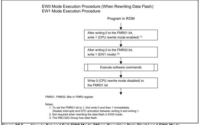
Figure 27.5 How to Set and Exit EW0 Mode (When Rewriting Data Flash) and EW1 Mode
