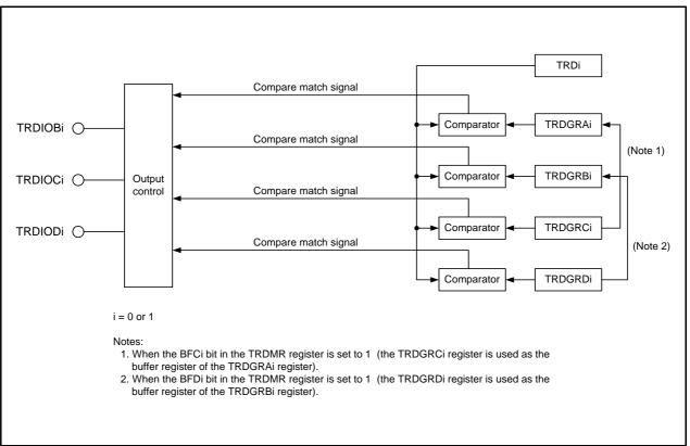
Figure 20.14 Block Diagram of PWM Mode
