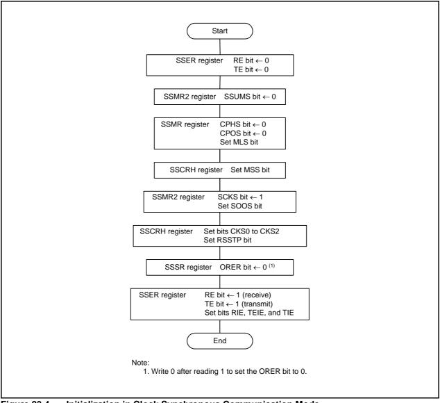
Figure 23.4 Initialization in Clock Synchronous Communication Mode
