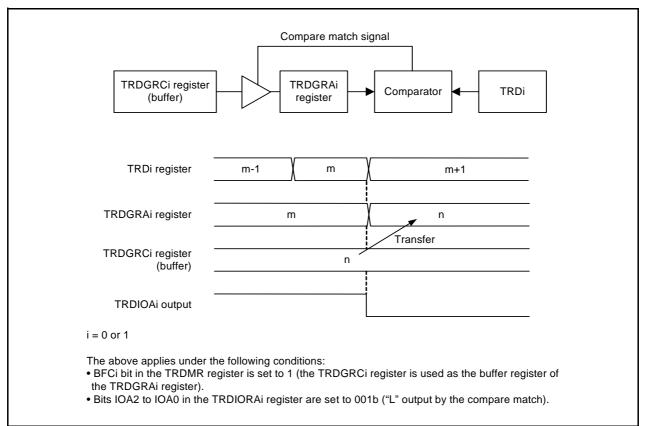
Figure 20.4 Buffer Operation in Output Compare Function
