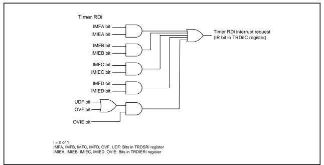
Figure 20.24 Block Diagram of Timer RD Interrupt
