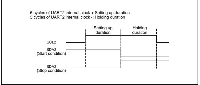
Figure 22.15 Detection of Start and Stop Conditions
