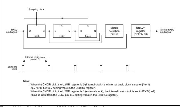
Figure 22.23 Block Diagram of RXD2 Digital Filter Circuit
