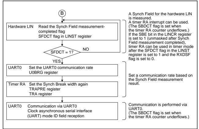
Figure 24.8 Header Field Reception Flowchart Example (3)
