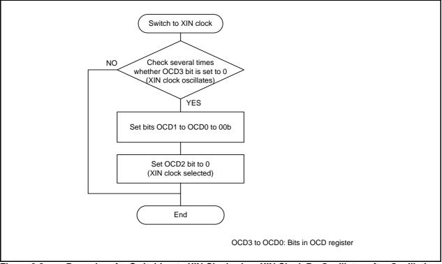
Figure 9.8 Procedure for Switching to XIN Clock when XIN Clock Re-Oscillates after Oscillation
