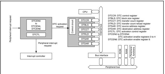
Figure 15.1 DTC Block Diagram
