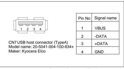
Figure 5.3 USB Host Connector (CN7) Pins
