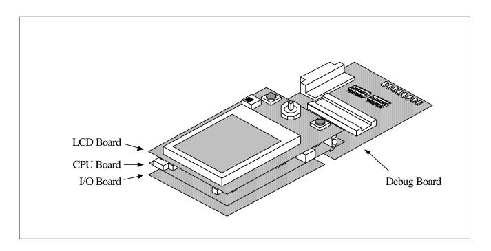
Figure 1.3 T-Engine - External View
