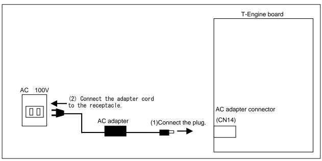
Figure 2.3 AC Adapter Connection Cord
