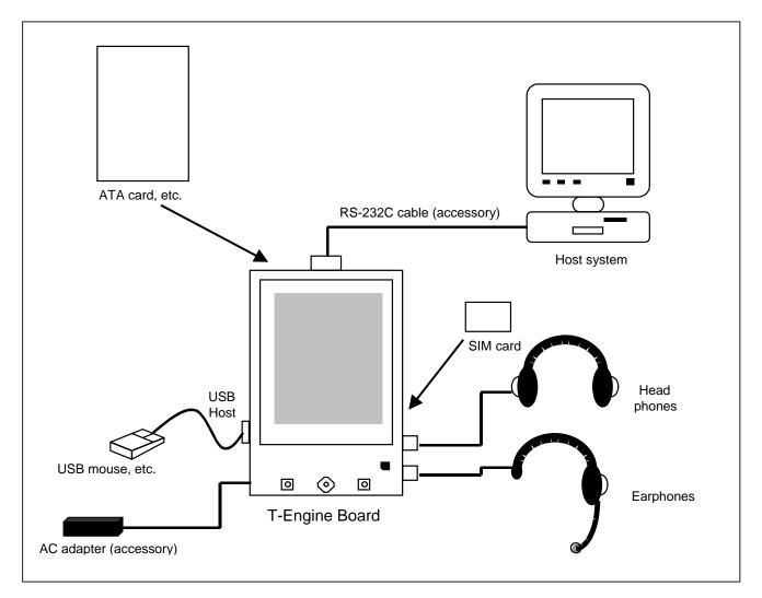
Figure 1.1 System configuration
