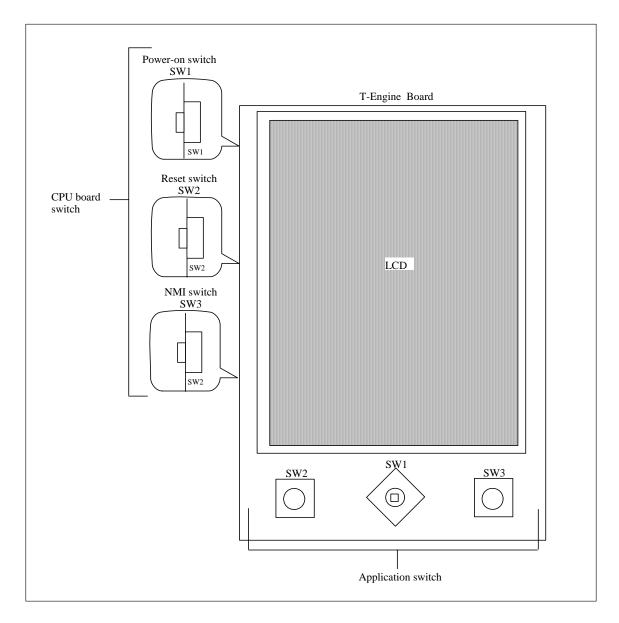
Figure 6.12 T-Engine Switch
