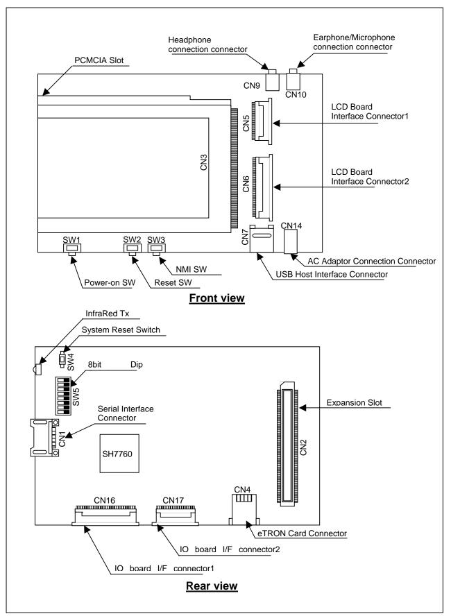
Figure 1.5 CPU Board - External View
