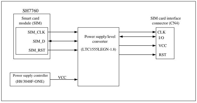
Figure 5.11 eTRON Interface Control Block
