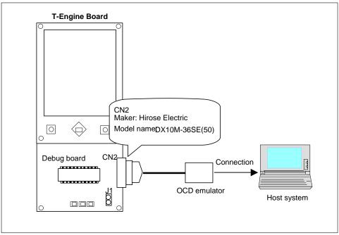
Figure 2.6 H-UDI Debugger Connection
