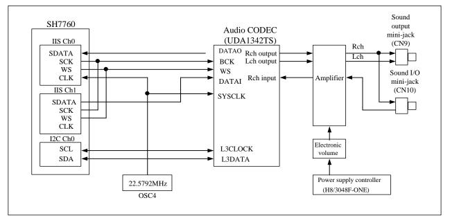
Figure 5.8 Sound Generator Control Block
