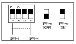
Figure 3.3 Setting the 4-bit DIP Switch
