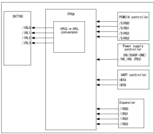
Figure 7.1 Interrupt Signal Mechanism
