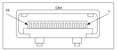
Figure 2.2 Serial Interface Connector Pins
