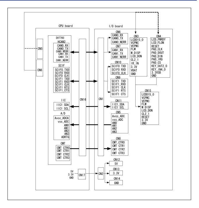
Figure 5.13 I/O Board Control Block
