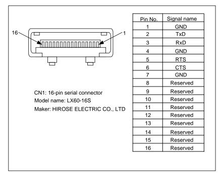
Figure 5.5 shows the pins of a 15-pin serial interface connector (CN1).
