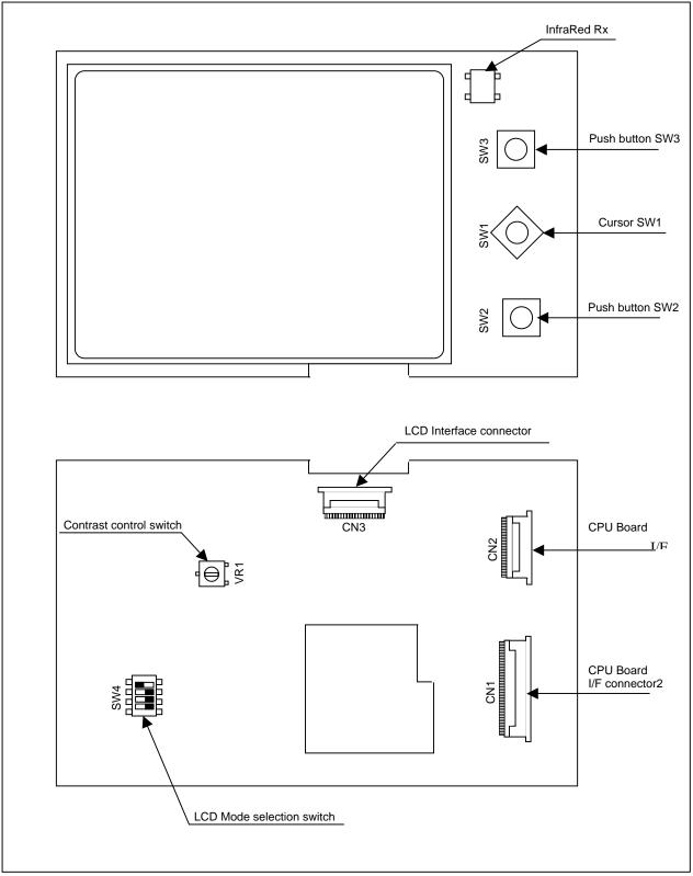
Figure 1.4 LCD Board - External View
