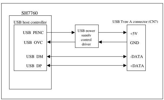
Figure 5.2 USB Host Control Block
