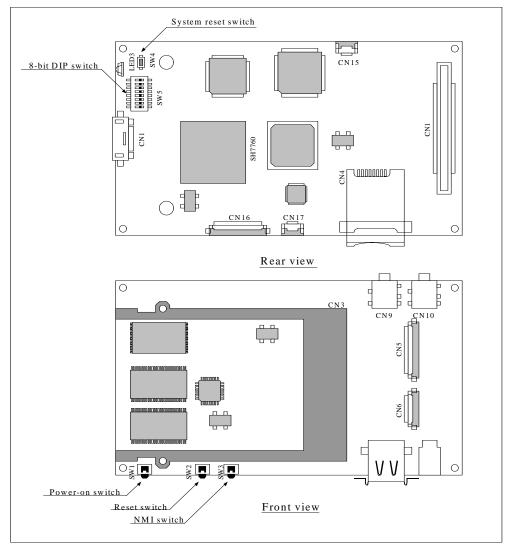
Figure 3.1 CPU Board Switches (SW1 to SW5)
