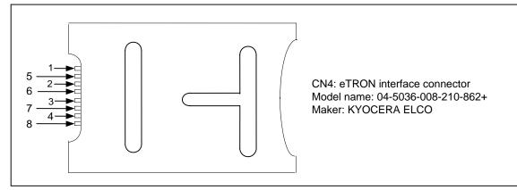
Figure 5.12 eTRON Interface Connector (CN4) Pins
