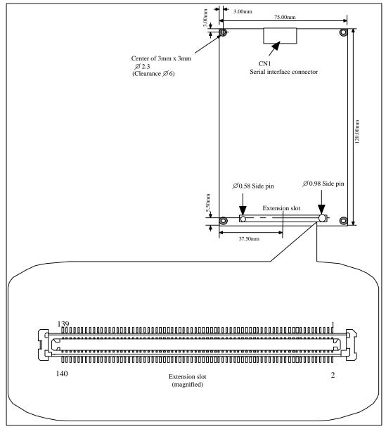
Figure 8.1 Extension Slot Position
