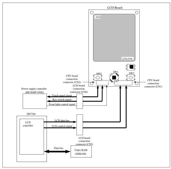
Figure 5.6 LCD Control Block
