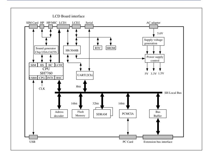
Figure 1.2 T-Engine Block Diagram
