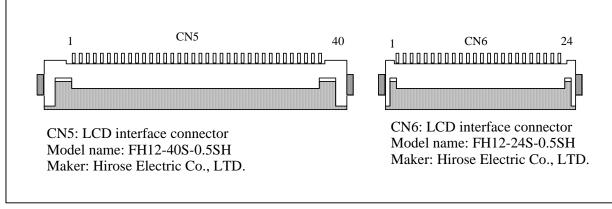
Figure 5.7 LCD Interface Connector (CN5/CN6) Pins
