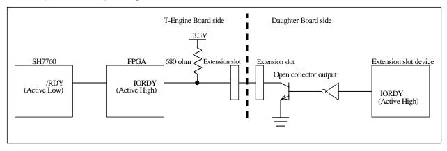
Figure 9.3 Extension Slot IORDY Pin Structure
