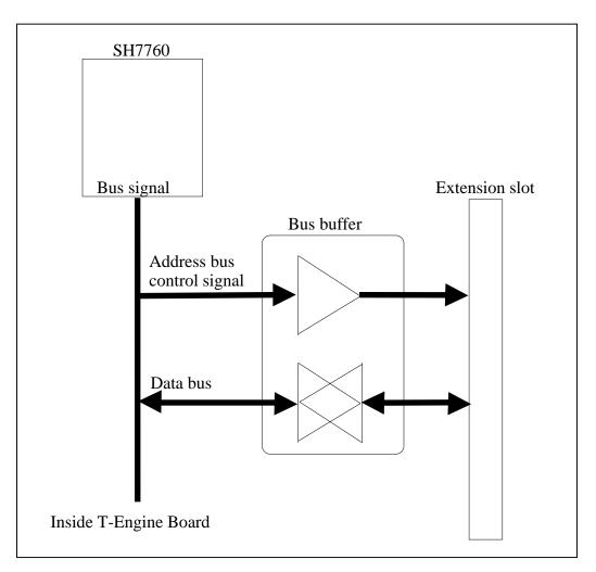
Figure 9.4 Extension Slot Bus Buffer Structure
