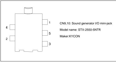
Figure 5.9 Sound Generator I/O Mini-jack (CN9, CN10) Pins
