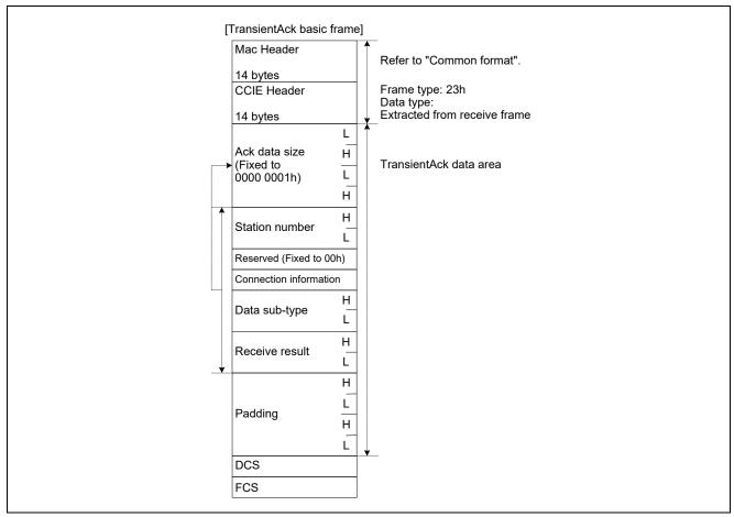
Figure 7.17Overview of TransientAck Frame Format
