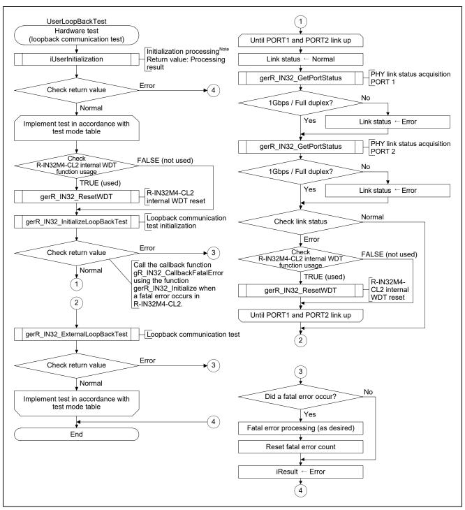
Figure 4.41Flowchart for Hardware Test (Loopback Communication Test)
