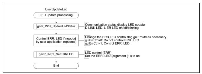
Figure 4.11Flowchart for LED Update Processing
