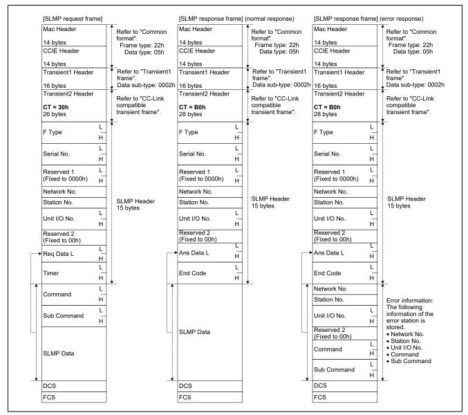
Figure 7.14Overview of SLMP Frame Basic Format
