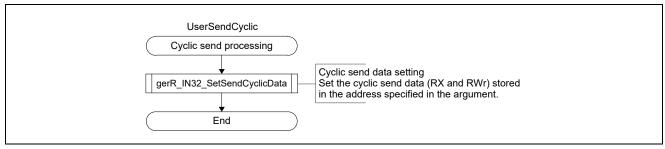
Figure 4.9 Flowchart for Cyclic Send Processing
