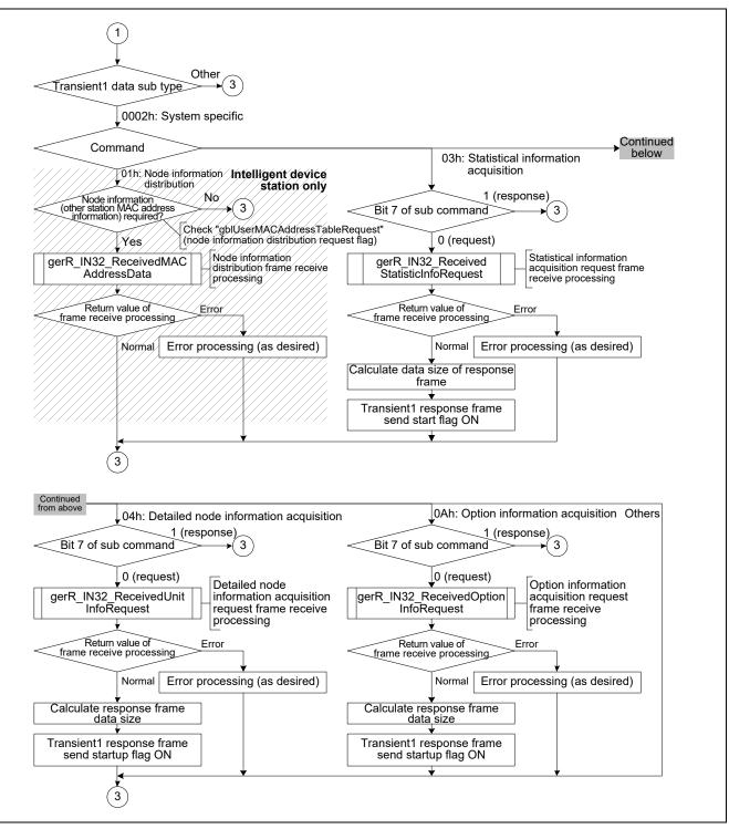
Figure 4.17Flowchart for Transient1 Receive Data Processing (2/4)
