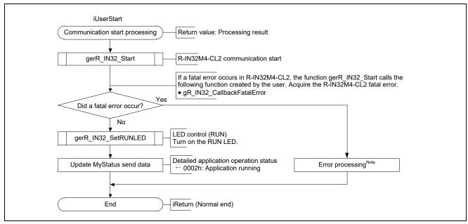
Figure 4.3 Flowchart for Communication Start Processing
