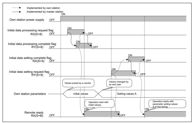
Figure 6.4 Timing Chart: Initial Data Processing and Setting
