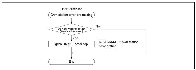
Figure 4.4 Flowchart for Own Station Error Processing
