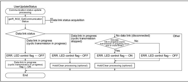
Figure 4.10Flowchart for Communication Status Update Processing
