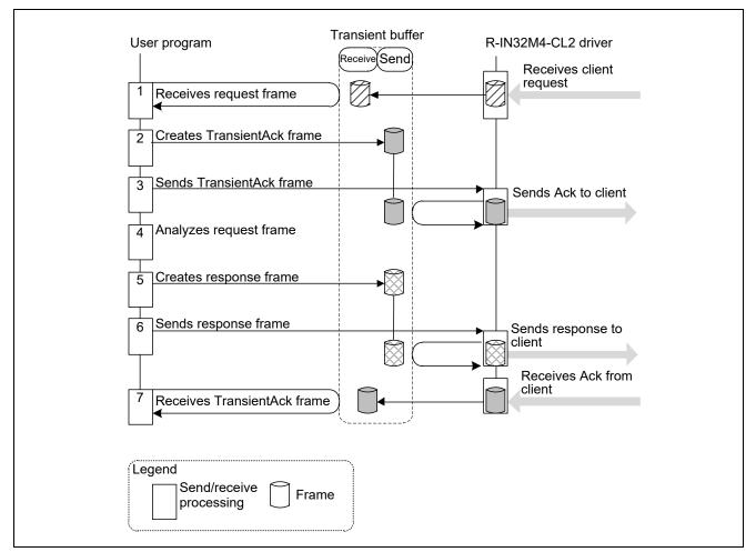
Figure 4.14Server Processing Procedure
