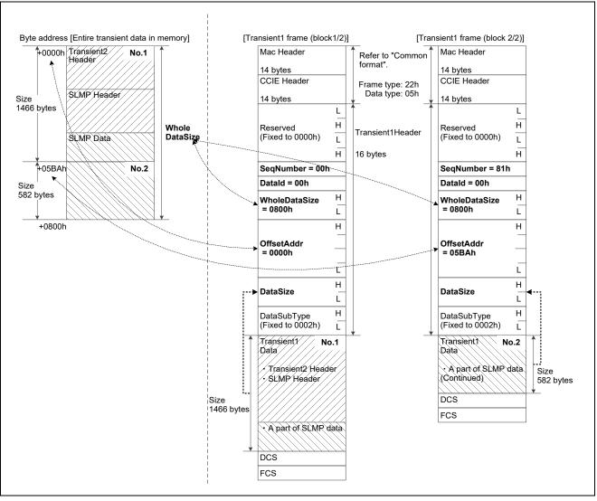
Figure 7.3 Example of Transient1 Frame Division
