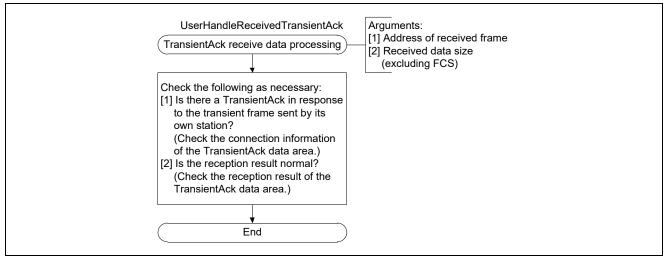
Figure 4.28Flowchart for TransientAck Receive Data Processing
