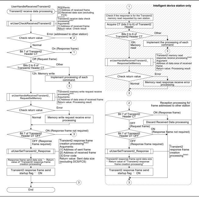
Figure 4.24Flowchart for Transient2 Receive Data Processing
