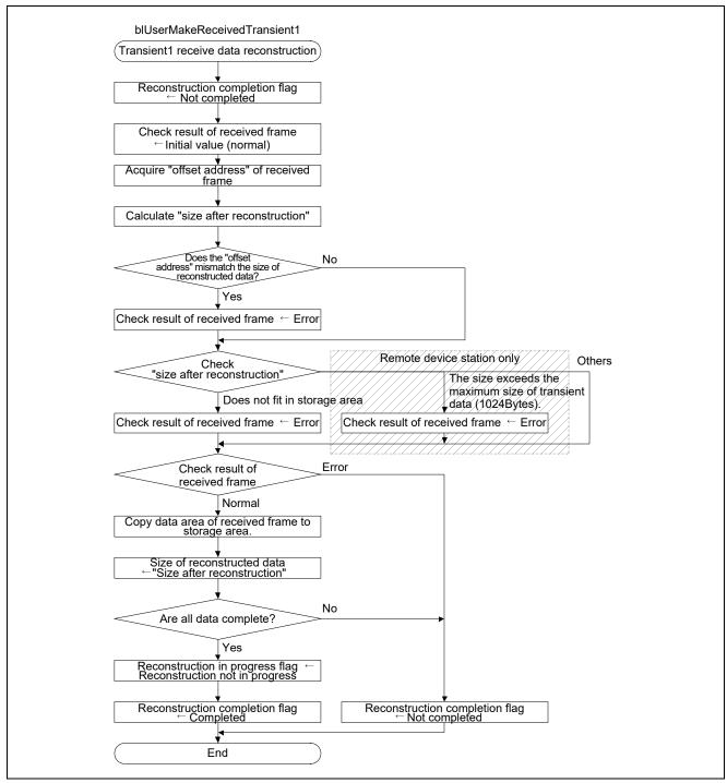
Figure 4.21Flowchart for Transient1 Receive Data Reconstruction Processing
