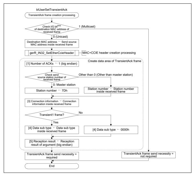
Figure 4.29Flowchart for TransientAck Frame Creation Processing
