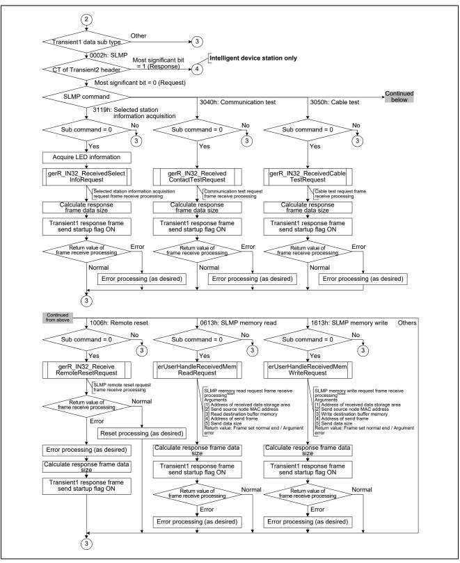
Figure 4.17Flowchart for Transient1 Receive Data Processing (3/4)
