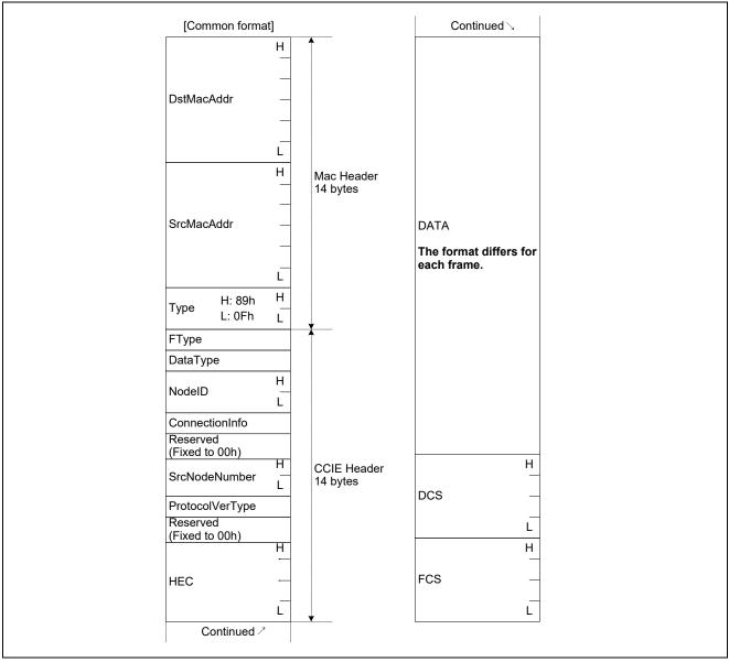
Figure 7.1 Overview of Frame Common Format
