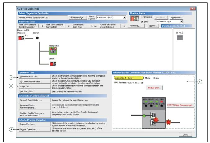
Figure 3.6 Diagnostic Window/Operation Locations (GX Works2)
