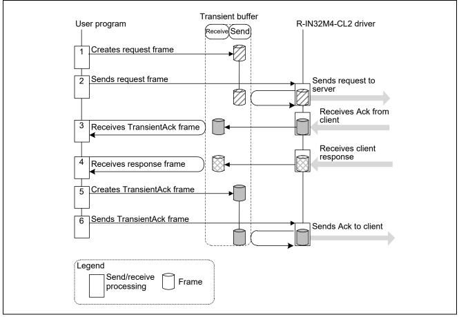
Figure 4.15Client Processing Procedure
