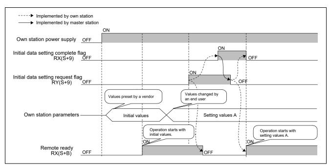
Figure 6.3 Timing Chart: Initial Data Setting Complete/Request Flag
