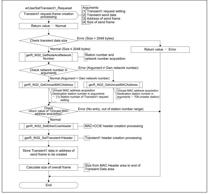
Figure 4.35Flowchart for Transient1 Request Frame Creation Processing
