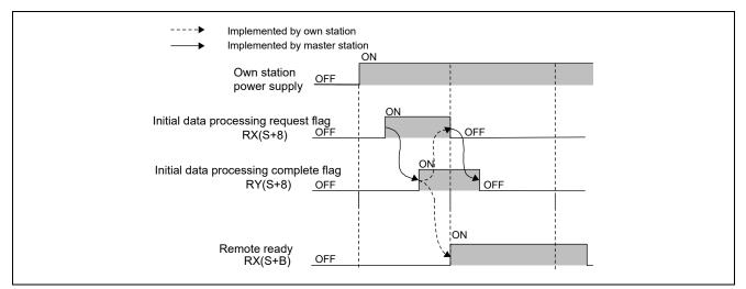
Figure 6.2 Timing Chart: Initial Data Processing Request/Complete Flag
