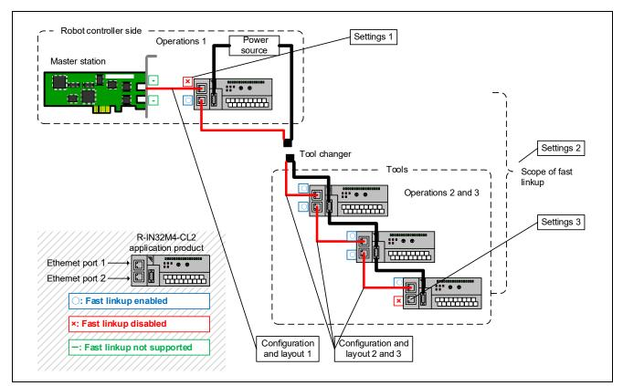
Figure 3.2 System Configuration with Fast Linkup (for an Industrial Robot Arm)
