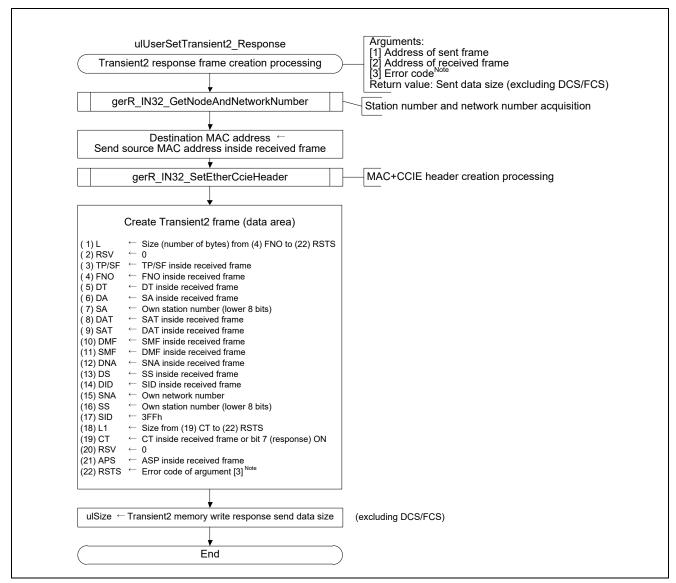
Figure 4.27Flowchart for Transient2 Response Frame Creation Processing
