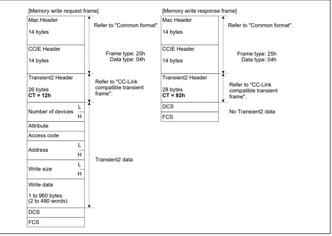
Figure 7.11Overview of Memory Write Frame Format
