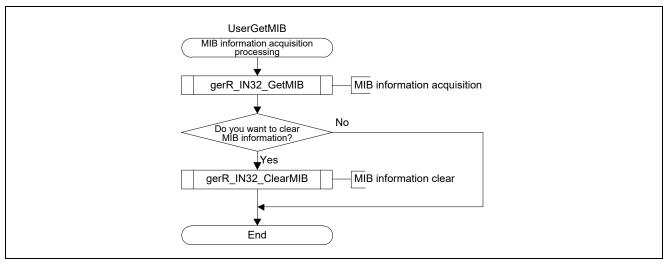
Figure 4.13Flowchart for MIB Information Acquisition Processing
