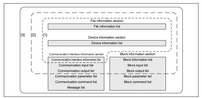
Figure 2.3 CSP+ File Section Configuration
