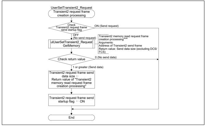
Figure 4.37Flowchart for Transient2 Request Frame Creation Processing
