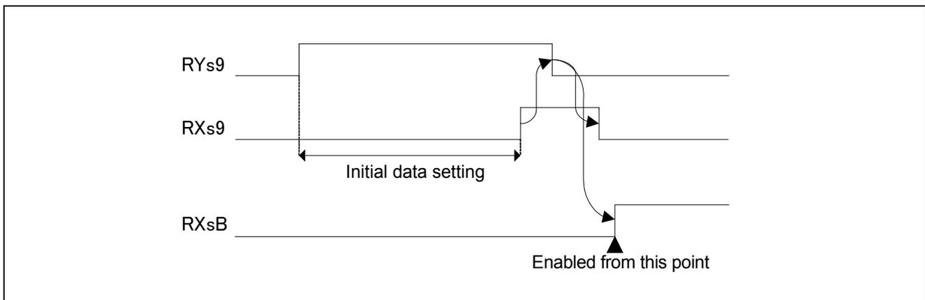
Figure 8.3 RXs9/RYs9 (initial data setting complete / setting request flag)
