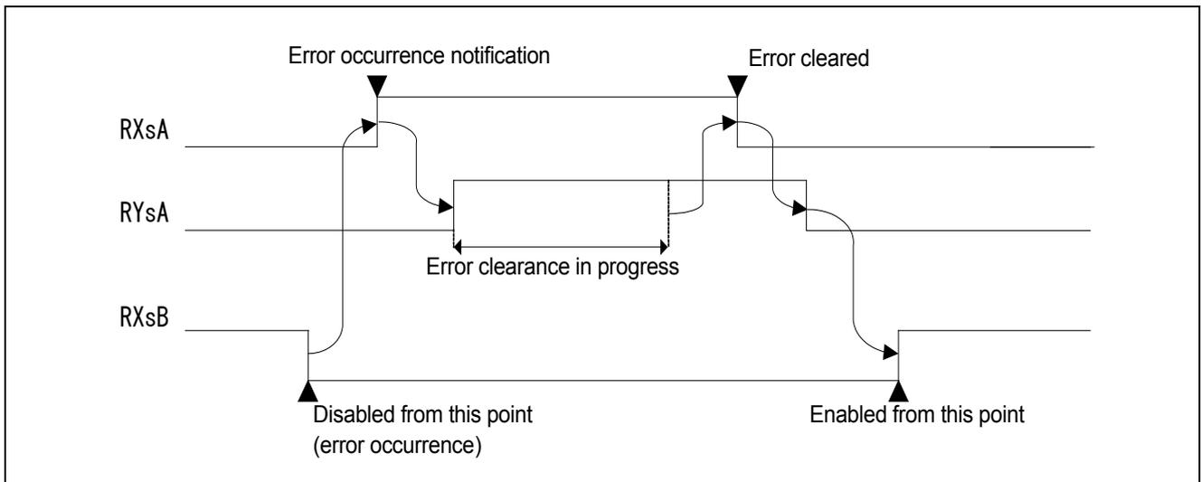
Figure 8.5 RXsA/RYsA (error status / reset request flag)
