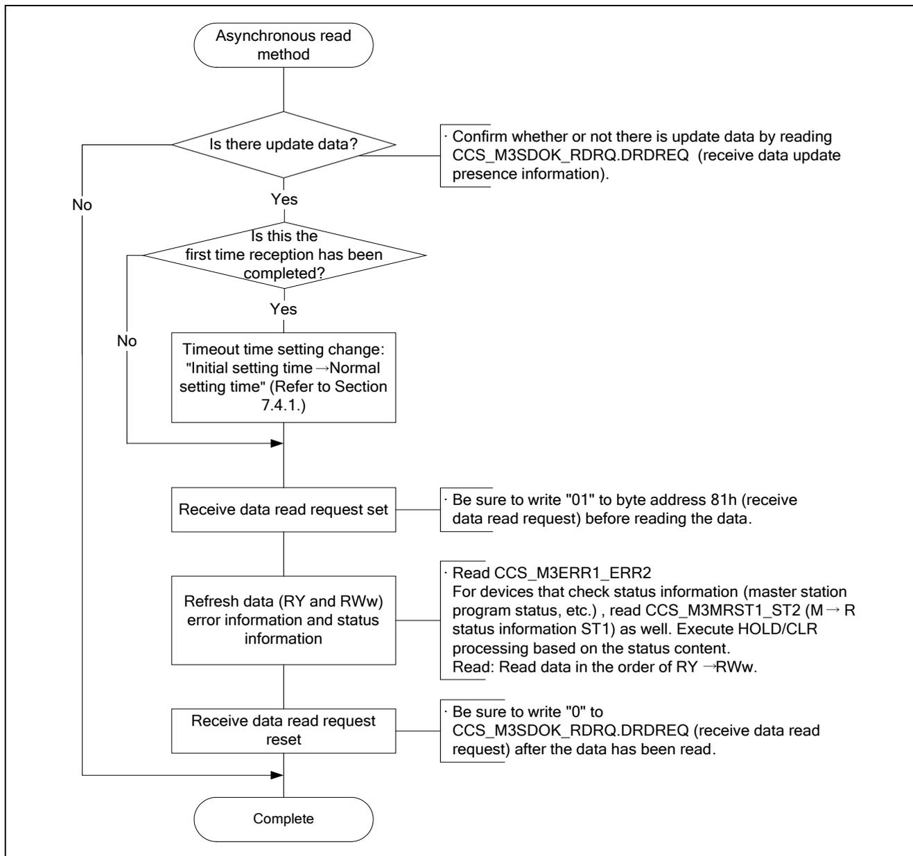
Figure 7.5 Asynchronous Read Method
