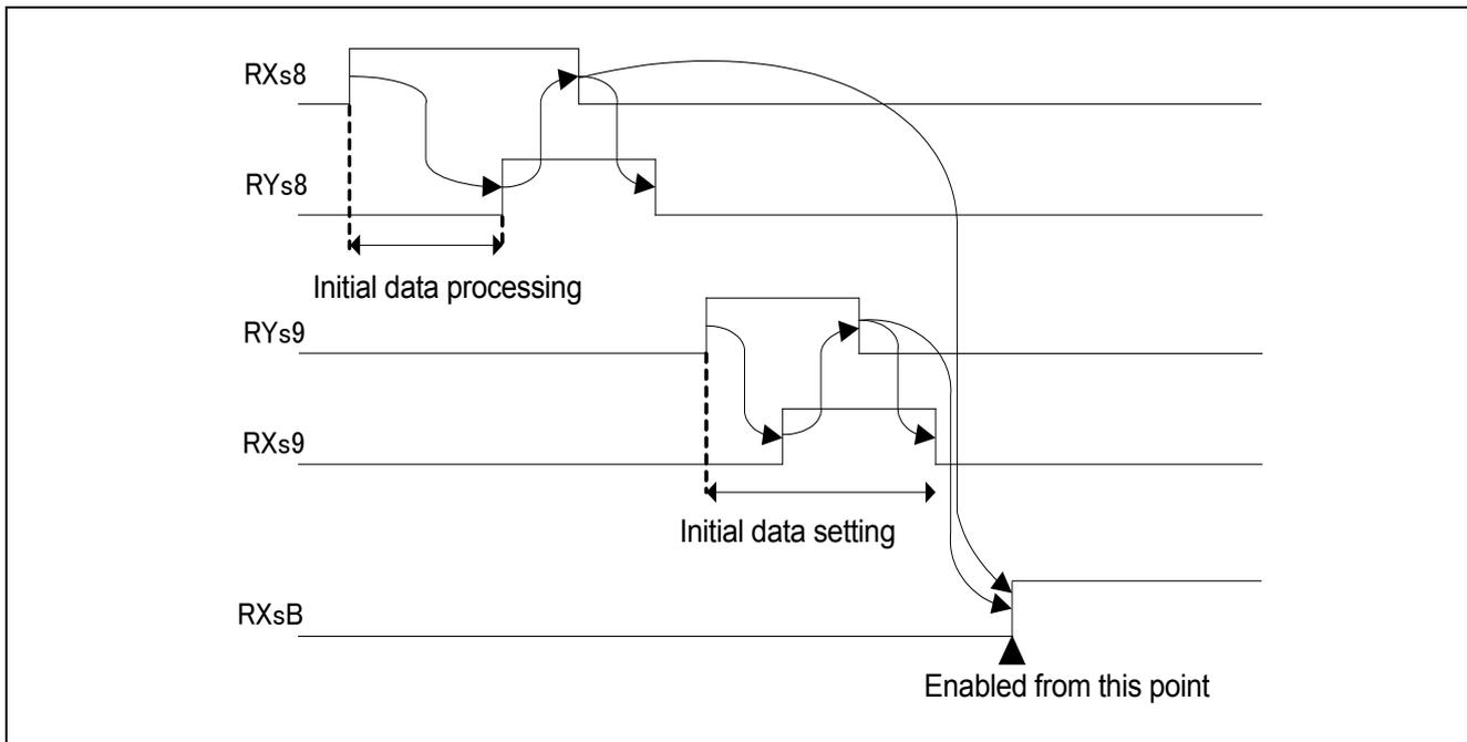
Figure 8.4 When both RXs8/RYs8 and RXs9/RYs9 are implemented
