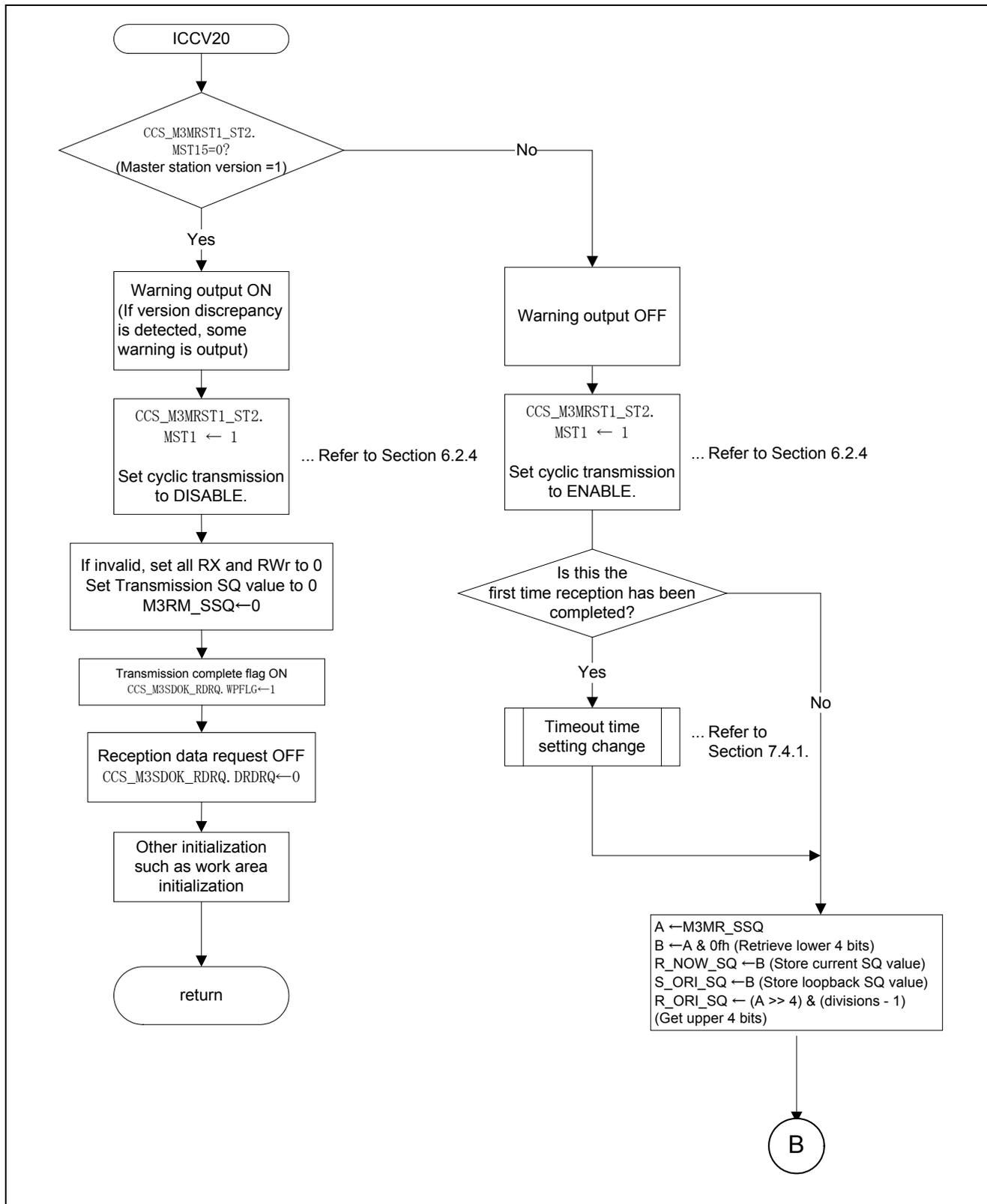
Figure 10.4 Transmission/Reception Processing Module (ICCV20)
