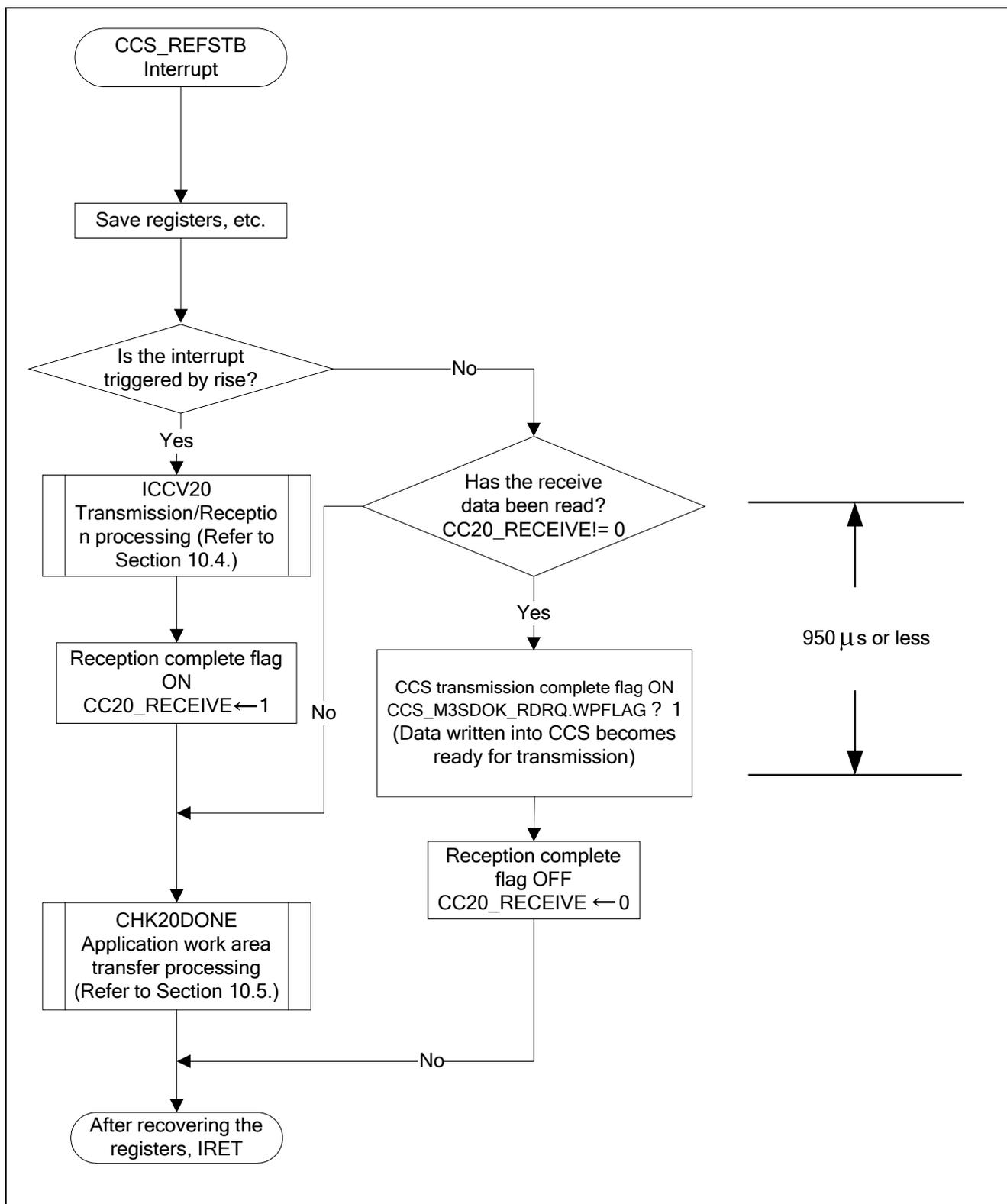
Figure 10.2 Transmission/Reception Processing Using Interrupt (CCS\_REFSTB signal)
