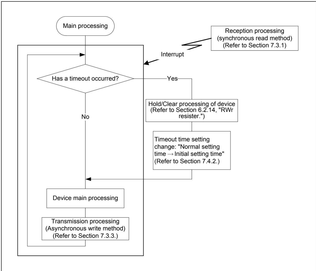
Figure 7.2 Synchronous Read Method / Asynchronous Write Method
