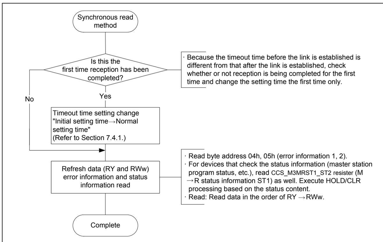
Figure 7.4 Synchronous Read Method
