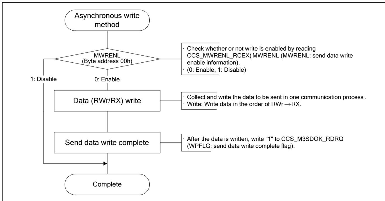
Figure 7.6 Asynchronous Write Method
