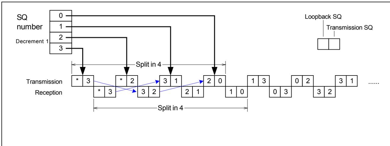
Figure 9.5 Details of SQ value(loopback)
