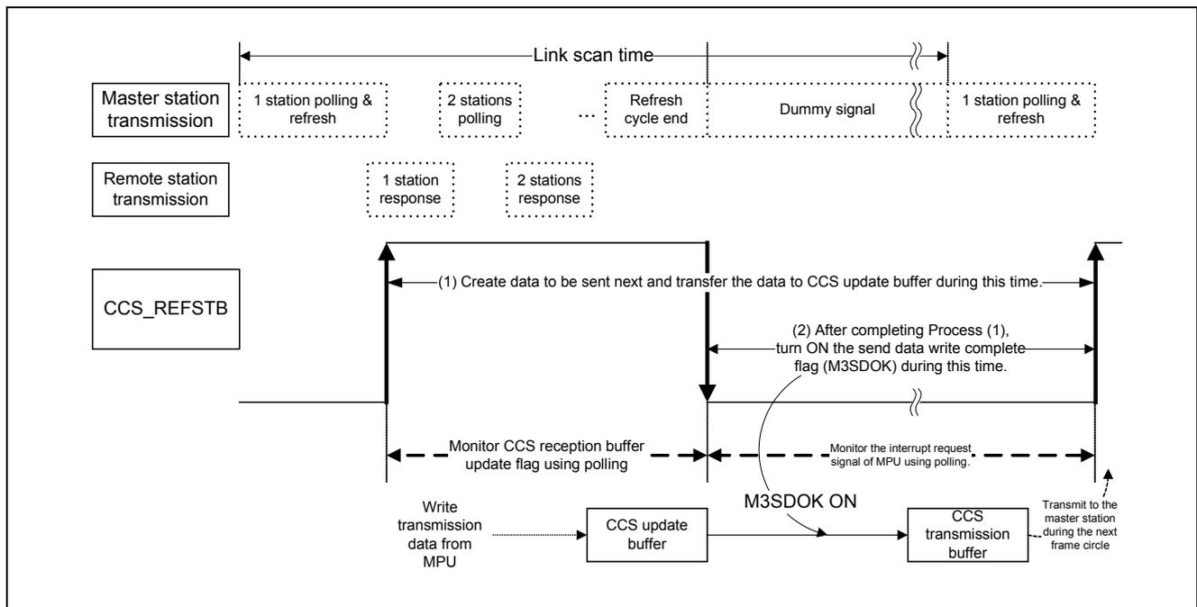
Figure 11.1 Link Scan Time and CCS\_REFSTB Signal Change
