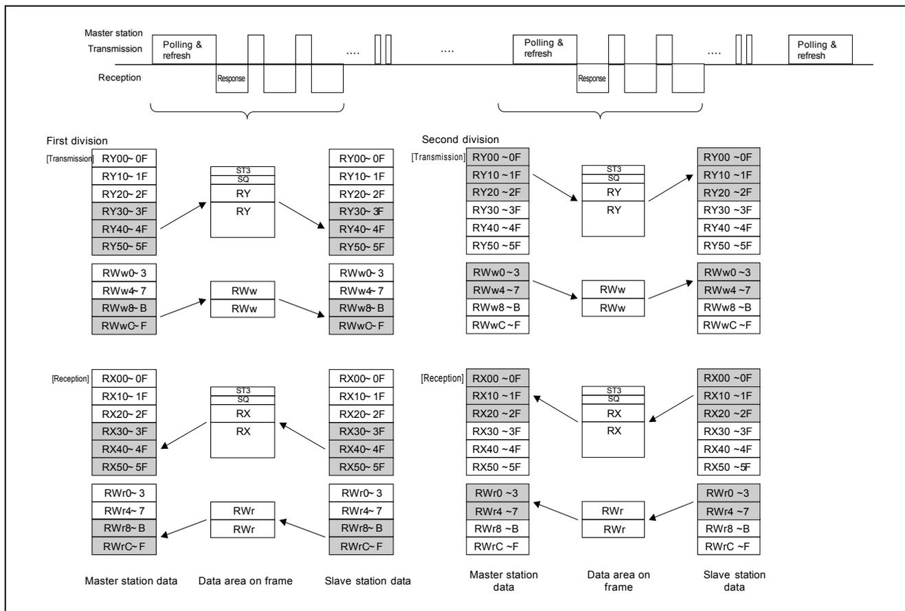
Figure 9.1 With 2 occupied stations and extended cyclic 2 × setting
