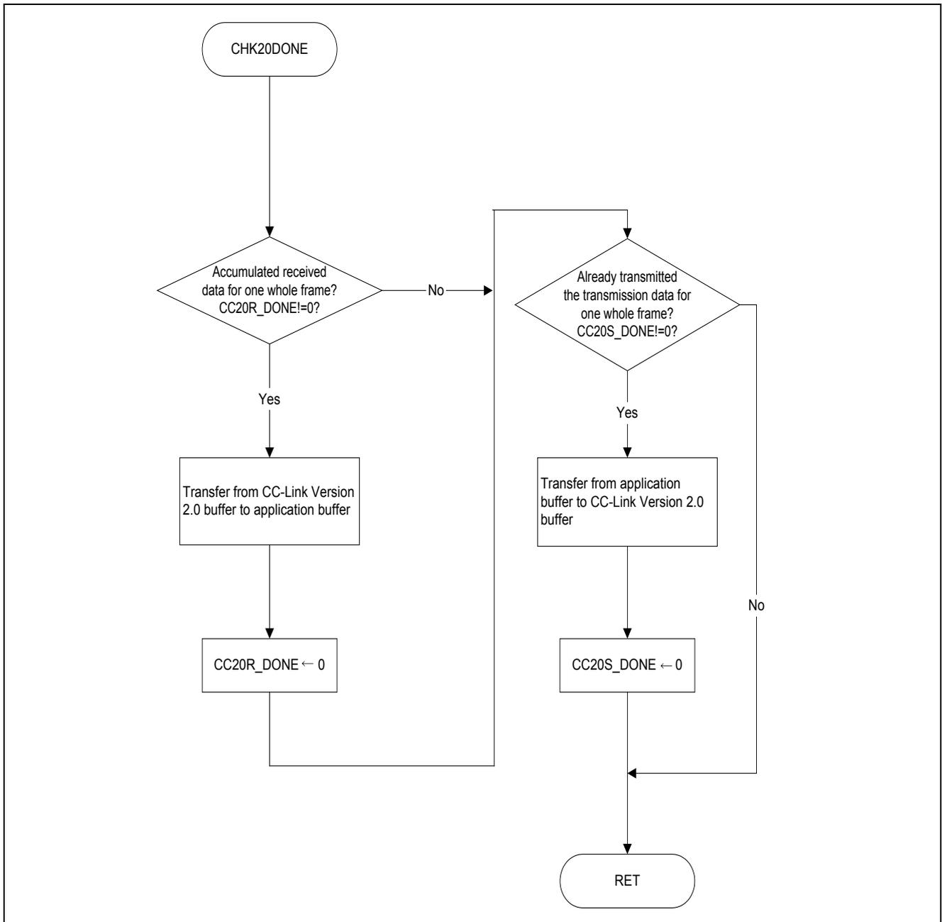
Figure 10.8 Application Work Area Transfer Processing Module CHK20DONE
