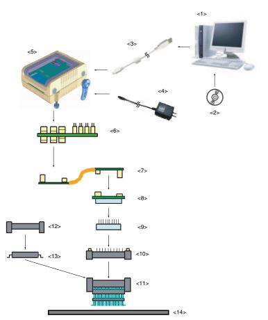
Figure 1-1. System Configuration
