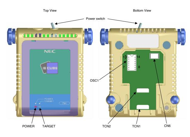
Figure 2-1. Names of Parts of QB-78K0RIX3
