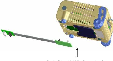
Insert CN1 and CN2 of the probe into TCN1 and TCN2 of the QB-78K0RIX3.
