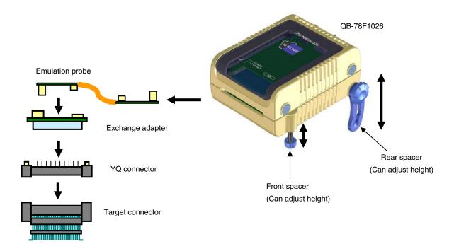
Figure 2-8. Connection Using Emulation Probe
