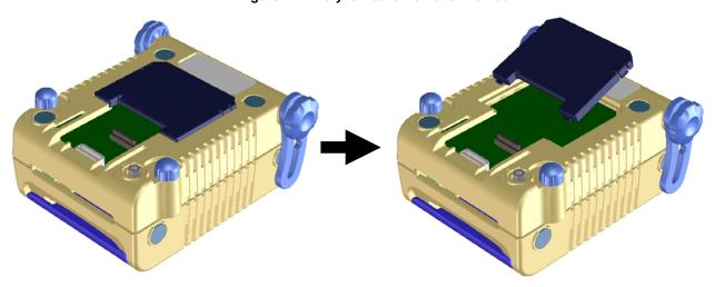
Figure 2-2. Acrylic Board Removal Method
