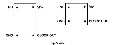
Figure 2-4. Mapping of Oscillator to Socket
