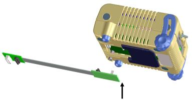
Insert CN1 and CN2 of the probe into TCN1 and TCN2 of the QB-78F1026.
