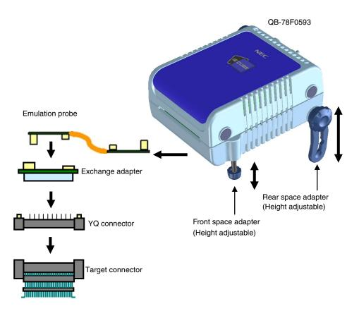
Figure 2-8. Connection Using Emulation Probe
