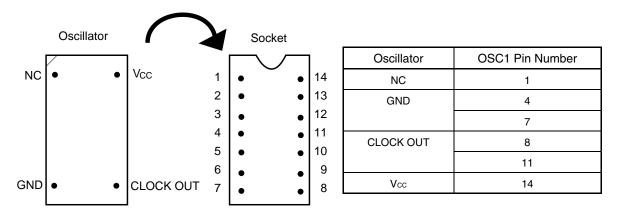
Remark Insert the oscillator into the socket, take care for the pin 1 position.
