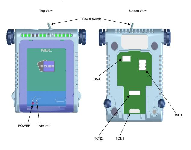
Figure 2-1. Names of Parts of QB-78F0593
