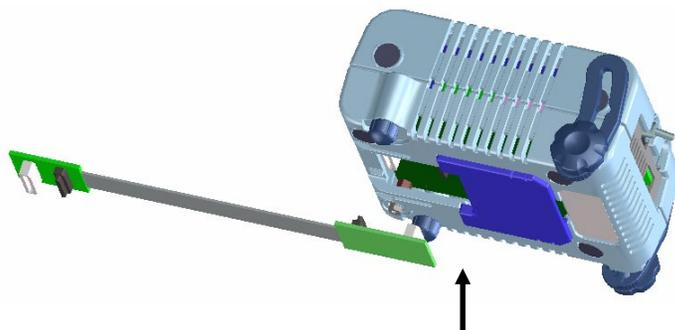
Insert CN1 and CN2 of the probe into TCN1 and TCN2 of the QB-780731.
