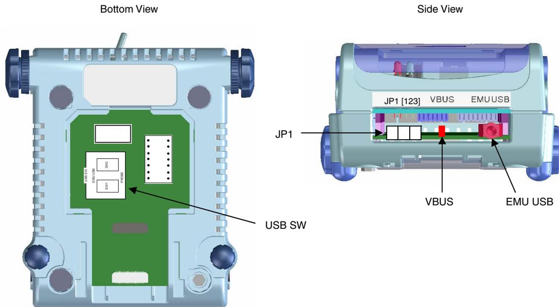
**Caution** When the USB connector on the target system is used, the difference in electrical characteristics from those of the actual device increase from when the USB connector (EMU USB) on the QB-780731 is used.
