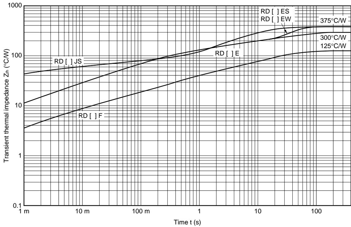
**Figure 21. Transient Thermal Impedance Characteristics<sup>Note</sup>**
