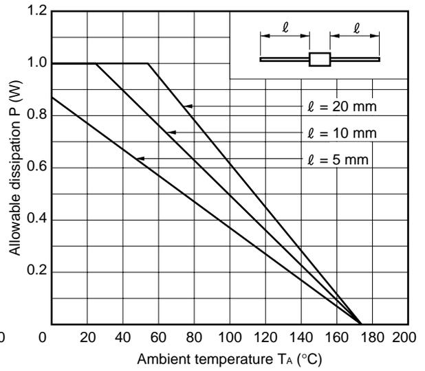
Figure 9. S - R<sub>th</sub> Characteristic Example (NNCD [ JB])
