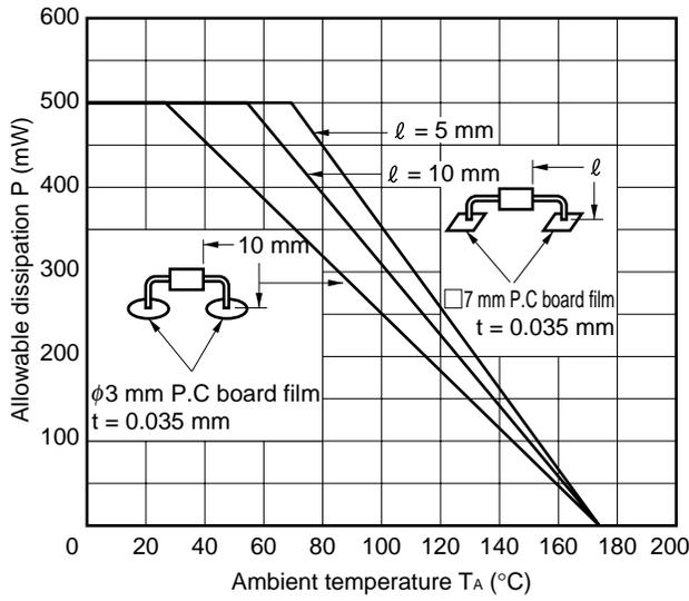
Figure 8. P - T<sub>A</sub> Rating (RD [ JF])
