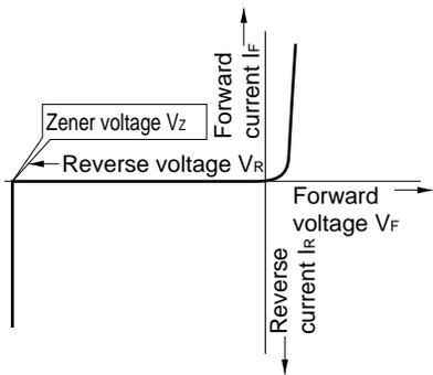
Figure 2.  $V_z - \gamma_z$  Characteristics Example
