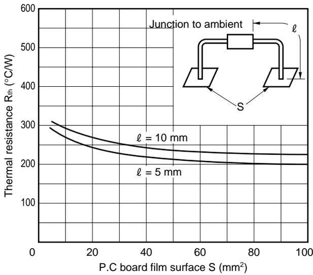
**Figure 6. Example of S -  $R_{th}$  Characteristics (RD[ ]F)**
