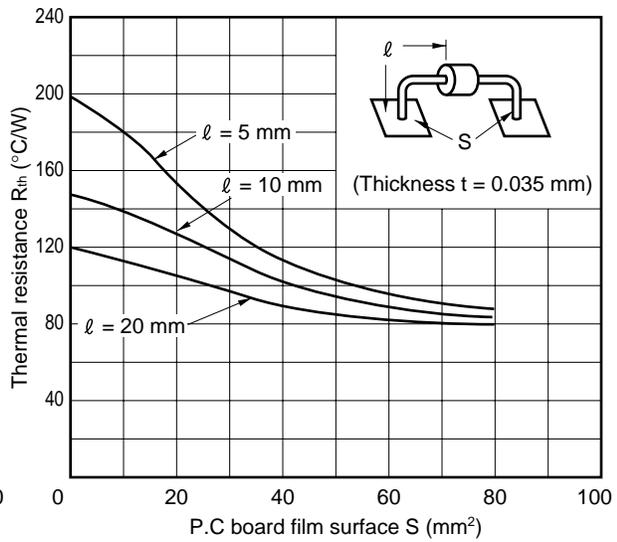
The heat radiation can be improved by increasing the surface size of the copper film on the printed wiring board. Attention must also be paid to the fact that the lead wire diameters for RD[ ]E and RD[ ]F are different, being respectively 0.5 mm and 0.8 mm. Their heat radiation efficiency also differs; The lead length should be shorter for RD[ ]E, and longer for RD[ ]F to make heat radiation more efficient. Thus the P -  $T_A$  rating can be improved as shown in Figure 7 and Figure 8.
