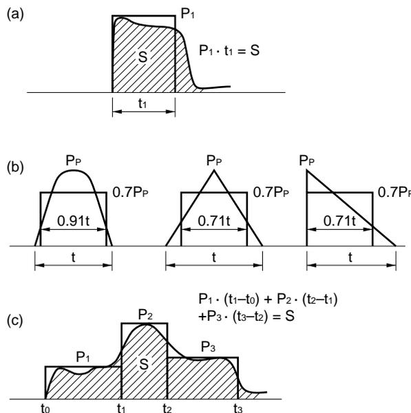
**Figure 19. Junction Temperature Rise for Triangular Power Consumption**
