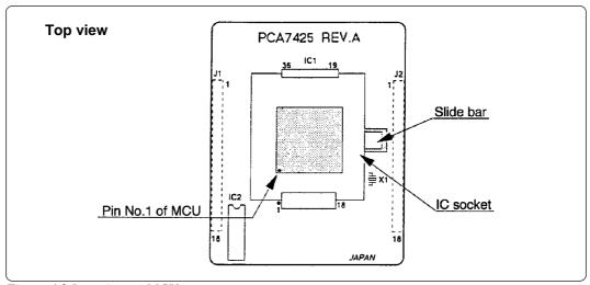
Figure 4.2 Inserting an MCU
