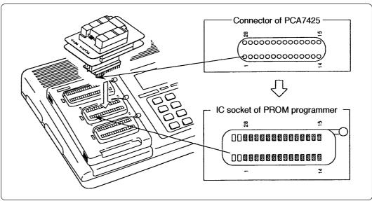
Figure 4.1 Attaching the adapter to a PROM programmer
