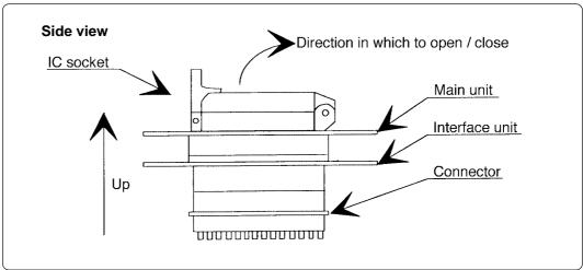
Figure 4.3 Opening and closing the IC socket
