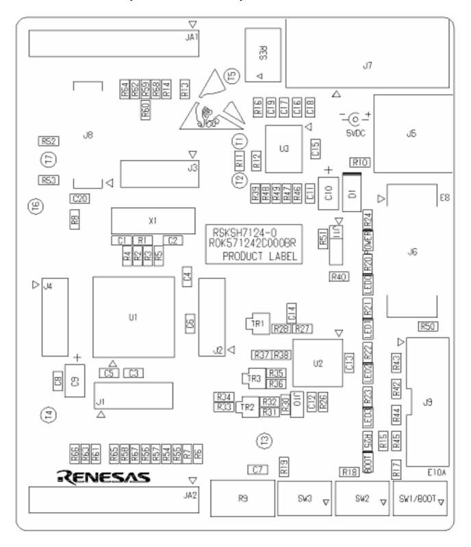
Figure 11-1: Component Placement
