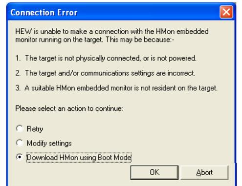
HMon will program the device in Boot mode and then swap back to User mode. A debug connection will then be attempted. If the connection fails the "Connection Error" dialog will be re-displayed.
